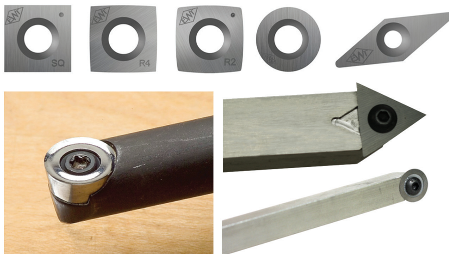
Round cutters make concave cuts, square ones shape convex cuts, and triangles do detailing.
