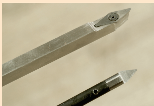
2 The tool shafts (between the cutting tip and the handle) can be square or round.
