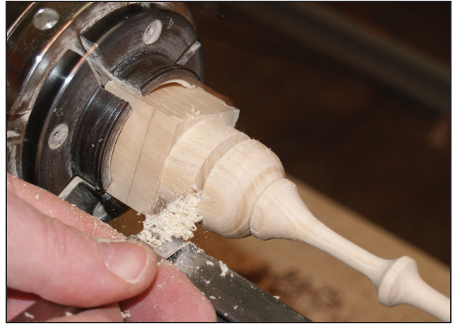
17 The detailer (pointed cutter) is used to define the bottom of the finial, and cut it loose.
