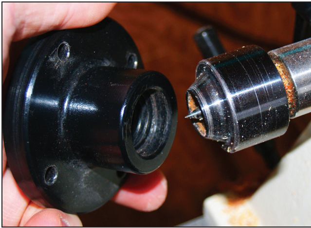
13 The cone on most live centers will fit perfectly in the opening of a 1"-8 TPI faceplate.
