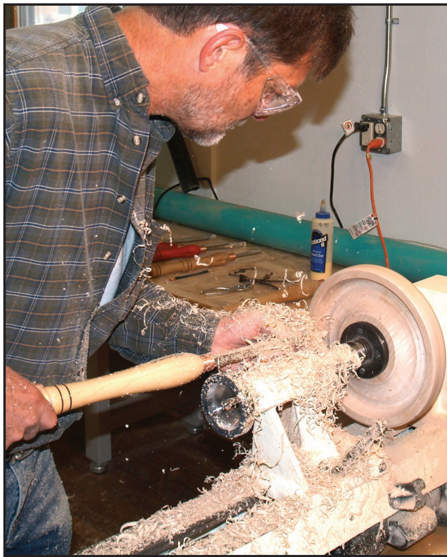
Tools with flat-topped carbide cutters such as EWT’s round Finisher are held parallel to the floor.
