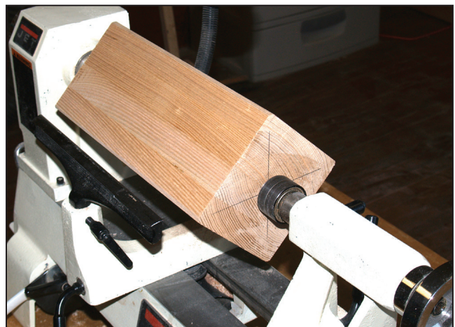
1 Long-grain vessels can begin with a glued-up blank (shown) or a solid piece of stock.
