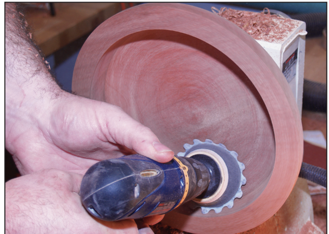
7 With the work spinning slowly on the lathe, a disc sander in a portable drill sands the inside.
