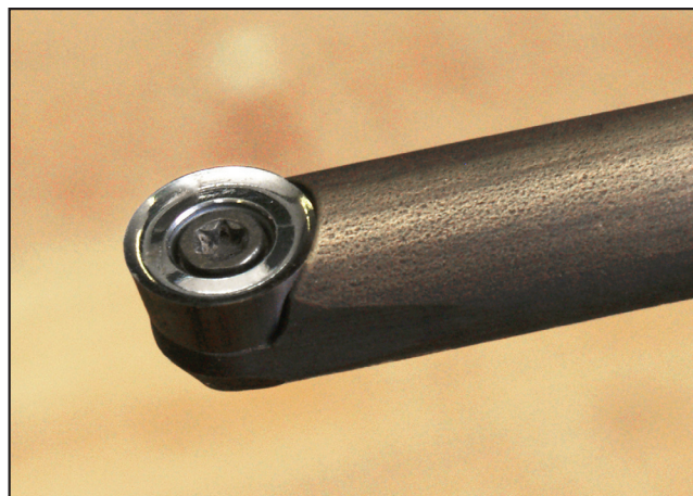
13 Mike Hunter's system is based on a high quality, saucer-shaped carbide cutter.
