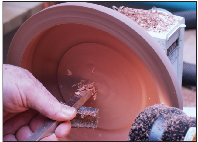
6 A square rougher is used to flatten and clean the bottom of the lower half of the orb.
