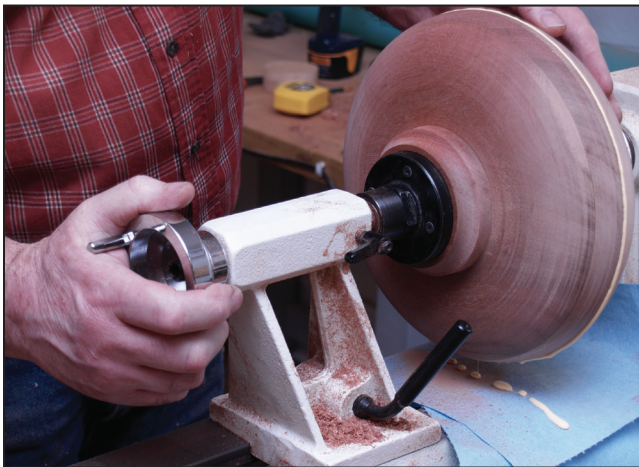
15 Crank the tailstock enough to achieve a nice, tight seal all the way around, but not too tight.
