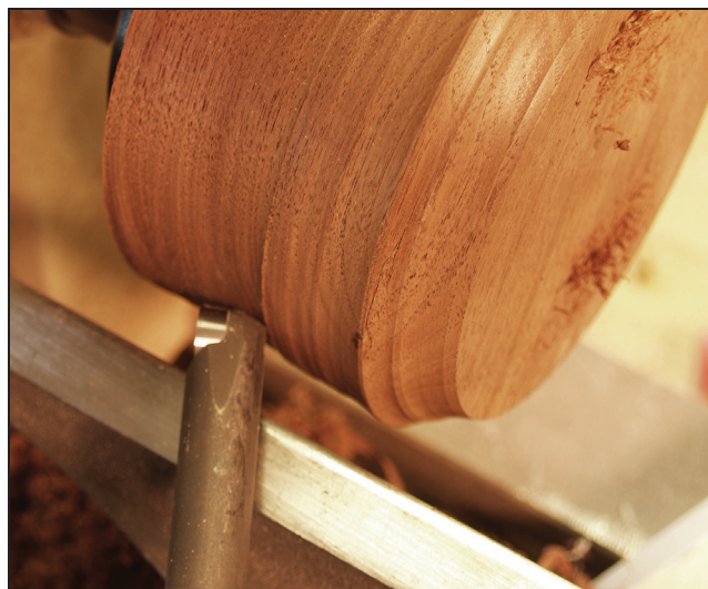
17 With saucer-shaped cutters, begin with the bevel under the cutter parallel to the wood.
