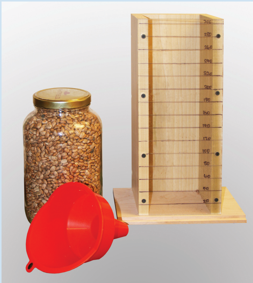
The jig shown uses beans from the grocery store to measure the volume of hollow vessels.
