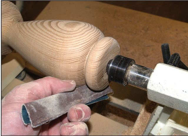
18 Re-engage the tailstock, increase the speed, and sand the outside down through the grits.
