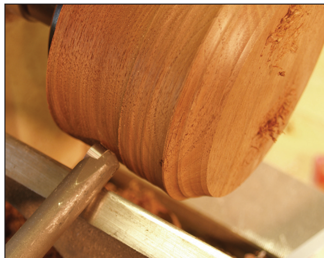
18 Without rotating it, the handle is moved to the left until the cutter makes contact.
