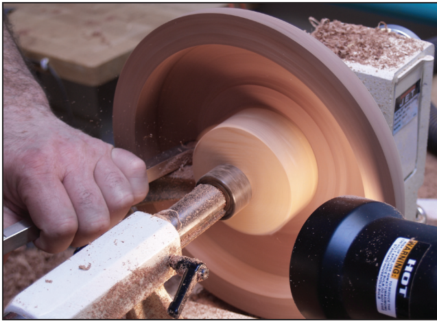
5 With the blank mounted on a faceplate, hollow the inside. Note the tailstock jam block.
