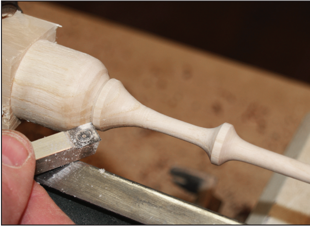
16 Rabbits, shallow grooves and outside curves, all cut with a square tool, add texture.
