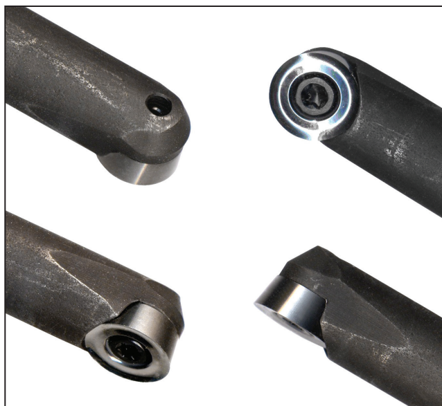
14 These four views of the same Hunter cutter also show the bevel on the bottom of the tool.
