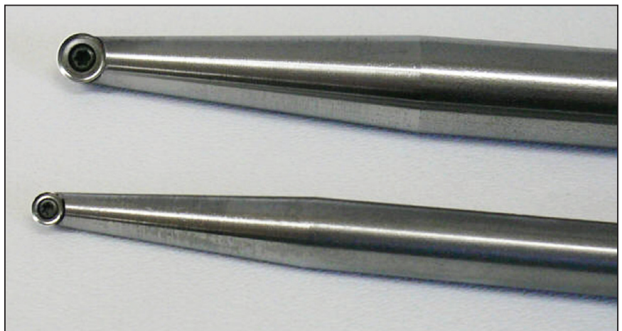
18 The standard Eliminator has a \frac{3}{8} " cutter, and the Mini Eliminator's insert is \frac{1}{4} " diameter.
