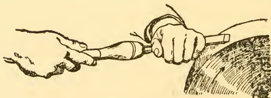
FIG. 34.—GRINDING THE TURNING CHISEL.
