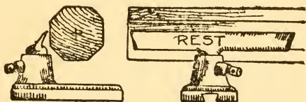
FIG. 9.—POSITION OF REST AND WOOD.
