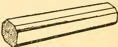
FIG. 6.—PIECE OF WOOD WITH CORNERS ROUGHLY PLANED AWAY READY FOR MOUNTING BETWEEN THE LATHE CENTRES.
