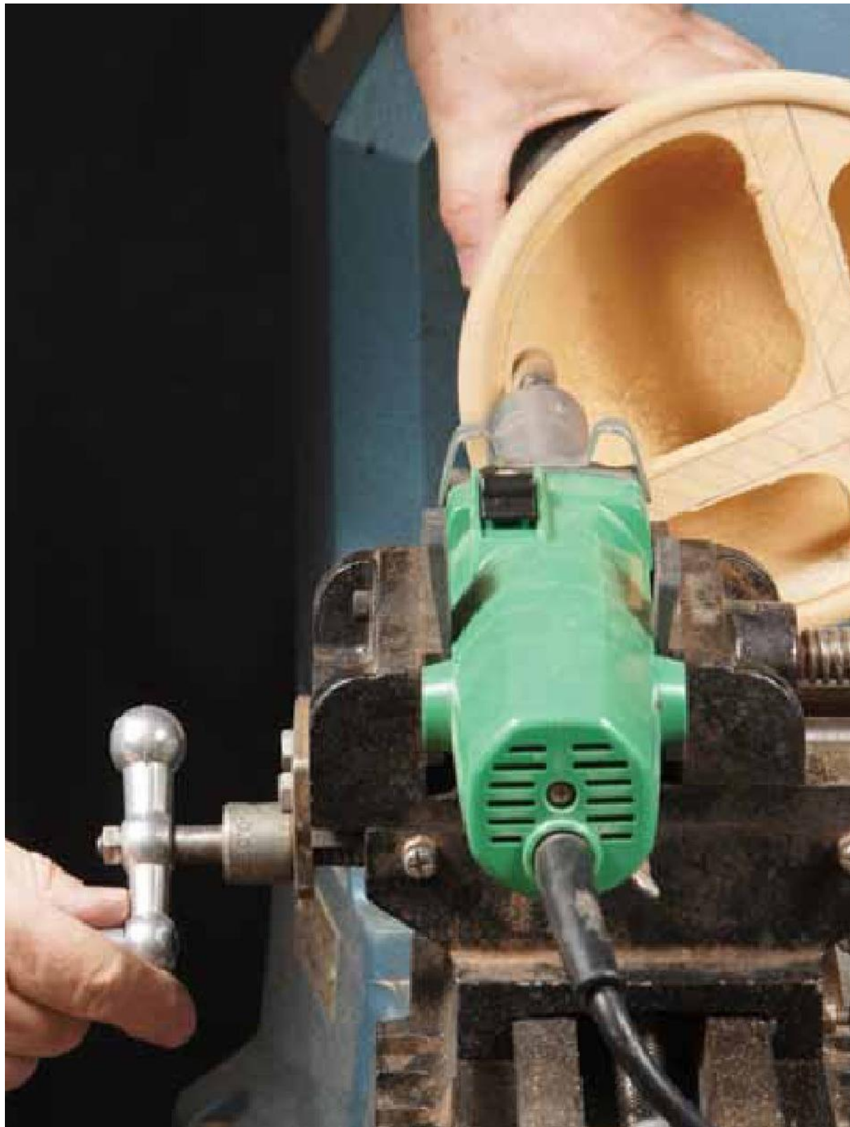
6-16 Blending the interior wall.
