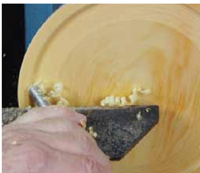
ABOVE 6-1 The bowl mounted in the chuck after the outside is finished.
