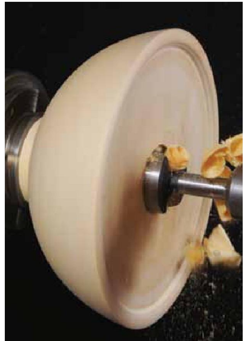
BELOW 6-5 Drilling out the depth.
