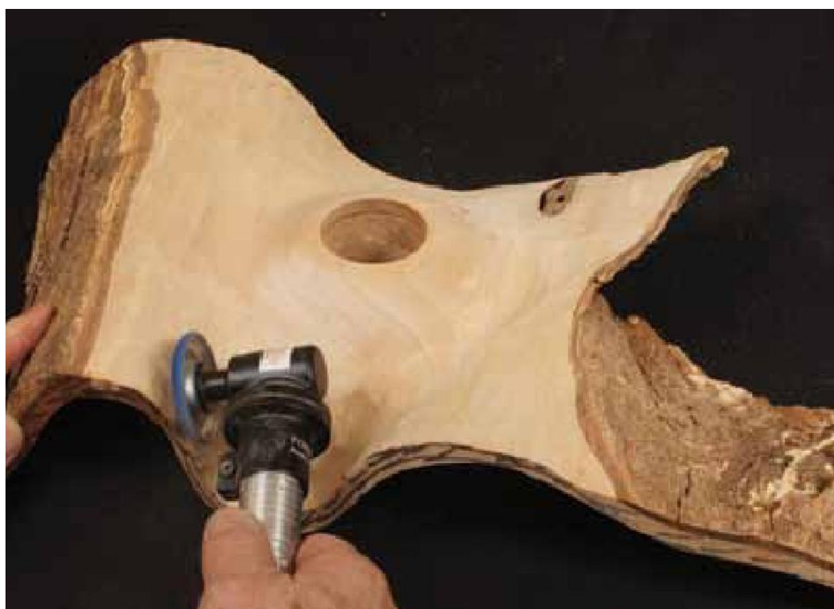
15-4 Refining the curves with the Foredom flexi-shaft tool. I am following the curve we marked on the base. The piece has not yet been hollowed.
