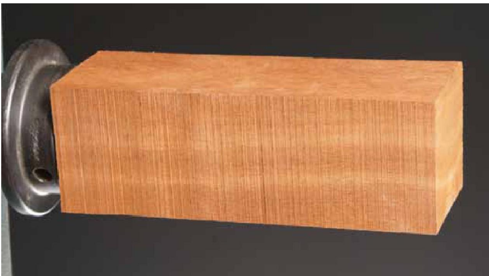
9-1 The rectangular blank on the screw chuck.
