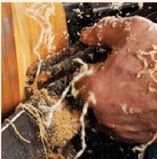
Cut A: the tool is held in a flattish position and the cutting edge is at about 20 degrees to the wood as it comes down onto the tool. Note how the shavings are turned back upon themselves by the flute in the tool.
