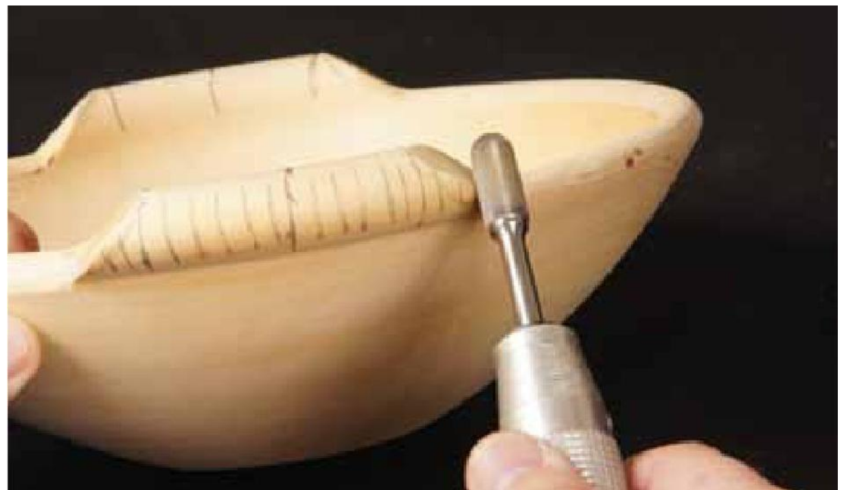
ABOVE 3-7 Transferring the depth mark to the opposite side.
