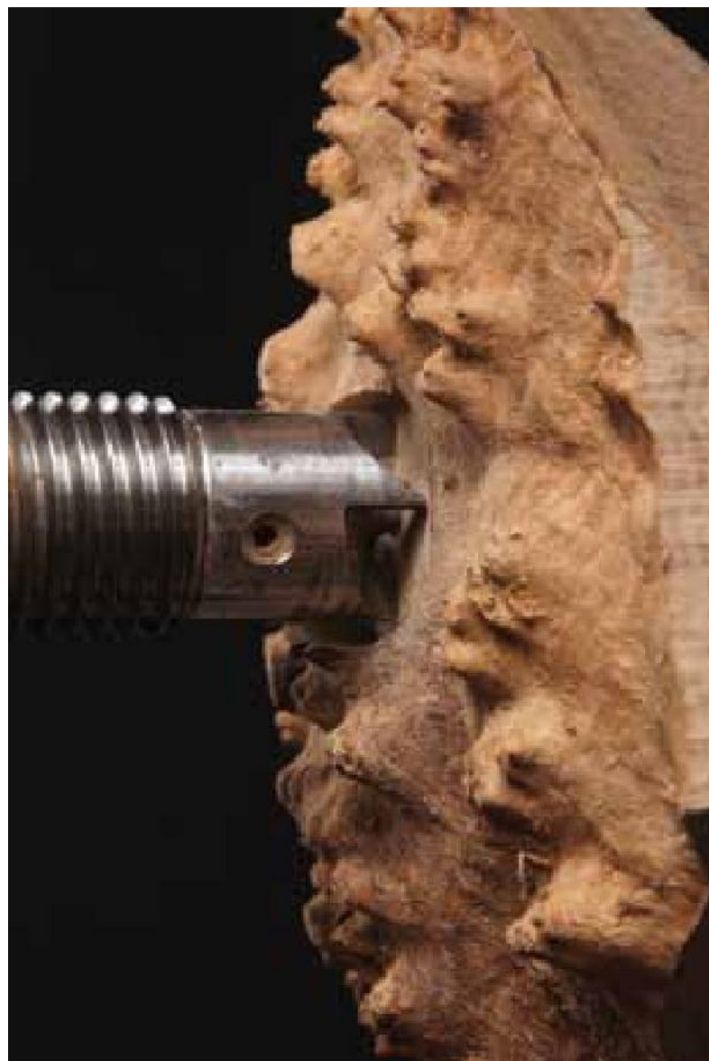
4-1 The rough surface of the blank is drilled away to give good contact with the drive dog teeth.
