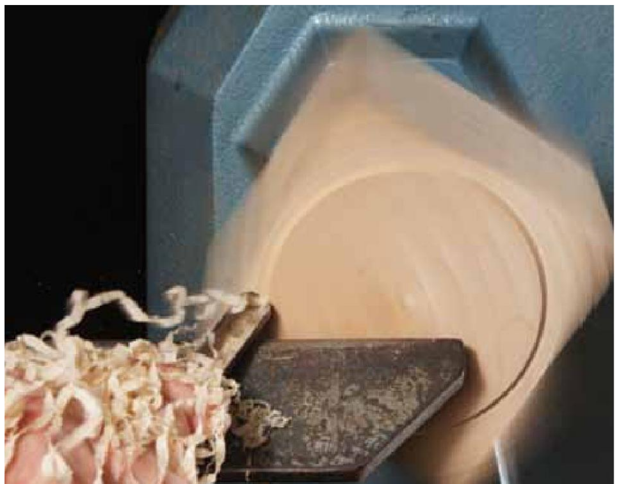
8-1 Turning the spigot on the base of the box.
