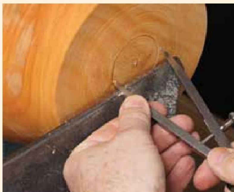
SB3-2 Transferring the internal diameter of the jaws to the blank. This is not the same wood as the handled bowl.
