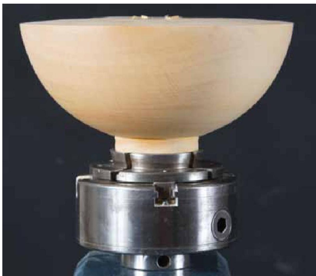
ABOVE 6-1 The bowl mounted in the chuck after the outside is finished.
