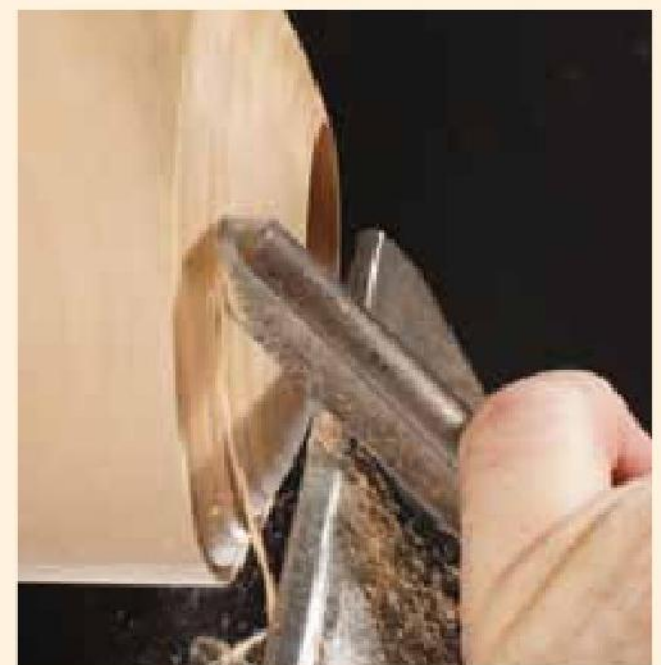
Cut C: I have rolled the tool “on its back” and the edge is presented to the wood at almost zero degrees. The wood is sliced very cleanly, falling away below the cut in an unbroken ribbon.
