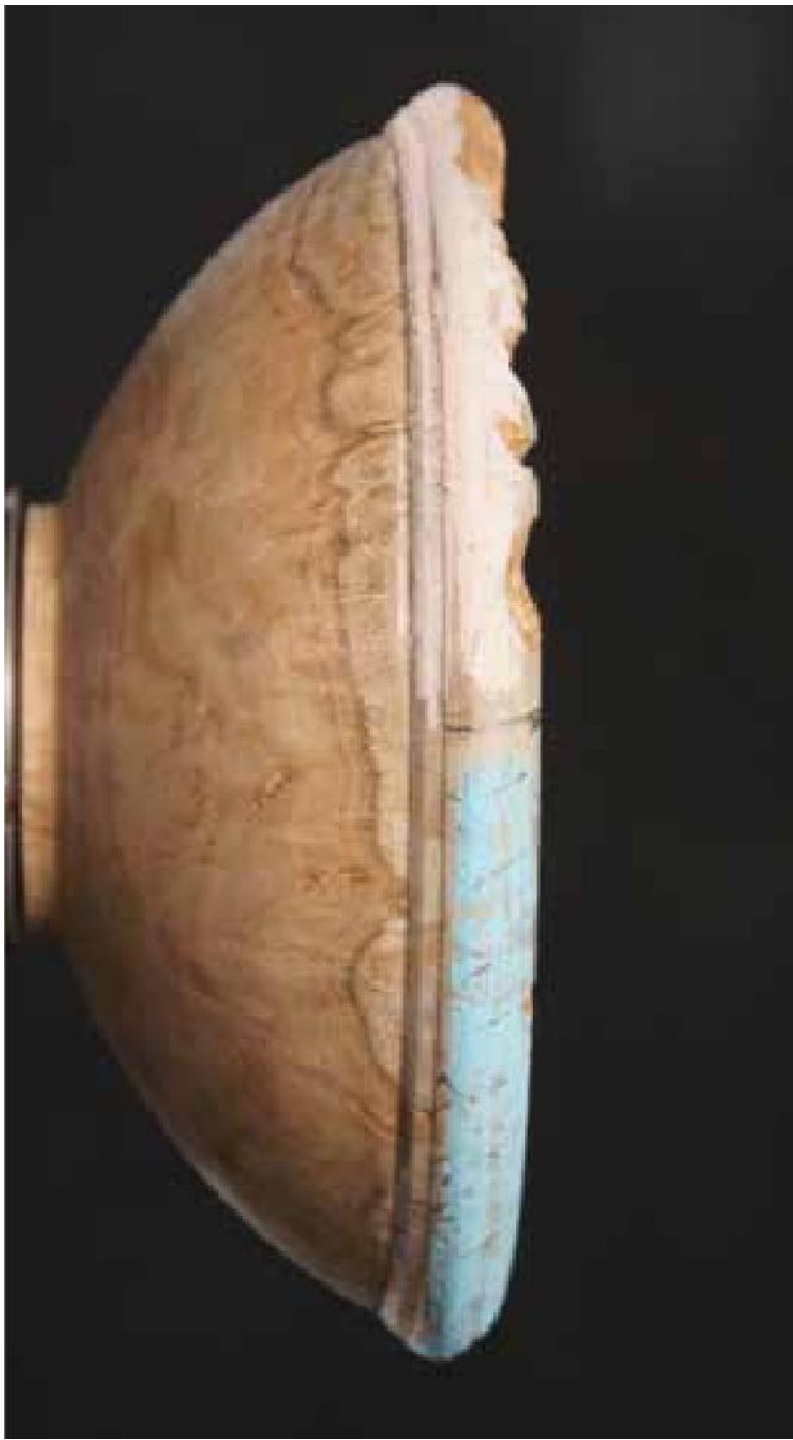
4-4 The turning is finished and the part of the rim to be removed is marked out with pink chalk.
