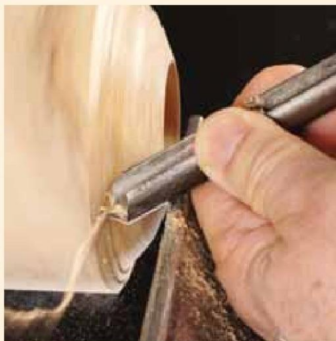
Cut B: by raising the handle, the angle between the wood and edge is decreased and the shavings can exit without hitting the flute.
