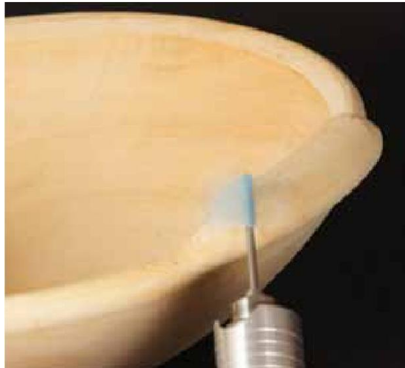
ABOVE 3-10 The butterfly split-pin sanding system.
