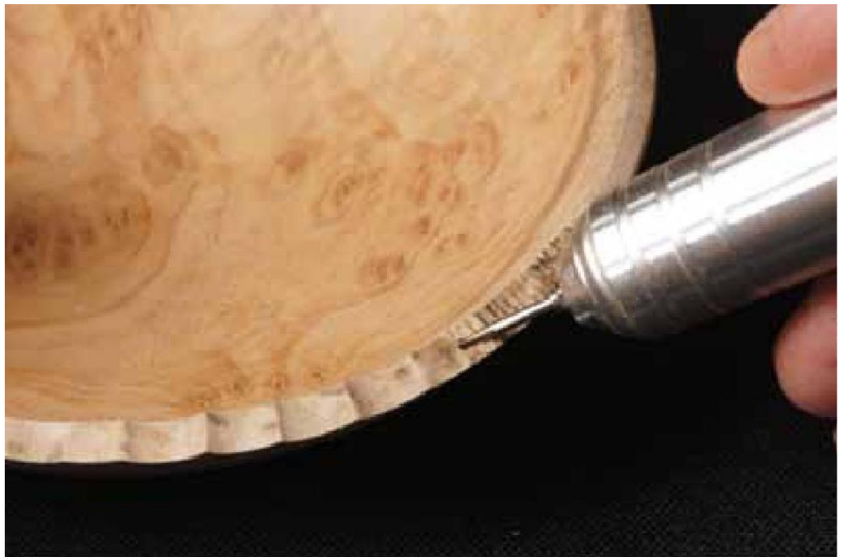
TOP 4-5 Removing the unwanted rim.
