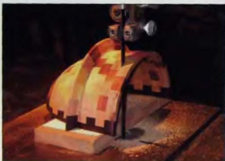
13-04 To maintain this particular pattern, one layer is removed from one side.
