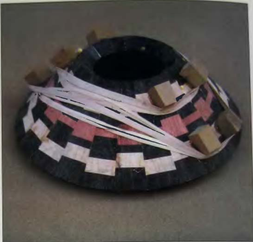
16-11 The last gluing step uses rubber bands anchored by little hot-glued blocks of MDF.
