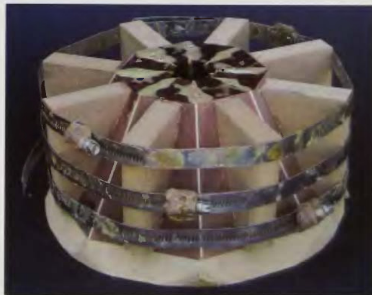
10-23 Glue blocks can also be used to assemble staves.
