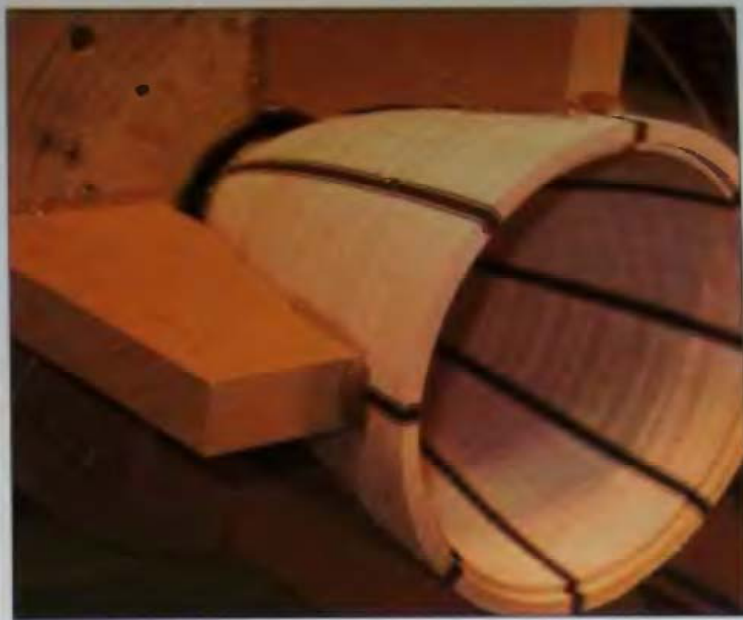
10-17 In lieu of a steady rest, braces can provide stability.
