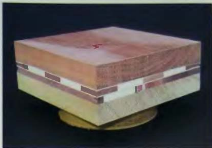
15-01 This is a six-layer laminated segment containing a mosaic Indian face design.
