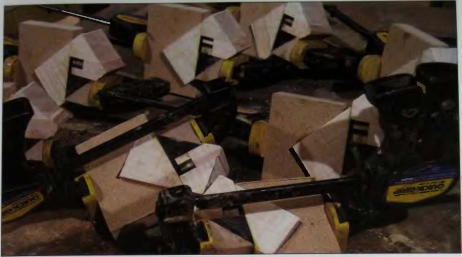
6-03 Gluing cauls enable pressure to be applied in the right direction.
