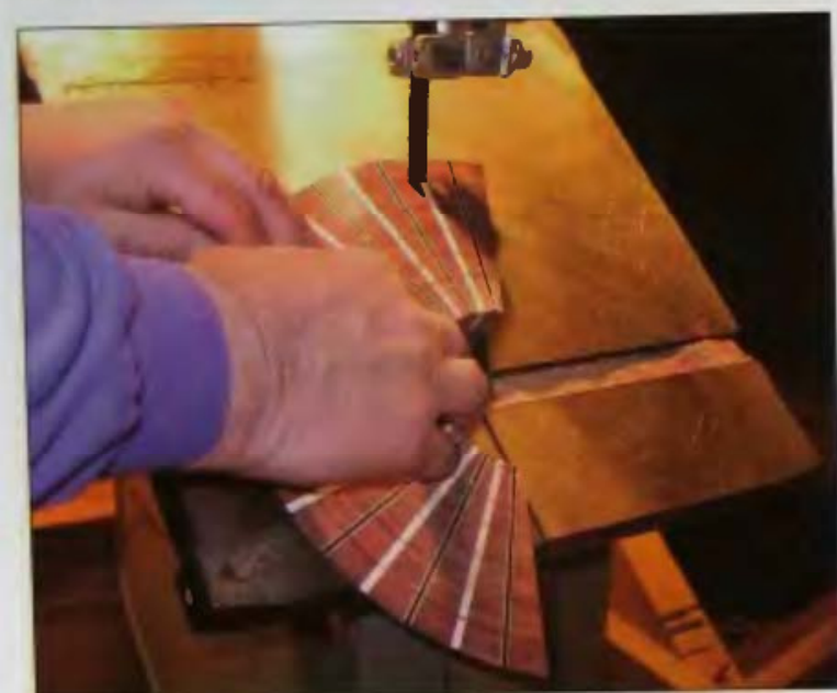
11-47 Cut carefully: the whole project depends upon following the lines.
