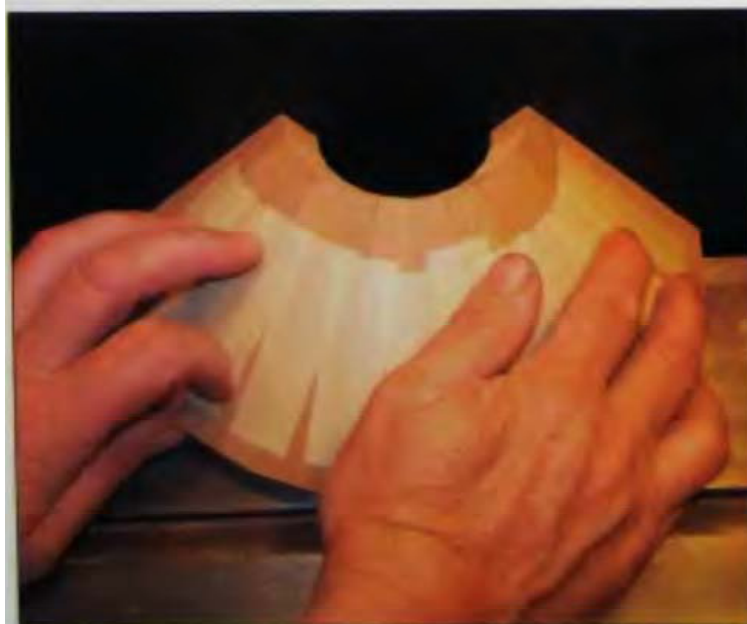
16-05 Test fitting and adjusting saw settings can take some time.
