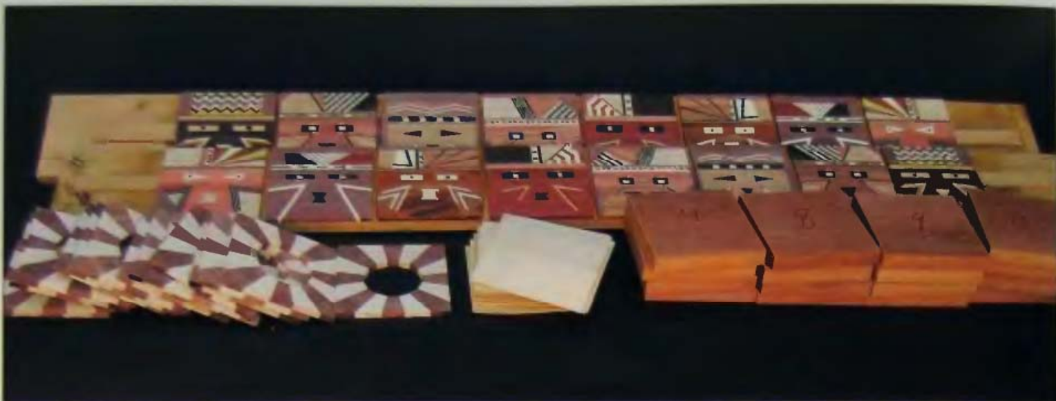
15-02 These are all the components that compose the laminated segment.
