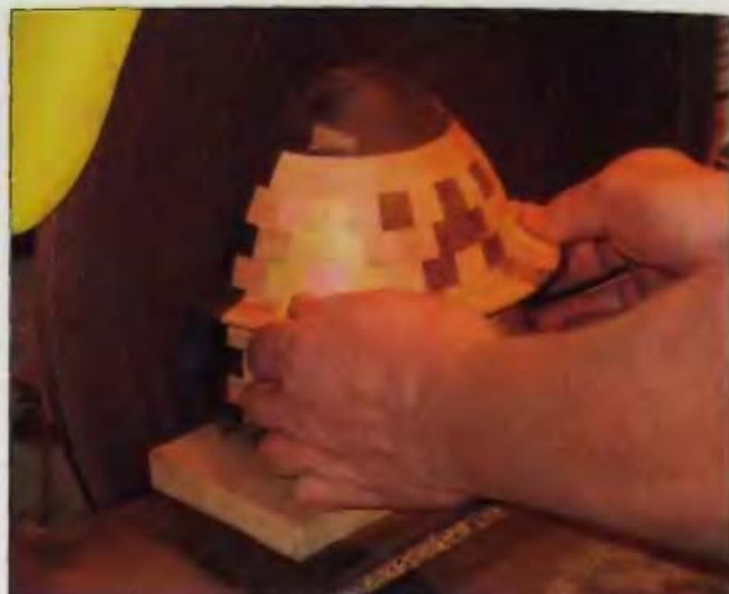
13-03 The cuts on the half-sections can be disc-sanded while still attached to the board.
