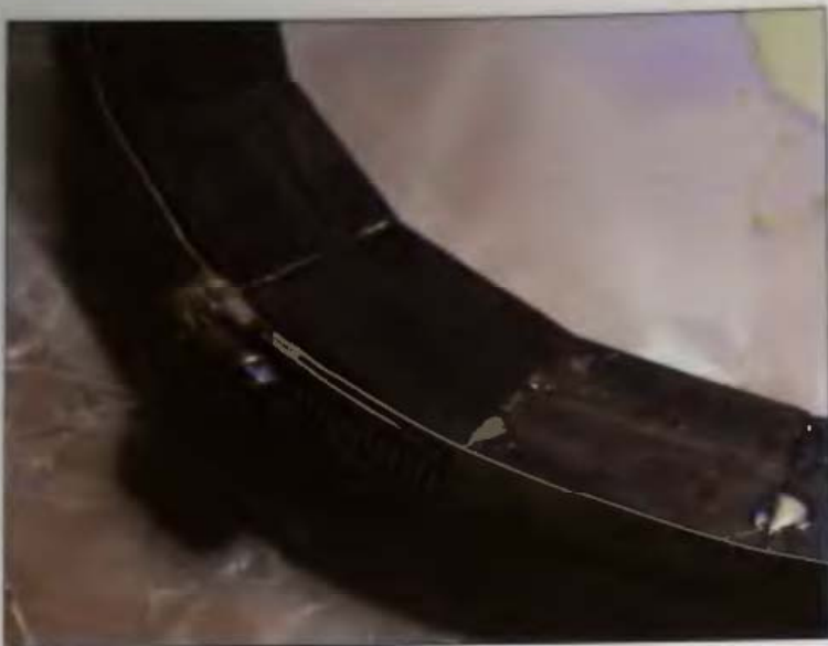
7-21 Gluing a full ring at one time requires perfect miters and extreme care.
