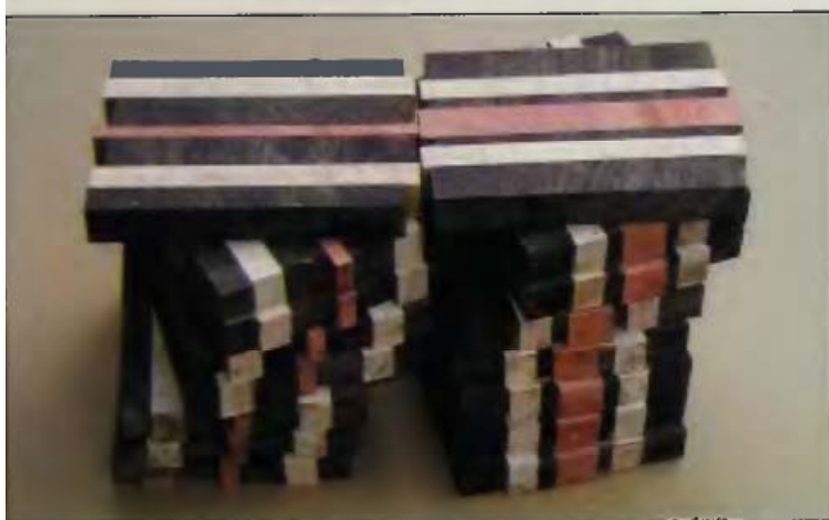
16-04 To accurately cut staves, the laminations must be smooth and consistent.
