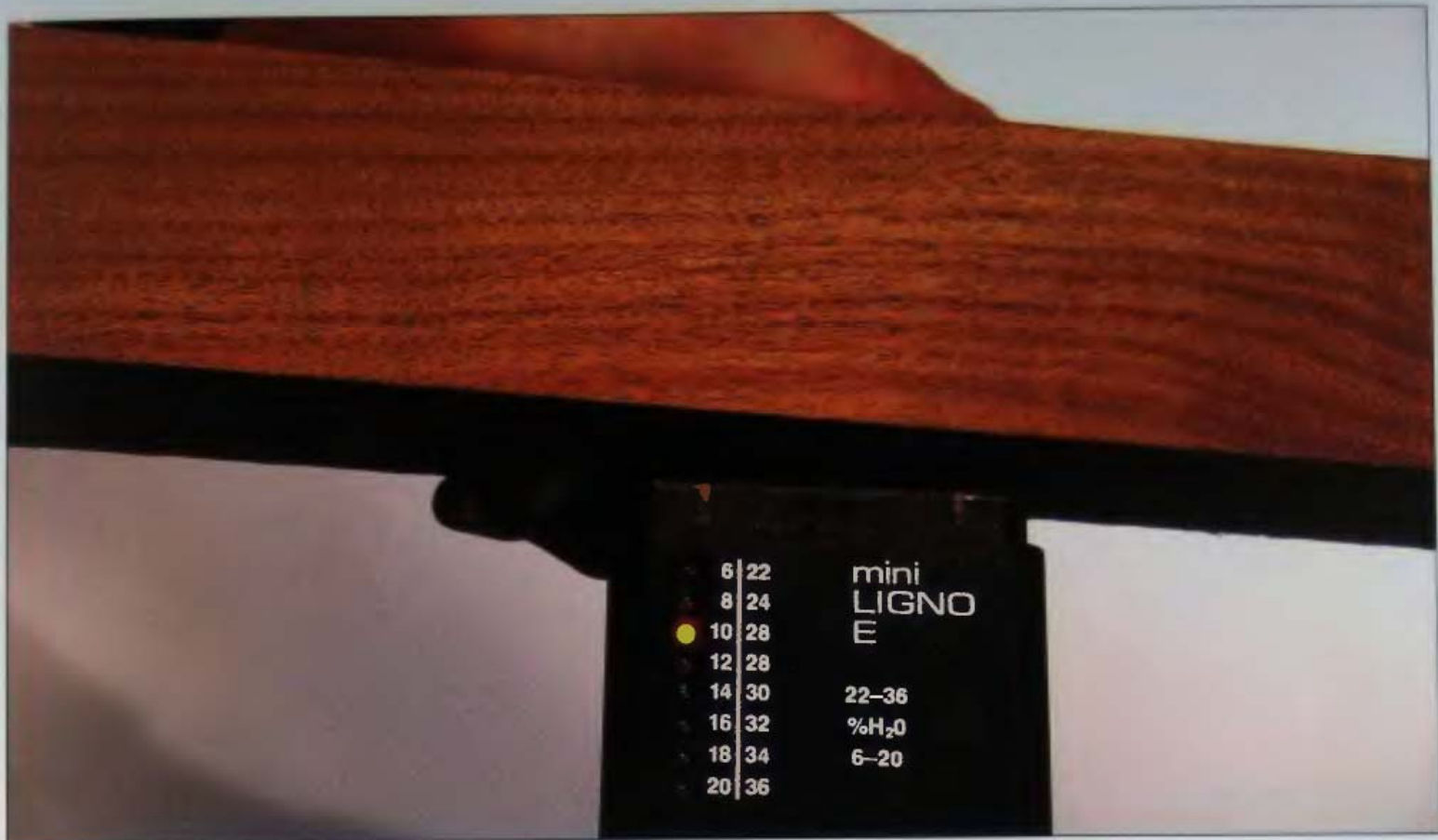
5-02 Wood must be tested for moisture content.
