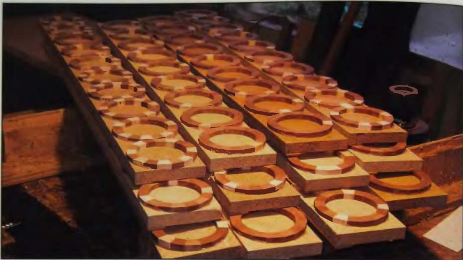
13-08 Rings are tapered using a drum sander and transport trays with a shim under one edge.
