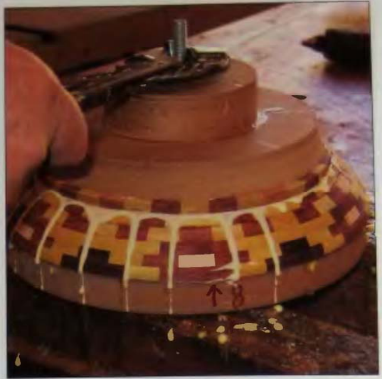
7-33 A centered bolt and nut works well for clamping small rings.
