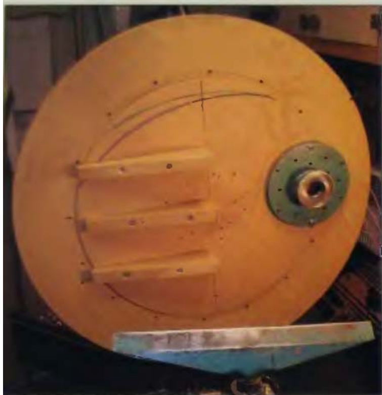
13-17 Off-center turning requires a large counter-balanced disc.
