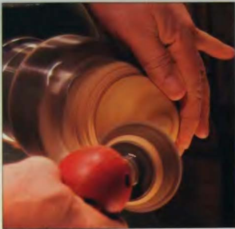
14-23 A small jam-chuck (and fingers) holds the spheres during sanding.
