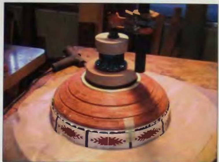
9-27 Masking tape can be being used as a positioning aid.
