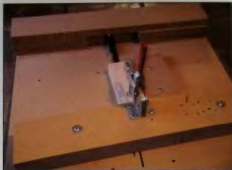
10-03 A table saw sled is used to cut compound miters.
