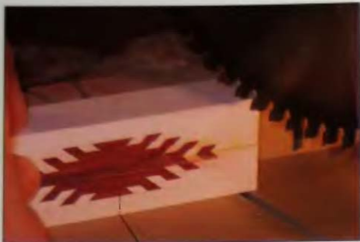
9-15 The miter saw is used to create segments from the glued assemblies.
