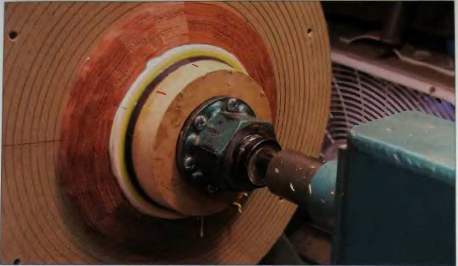
7-30 Using your lathe's tailstock works well for centering and clamping.
