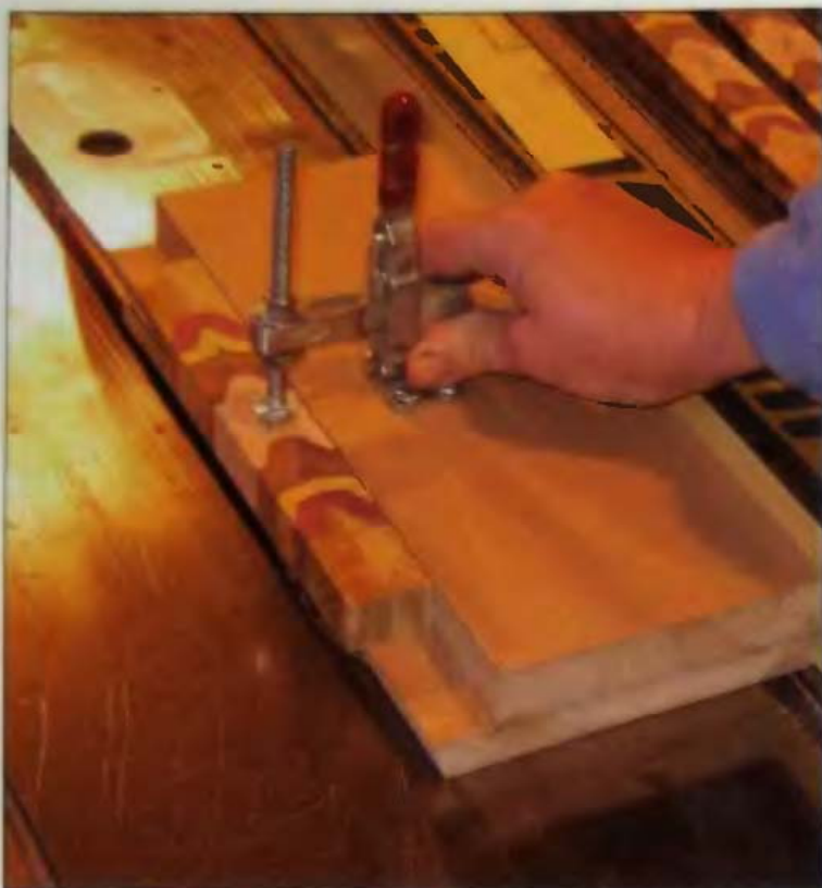
11-16 A simple sled enables safe and accurate trimming of small strips.
