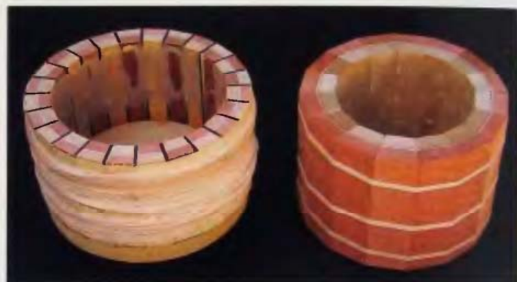
11-32 Two cylinders, constructed differently from the same laminated strips.
