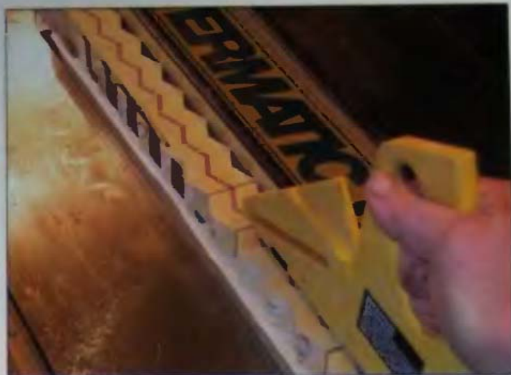
11-06 The table saw makes short work of creating rectangular segments.
