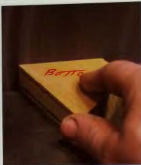
7-07 Freehand disc sanding (second step).
