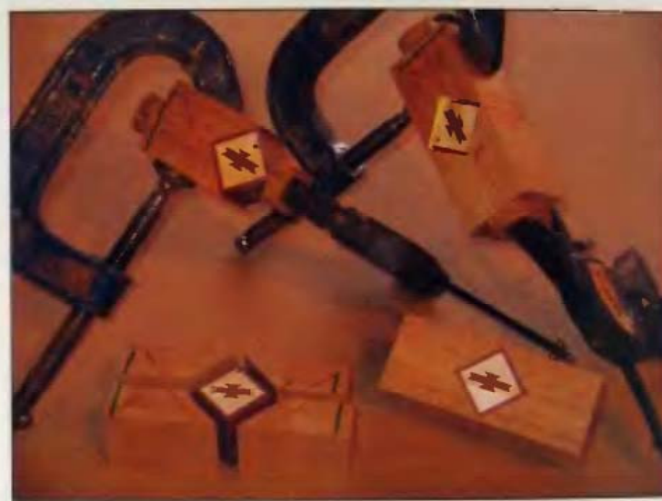
15-27 Follow the gluing steps clockwise, starting from the lower left.
