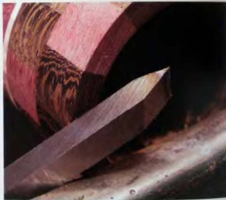
7-27 This diamond-point tool is versatile, quickly resharpened, and does a great job on MDF.
