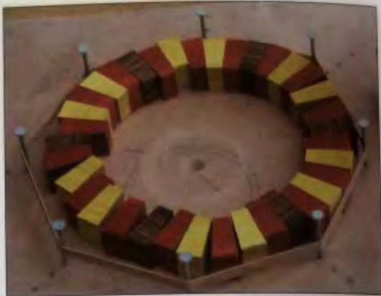
7-22 A rubber band gluing jig is just a board with small holes and nails.
