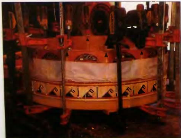
15-20 When spring clamps are too small, bar clamps can be used.
