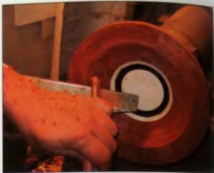
9-23 Initially, keep the vessel walls at maximum thickness.
