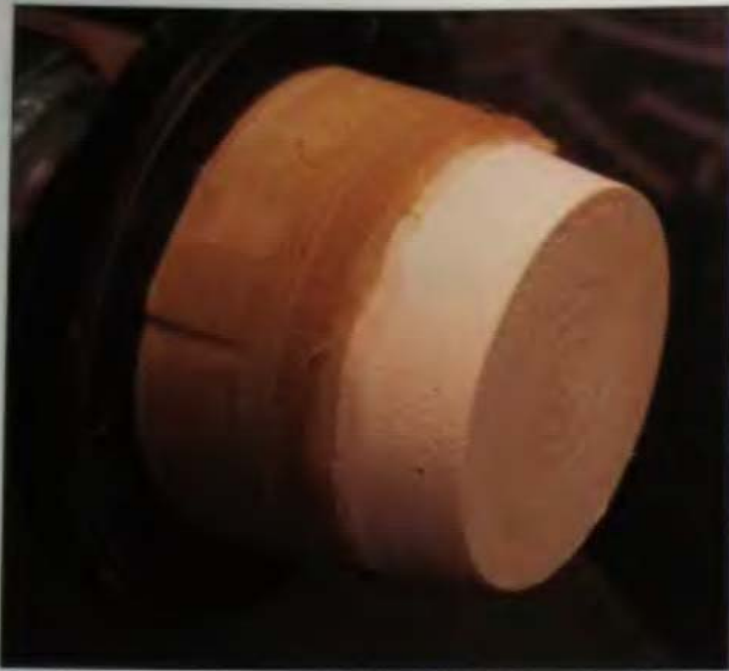
7-38 Small plugs can be used in vessel bases.
