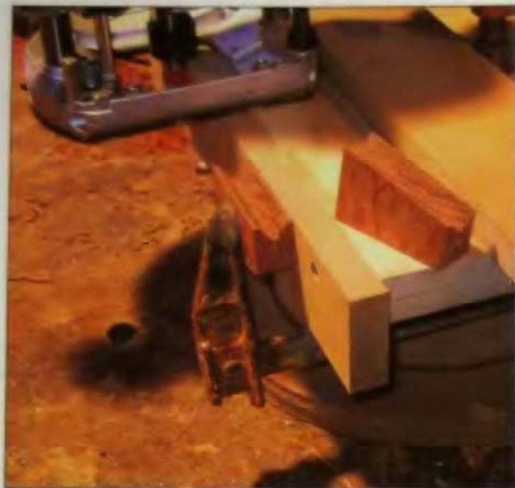
11-23 Firmly clamp the segment before cutting the notch.
