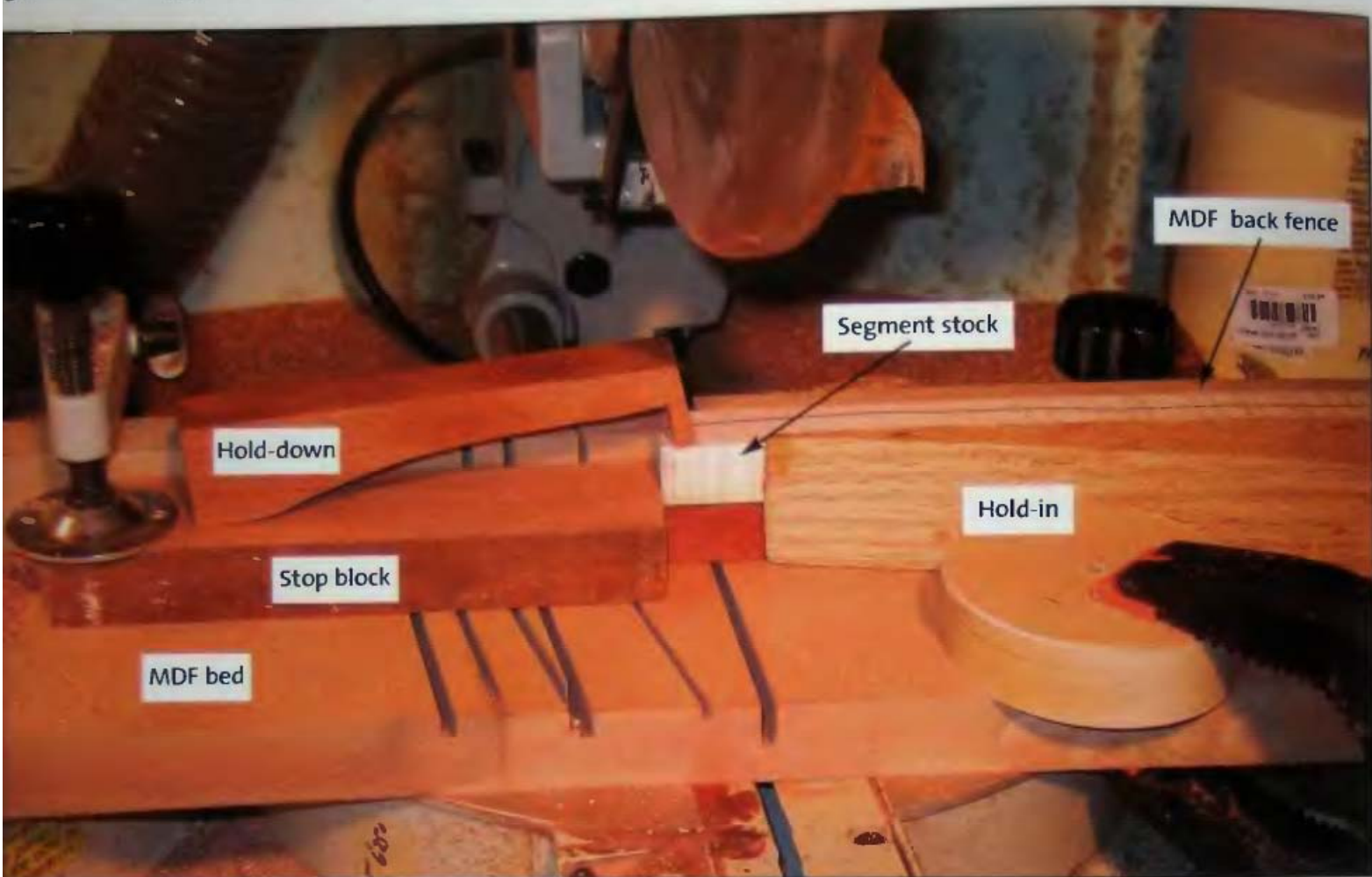
7-01 This miter-saw setup is how I cut most of my segments. Note the hold-down device.
