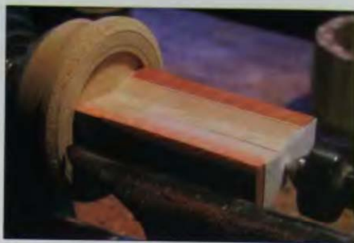
11-33 Staves can be turned two at a time, with a spacer in between.
