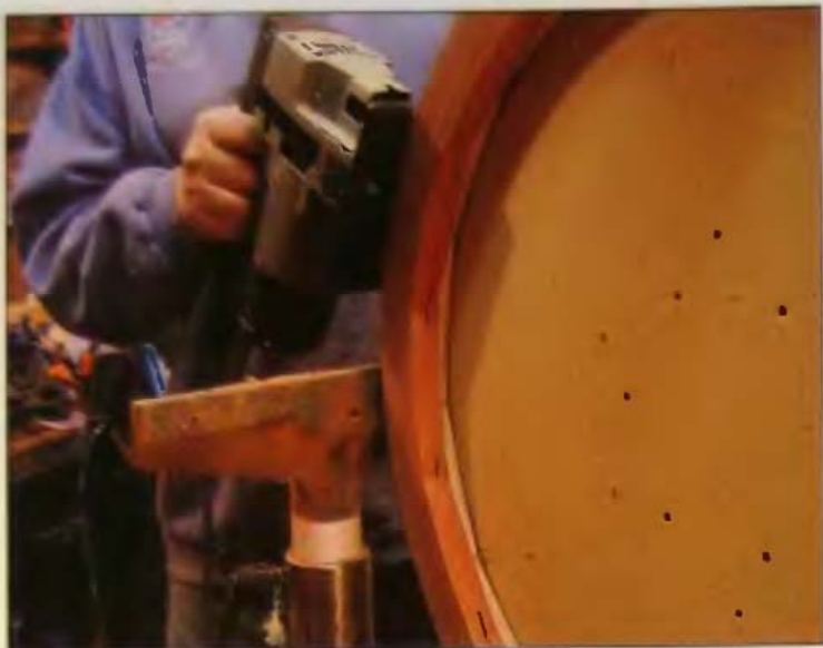
15-16 Notice the small slots where the parting tool cut through at the glue joints.
