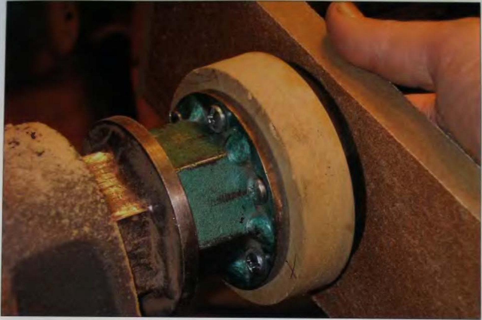
7-28 Using a flat sanding block is the final step prior to gluing the next ring.
