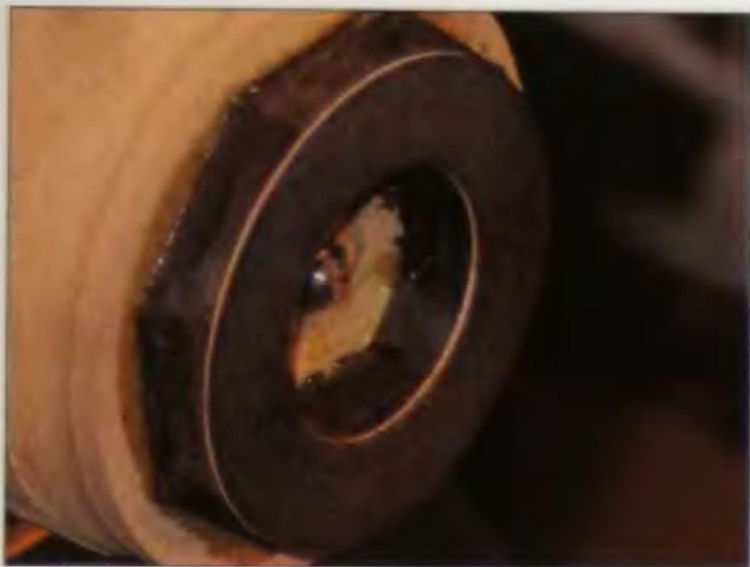
10-18 Veneer layers are added to the vessel top.
