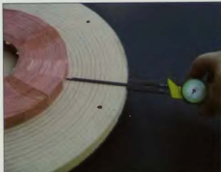
9-21 Precise centering of rings is important.
