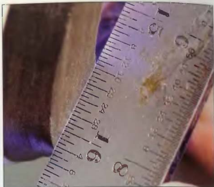
7-25 Checking for flatness requires a good quality straight edge..
