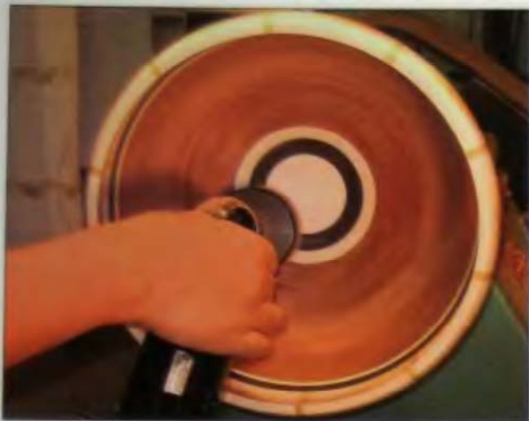
9-28 Finish-sand the inside prior to joining the two halves.
