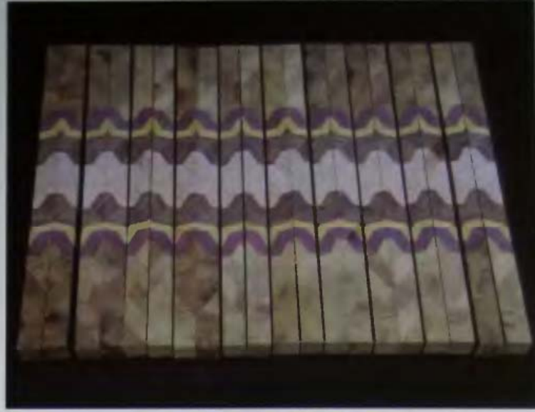
11-15 A new pattern emerges as a result of another series of cuts.
