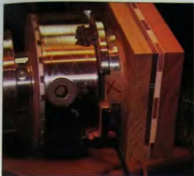
15-04 The circle of MDF is attached with hot-melt glue.
