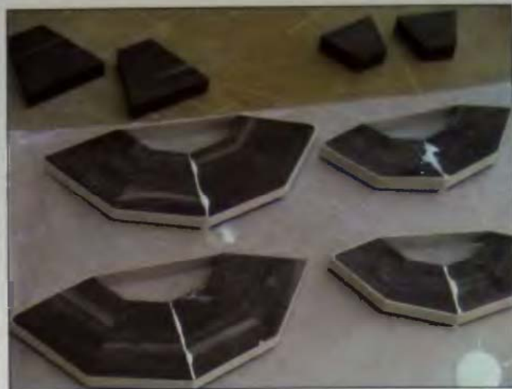
9-19 Construction starts with both top and bottom ebony rings.
