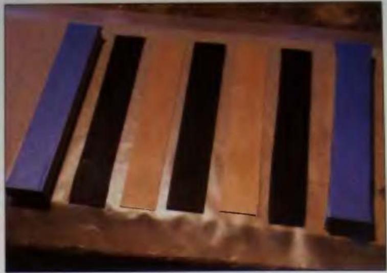
10-06 The splines are a five-layer lamination.
