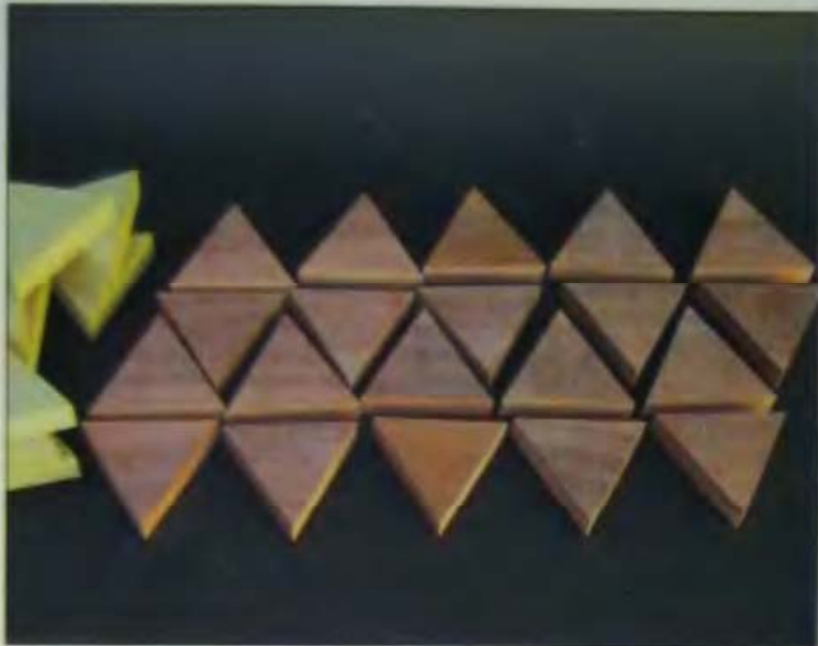
14-05 An icosahedron is composed of 20 mitered triangles.
