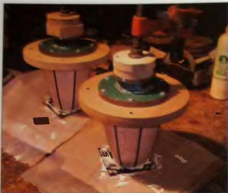
10-14 Veneer layers are added, with the clamps pressed against the ceiling..
