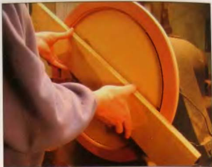
15-17 Sanding blocks must be very straight and flat.
