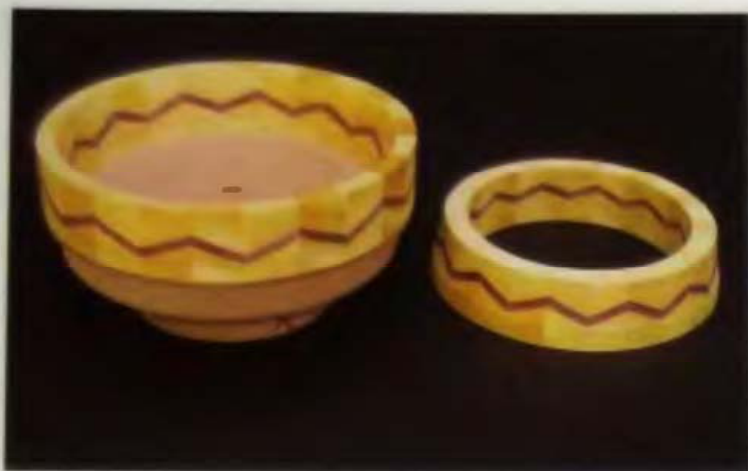
11-09 The use of a parting tool creates a two-for-one opportunity.
