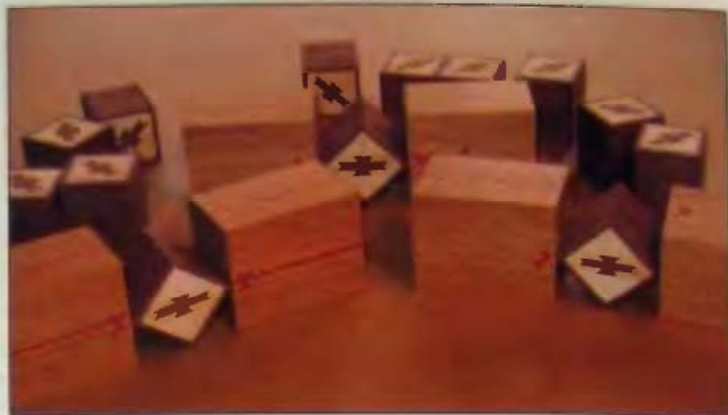
15-26 Almost invisible glue lines are a result of maintaining grain orientation.
