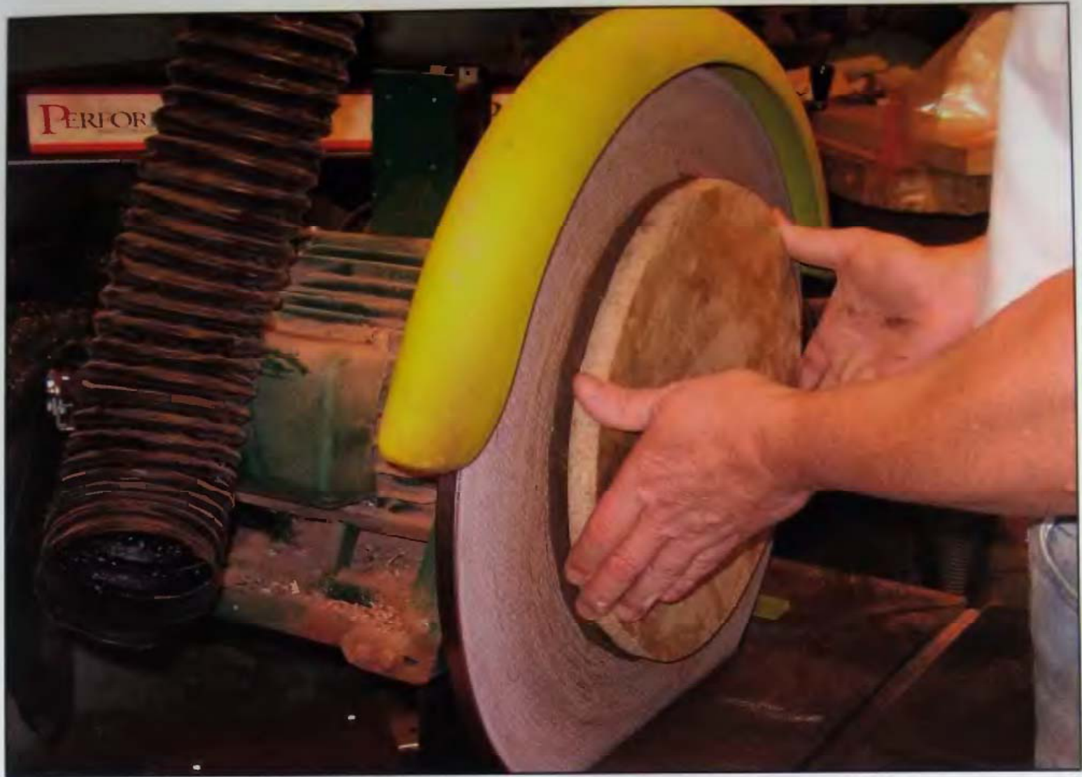
7-23 A disc sander can be used to flatten one side of a ring.
