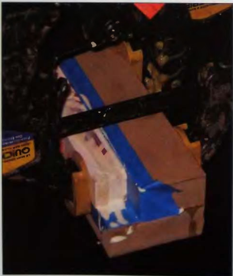
9-11 A gluing tray is used to assemble the thin strips.
