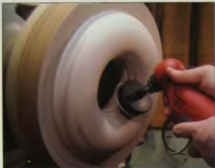
13-12 A large jam-chuck provides access to the inner surface.
