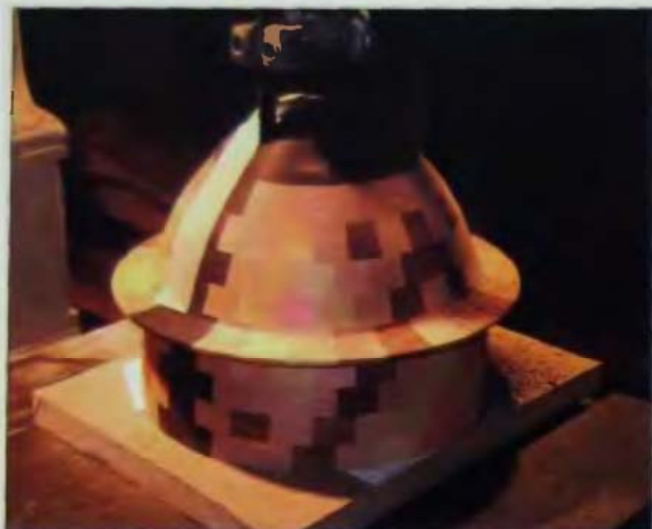
13-02 Mounting the bowl on a flat board provides stability during cutting.
