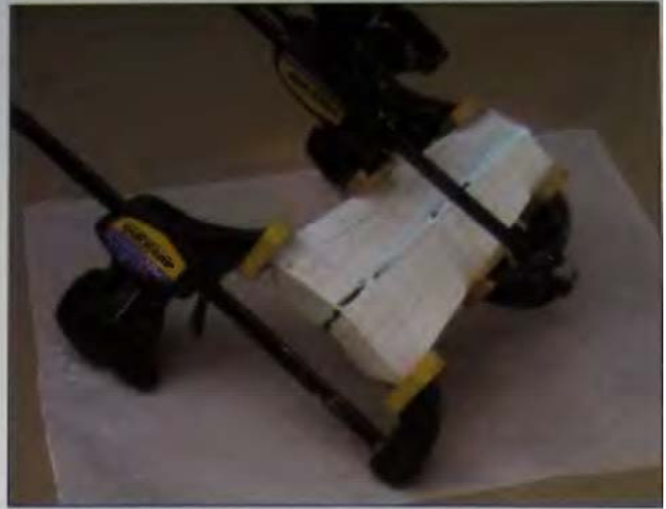
10-11 This is another method of joining staves.
