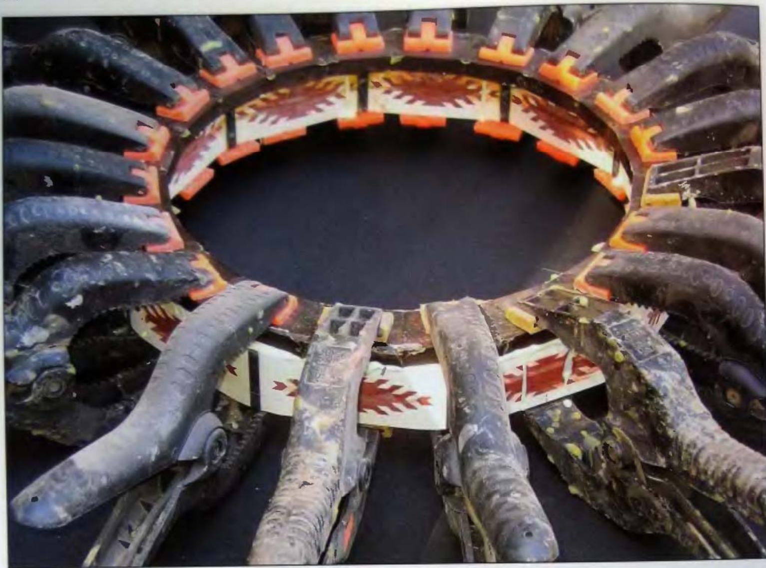
7-31 Unmounted thin rings can be joined with spring clamps.
