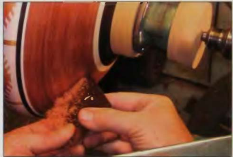
9-33 Before sanding, a fine burr on a cabinet scraper can improve the surface quality.
