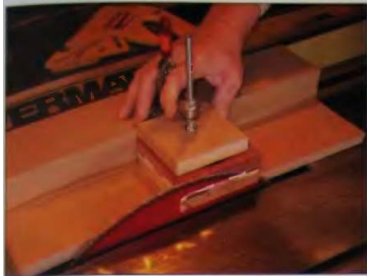
15-09 A table saw sled results in a smoother cut.
