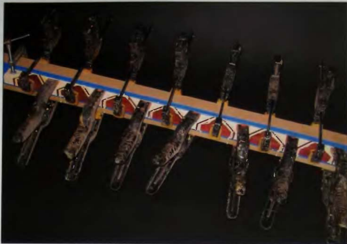
9-07 Here are the components of one strip all glued and clamped.
