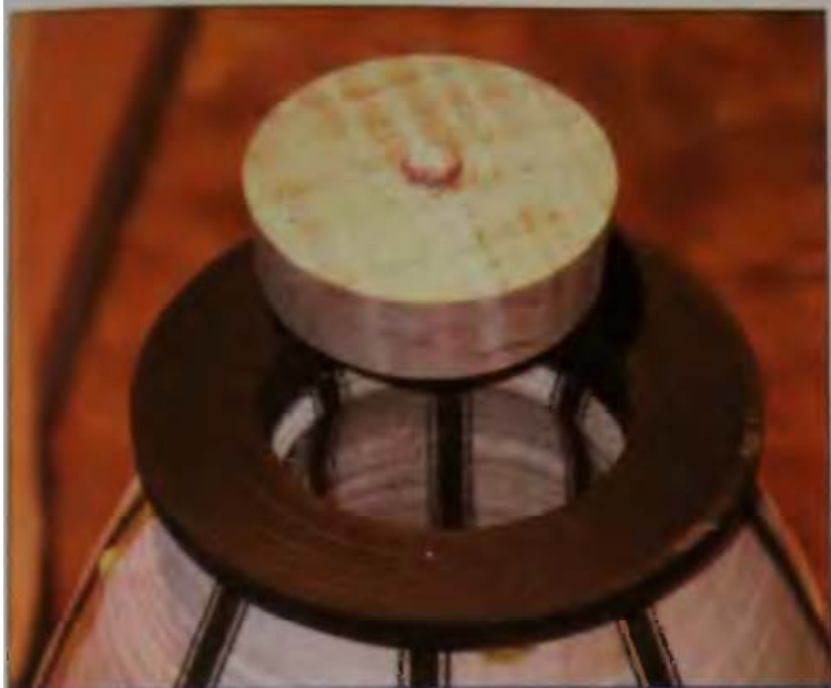
10-16 A tapered plug completes the vessel base.
