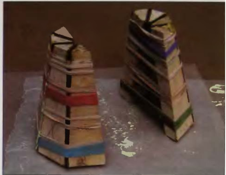
10-12 Rubber bands can provide plenty of clamping pressure.
