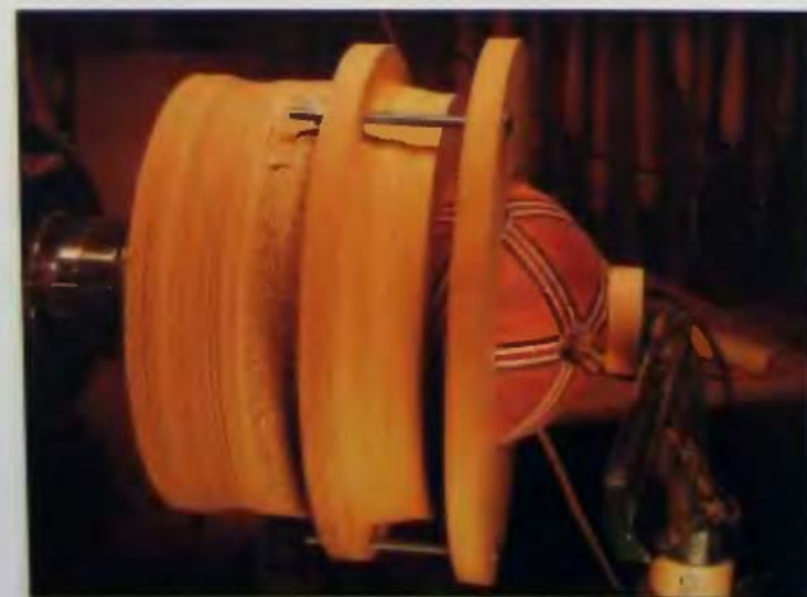
14-14 A Large jam chuck with keeper ring secures the sphere.
