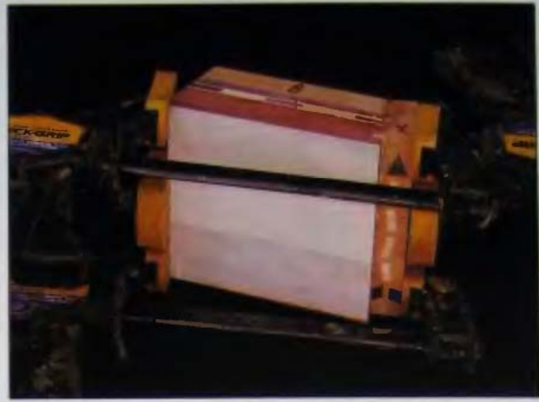
15-10 Gluing on the splines saves time later.
