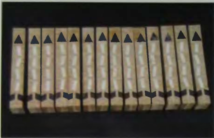
15-06 While the arrows point vertically, the wood grain in the splines is positioned horizontally to match the adjoining segments.
