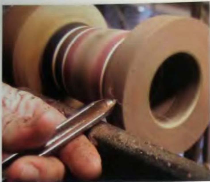
7-24 The 1/2-inch bowl gouge is by far my most-used cutting tool.
