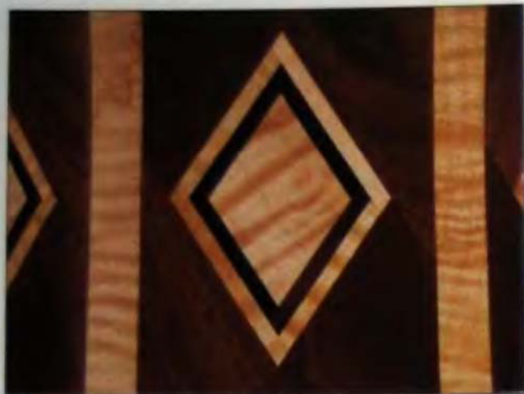
8-05 Large diamonds require the use of a disc sander.
