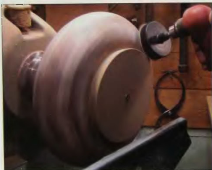
13-13 An inner jam-chuck allows the outer surface to be worked upon.
