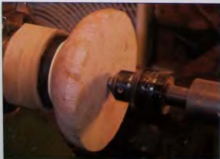
10-20 The tailstock effectively clamps these sections together.
