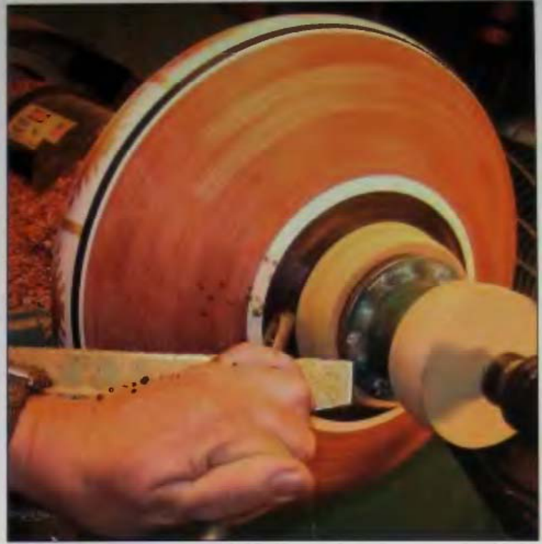
9-32 A perfect glue job allows lathe mounting from either end.
