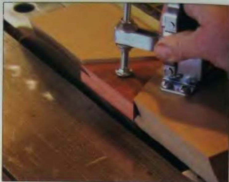
14-06 Triangle edges can be mitered using a table saw jig with a hold-down clamp.
