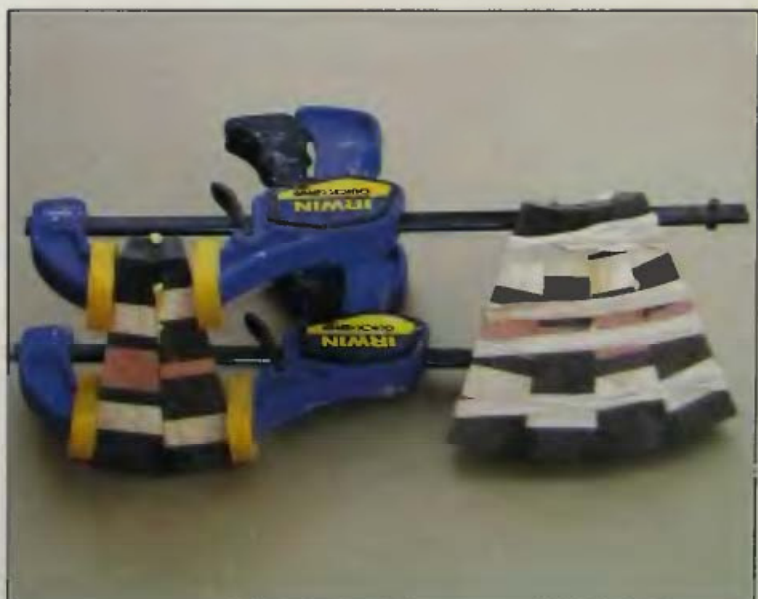
16-08 Gluing the staves together is a multi-step process.
