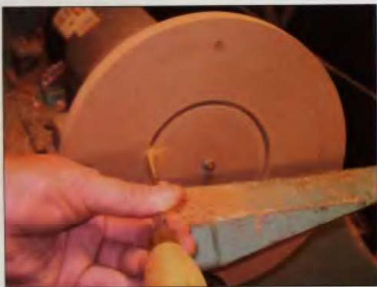
10-09 A parting tool is used to cut donut-shaped rings for the gluing jig.
