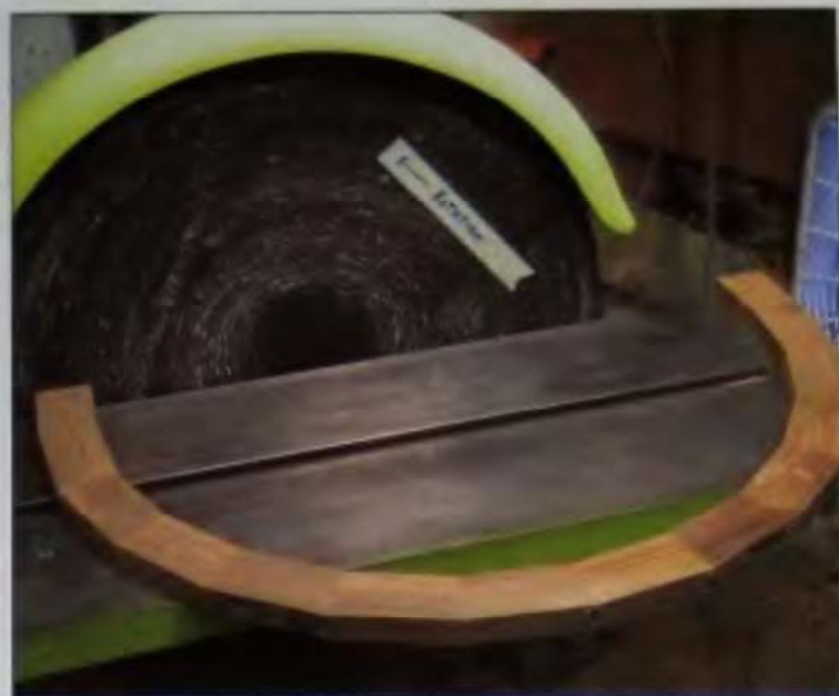
7-12 This ring is too large to sand both ends at one time.
