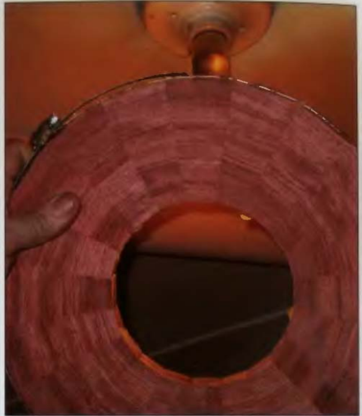
7-18 A bright light can help expose imperfect joints.
