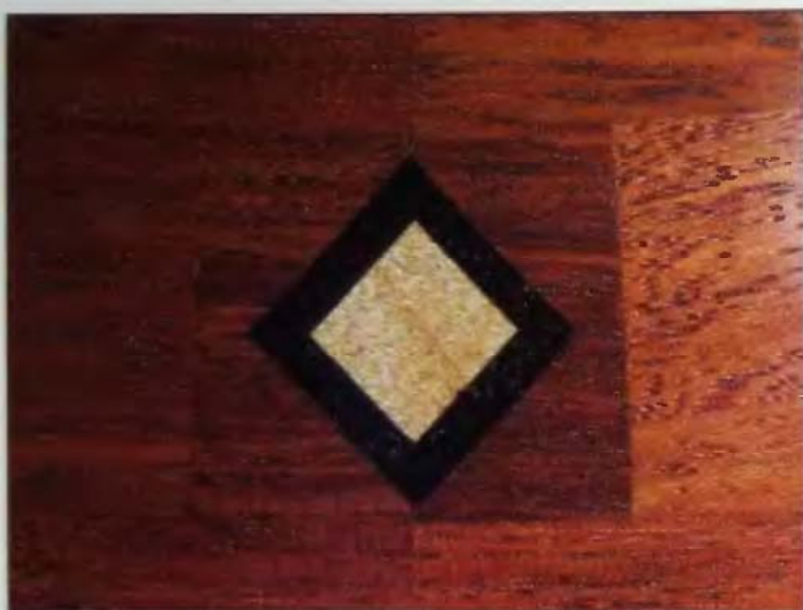
8-06 A router created the opening for this small diamond shape.
