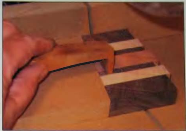
16-06 The compound-mitered stop block provides stability and accuracy.
