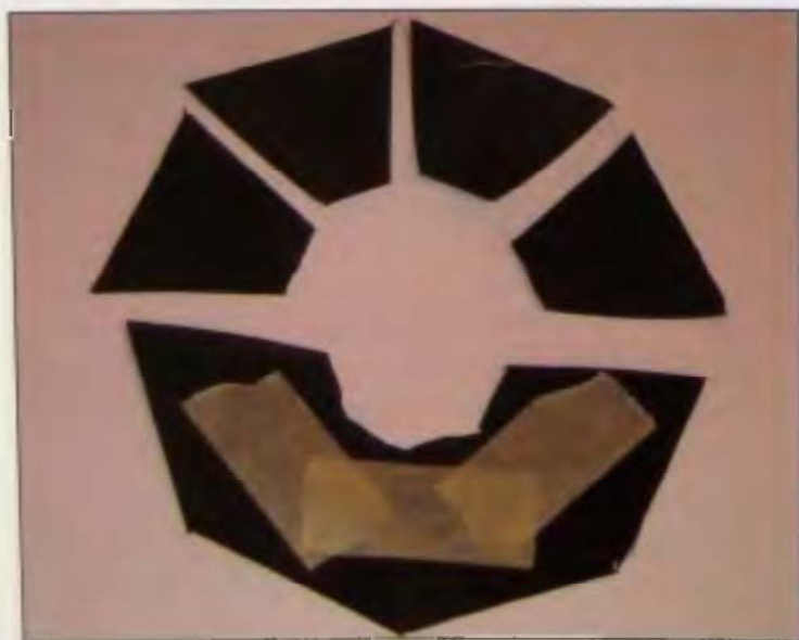
7-36 Using veneer segments (as opposed to one piece) maintains consistent grain alignment.
