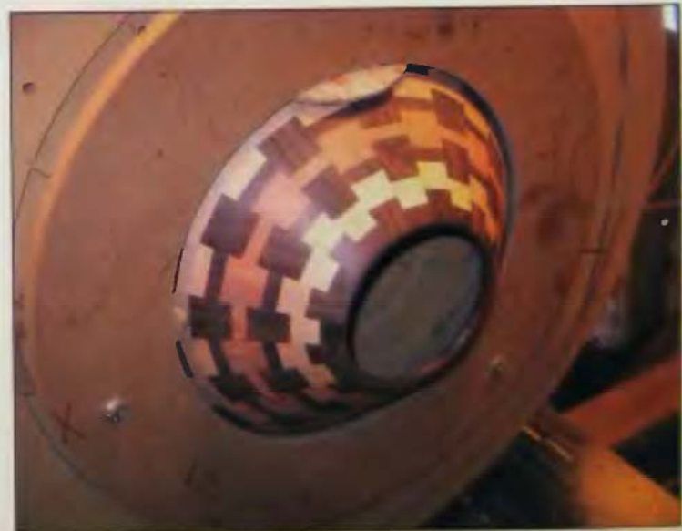
16-14 Attach the retaining ring, turn the donut ring, and then secure the cone shape.
