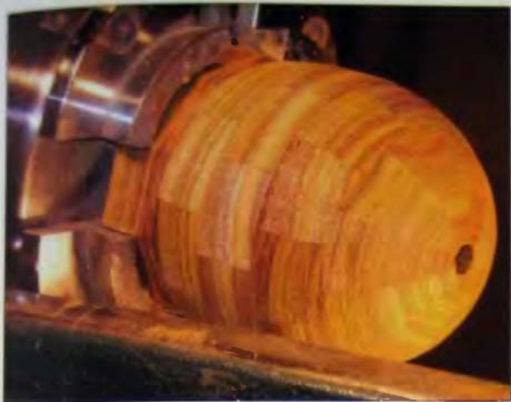
14-19 Turning a stack of rings into a sphere.
