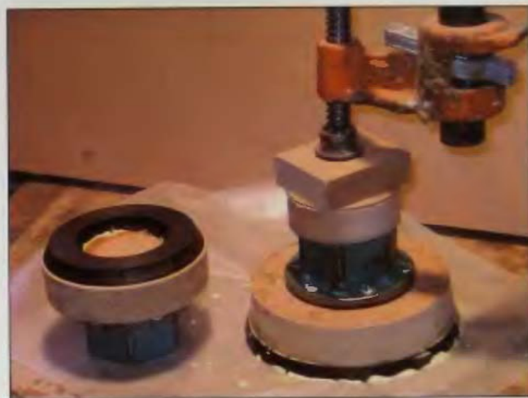
9-20 Top and bottom rings are secured to faceplates.
