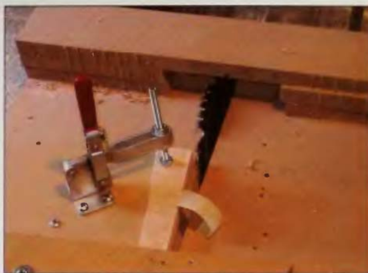
10-04 After cutting one side, set up the sled for the second sides.
