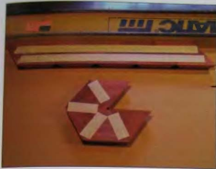
14-07 Masking tape holds pieces in alignment.
