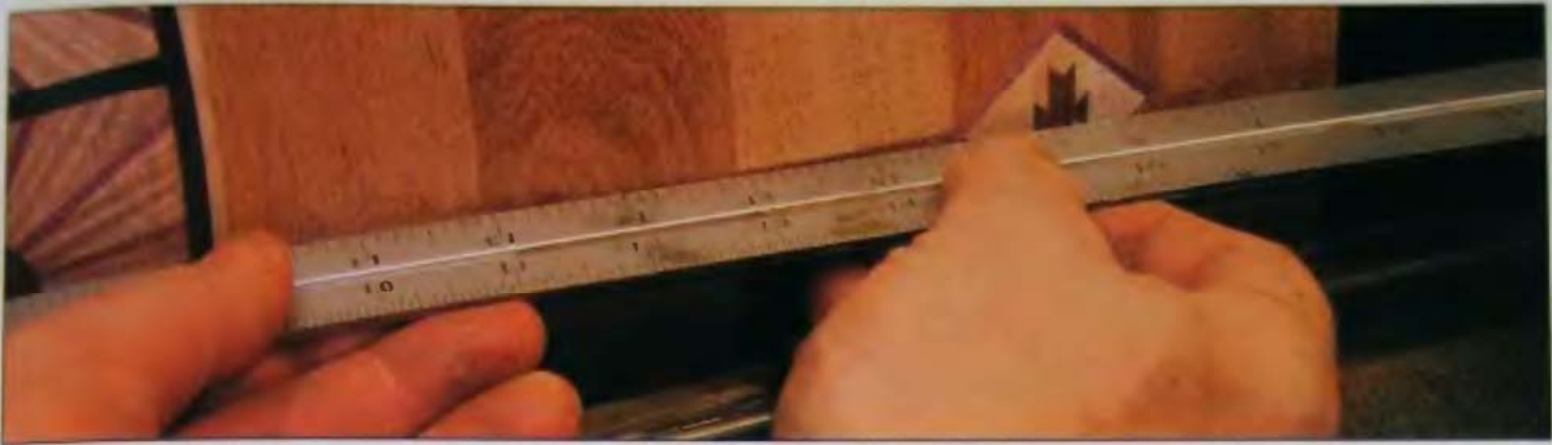
15-28 A straight edge can be used reveal a flat spot on the profile.
