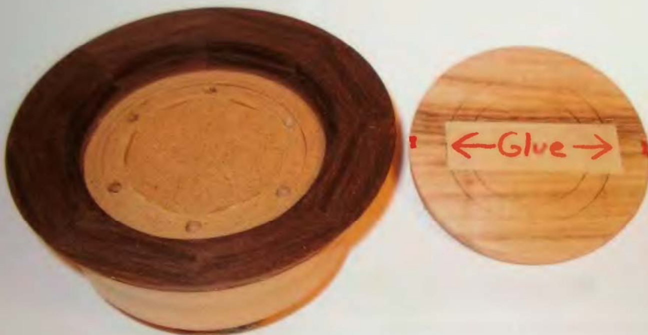
7-40 Large bases require a floating plug.
