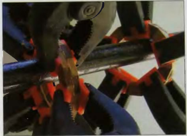
13-10 Gluing the ring together starts by gluing pairs.
