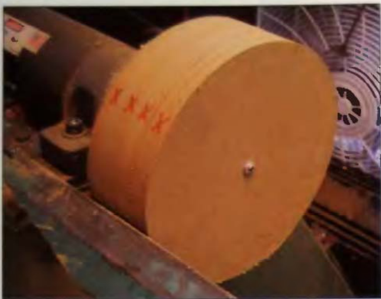
10-08 This will become a gluing jig for all-at-one-time stave gluing.
