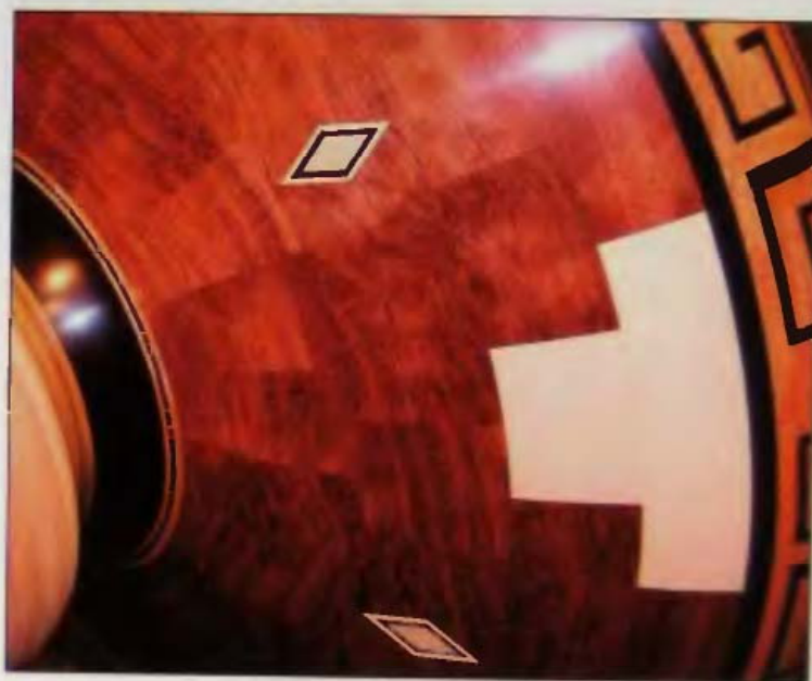
11-21 An example of router-created diamond-shaped elements.
