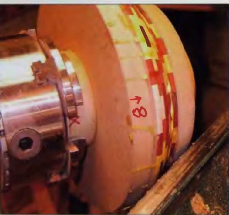
12-07 This is a section of one bowl being assembled, one layer at a time.
