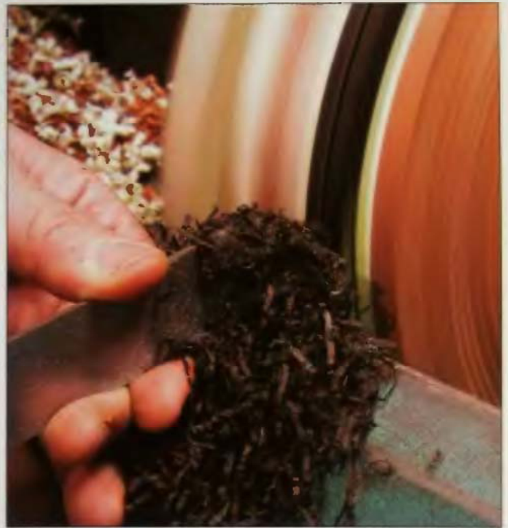
7-37 Making two rings from one can save time.
