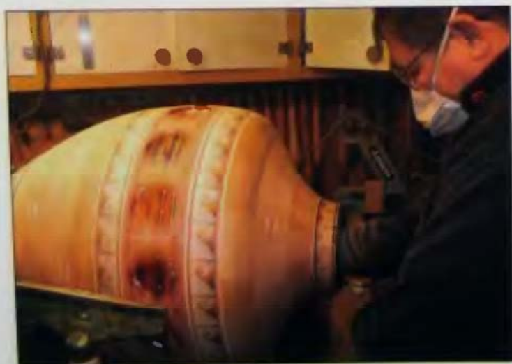
15-31 A hand-held cabinet scraper and power sanding finishes the inside seam.
