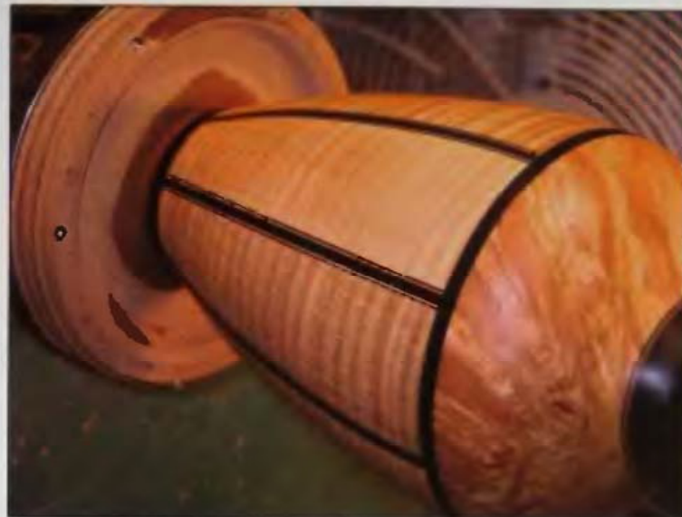
10-22 Generally, I like to apply finish while the vessel is still mounted.
