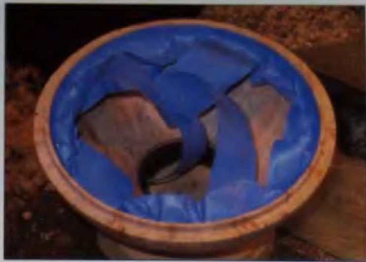
10-21 Tape can be used to prevent glue squeeze-out contamination.
