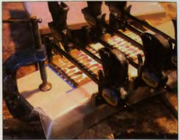
11-13 A gluing jig can help keep components square during gluing.
