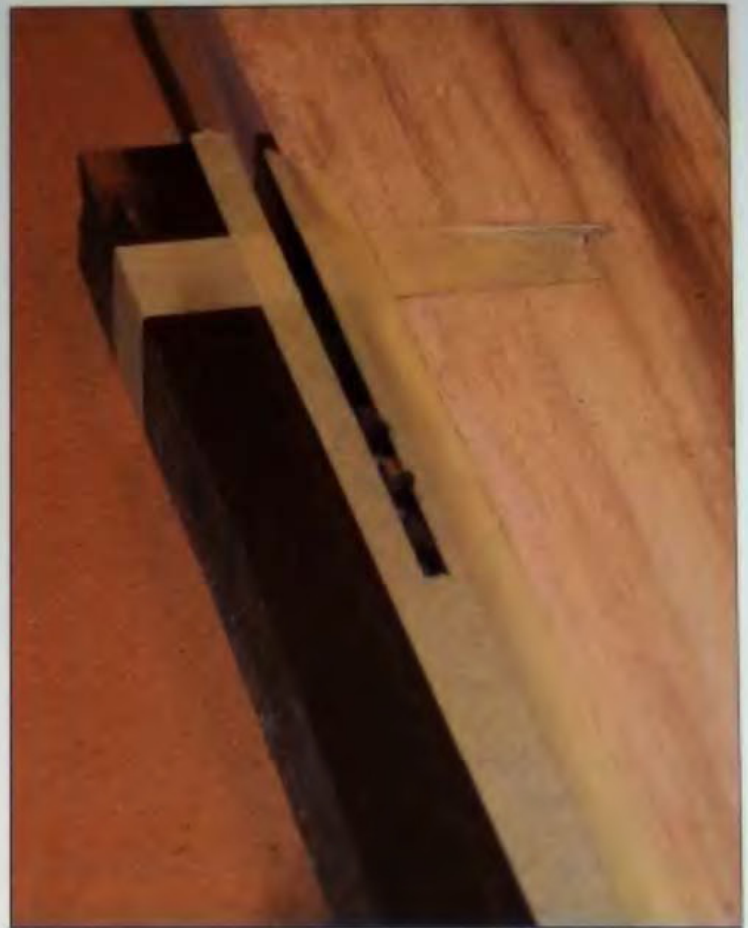
7-05 Cut thin strips by taping the ebony to a wider board.
