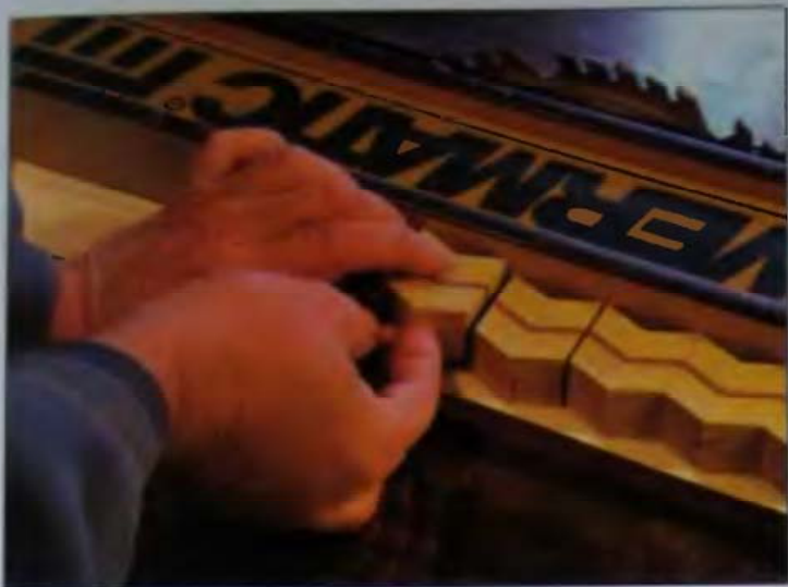
11-05 Double-sided tape can be used to secure segments for table saw trimming.
