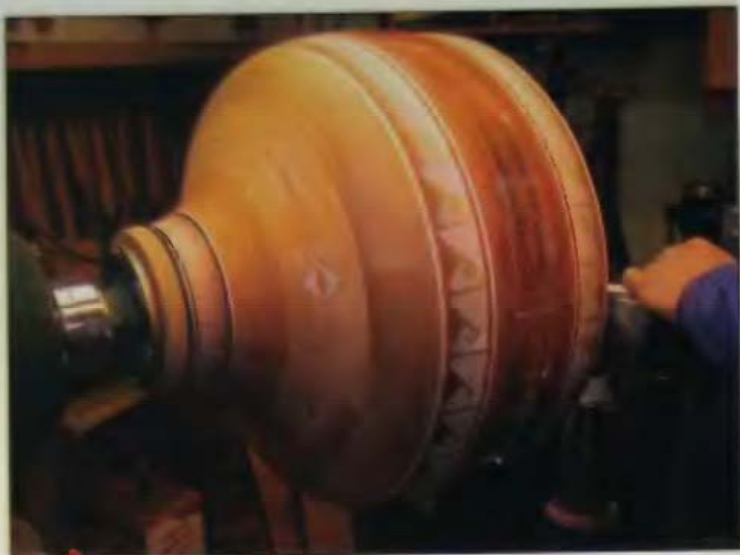
15-29 The top half is almost ready for the last gluing step.
