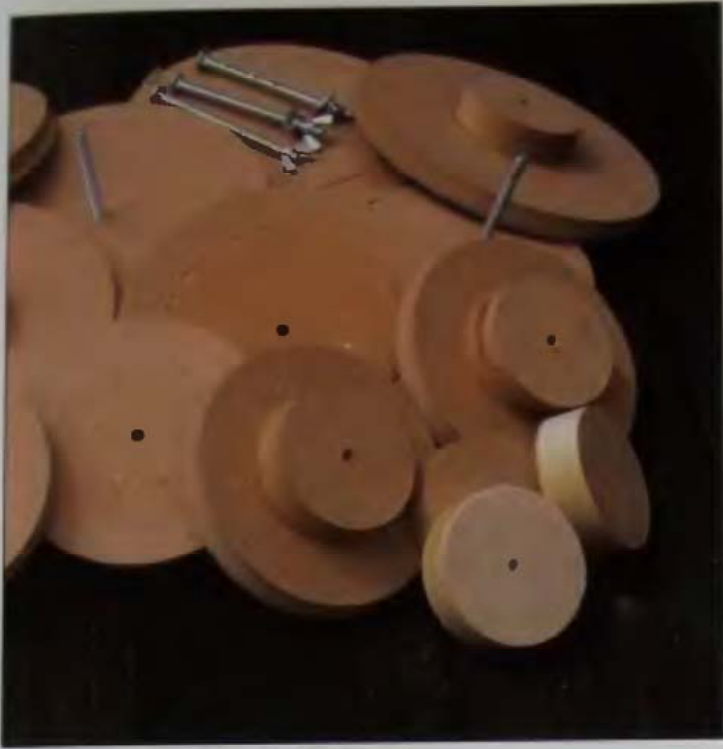
7-32 MDF circles are very handy as temporary waste blocks.
