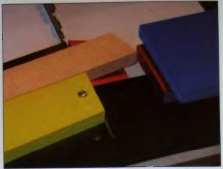
7-03 Notice the red ramp that keeps the cut segments away from the blade.
