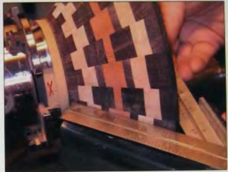
16-13 A straight edge and 45^\circ square are used to check the slope angle.
