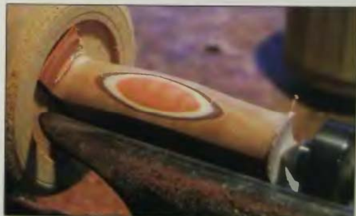
11-35 Carefully turn away the outside layers.
