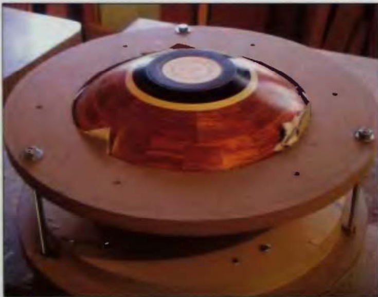
9-35 This is an effective method of reverse mounting the vessel.
