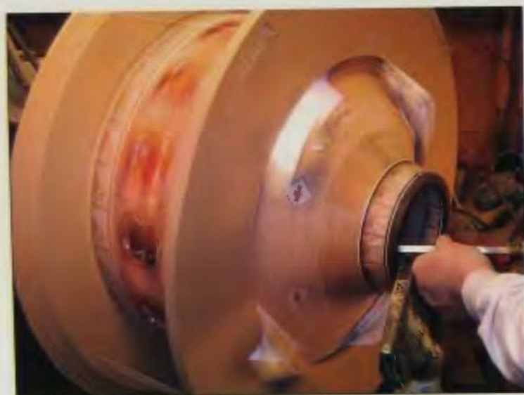
15-30 Reverse mounting at this stage allows the top to be finished.
