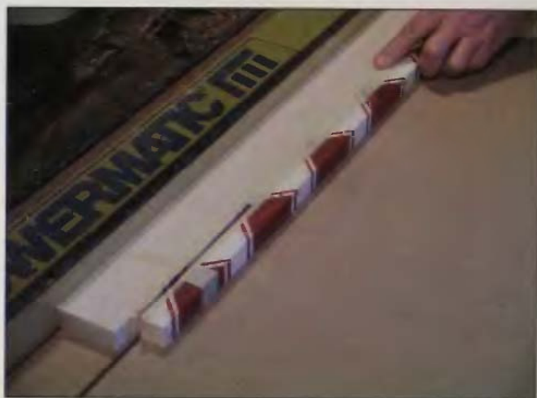
9-08 To rip-cut thin strips, attach the board to a wider push board.
