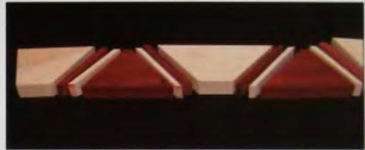
9-03 This is the arrangement of components prior to gluing.
