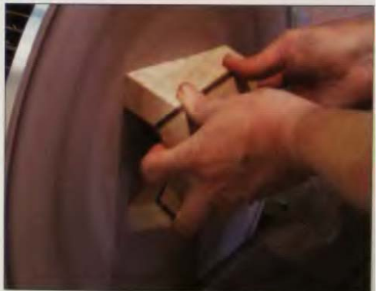
10-13 A disc sander makes short work of flattening the half-cones.
