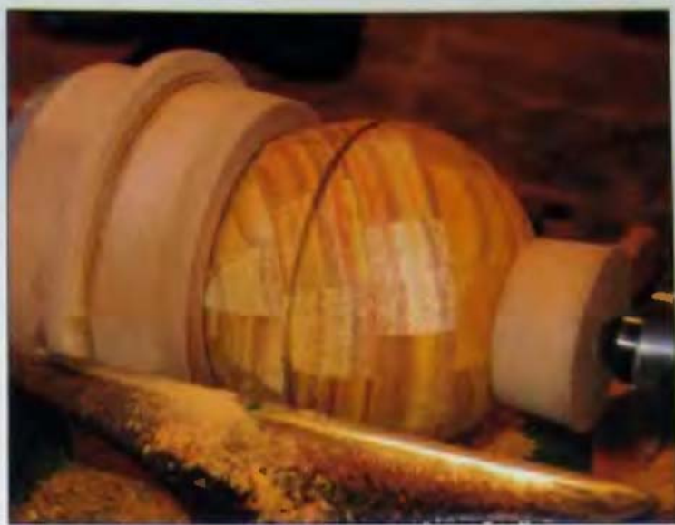
14-20 The tailstock holds a sphere as it is split with a parting tool.
