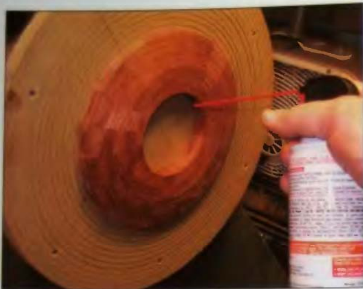
9-22 Clean surfaces help ensure good glue joints.
