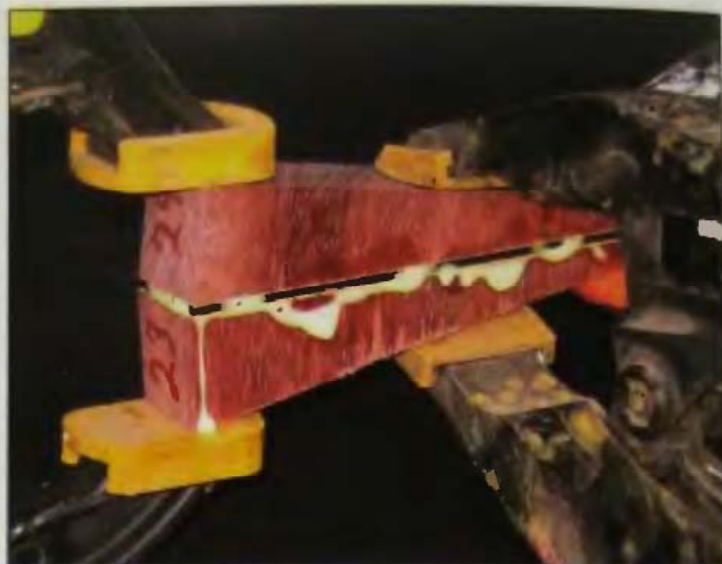
11-43 Assembly starts by gluing pairs together with splines.
