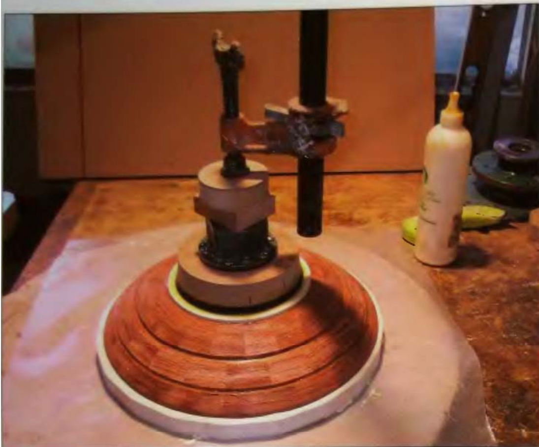
7-29 Using a clamp against the ceiling is one way to join rings.
