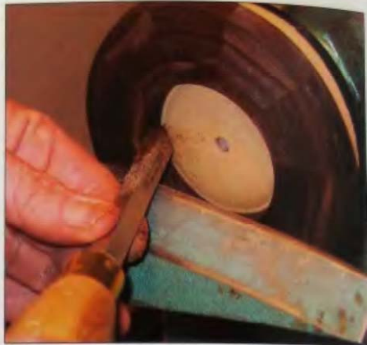
7-39 Make tapered openings for plugs.
