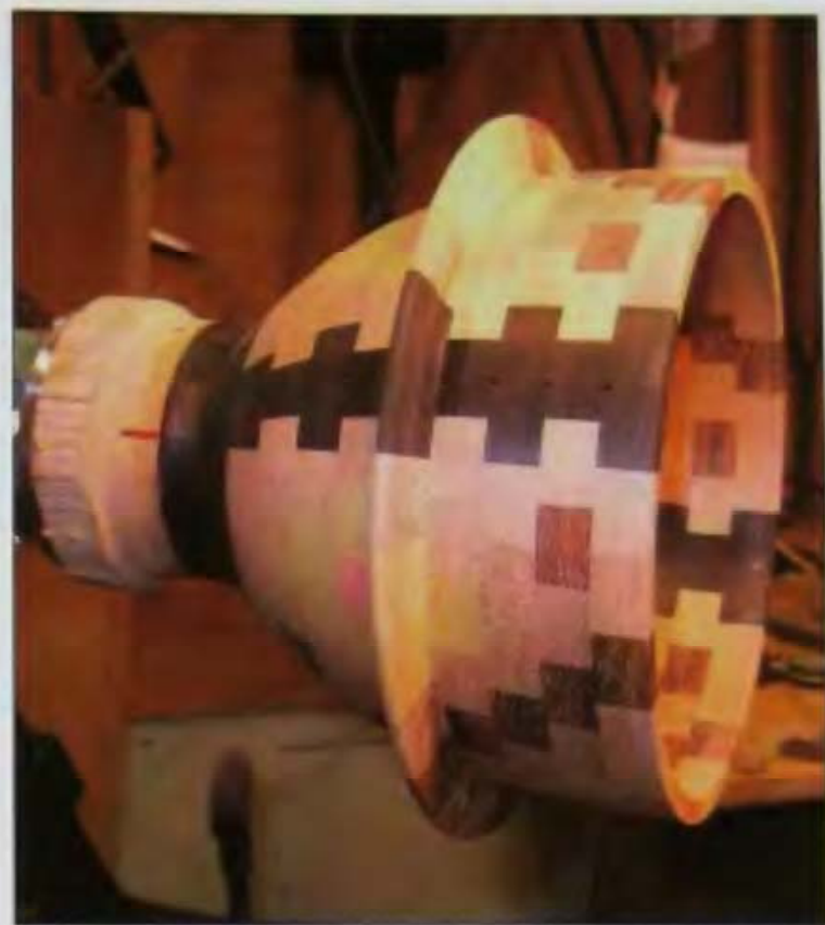
13-01 Notice the small drilled holes that can be used to check wall thickness.
