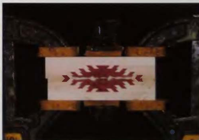
9-14 Precise alignment during gluing is essential.
