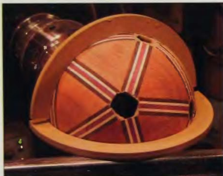
14-13 A thin, turned ring makes an effective template.
