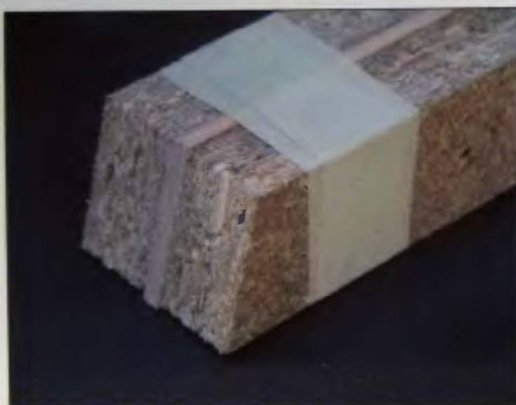
7-35 Veneer strips stacked between MDF cauls can be quickly cut into segments.
