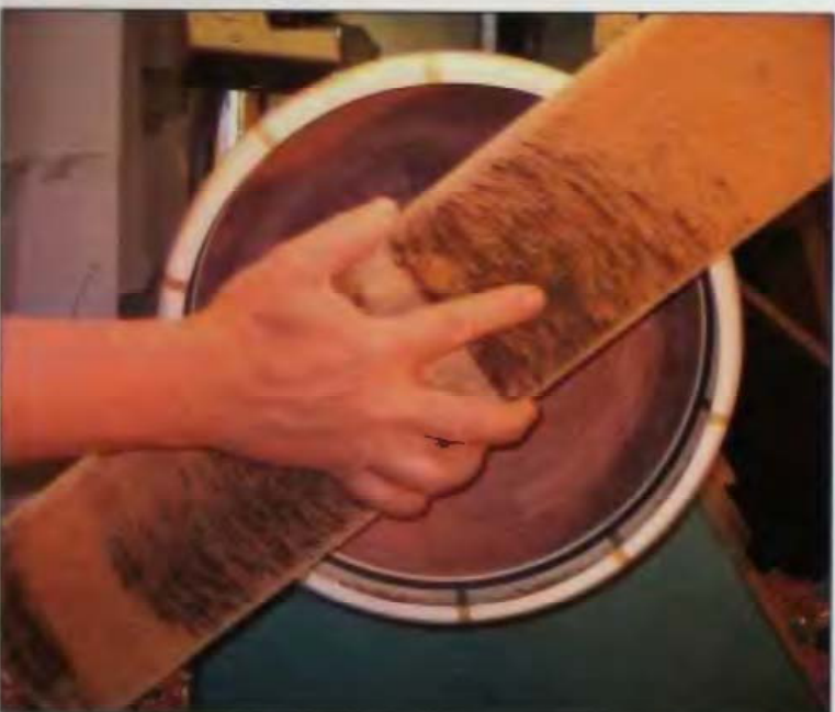
9-29 This is the last sanding step prior to gluing the halves together.
