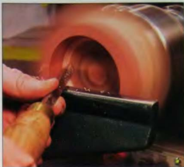
15-05 Do not turn too deep, the design is only 1/8-inch thick.
