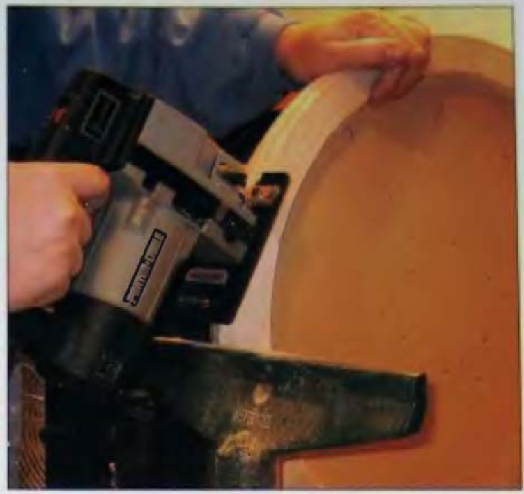
15-15 A sabre saw can be used to split a large ring.
