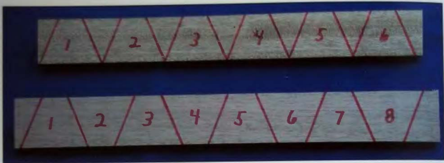
7-04 There are two basic ways to cut a board into segments.
