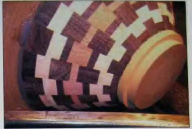
16-12 This waste block is ready to be mounted in a four-jaw chuck.
