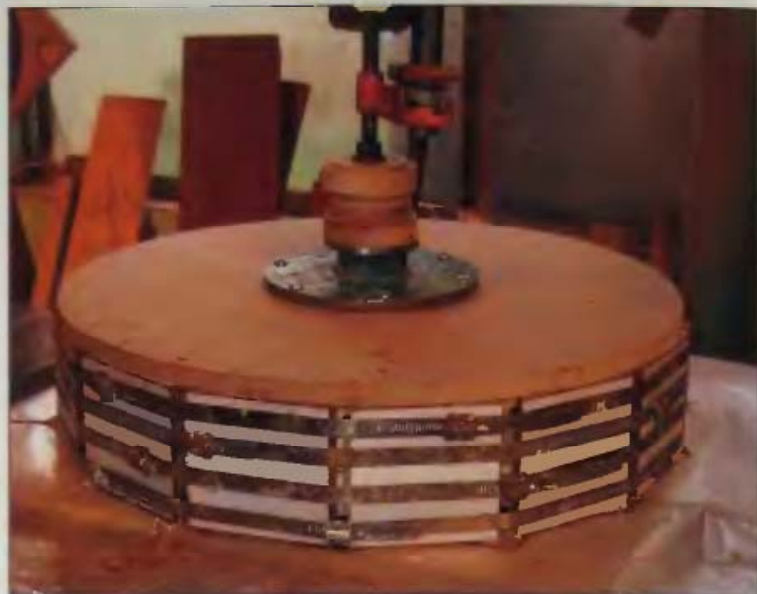
15-12 A waste block can be attached at the same time that the ring is glued.
