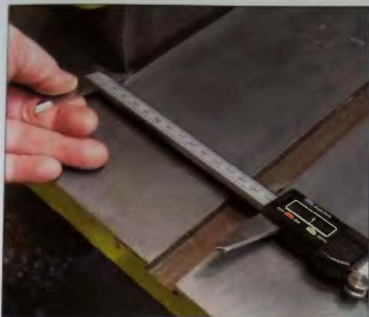
7-14 The sanding table alignment is important.
