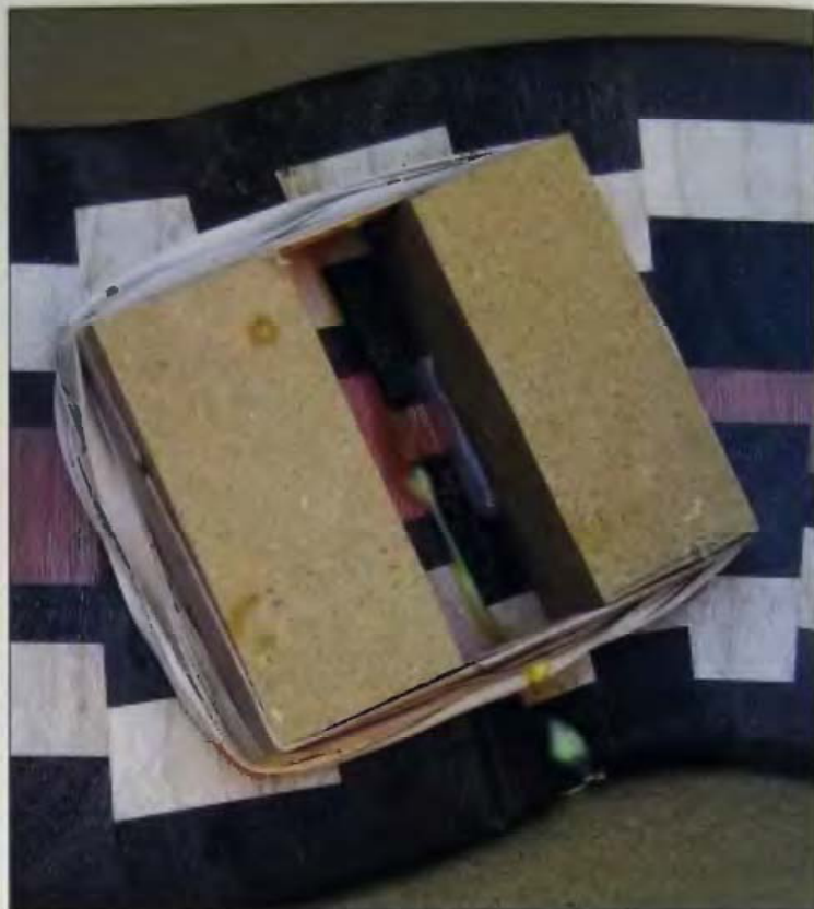
16-16 This method requires equal pressure on both sides of the glue joint.
