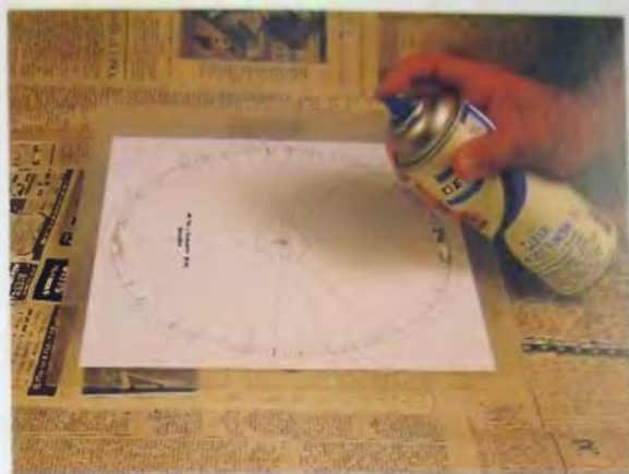
11. Spray on a couple of coats of clear finish to protect the paper from abrasion and tears.
