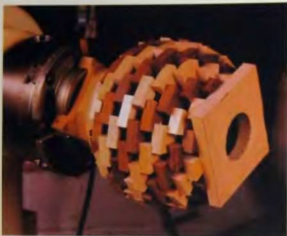
4. Finished glue-up ready to turn. Ten layers of segments are glued on a solid maple base with a solid maple rim.
