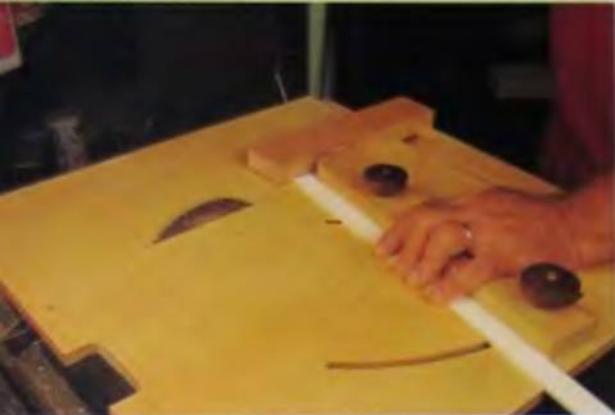
115. The converted lead type slitting saw used to cut very small segments. It uses a 6 inch blade with a thin kerf and no tooth offset.
