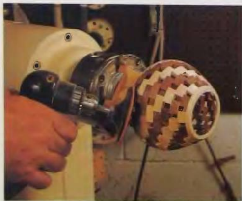
102. Use a power sander if available for rough sanding.
