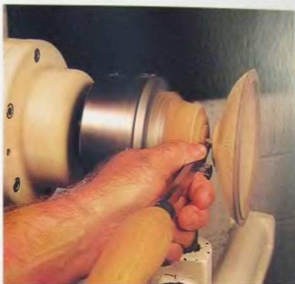
158. A parting tool is used to cut through the excess on the hub. Leave the hub about 1/2 inch thick for detailing. I apply spray finish to the inside at this time.
