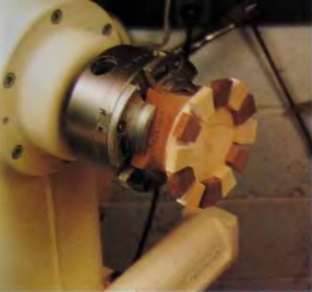
77. The first layer of segments glued to the base.
