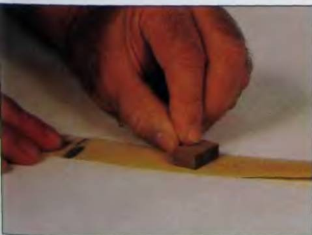
69. A quick swipe on 240 grit sandpaper will remove the burr.
