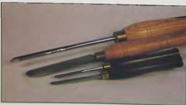
95. Tools I use to turn the outside include a 3/8 inch bowl gouge and a 1 inch round nose scraper. The small gouge and scraper are used to form the rim and foot region on more intricate turnings.
