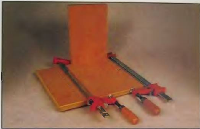
24. Glue and clamp the two pieces of plywood together. The height of the upright plywood should be about 1/8 inch less than the height of the spindle from the ways.
