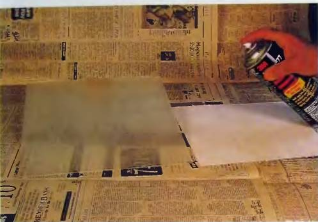
9. Coat both the Plexiglas and copy of the index wheel with contact cement.
