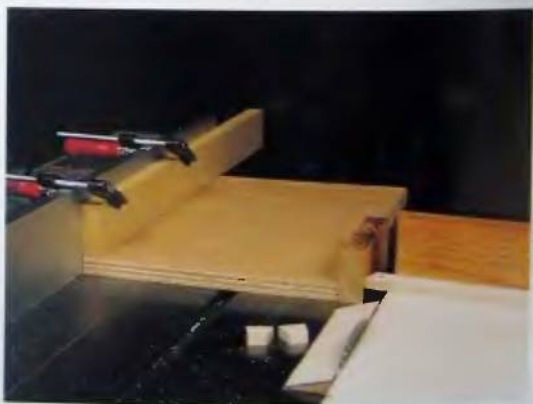
57. Alternate arrangement with standard fence. A spacer has been placed between the fence and blade to provide clearance for cut segments.
