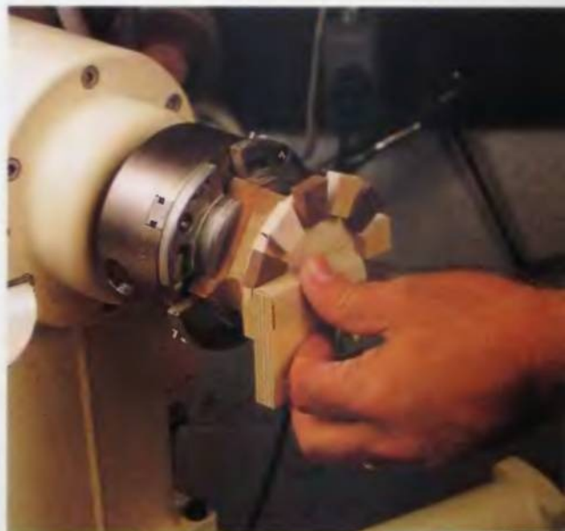
80. A sanding block can also be used to remove small amounts of unevenness.
