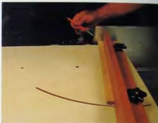
56. The Delta Unifence™ set back behind the blade to provide clearance for cut segments to slide away from the blade.
