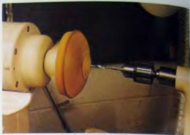
162. A 1/8 inch hole is drilled to accept a tenon on the finial. This should NOT go all the way through the hub. Apply spray finish to the outside at this point.
