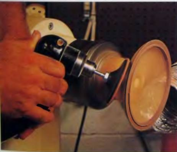
157. The outside can be sanded with strips of sandpaper or a power sander. Use light pressure and work through the grades carefully.
