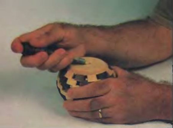
109. A carving gouge is used to remove the nub in the center left by the saw.
