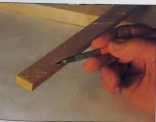
44. The strips will have saw marks when they come from the table saw. These must be removed for sound glue joints.
