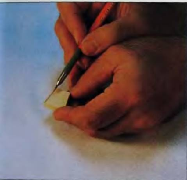
68. A small burr will usually be found on the edge of the segment. This must be removed for a good glue joint.
