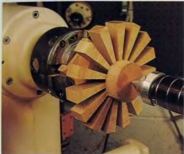
148. A 2 inch waste block is glued to the segments to provide additional support.
