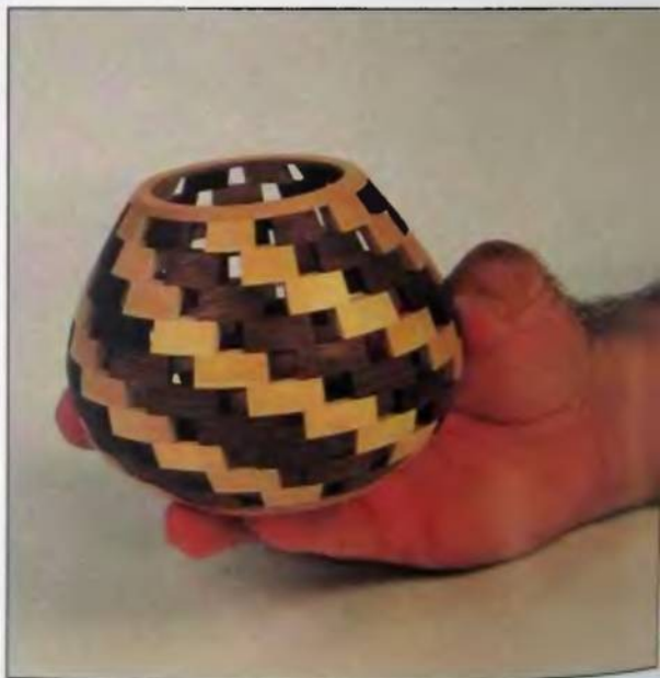
112. The finished open segmented turning.
