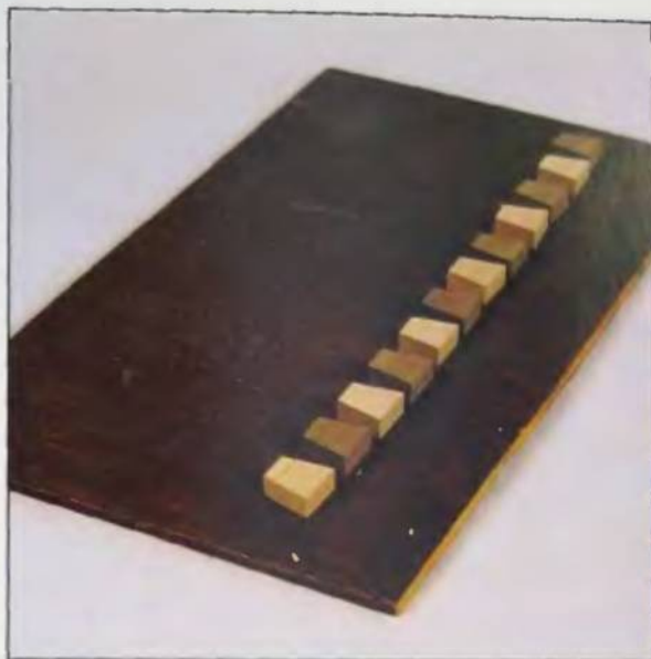
70. Line up the segments in the order they are to be glued. This step can greatly reduce pattern errors, especially in more complicated designs.
