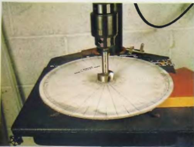
14. Use a fostner bit to cut the center hole. This should be sized to fit your spindle.
