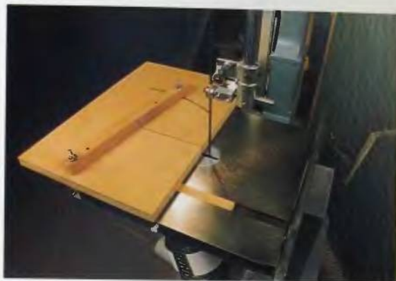
52. The sliding table installed on the band saw. A regular miter gauge can be used in place of the table for our project.
