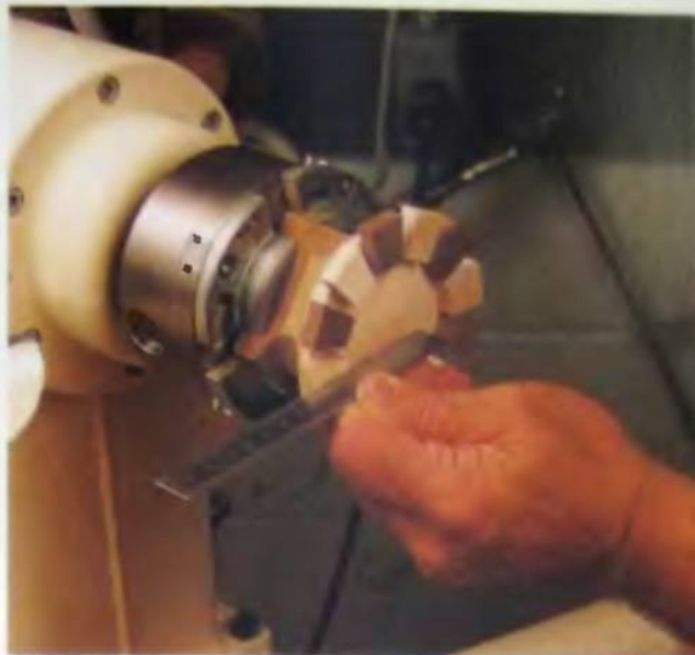
79. Check for flatness after making the cut. Any unevenness must be removed to guarantee a strong glue joint with the next layer.
