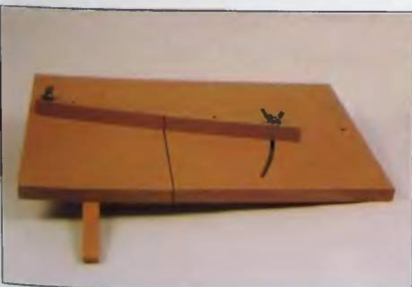
51. The sliding table for the band saw made of MDF with a hardwood runner for the miter slot.
