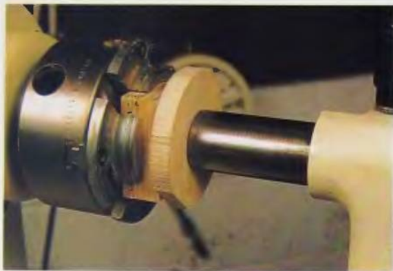
64. Glue the base piece to a waste block. I am using the tailstock in place of a clamp while the glue sets.
