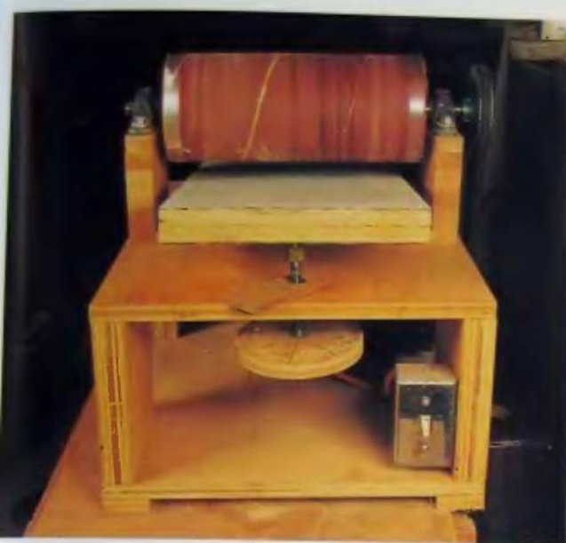
43. Dust cover removed, showing 6 inch plywood drum and pillow block bearings. The Formica™ covered table is raised and lowered by the lead screw epoxied to the adjusting wheel. The 1/2 hp motor is more than enough power for the narrow strips used on open segmented turning.
