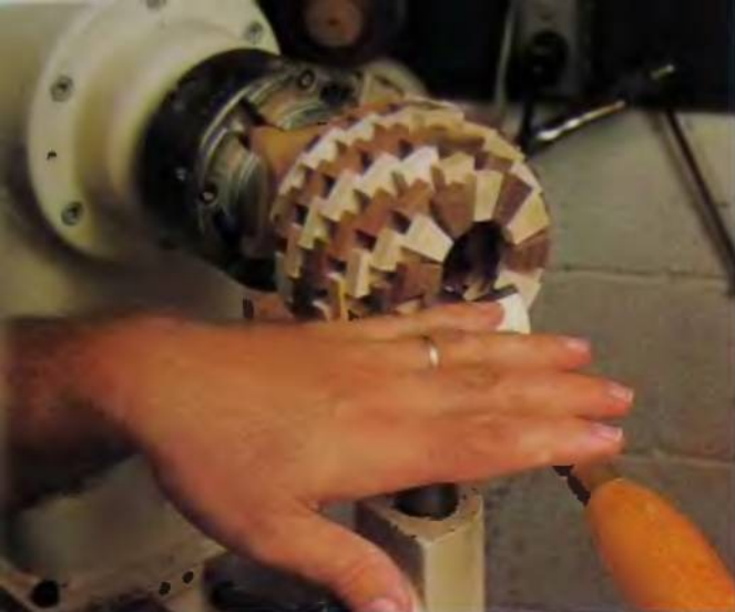
91. A facing cut must be made to flatten and true the top layer of segments.
