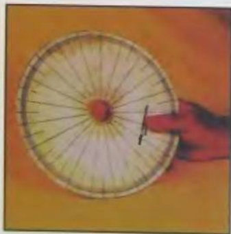
7. The finished index wheel. This is a 21 sector wheel, which I am making for a future project.
