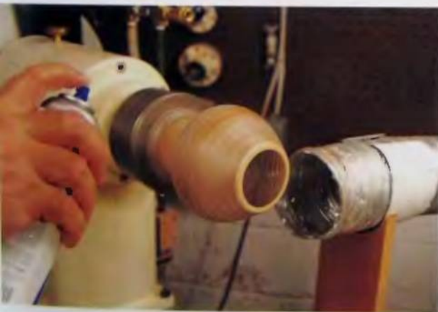
106. The outside is finished with three light coats of the same finish.
