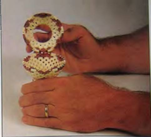
131. The two sections may now be glued together. Place a small drop of glue at each glue point, align the pattern and press them together lightly. The total area to be glued is small, so excess clamping pressure may squeeze out too much glue leaving a weak glue joint.
