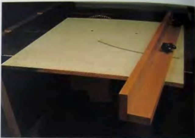
47. Overall view of sliding table for the table saw. A hardwood strip on the bottom rides in the miter slot of the saw.
