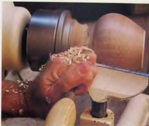
107. Use a parting tool to cut the bottom.
