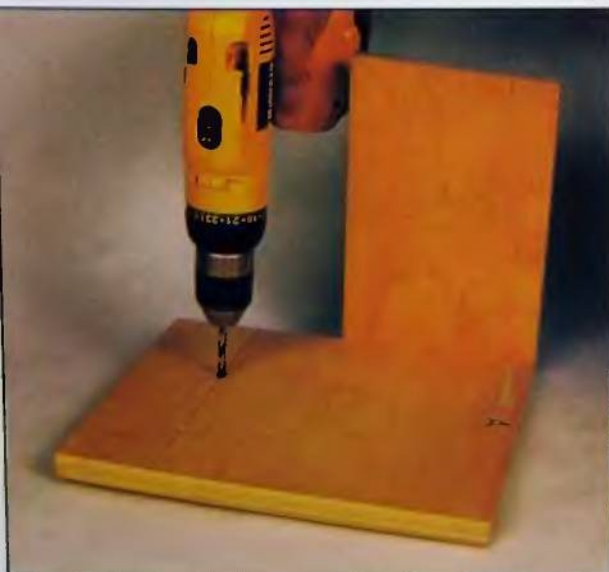
25. Drill two holes through the base, the guide, and the clamp block. These should be positioned on the centerline of the ways.
