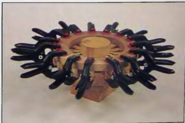
151. Many clamps are required. Each spoke must be clamped securely to the rim. I found these clamps at my home center for $1.00 each.
