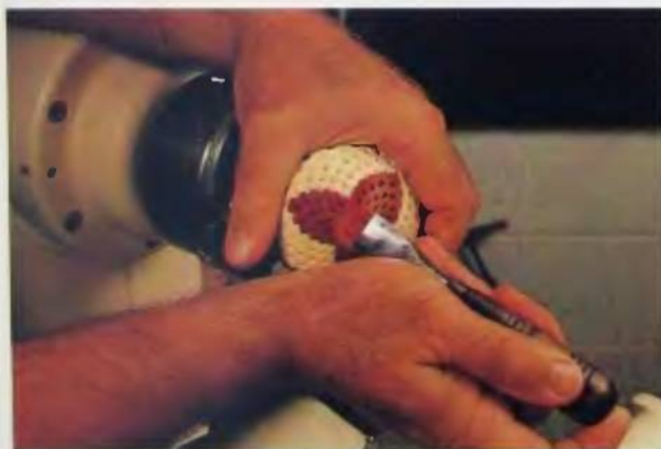
138. A carving sweep is used to clean up the tenon.
