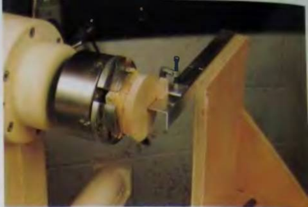
74. First segment glued in place. Light finger pressure for about five seconds is all that is necessary. Here I used Titebond™ glue. Any similar carpenter's glue will work.
