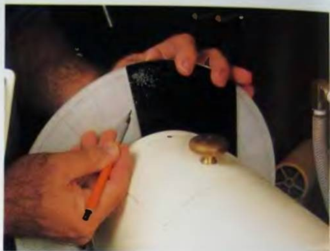
83. Set the index wheel to one of the short marks for the second layer.
