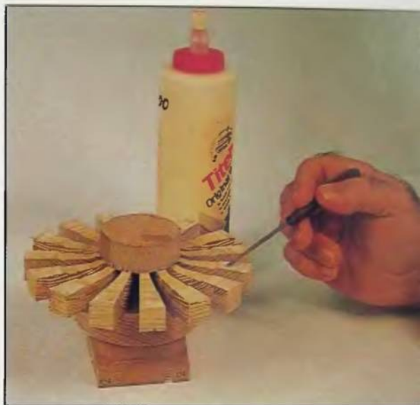
150. Glue is applied to all of the segments and the rim positioned and clamped. Allow this to dry thoroughly before proceeding.
