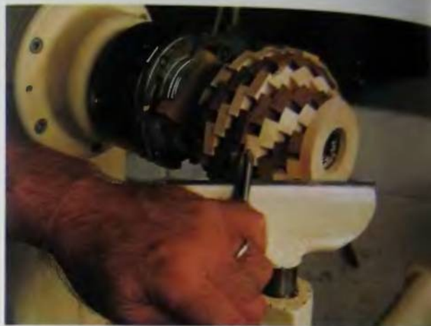
96. Begin turning by using the gouge to take off the corners and smooth the steps between layers. Read the paragraph on safety before doing any turning.
