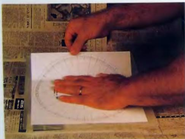
10. Allow the contact cement to dry until it is tacky, then carefully place the paper copy of the wheel on the Plexiglas. Avoid bubbles and creases and position the paper carefully. I usually cut the Plexiglas about an inch or two larger than the finished wheel to allow for positioning errors.
