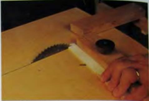
116. During the cutting process the fence remains behind the blade so the cutoff segment will not become wedged between blade and fence.
