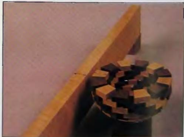
36. The thickness of the boards becomes the wall thickness of the final glue-up.
