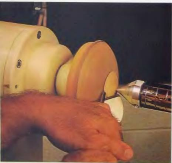
161. A small gouge is used to finish off the hub. I usually add one or two undercuts to match the undercut between the spokes and the hub.
