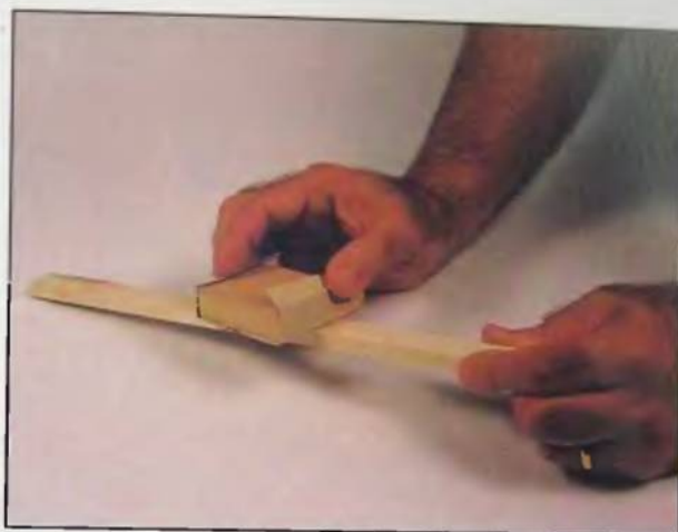
45. If a thickness sander is not available, use a sanding block to remove saw marks.
