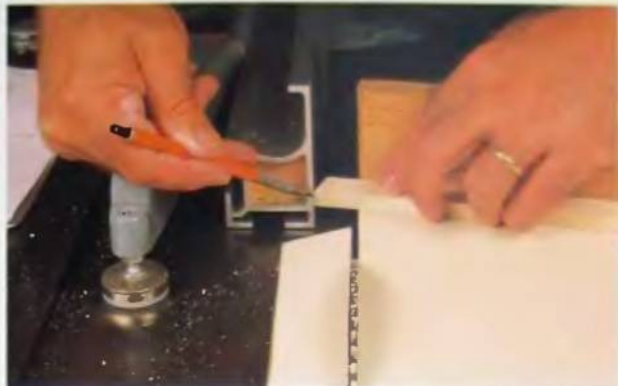
60. When cutting segments the fence is used as a stop.
