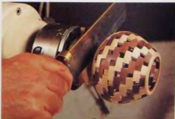
108. I do not completely cut all the way through with a parting tool. The last 1/4 inch or so is cut with a hand saw while the lathe is turned off.
