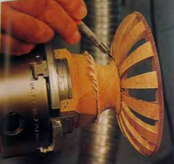
156. Carefully turn away the excess material on the hub to reveal the undercut made before gluing the spokes to the hub. This undercut is a nice decorative feature for the transition between spokes and hub.
