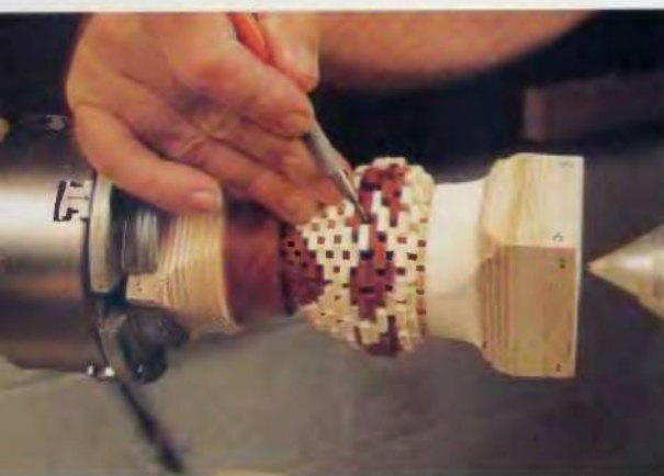
123. Overlap the segments where the layers are taped together in order to provide a little extra strength. This joint will be split apart and glued with the normal offset during final assembly.
