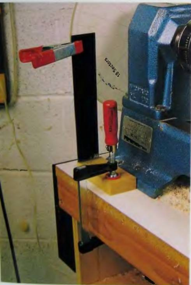
18. An alternate pointer that can be clamped to the benchtop.
