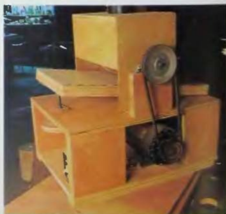
42. Shop made thickness sander constructed of mostly found materials.
