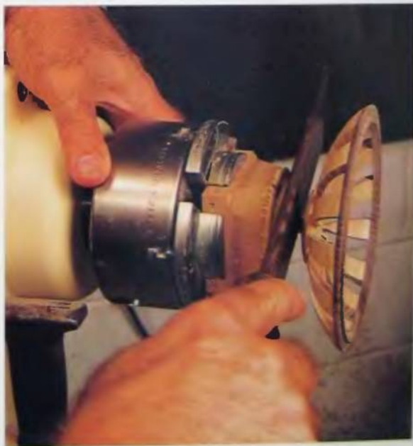
159. A small hand saw is used to cut through the final 1/4 inch.
