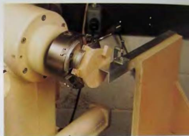
75. Advance the index wheel 30° to the next long index mark. You will be rotating the piece toward you.
