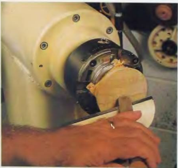
65. Use a scraper to face off the base. A nice smooth, flat surface is needed here.
