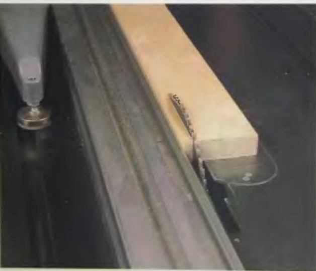
40. Use a table saw to cut your board into strips.
