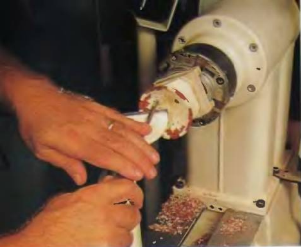
129. Finish the inside of the top section. It is difficult but get the rim as close to the final shape as possible.
