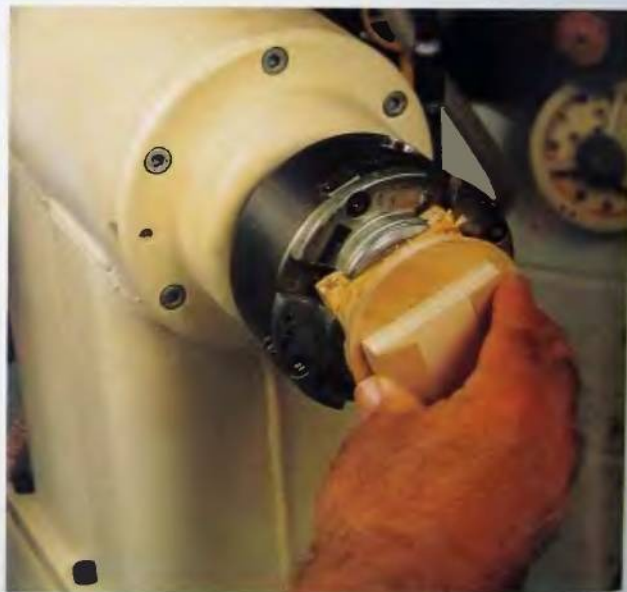
67. The base piece becomes the inside bottom of the turning. This is a good time to sand it but do not apply any finish as that could interfere with the glue joint.
