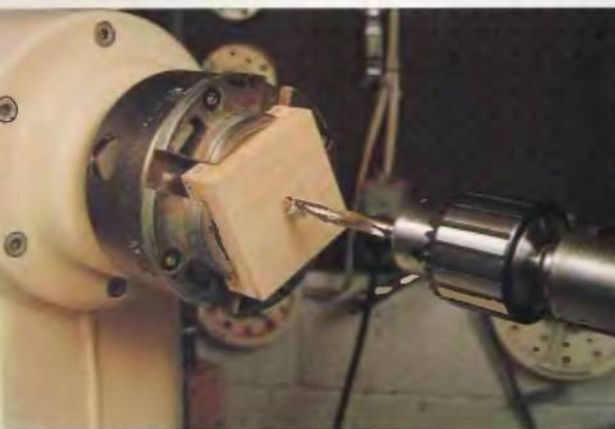
117. Mount a waste block in a chuck and drill a 1/4 inch hole in the center. The numbers on the corner of the waste block are used to indicate the corresponding chuck jaw so the block can be repositioned exactly.
