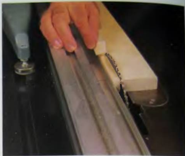
41. The height of the segments is determined by the thickness of the strips you cut.
