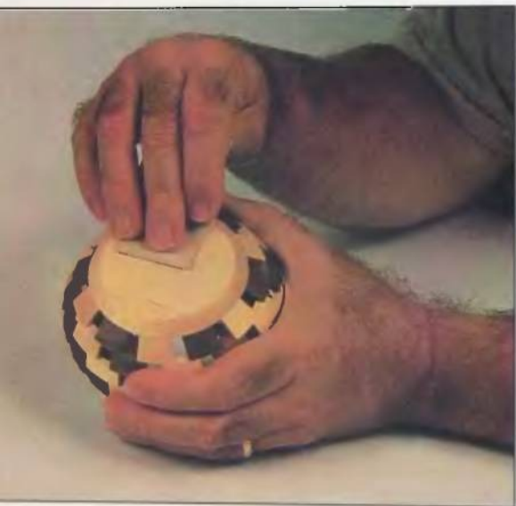
110. Sand and put a little finish on the bottom.
