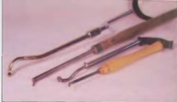
99. My favorite tools for hollowing. At top is the Sorby system, followed by a David Ellsworth tool, a miniature Sorby, and a Robert Rosand hollower. These all work well for open segmented turning.
