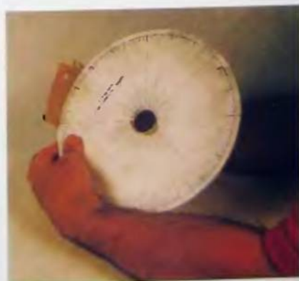
12. Use a band saw to cut out the wheel. Leave a small amount of extra stock so that you can sand down to the finished size.
