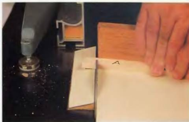
61. I have labeled the two faces of the stock "A" and "B". Here I am cutting the "A" surface.
