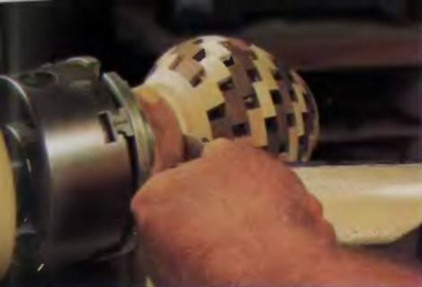
97. Use a parting tool to cut a shallow groove where the bottom will be located. This helps visualize the shape when developing the final form.
