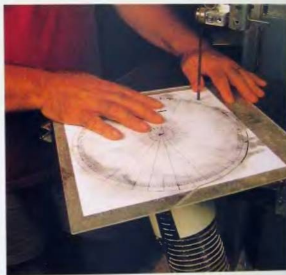
12. Use a band saw to cut out the wheel. Leave a small amount of extra stock so that you can sand down to the finished size.
