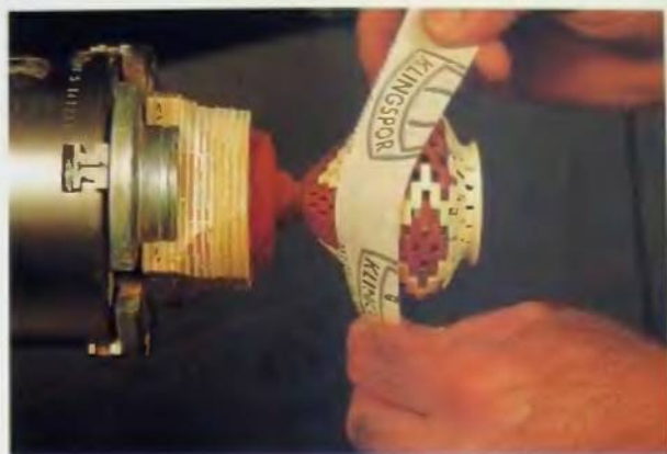
135. Use a strip of sandpaper for your final sanding. Do not use sanding blocks as they deform the segments.
