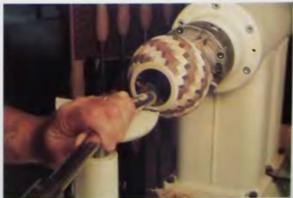
101. I switch to the hollowing tools as I get further down inside the turning.
