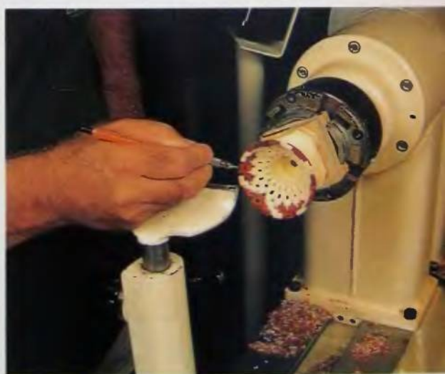
128. Turn the top section next. Pay close attention to the wall thickness in the beginning so it matches the wall thickness on the bottom section.
