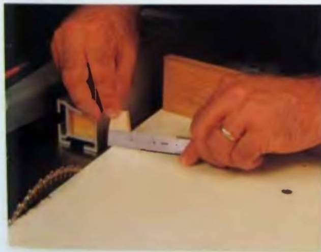
59. Cut a segment, then check the Dimension C. Make adjustments to the fence/stop as needed.
