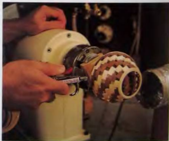
104. Compressed air does a great job of removing sanding dust and chips that may still be inside.
