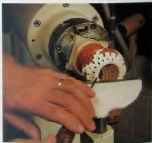
132. The rim is cleaned up using small tools and very light cuts. When possible I will use a cone center in the neck of the turning to stabilize it.
