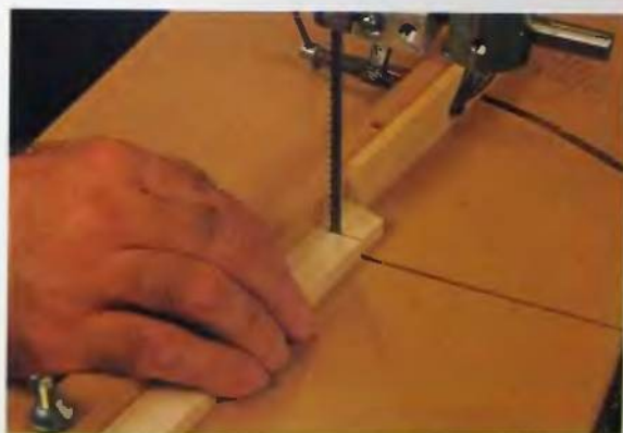
53. Using the sliding table on the band saw to cut segments. A stop is made with a C-clamp and scrap of wood.
