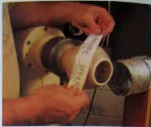
103. For fine sanding, or if you do not have a power sander, cut the sandpaper into strips and use as shown. Do not use sanding pads or your fingers as the segments will get a pincushion look as the edges are rounded over.
