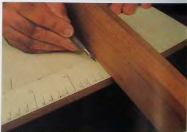
48. An advantage of the sliding table is the length of the miter arm. This makes it easy to get accurate degree settings. I can set the arm to about 1/4 of a degree, which is necessary on turnings with 35 or 40 segments per layer.
