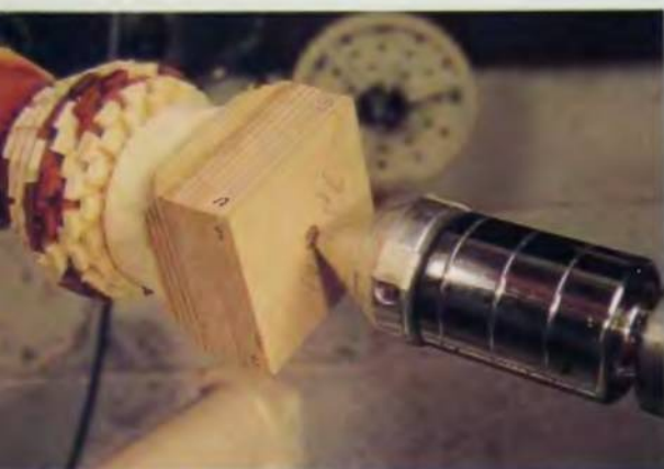
122. The hole previously drilled in the waste block for the top section is supported with a cone center while the base is mounted in a chuck.
