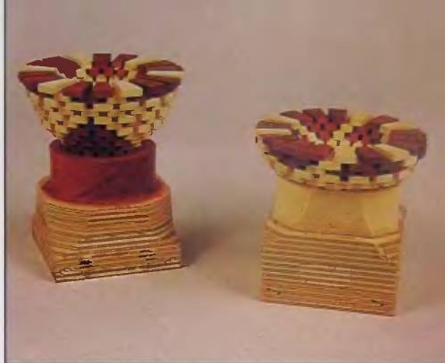
120. You should have two glue-ups at this point that, if joined together, would be the complete turning. Use care to insure the pattern will come out correctly when the two sections are joined.
