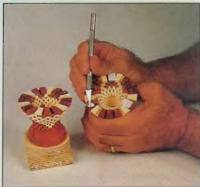
126. All residue from the tape must be removed to get a good glue joint during final assembly.
