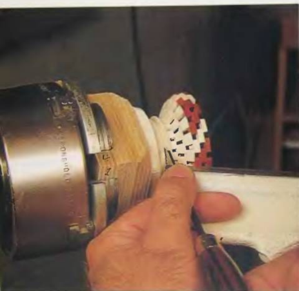
130. The top section is parted off. The rim should be close to the final desired shape.
