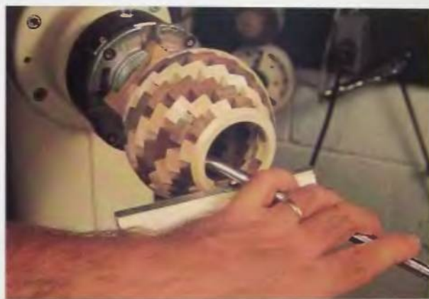
100. I use a gouge to cut the inside rim and top segment layer. The gouge seems to cut the inside better than scrapers but there is only so deep you can go with a gouge.
