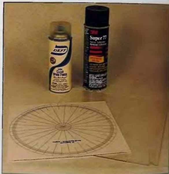
8. Materials needed to make an index wheel. Plexiglas, a copy of the wheel from Appendix II, spray-on contact cement, and clear finish.
