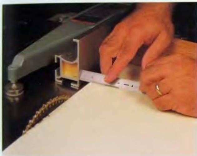
58. Use a scale to approximate the setting of the fence used as a stop.
