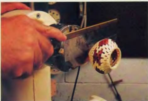
137. Use a handsaw with the lathe turned off to cut the tenon on the base.
