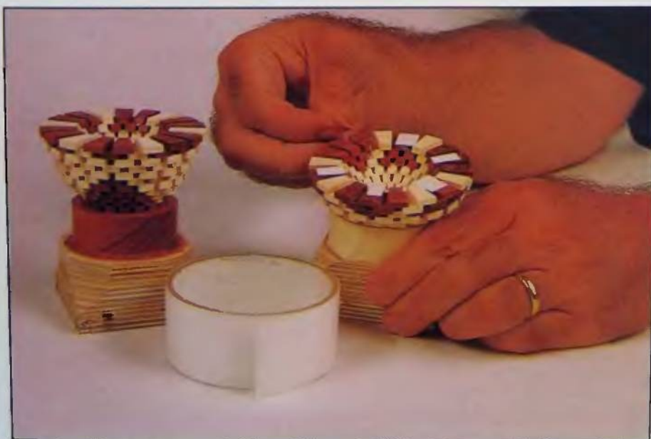
121. Four to six small pieces of indoor carpet tape will hold the two sections together. Note placement of the tape near the inside of the turning.
