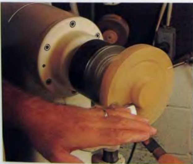
149. Make a facing cut in the area where the rim is to be glued. I use scrapers for this cut. A flat surface is a necessity for good glue joints.
