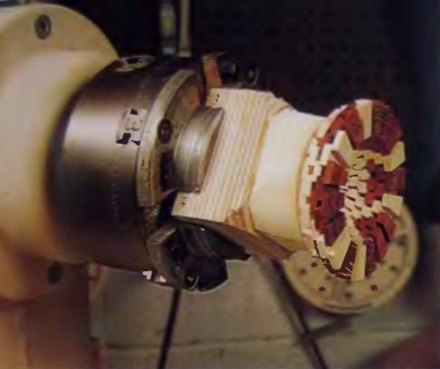
119. Build the top section from the rim piece down to the widest diameter.
