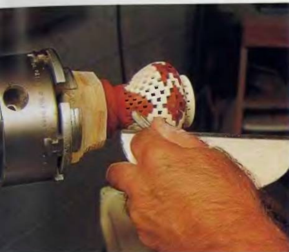
133. Cut away the excess wood on the lower three layers. The turning will be very delicate at this point.
