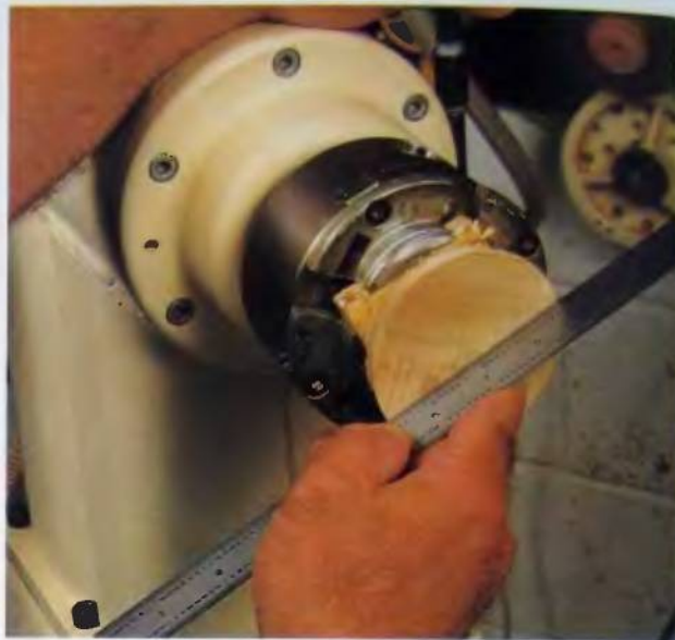
66. Use a straight edge to check for flatness and correct any unevenness.
