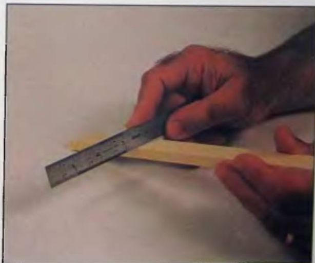
46. If you hand sand be sure you have not rounded over the surface of the strip. Use a straight edge to check for flatness. Do not use wood that has been rounded over as the glue joints will fail.
