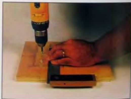
23. Attach the guide to the bottom of the base with two screws. The guide should be square with the edge of the base nearest the headstock.
