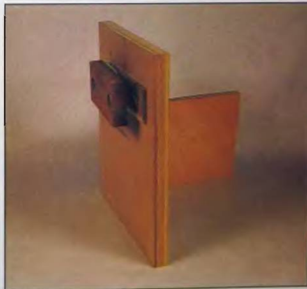
26. The clamp block attached to the positioning jig. In use, it goes under the ways and is used to clamp the jig to the ways.
