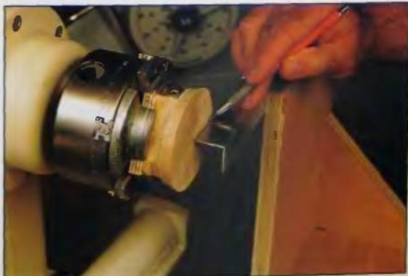
71. Clamp the positioning jig to the ways so the aluminum rail is about 1/8 inch from the base.
