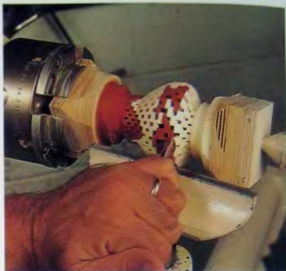
124. Use normal turning techniques to turn the outside, paying close attention to the final shape. Note the lower three layers have been left purposefully thick to provide strength during hollowing.
