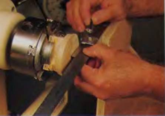
72. Place the stop at a distance from the rail edge of 1/2 of the diameter of the first layer. This would be 2-1/8 inches for the first layer of our project.
