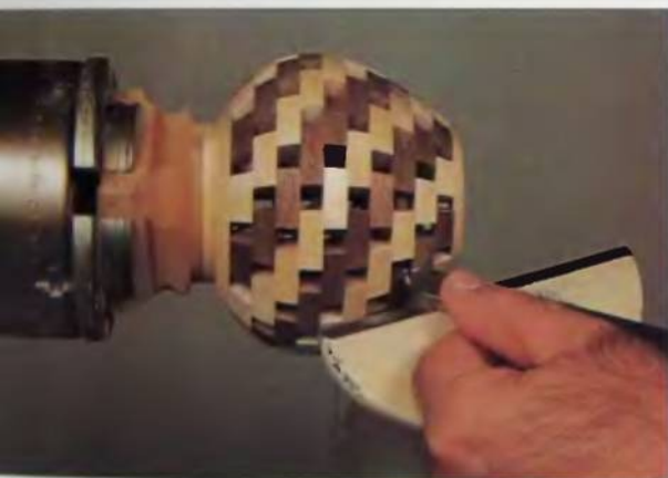
98. Use scrapers for finalizing the shape. Scrapers are very effective, as all cutting in this project is side grain with no end grain.
