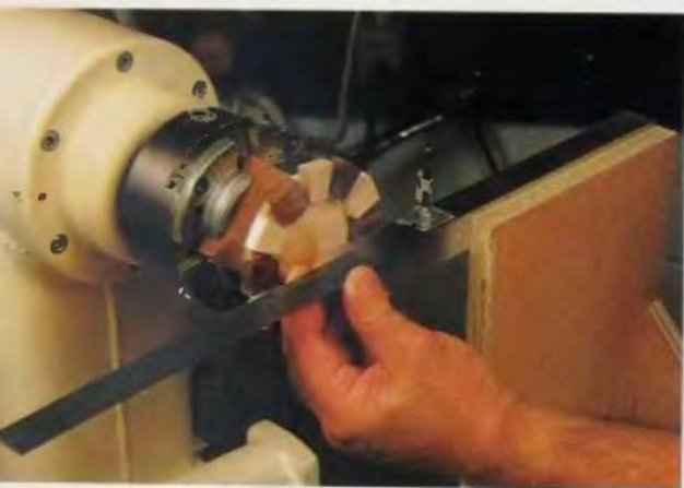
82. Adjust the stop to 1/2 the diameter of the second layer.
