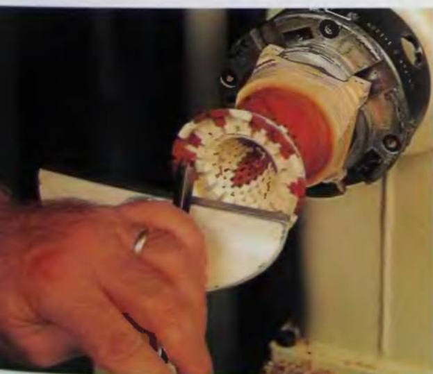
127. Turning the bottom is comparable to turning a small bowl. Pay attention to wall thickness as you go.
