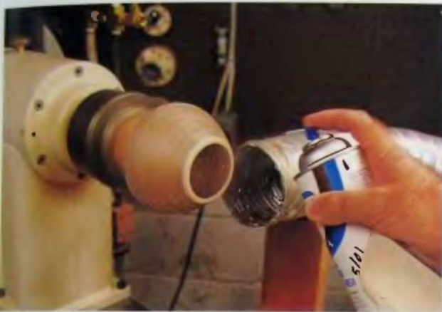
105. One or two shots of spray finish inside while the lathe is running will seal the interior. Excess will be thrown out the gaps so wipe the outside before it dries. Deft™ satin finish is one of my favorites.
