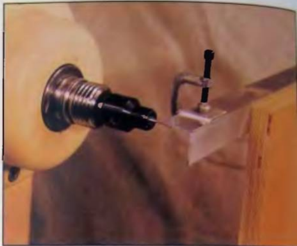
28. It is important that the leading edge of the rail align with the center line of the lathe. This is the only truly critical part of the jig construction.
