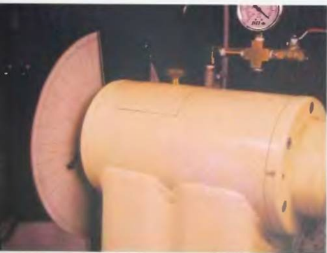
15. The finished degree wheel mounted on the lathe.
