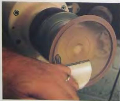
155. The top should be finished to the hub at this point.
