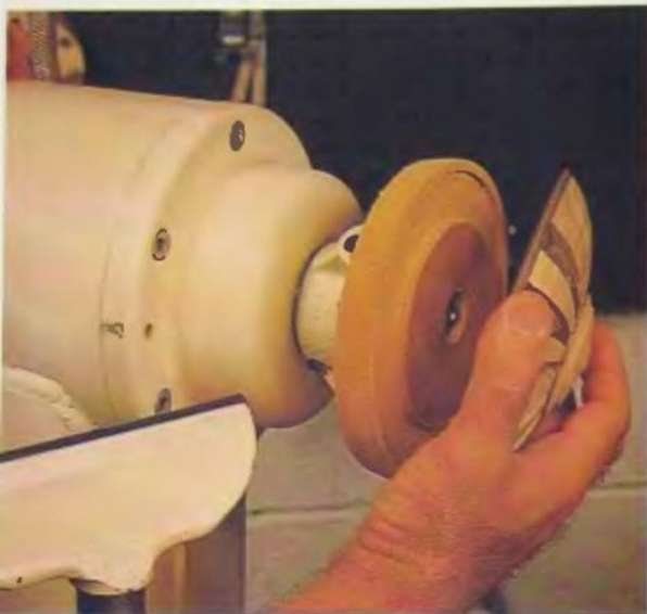
160. Use a jam chuck to remount the lid for work on the hub.
