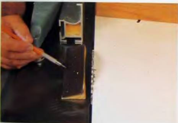
50. A magnetic strip from a sign company holds the ramp securely to the table saw.
