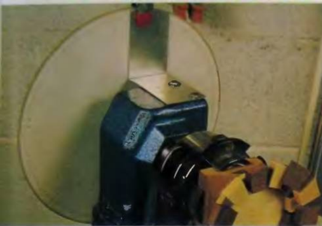
17. Aluminum pointer attached to the headstock on Vicmark minilathe with two machine screws.
