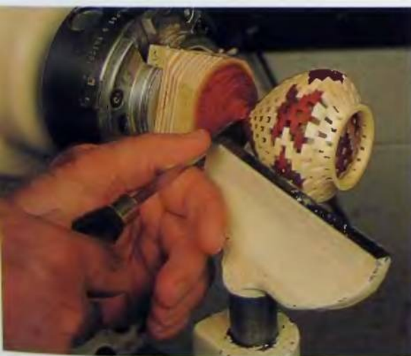
134. A small parting tool is used to define the bottom. This helps visualize the final shape.
