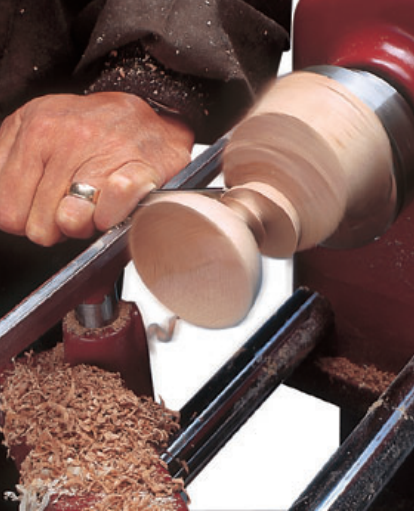
Turning a goblet with off-set stem using 0, 10 and 20mm settings.
