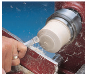
External shaping (Ref: 827H )
