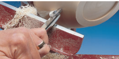
Use the straight edge for external work
