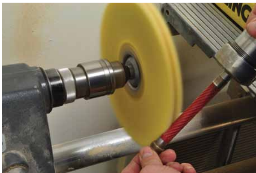
5. Angle the pen on the buffer so as to buff along the grooves and keep the ridges crisp.
