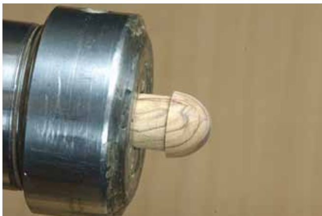
14. Reverse-chuck the finial to shape and finish it.
