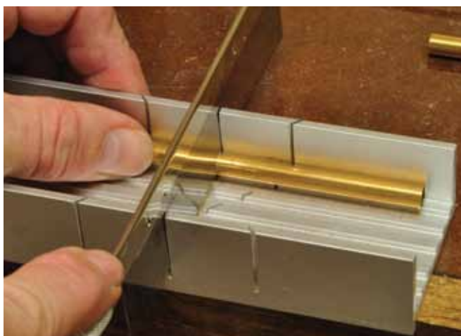
3. An X-acto miter box and saw can be used to cut brass tubes without damage.
