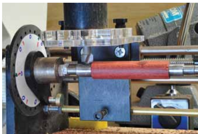
2. The cutter height is set to just above the bushing.
