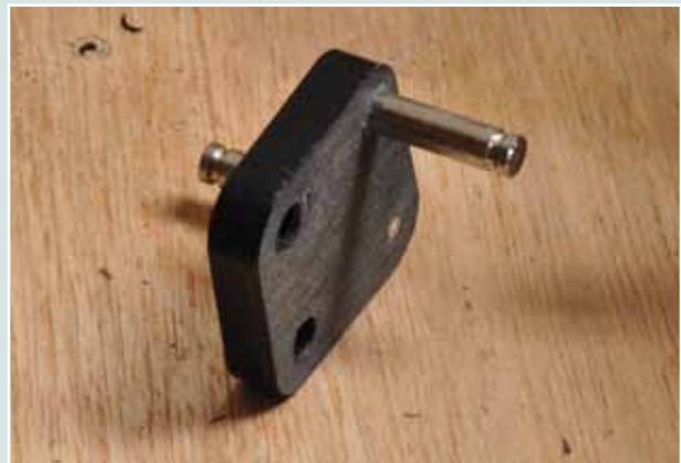
7. The reverse tumbler needs to have its shafts flipped.
