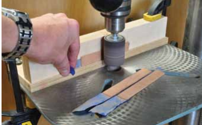
5. Use tape to pull the strips through the sander.
