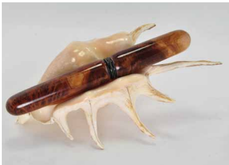
7. A large clipless, closed end pen, made using expansion mandrels.
