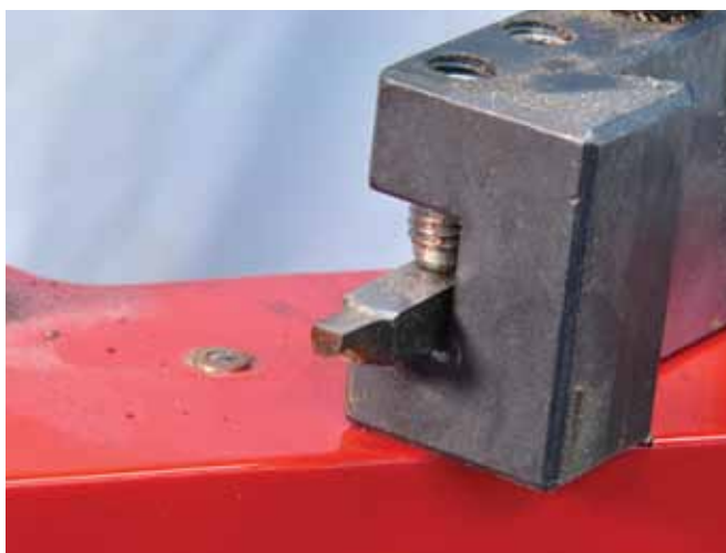
2. A specially ground tool bit for machining small recesses.
