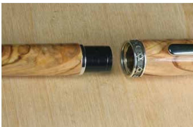
16. Mount the threads on the center coupling and epoxy them into the cap.
