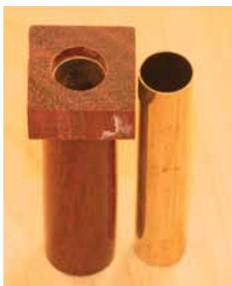
15. Add some of the same wood, beyond the brass tube end. Use the brass tube from another kit as a gauge to set the proper length.
