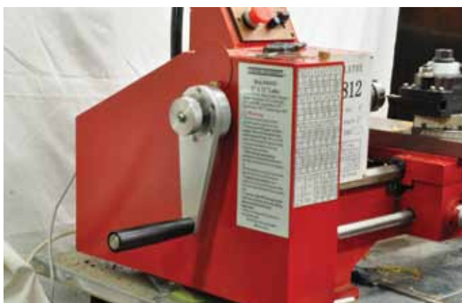
2. A hand crank is very useful for threading, unless the lathe has extremely low gearing.
