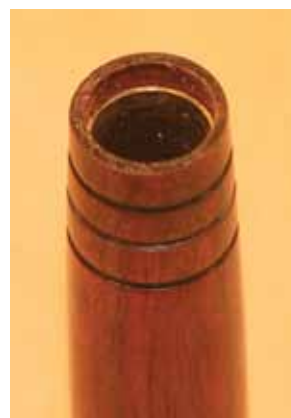
16. The new, longer tube, with wood extending beyond the brass tube.
