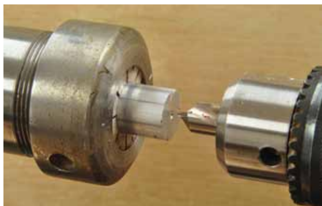
1. Center drill the aluminum blanks.
