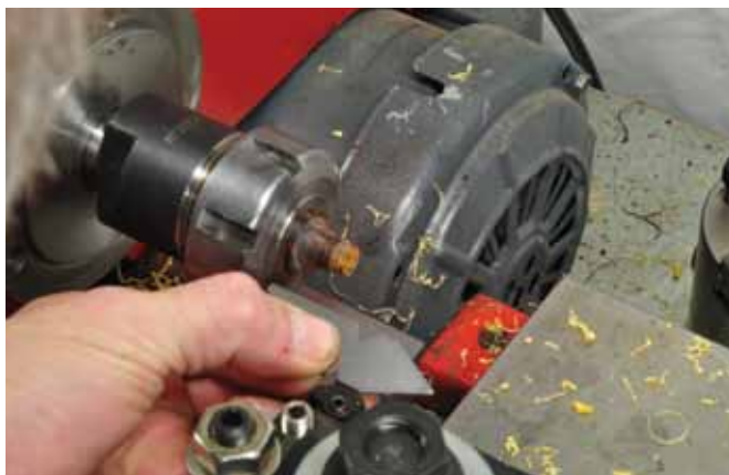
5. A fishtail gauge is used to set the thread cutter square to the lathe. When there is no long, straight section of the workpiece available, sight against the lathe bed.
