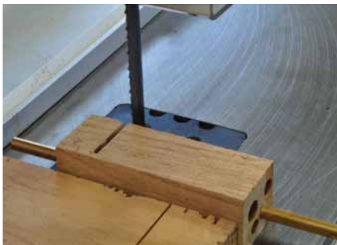
4. A wood block with a hole for the brass tube prevents the tube from collapsing when sawn on the band saw.
