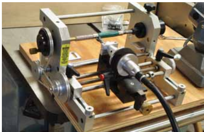
1. The MillLathe used belts to synchronize motions. An excellent tool, it is only available on the used tools market now.
