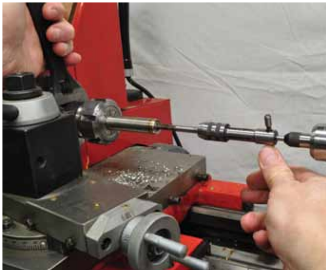
2. Use a tapping center to keep the tap straight.
