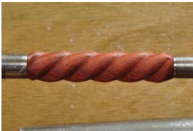
3. The ends are rounded down to the bushings.
