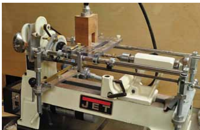
2. The Beall Lathe Wizard. This was a capable tool but is now only available on the used tools market.
