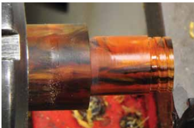
8. The first groove of a triple-lead thread is cut.
