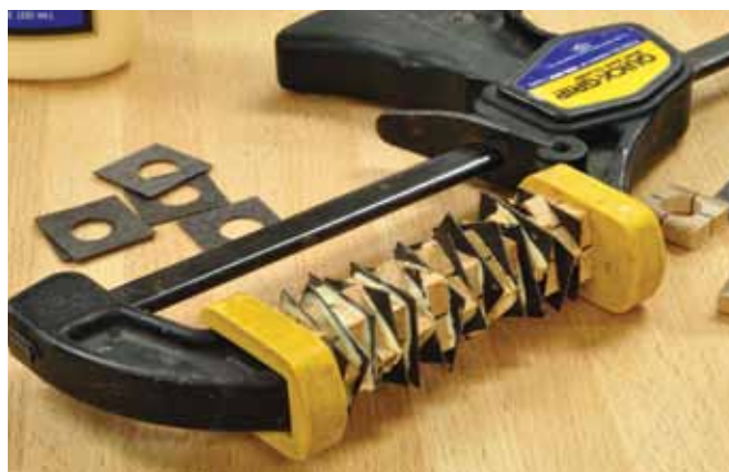
4. Stack the layers, over-filling the blank.
