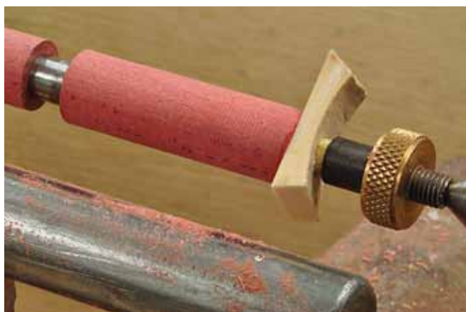
4. A piece of mammoth ivory, flattened on one side, is glued on as an accent.
