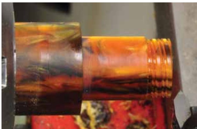
9. After moving the tool over exactly 1 pitch the second groove is cut.
