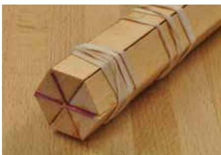
7. A hexagonal starting blank.
