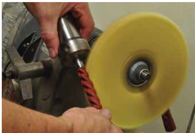
4. Buff with the pen angled so the wheel follows the twist direction.
