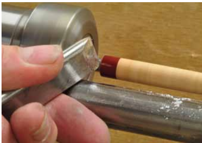
6. Square the center band with the long point of the skew.
