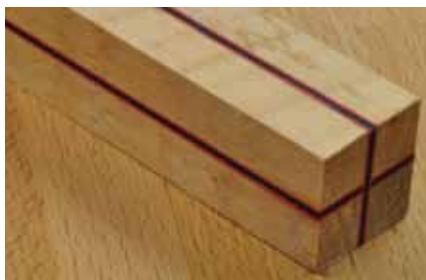
1. Sandwiching some veneers into a blank makes a good starting blank for a segmented pen.
