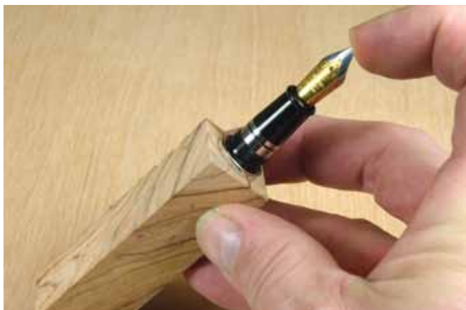
5. Test the depth of the main body bore with the assembled section, trim ring, and conversion pump.
