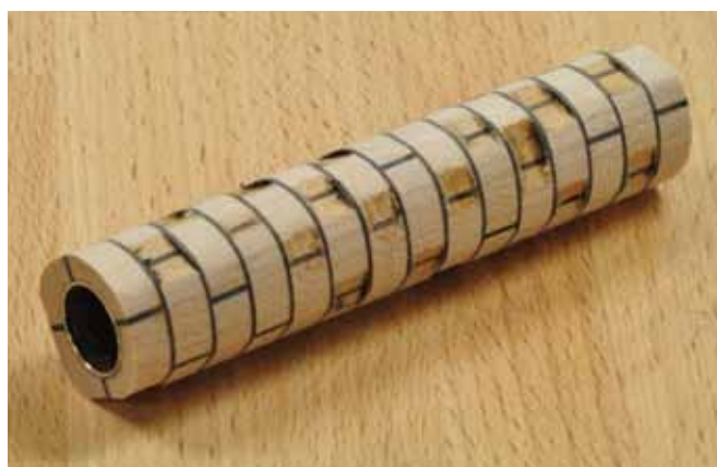
6. If you knock the corners off on a belt sander it is easier to begin turning.
