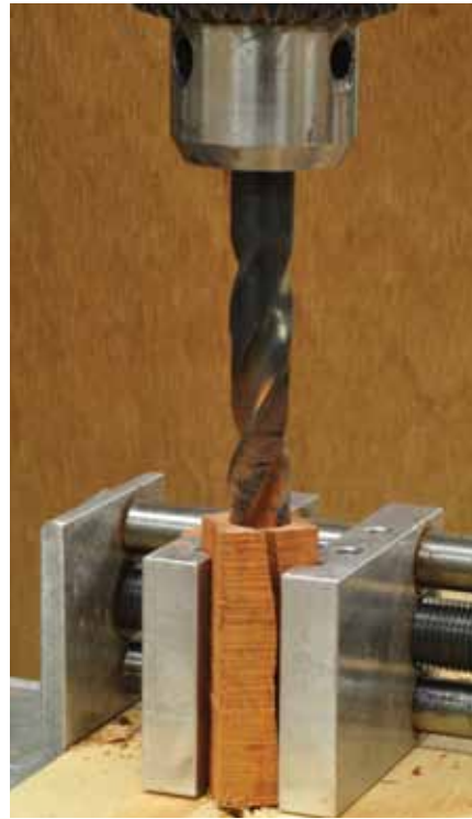
1. Drilling blowouts frequently happen when the bit exits the blank.
