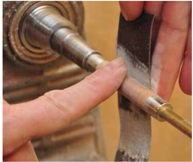
11. Hold the sand paper behind the blank to let the dust fall away.
