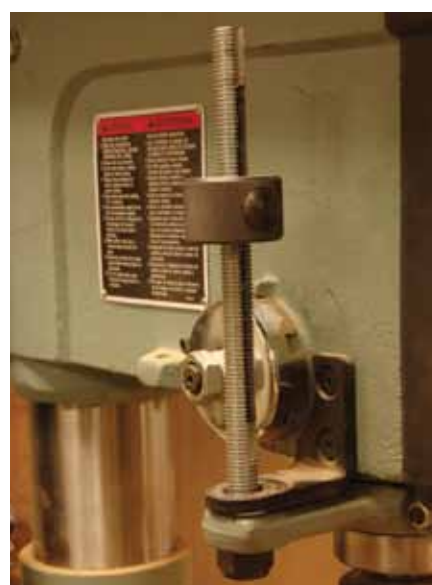
3. A rod-type depth stop has some advantages.
