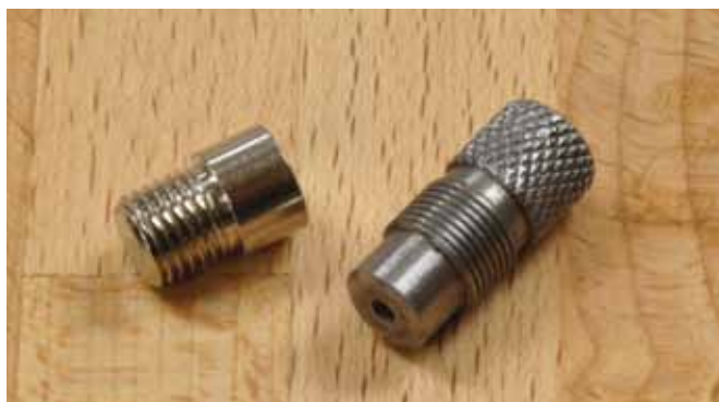
18. A commercial knock-out plug next to a homemade one.
