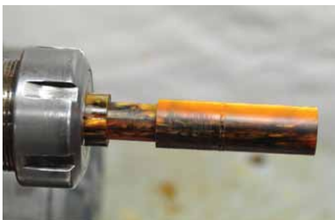
12. A test fit verifies a good thread. The carriage should remain engaged to the lead screw.
