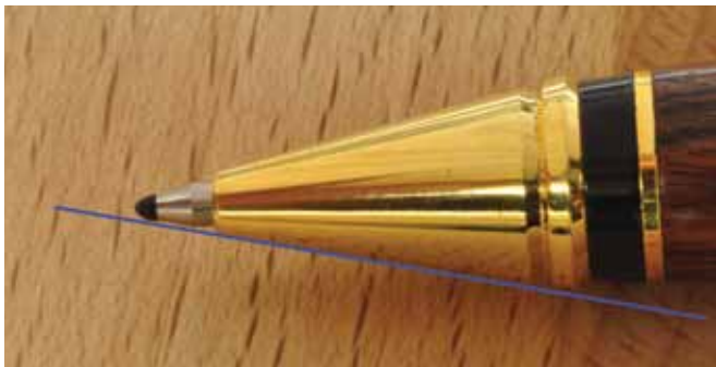
8. Proper ballpoint tip extension.
