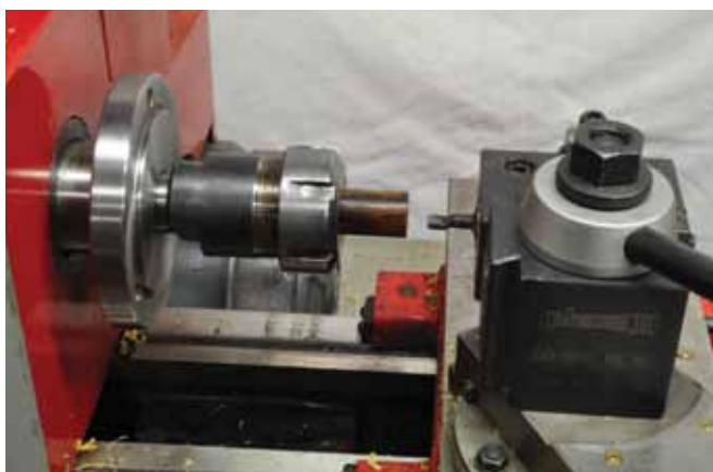
14. A boring bar is used to cut a recess for the center band fitting.
