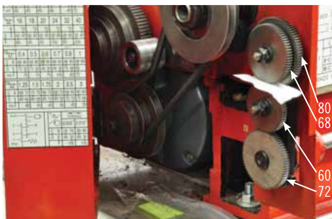
4. Change gears are used to set up the metric thread on the imperial lathe. The temporary piece of typing paper between the gears is a convenient way to set the proper clearance.
