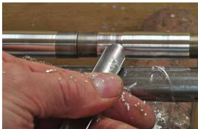
3. The \frac{1}{2} " gouge works quickly on aluminum.
