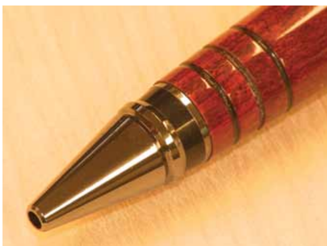
15. Add some of the same wood, beyond the brass tube end. Use the brass tube from another kit as a gauge to set the proper length.
