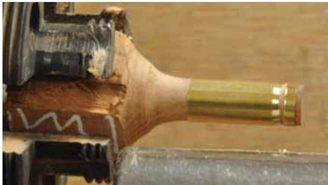
11. Turn a dowel to fit inside a brass tube. Proceed to part off a narrow ring.
