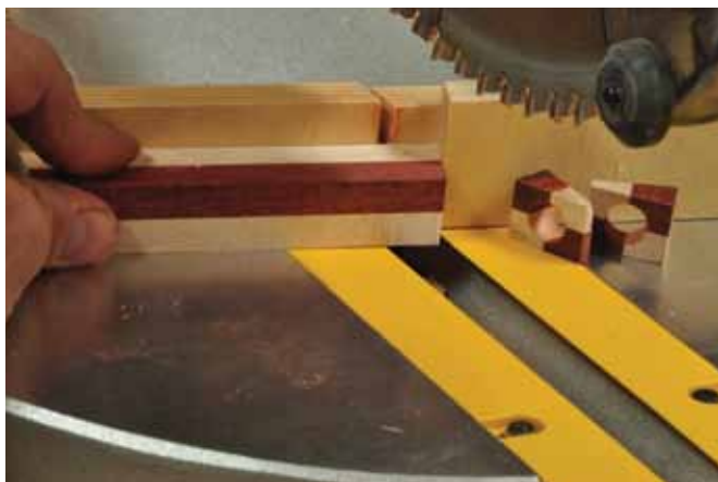
3. Cutting wedges on the chop saw.
