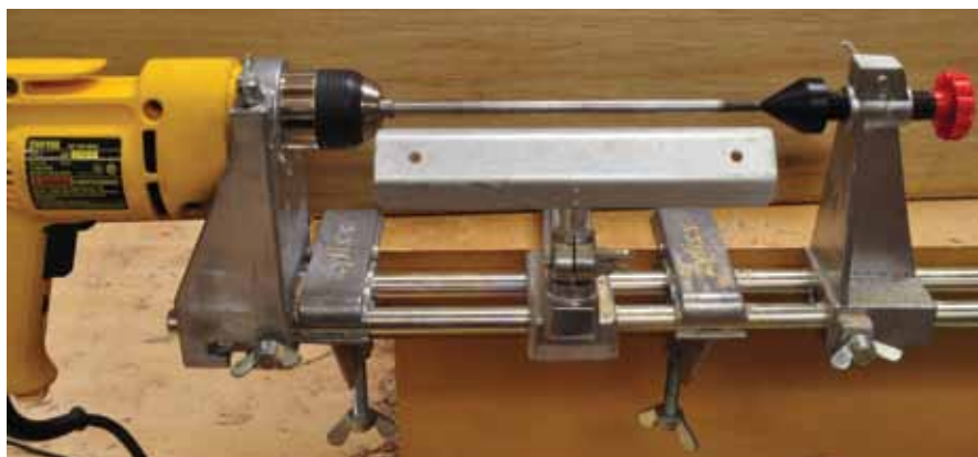
1. Drill-driven jigs can be used but it is difficult to produce a good pen on one of these.
