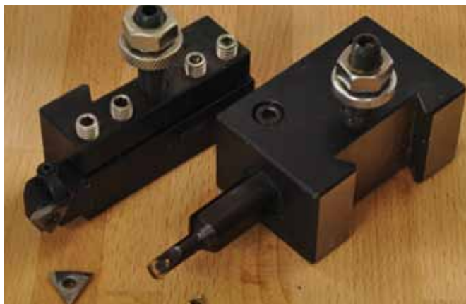
1. Threading tools. The interior tool can be used for exterior threads also, but working on the backside of the lathe.
