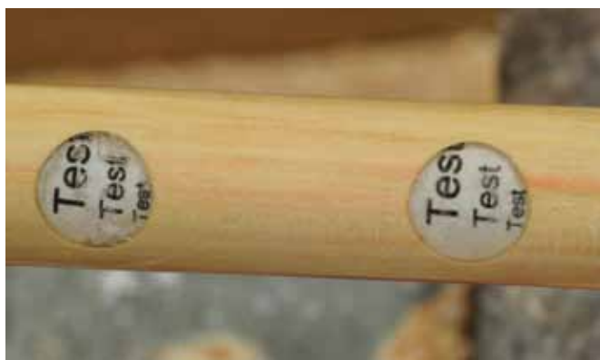
5. After polishing it is clear, the epoxy fill works much better.
