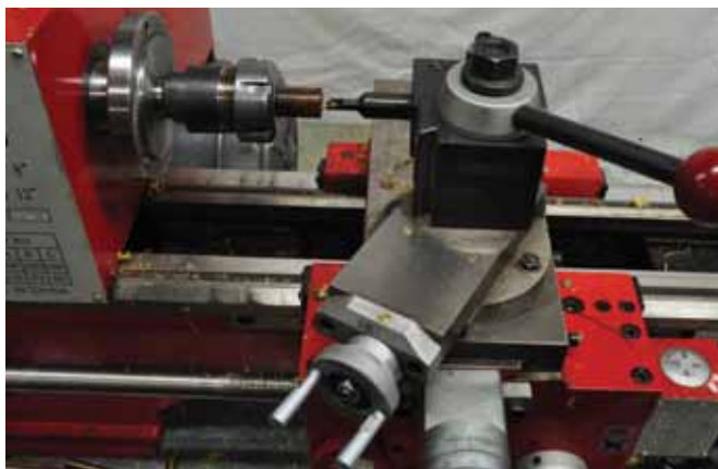
11. The interior threading tool ready for use. Notice the compound is swung 29.5 degrees to the left for the proper feed.
