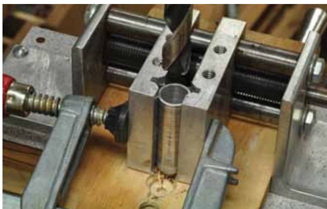
2. Drilling the cap barrel.
