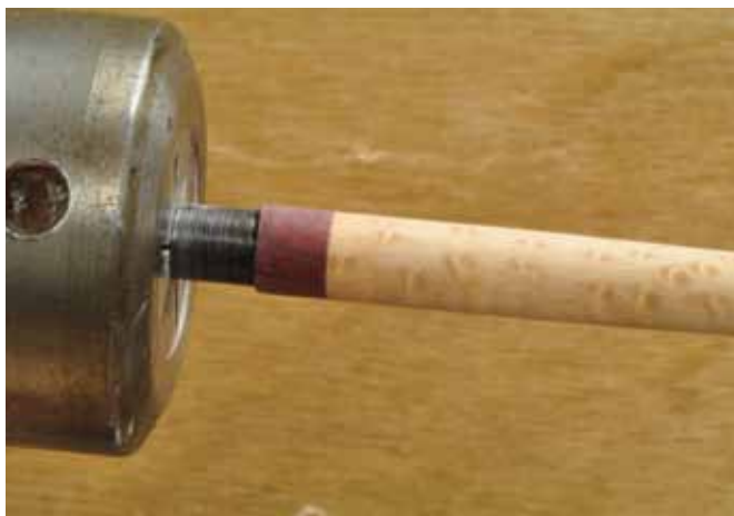
4. An integral center band is added.
