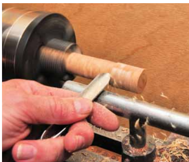
2. Pre-rounding a blank in a four jaw chuck.
