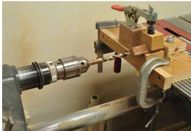
5. A shopmade drilling jig for a Shopsmith.
