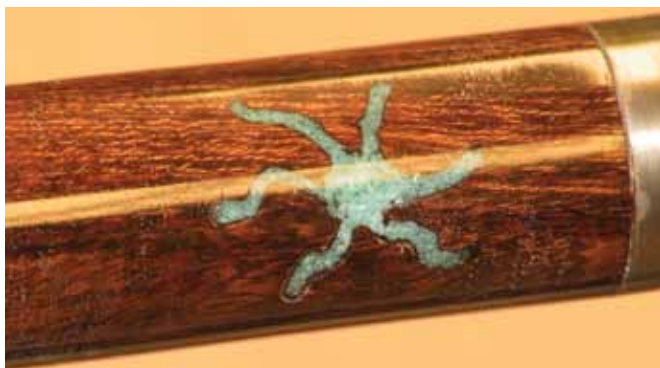
3. This little critter once was a accidental hole. Enlarged and filled with crushed stone it adds something unique to the pen.
