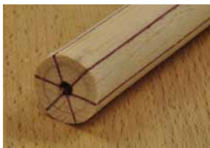
8. The hexagonal glue-up after turning round.
