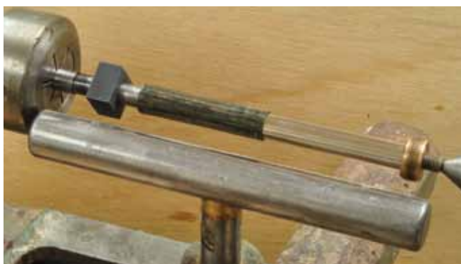
4. Use filler pieces to mount a single center band on a mandrel.
