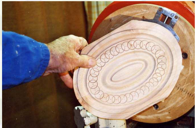
Figure 6306 Lid of a chip box with 32 equally spaced circles forming the Barley-Corn-Pattern (Workshop J. Volmer, Chemnitz 2003)
