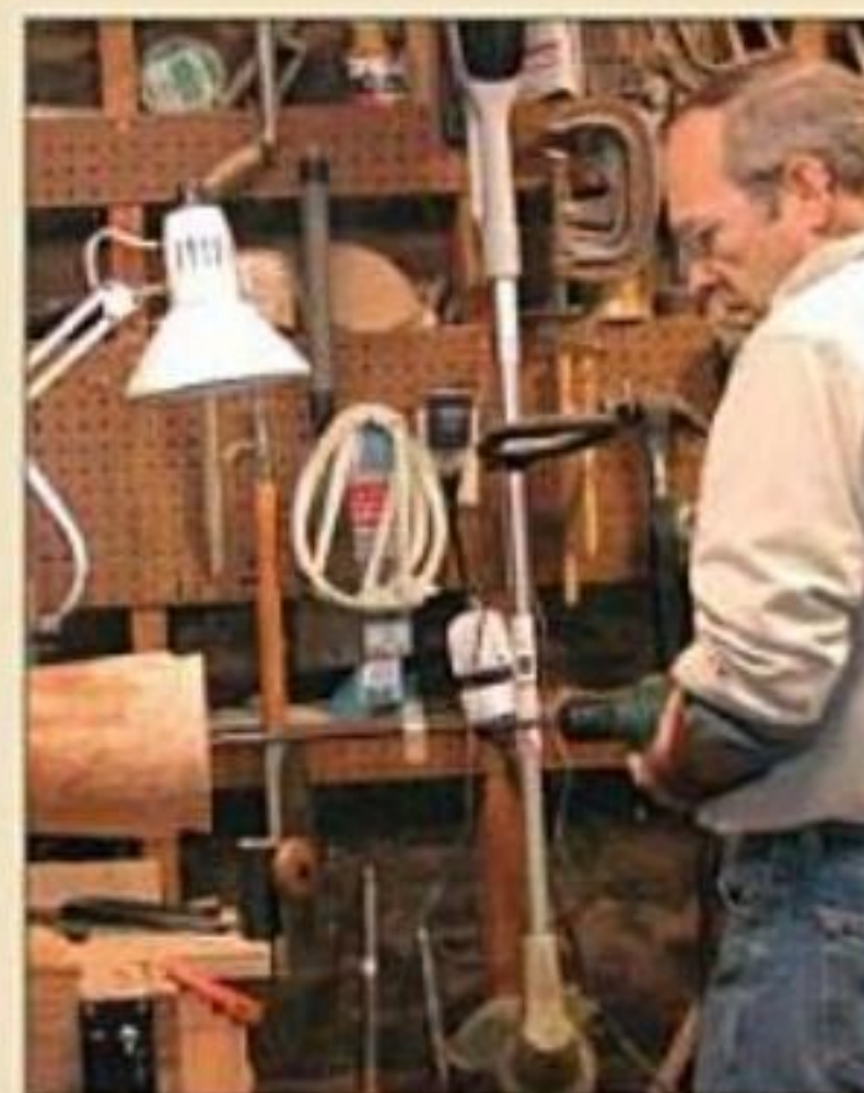
Garrett bores a center hole, to begin turning the inside of the palm block and also to gauge its depth.
