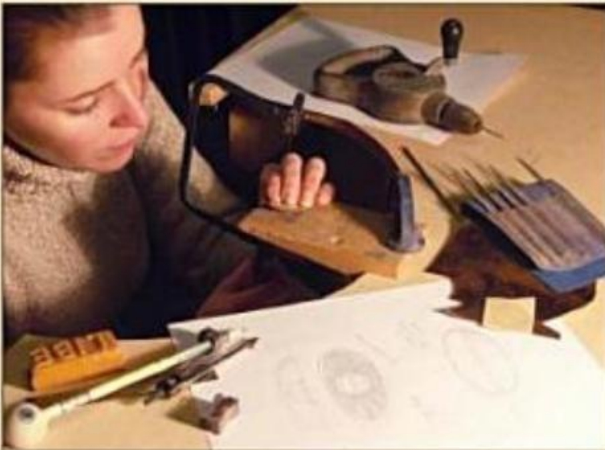
She uses a jeweler's saw to cut tiny wood and metal inlays.
