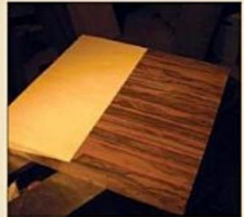
Mode machines a long bevel on the blank, and glues on a wedge of light-colored wood.
