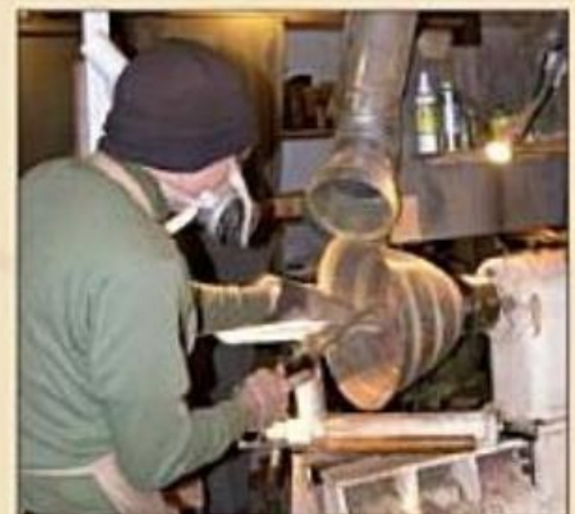
Mode mounts the stacked blank on the lathe and refines the bowl.
