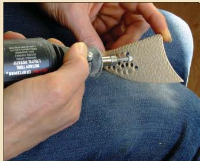
After turning, Campbell removes the thin skin from the mold and cuts, shapes, textures and pierces it to create the overlay components.
