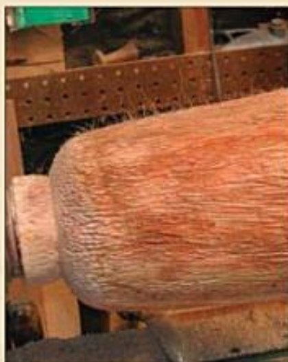
Garrett works over the palm wood with a stiff wire brush, creating the rough texture he prefers.
