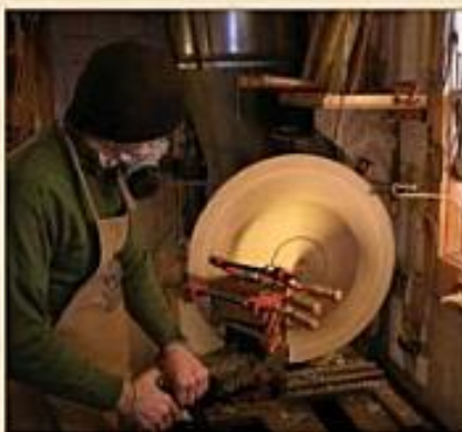
Mode goes to the lathe to cut the disk into a series of concentric rings with sloping sides.
