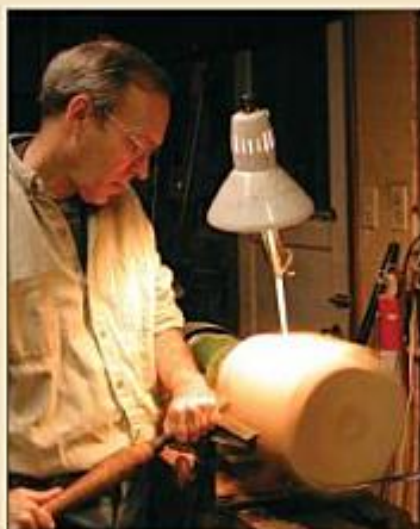
Conventional turning converts the palm block into a vessel form.
