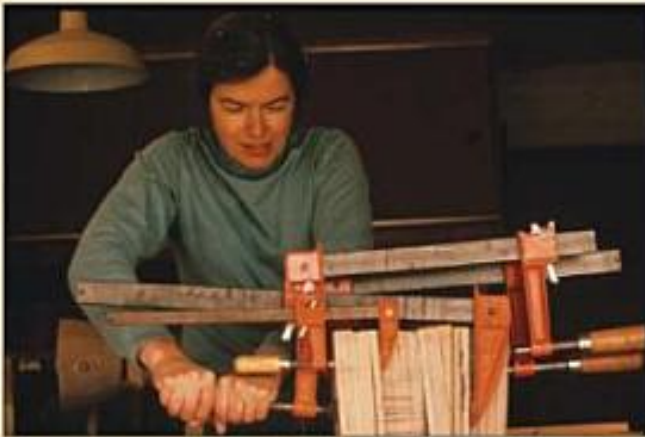
Dotson prepares a turning blank by gluing layers of plywood together. She visualizes how the turning is to look when done, and inserts wedge-shaped layers accordingly.
