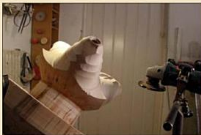
Hromek continues to shape the wood using a power carving tool mounted on the lathe's tool post, at right, while he slowly rotates the workpiece by hand. He's left lots of wood opposite the lobes for later shaping to form the lips around the vessel's finished opening.
