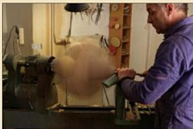
Hromek hollows out the new section with a gouge. You can see in the whirling wood a shadow view of the final shape of this part of the vessel.
