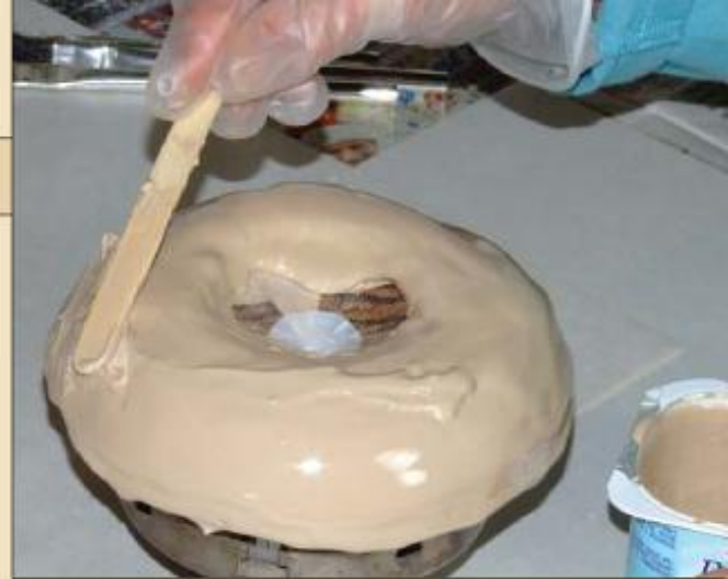
To make the overlay, Campbell uses the turning itself as a mold, spreading on an epoxy mixture, which, when cured, she will turn down to a thin skin.
