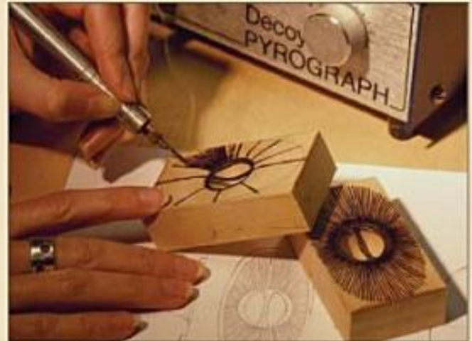
A pyrography machine allows Hibbert to burn small details into the wood.
