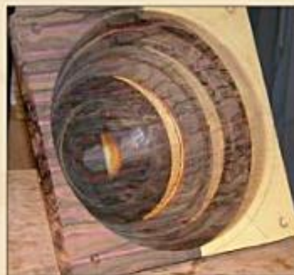
He stacks the rings and glues them into a bowl-shaped blank with the center already hollowed.
