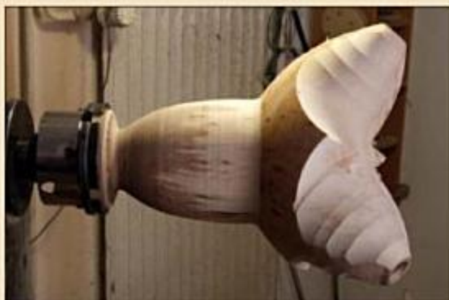
With the piece remounted on its central spigot, Hromek turns the final shape of the base. After refining the details by carving, Hromek sets the piece aside so the wood can dry out, after which he will complete the carving. The walls are about 1/4" thick.
