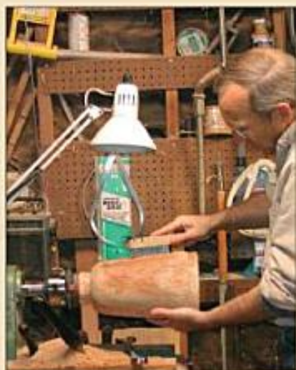
Garrett works over the palm wood with a stiff wire brush, creating the rough texture he prefers.
