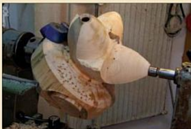
The artist repeats the process twice more and the three-lobed shape begins to emerge. When all of the insides have been hollowed, he turns the outside of each with support from the lathe's tailstock (right).
