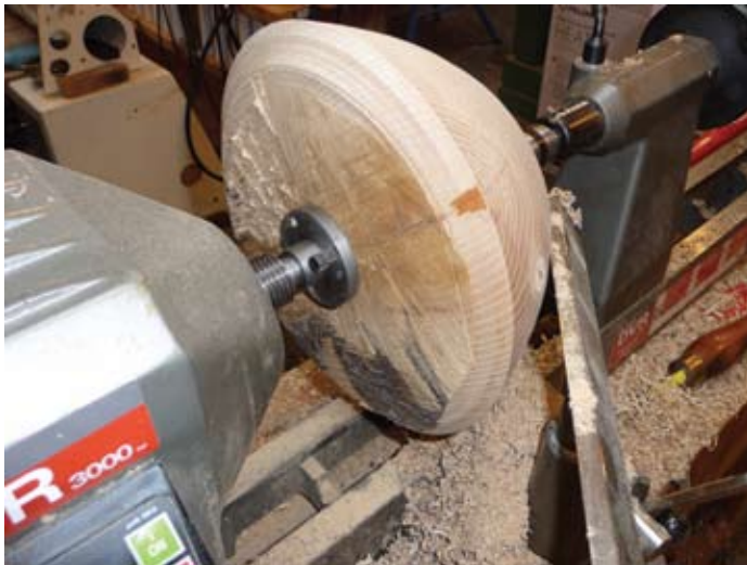
Figure 4. This shows the mounting used while turning the outside of the bowl to shape.
