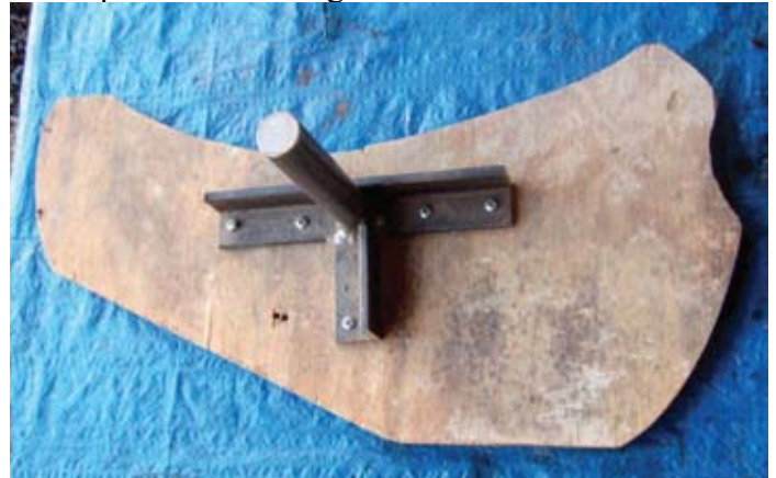
Figure 2. Platform that Author build to use during fluting.
