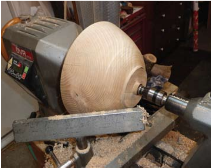
Figure 3. Outside of bowl turned between centers.
