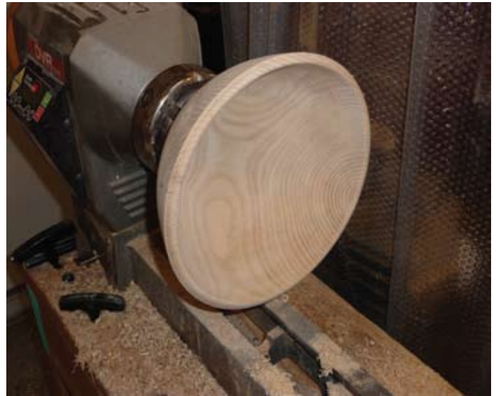
Figure 5. Bowl has been fully turned and is now ready to be reversed to final turn the foot.
