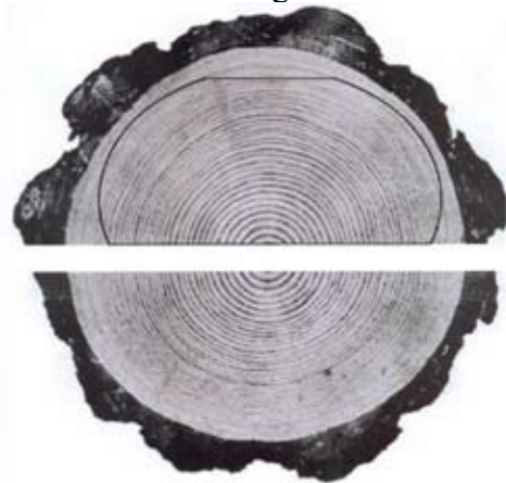
Figure 2. Layout of a normal bowl on the end grain portion of the half log.
