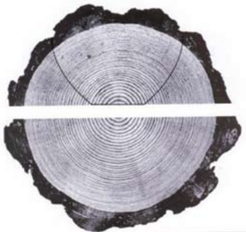
Figure 4. Layout of a natural edge bowl on the end grain portion of the half log.
