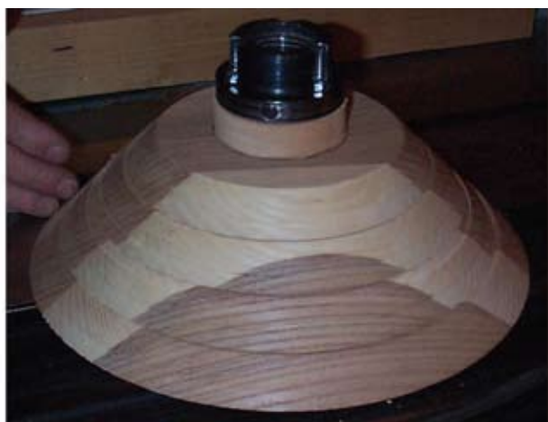
Figure 6. This photo shows a faceplate mounted to a glue block, which is glued directly to the bowl blank.
