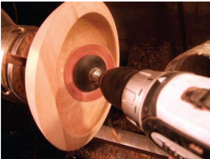
Figure 1. Sanding the inside of the bowl before beginning the fluting.
