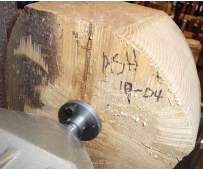
Figure 4. A larger view of the faceplate mounting on the Ash blank that I was using. This was very dry and extremely hard.
