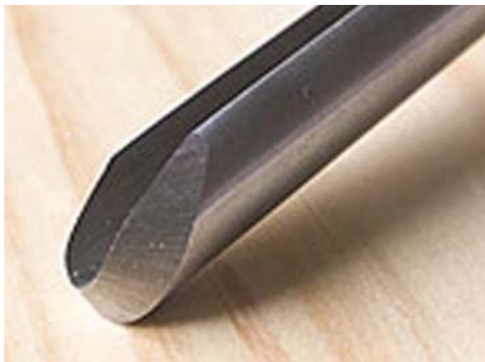
Figure 7. Ellsworth Grind on 5/8" bowl gouge.
