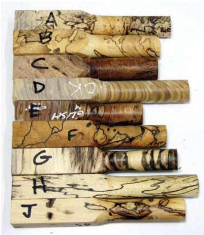
Figure 3. This photo shows the blanks from Figure 2 after turning half of the blank round.
