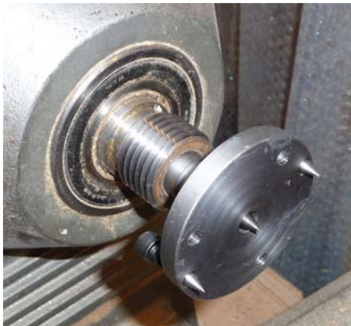
Figure 2. The Elio Drive mounted in the spindle Morse taper of my Nova DVR lathe.
