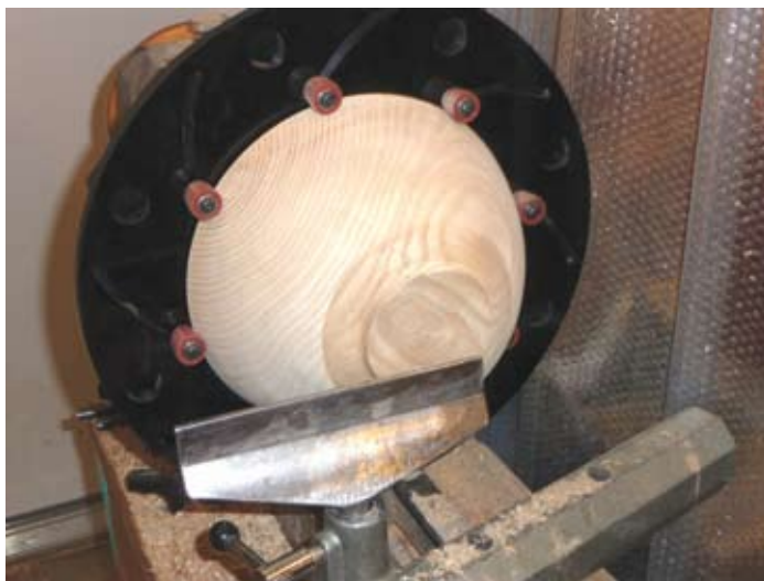
Figure 7. The bowl foot has been final turned at this point.
