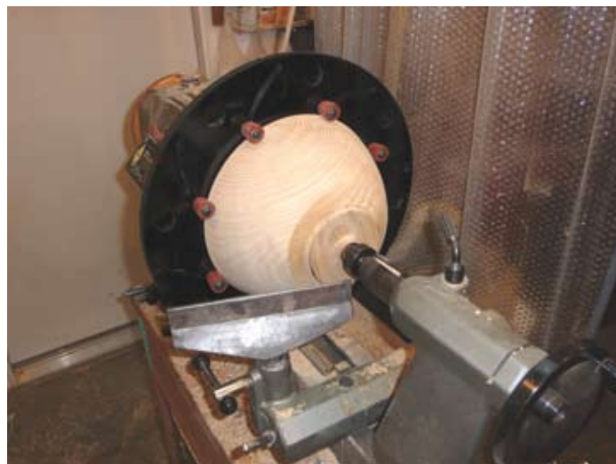
Figure 6. Bowl mounted in the Longworth Chuck and additionally supported by the live center in the tailstock.
