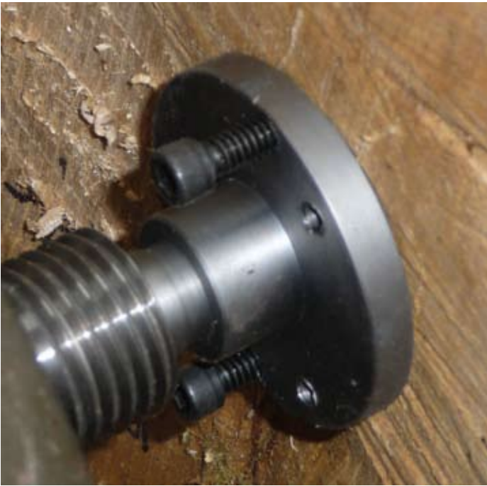
Figure 3. This picture shows the Elio Drive mounted against the bowl blank that I was using for a test.
