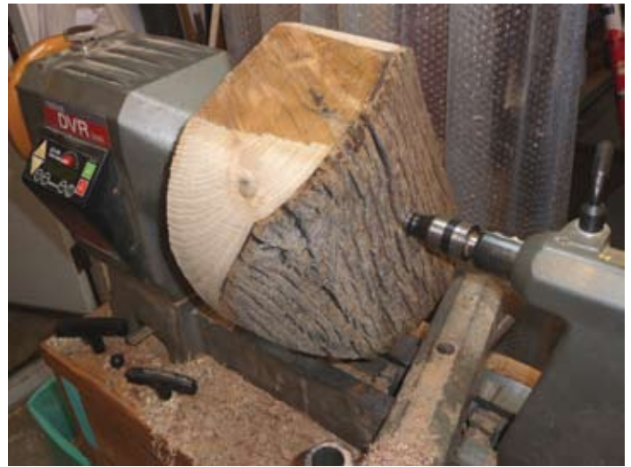
Figure 5. This photo shows the tailstock mounting.
