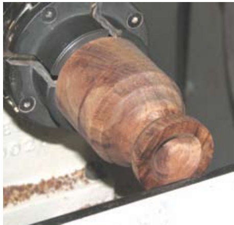
Figure 9. Central depression is turned to 15/16 inch deep.
