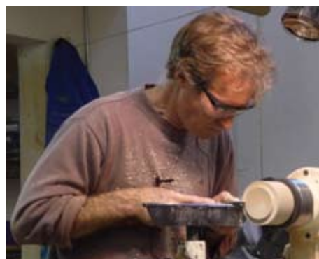
Figure 10. Matthew is turning the tenon on the lid to fit the bottom portion of the box. Since he has already final turned the bottom of the box, this tenon does not need to be a tight fit. Once the tenon to fit the bottom portion of the box has been completed, Matthew began to shape the top of the lid.
