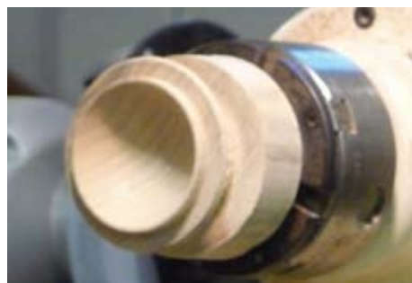
Figure 12. The hollowed lid is as smooth as Matthew makes the insides of his boxes. He turns them very smooth and does not sand.
