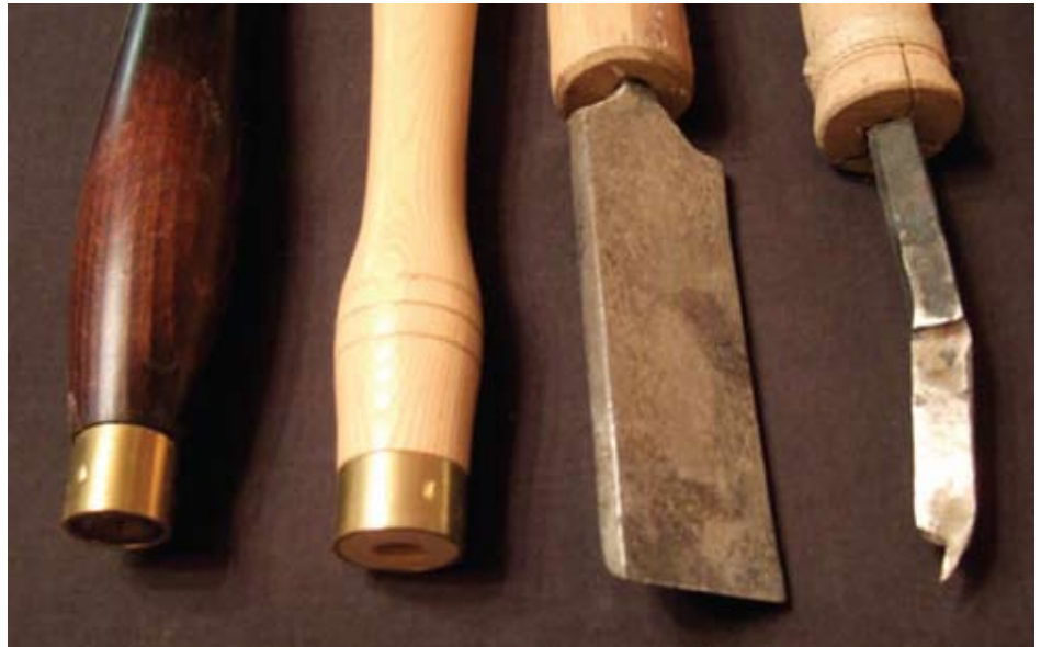
Figure 1. This photo shows 4 tools; the left two are commercial handles; note the tubings used and dimples to keep the ferrules in place. The wide scraper in an oak handle uses no ferrule, and the little hook tool, forged and ground from a stone chisel, shows a split handle "saved" by a string ferrule superglued (desperate maneuver, but still working after many years).
