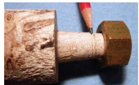
Figure 3. When the nut has been screwed on finger tight it leaves marks as shown by the pencil point.
