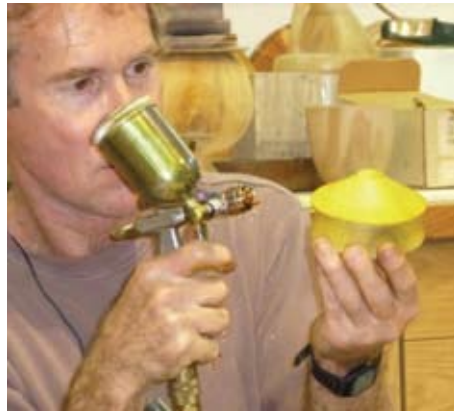
Figure 24. At this point, Matthew had shifted to the dying process using dye sprayed onto the surface of the item. Here he is spraying yellow dye on first. He later followed with red and black.
