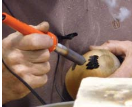
Figure 17. Here Matthew is doing some texturing on a sample piece. This tip burns a shape that look something like this ( ) with the top and bottom coming to a point.
