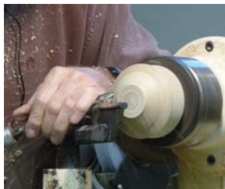
Figure 13. With the lid fitted into its jam fit chuck, Matthew final shapes the top of the lid. The pencil mark near the center is the size to which the lid top will be turned.
