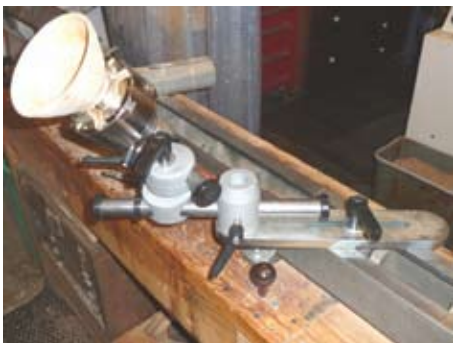
The Vermec Carving Mount fitted to my Nova DVR Lathe. The mounted bowl is being held with the Vermec chuck.
