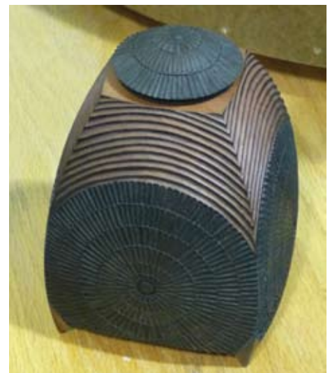
Figure 28. This photo is a close up of a vessel that was turned square on a rig that Matthew had made up to allow him to turn it square.
