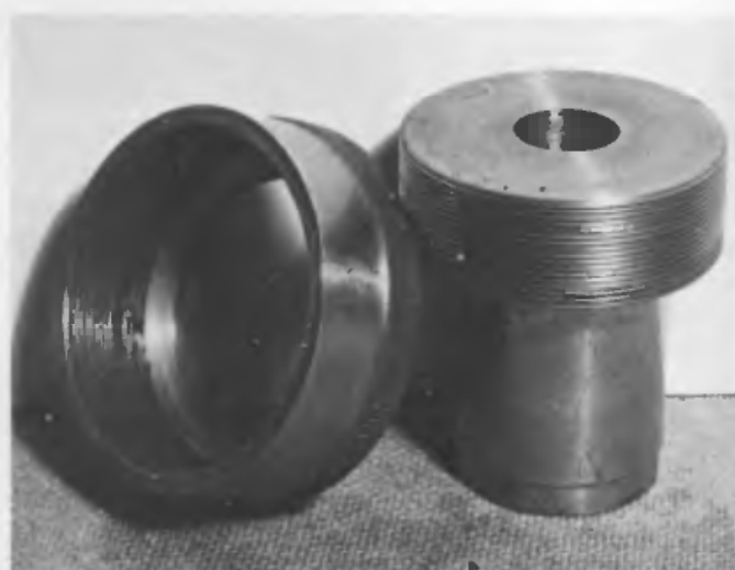
Fig. 31 Special chuck which can be made easily by a metal worker for holding blanks for egg cups. These must first be turned to a cylinder with a flange at the bottom to fit the flange in the chuck
