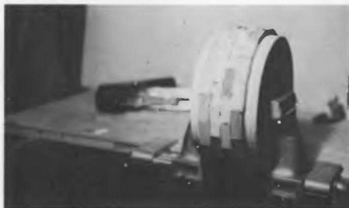
Fig. 21 Built-up assembly cramped in a vice between two pieces of ply while the glue sets
