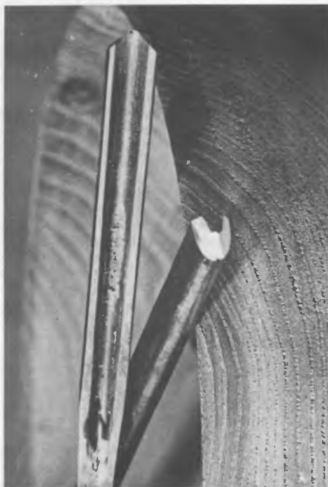
Fig. 10 A good example of roughness across the grain on elm, and two very sharp gouges which will be used to remove it
