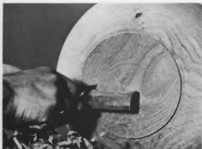
Fig. 3 Marking concentric circles on the base of a bowl, in preparation for reversing it on the faceplate
