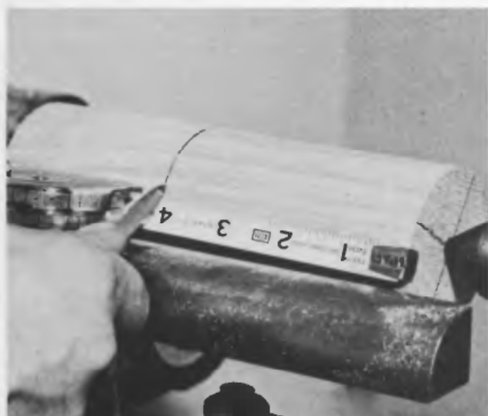
Fig. 17 Marking off with a pencil 4 in. [101.6 mm.] along from the end of the blank before parting through to separate cap and body
