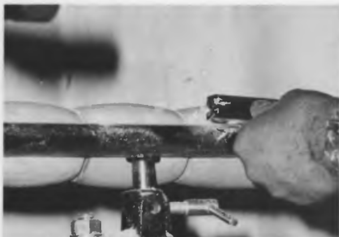
C Parting tool cuts have been made to separate the barrel sections, leaving enough wood to keep the work steady. Here the shaping is being done with a 2in. skew chisel
