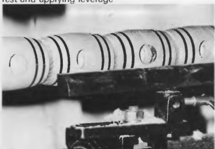
D Burning on the 'hoops'. This is done by forcing the tang of a file or old scraper between work and rest and applying leverage
