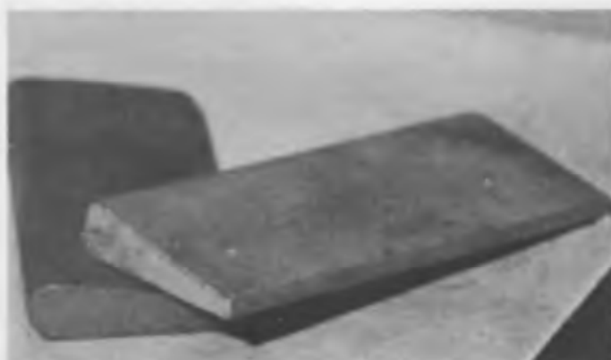
Fig. 5 Two small oilstone slips, which are most useful. One is kept for gouges and scrapers, the other for chisels
