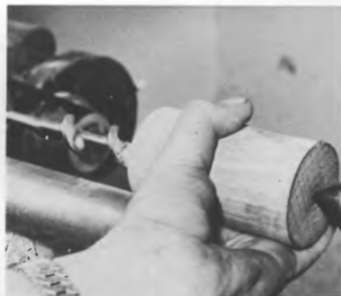
Fig. 18 Boring \frac{5}{8} in. [15.9 mm.] deep into the bottom of the body section with a 1 in. [25.4 mm.] drill
