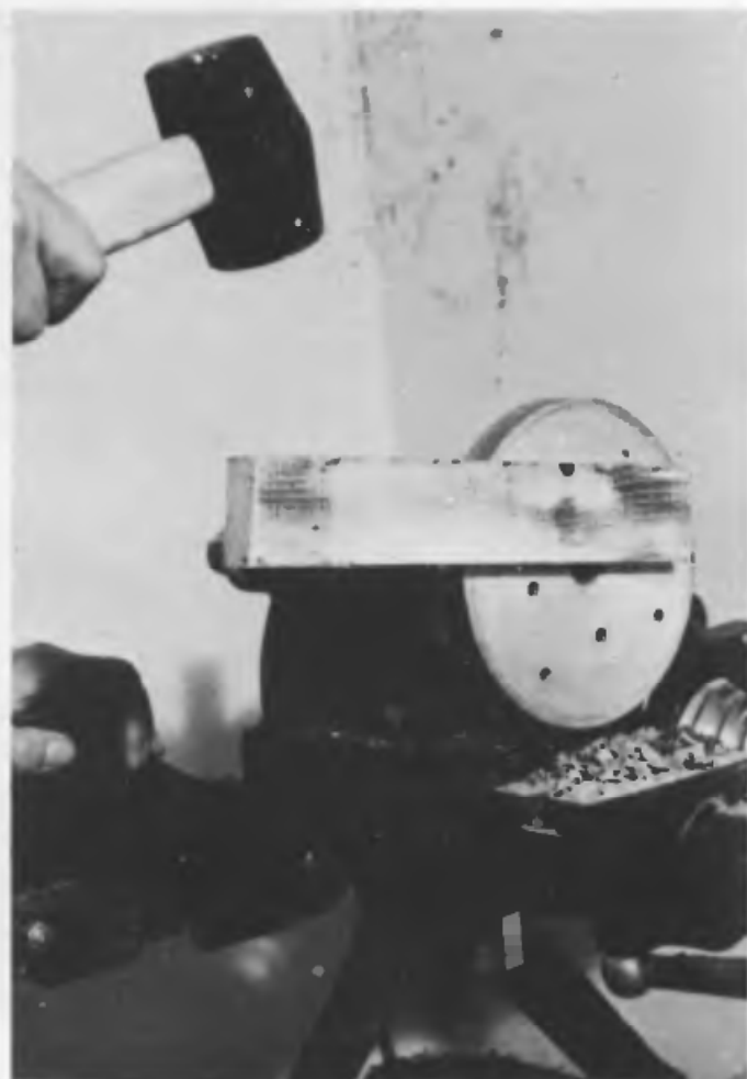
Fig. 8 Removing a jammed faceplate by striking a batten which has been screwed to it
