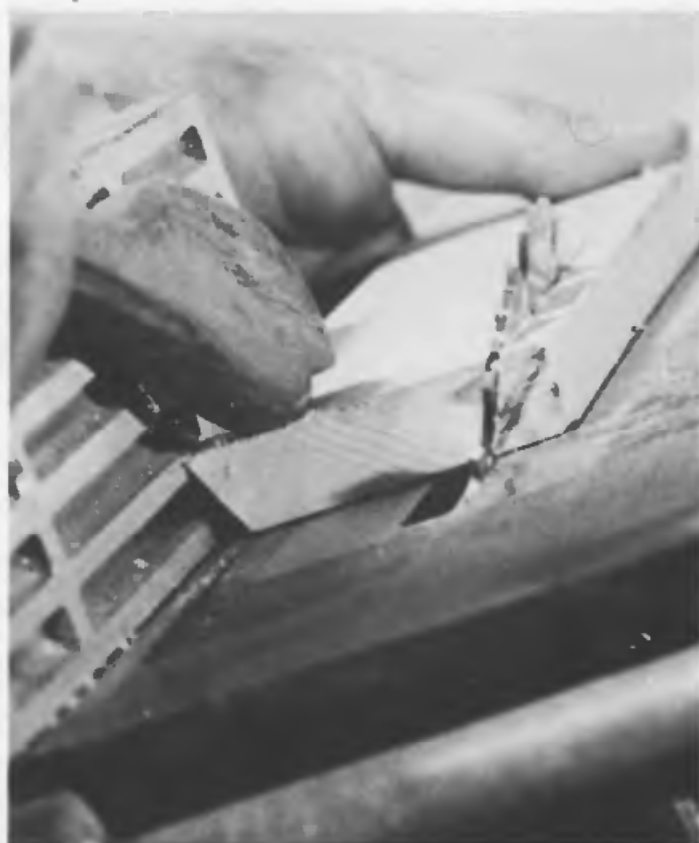
Fig. 3 Bevel ripping the staves for coopered blanks, on a sawtable which has been tilted to the required angle. A push stick must be used, and the guard has been removed purely for clarity
