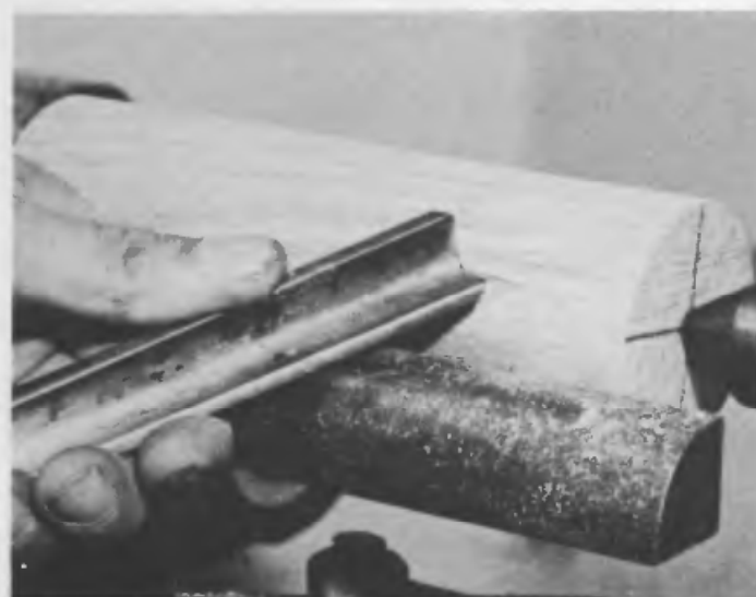
Fig. 15 Running the blank down to a cylinder for making a pepper mill. Note how roughing gouge is held
