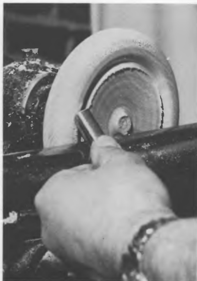
Fig. 29 Shaping the ring, with a \frac{3}{8} in. [9.5mm.] gouge on its side
