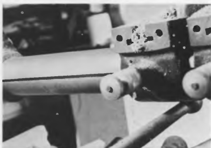
Fig. 16 Showing the solid steel lathe bed bar, and the slot which accepts the spring-loaded plungers of saddles and tailstock
