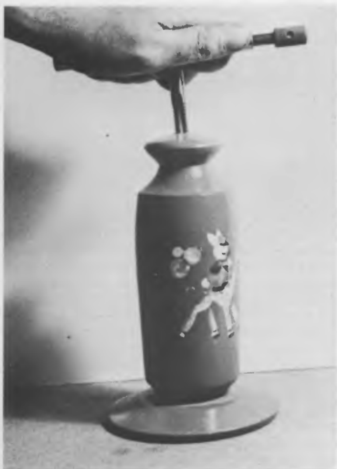
Fig. 14 A \frac{3}{8} in. [9.5mm.] Whitworth tap being used in a lamp to take the brass fitting
