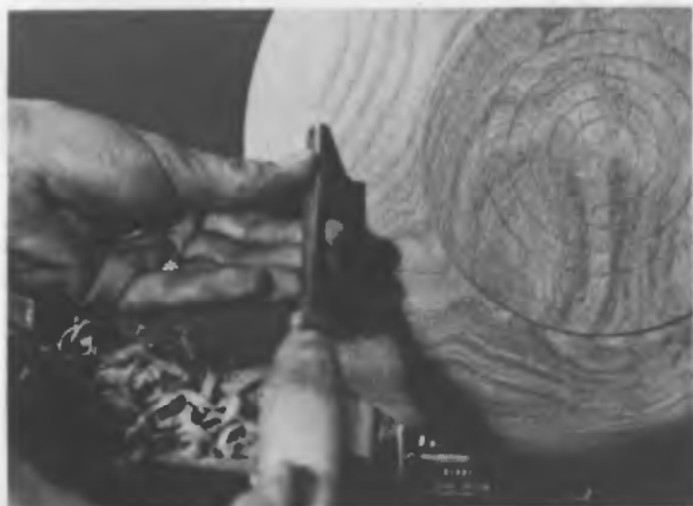
Fig. 9 A \frac{1}{4} in. [6.4mm.] gouge being used for final cuts on the outside of a bowl blank, to remove roughness on the end grain. The bevel must rub
