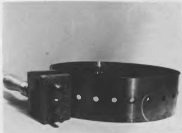
Fig. 15 A cramp, such as the Flexicramp , is useful for clamping bowls built up by the brick method
