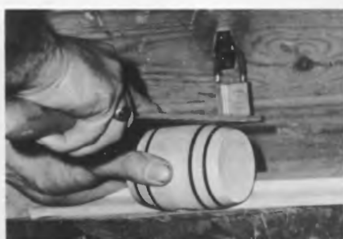
G Filing two flats in readiness for the fitting of the feet. This can be done better with the aid of some simple form of jig
