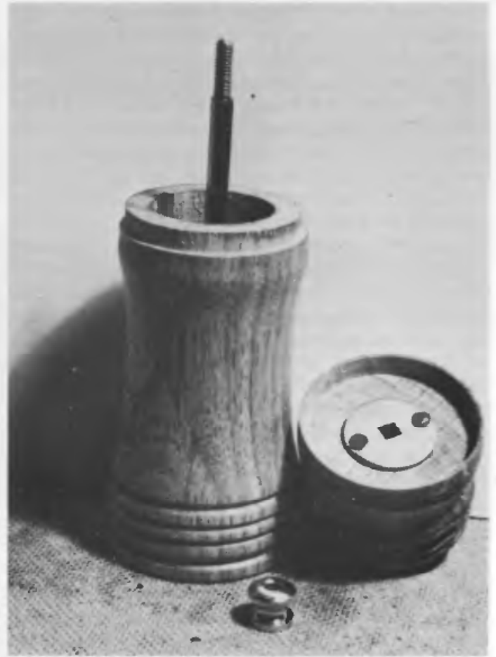
Fig. 22 The small metal disc has been fitted inside the lid. Note the square hole which turns the shaft when the top is revolved
