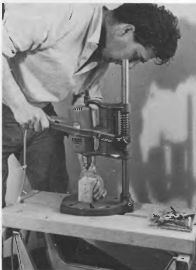
Fig. 32 Pre-drilling with a \frac{1}{16} in. [1.6mm.] drill on egg cup blocks
