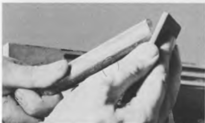
Fig. 18 Honing a gouge with the oilstone. The tool must be firmly supported, and if the handle can be steadied against the body so much the better. Use a circular motion of the stone, rolling the tool at the same time
