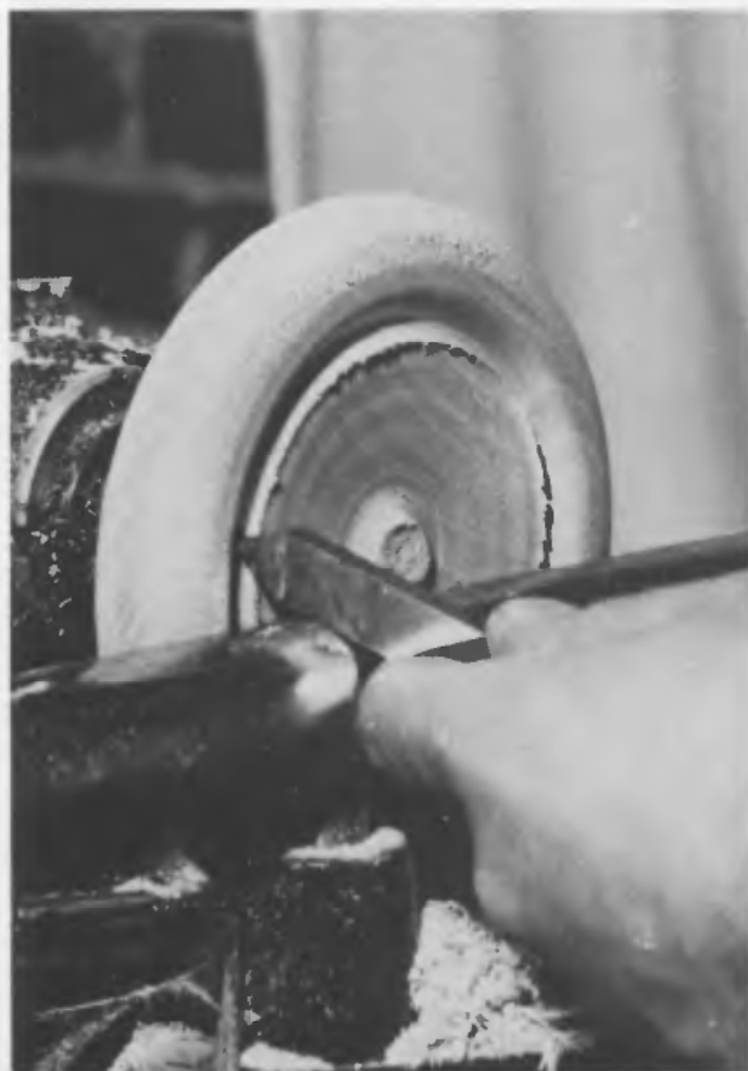
Fig. 28 Forming the ring by cutting in with a parting tool, the work will be reversed into a hollow chuck
