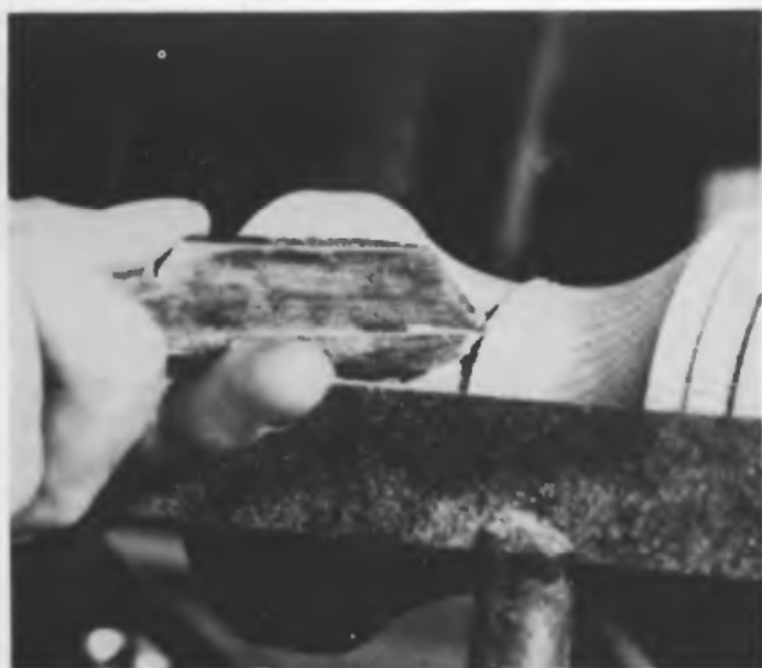
Spindle gouge, ground to a nose, being used in a deep hollow
