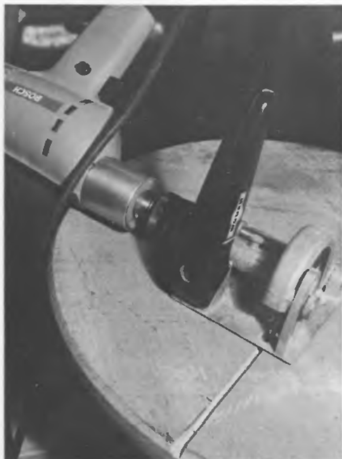
Fig. 4 A groove must be run in the bases of some lamps so that the wire can be glued into it before baize is fitted
