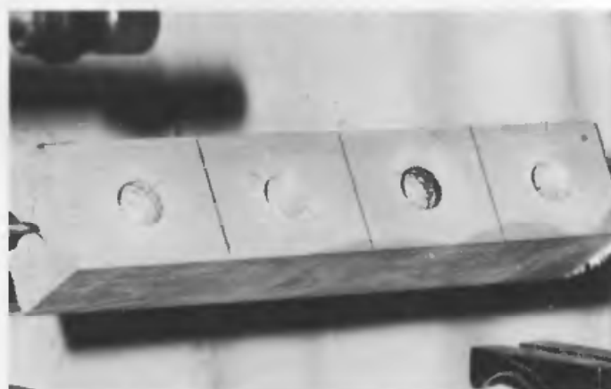
A block has been marked in sections, the centre of each section found, and a 1in. by 1in. (25mm. by 25mm.) hole drilled. Here the block is securely mounted in the lathe ready for turning
