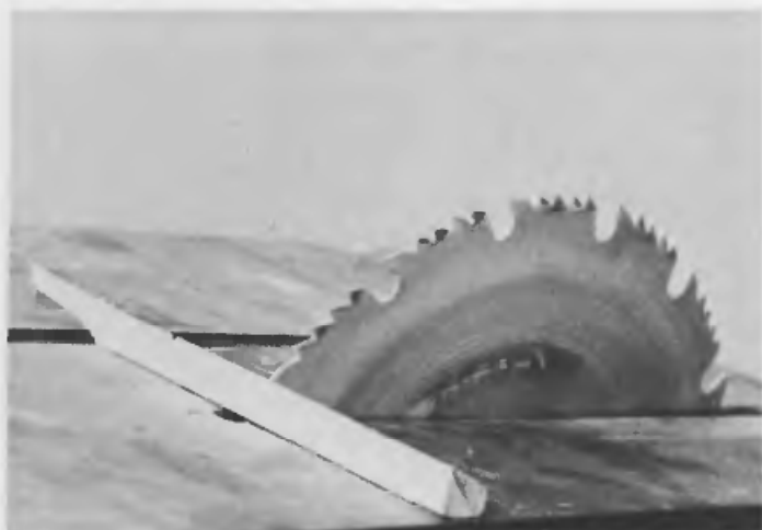
Fig. 24 A simple method of using a circular saw-blade on a universal machine to divide work equally, the tool rest being used as a ruler to mark the wood
