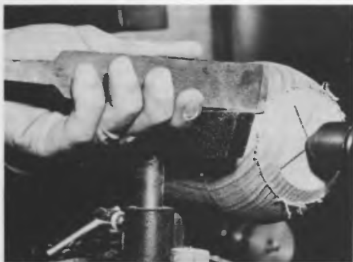
Fig. 18 Rounding over the end of a cylinder with the skew. The bevel must rub all the time, and the handle must therefore be swung as the cut proceeds
