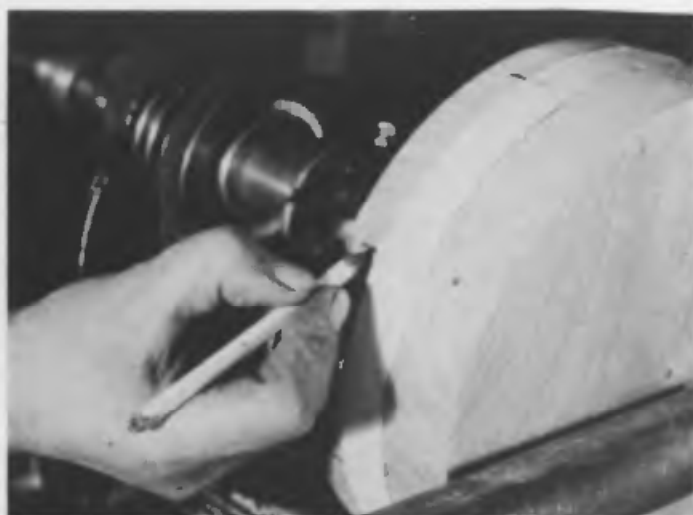
Fig. 11 If a piece of paper which exactly fits round the outside of the blank is folded the required number of times and marked at the folds, it can be used as shown to divide the work prior to drilling for the insertion of plugs
