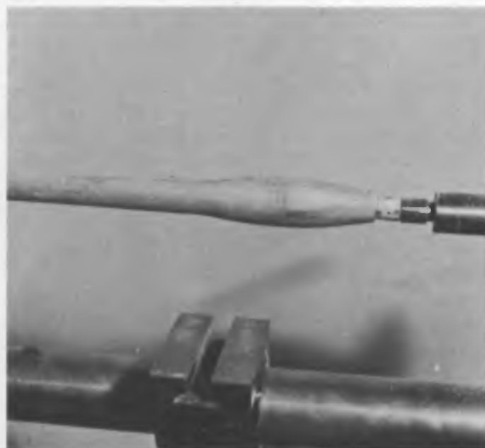
Fig. 7 Shaping the end of a tool handle for the fitting of brass or copper ferrule
