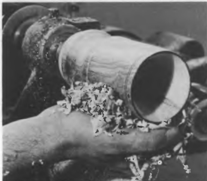
Fig. 7 Blackening the edge of the small vase, by means of pressure from a piece of scrap wood
