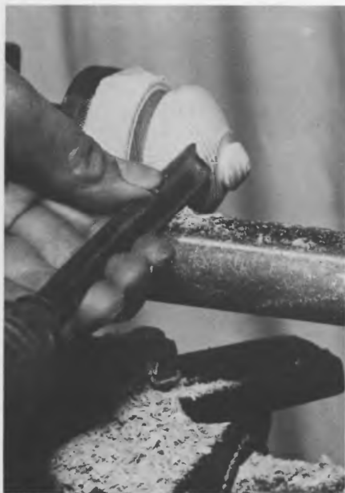
Fig. 26 Lid of mustard pot being turned from a block on woodscrew chuck
