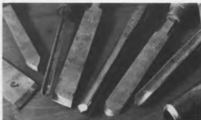
Fig. 1 A useful set of tools for the beginner. Two skew chisels, a parting tool, two gouges for spindle work, a bowl gouge, roughing gouge, and a round-nosed scraper
