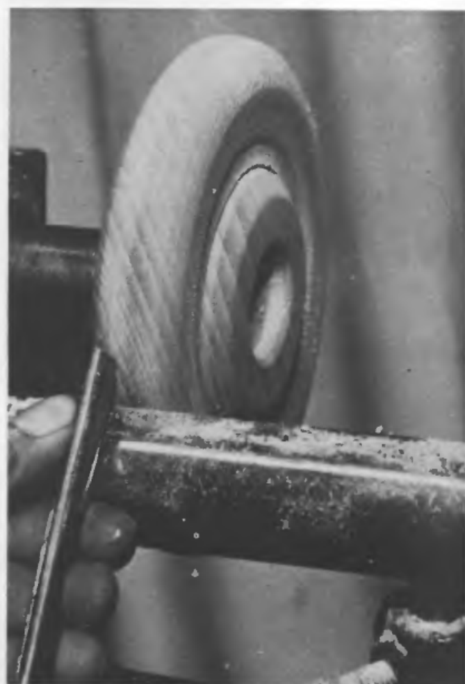
Fig. 27 Shaping the outer edge of a disc which is to be made into a ring
