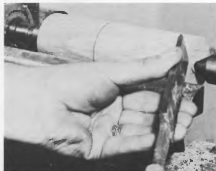
Fig. 16 The base of the article is made slightly concave with the long corner of a skew
