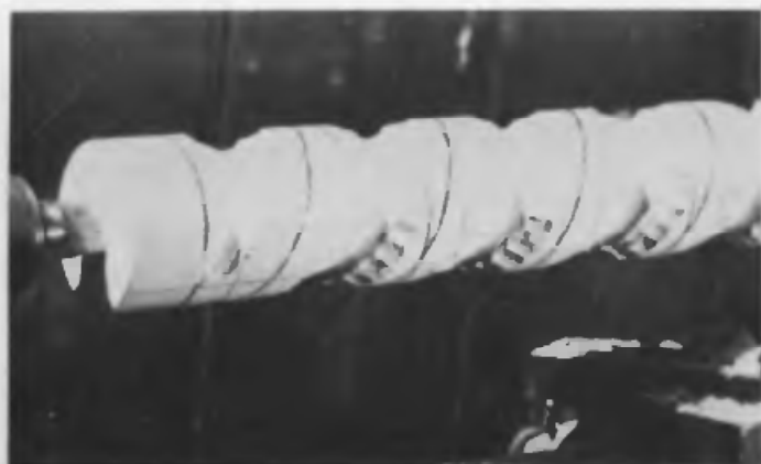
Fig. 6 The roughing out continues, but there is a lot left to do
