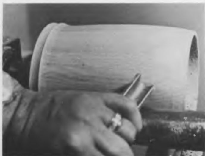
Fig. 13 Shaping the outside of the blank, using a sharp \frac{3}{4} in. [10·1mm.] roughing gouge, with light cuts. A tapered plug could be inserted in the end and tailstock support given if required
