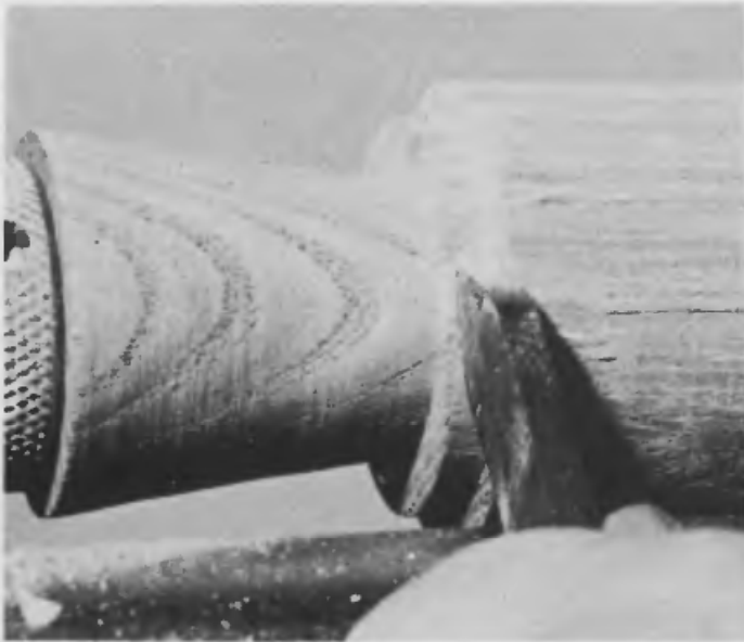
Fig. 20 Cutting the flange on the mill body to take the lid
