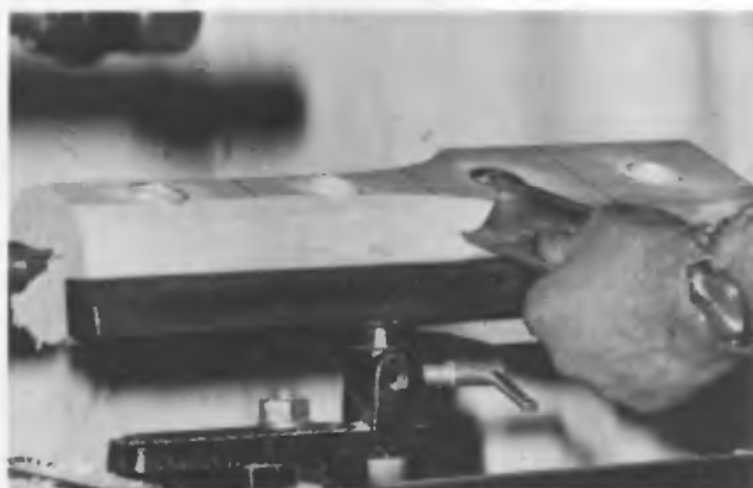
B Big half round roughing gouge in use bringing the work to a cylinder. Note the angle at which the tool is held
