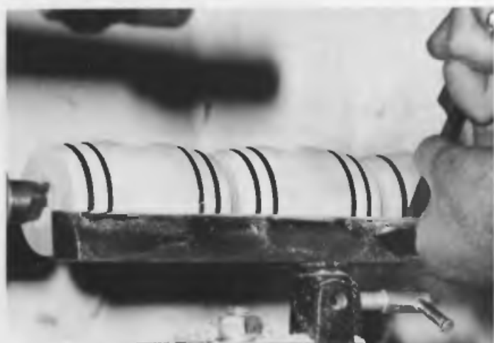
D Burning on the 'hoops'. This is done by forcing the tang of a file or old scraper between work and rest and applying leverage
