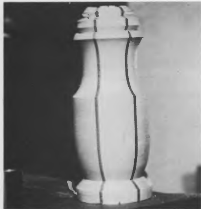
Fig. 14 A coopered blank made with tempered hardboard spacers
