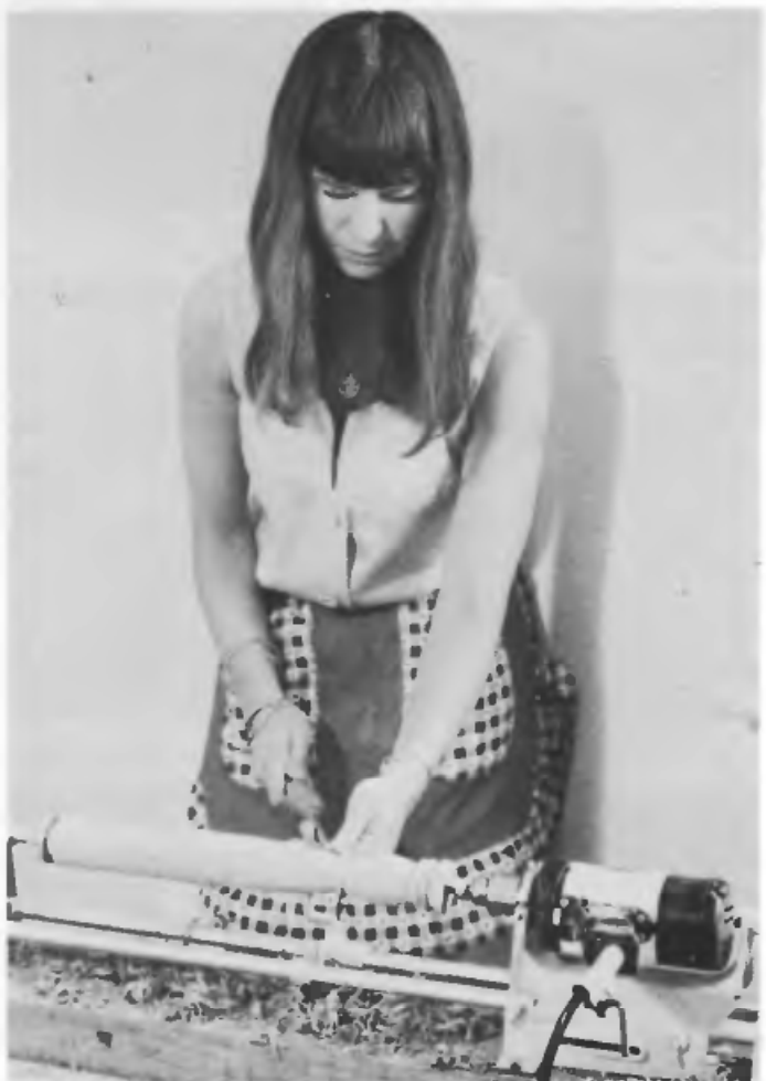
Fig. 17 Lathe attachment and drill in use. These small machines are excellent for anyone wishing to learn the basics of the craft, and also for the turning of small items
