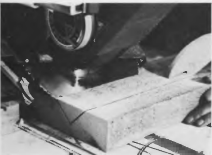
Fig. 8 Cutting a vee block to hold a cylindrical blank for drilling. Tool in use here is the De Walt radial arm saw
