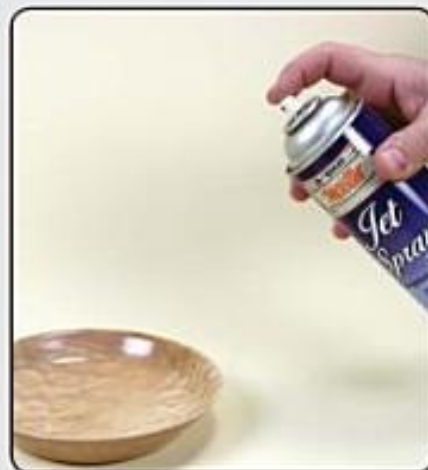
Photo 1.76. Spray approximately 12" away from the piece and use a back and forth motion, applying many light coats.
