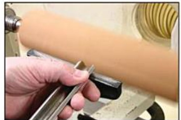
Photo 2.11. With the underhand tool grip, the thumb holds down the gouge.
