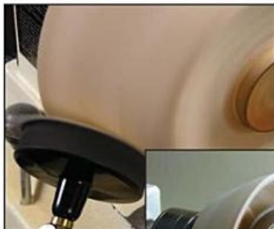
Photo 1.51. An angle sander's articulated head allows it to sand in a variety of angles, making it easy to sand the outside of a bowl.
