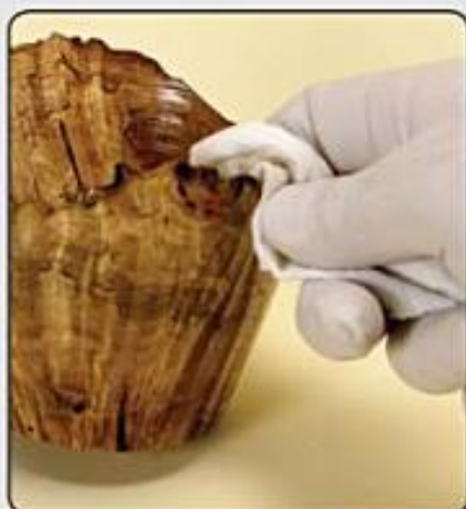
Photo 1.69. Apply salad bowl finish with a lint-free cloth. To protect your hands, wear gloves when you are applying any finish.
