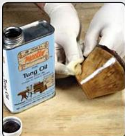
Photo 1.71. Apply diluted tung oil with a rag and allow it to dry for 24 hours.
