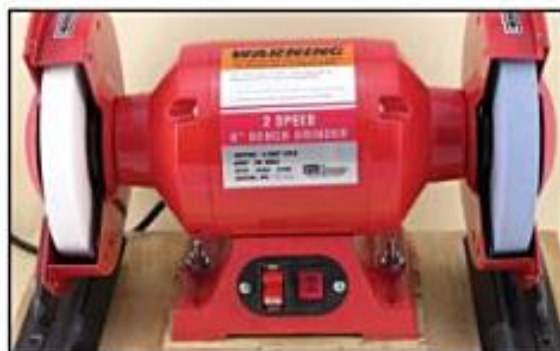
Photo 1.40. Choose a grinder with at least a 1/2 hp motor and 8" wheels. This particular model has two speeds and is attached to a plywood frame.
