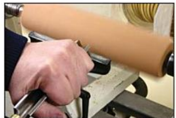
Photo 2.12. With the overhand tool grip, the front hand holds the tool against the tool rest.
