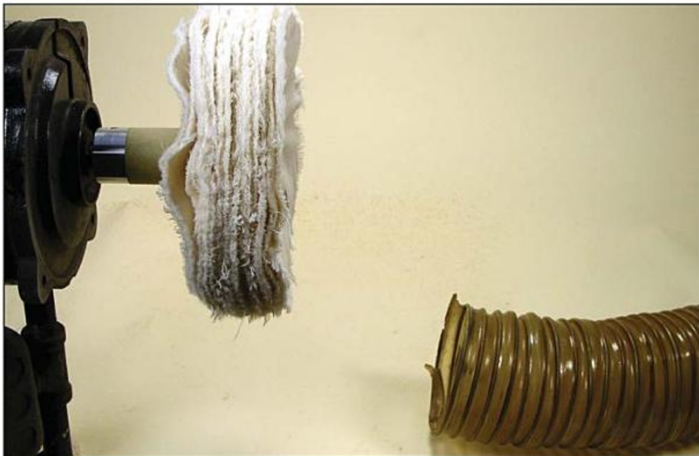
Photo 1.94. Use dust extraction if you will be using a buffing system for extended periods of time.
