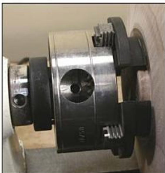
Photo 1.27. A four-jawed chuck secures a bowl with a spigot for faceplate turning.
