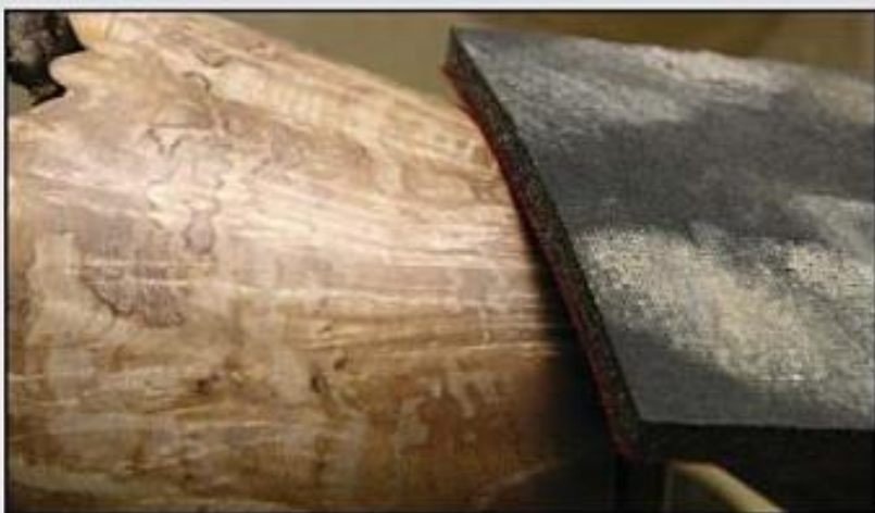
Photo 1.67. Whether you are preparing for finishing or repairing a bad finish, the first step is to sand through 800 grit. Here I am using an Abralon sanding pad to prepare the surface for the finish.
