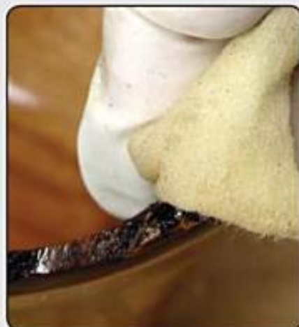
Photo 1.73. Apply extra tung oil to the bark to ensure that the bark stays on the bowl edge.
