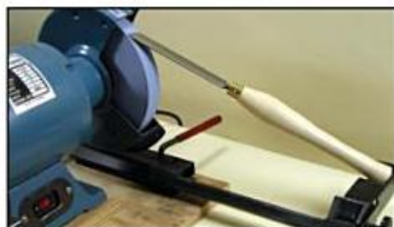
Photo 1.31. A grinding system grinds consistent bevels on your tools.
