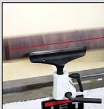
Photo 1.14. Tool rest height should be set so that the tool will be at the center of the workpiece, and the tool rest should be approximately \frac{1}{8} " away from the spinning work.
