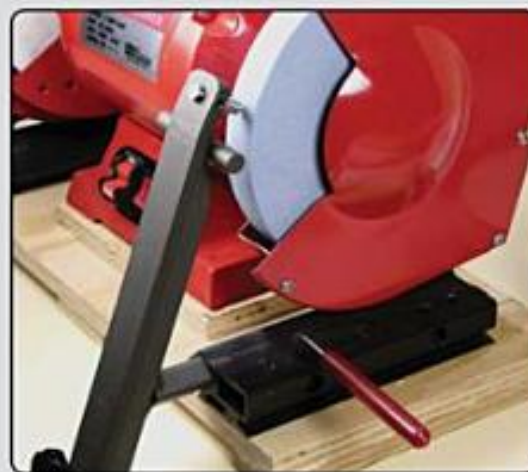
Photo 1.43. This dresser uses a single-point diamond held in an adjustable arm.
