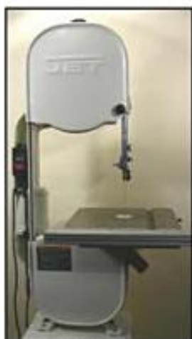
Photo 1.29. A band saw is a great tool for cutting larger pieces of wood into suitable pieces of turning stock.
