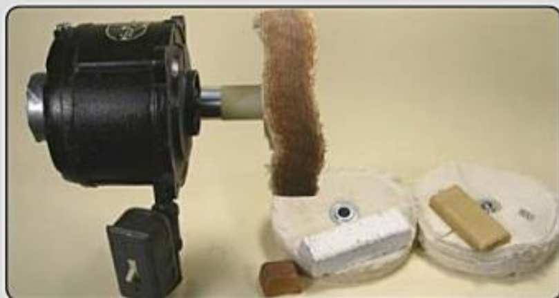
Photo 1.83. A buffing system, such as the Beall Buffing System, can be a fast, easy way to apply a beautiful finish.
