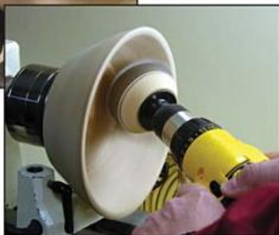
Photo 1.52. Sanding pads chucked into a hand drill can also work well for power sanding.
