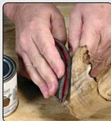
Photo 1.70. Lightly sand between coats of salad bowl finish with a 4000-grit sanding pad, such as the Abralon one I'm using here.
