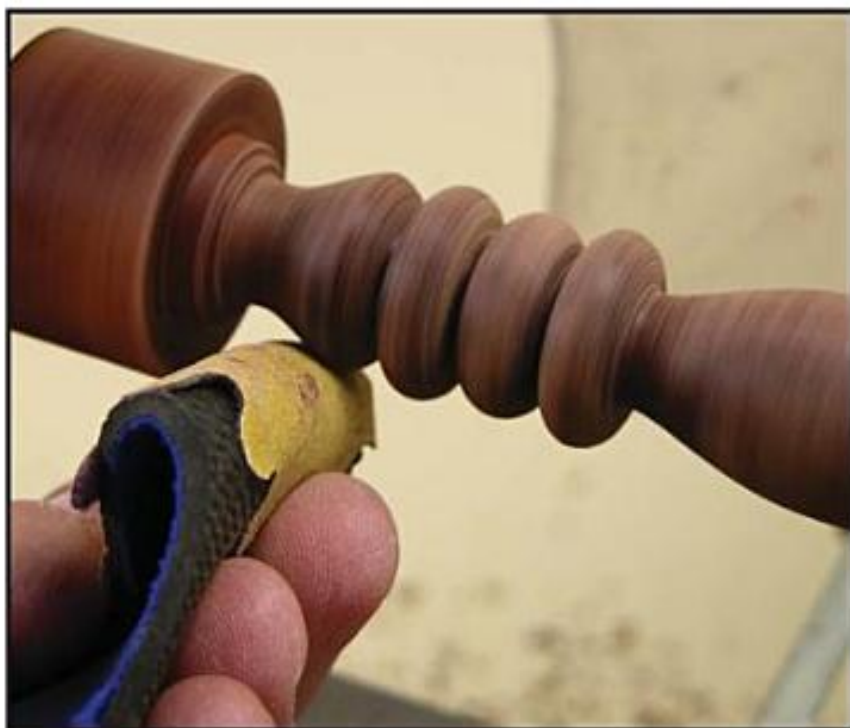
Photo 1.56. To assist your sanding efforts, use a pad that will conform to the coves. Any piece of soft material, such as part of a rubber mat, can be used as a sanding pad.
