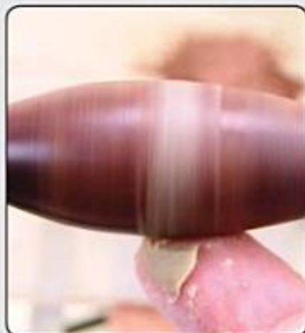
Photo 1.78. Apply a small amount of EEE polish with your finger while the lathe is running at a medium speed (approximately 700 rpm).
