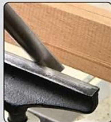
Photo 2.14. If the tool rest is not close to the workpiece, a catch can tear the tool from your hand.
