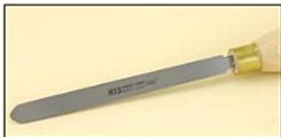
Photo 1.23. For those individuals who are “skew challenged,” a Spindlemaster is a useful tool combining a spindle gouge and a skew without the fear of the dreaded catches associated with a regular skew.
