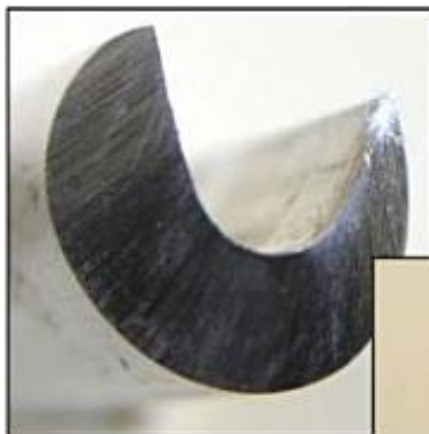
Photo 1.48. A properly sharpened tool shows no shiny surface on the edge of the tool.
