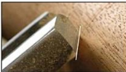
Photo 2.8. Make sure that only the lower portion of the bevel of the gouge is touching the surface.
