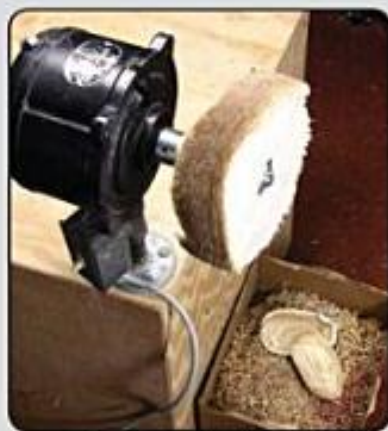
Photo 1.85. Here an old oil burner motor is used to drive the buffing system.
