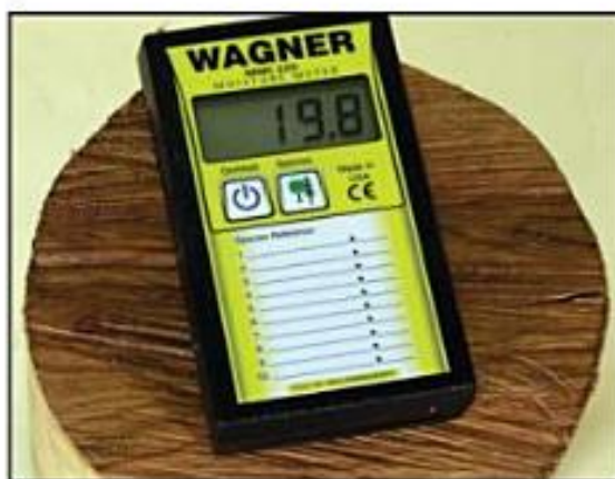
Photo 1.39. The moisture meter shows a higher moisture content from only the top portion of a different maple burl.
