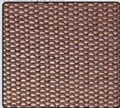
Photo 1.59. This sanding material, called Abranet, does not load up as frequently as normal sandpaper.
