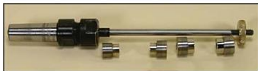
Photo 1.28. Mandrels allow you to turn hollow objects, such as pens.
