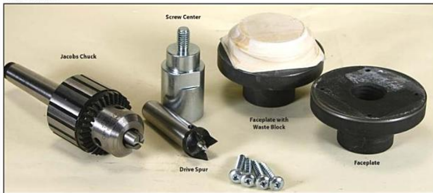
Photo 1.25. Pictured here is a variety of mounting devices. The Jacobs Chuck holds a drill in the headstock or the tailstock. The others pictured mount the workpiece on the lathe.
