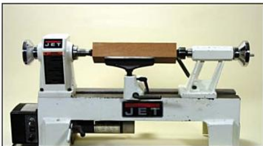
Photo 2.1. With spindle turning, the grain is running parallel to axis of the lathe.
