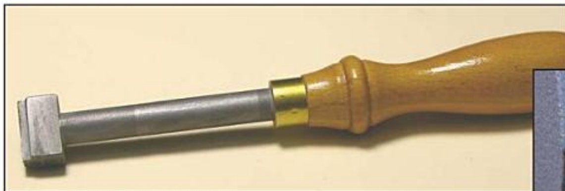
Photo 1.45. This dresser features a large surface that comes in contact with the wheel.
