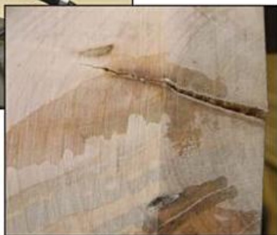
Photo 1.54. Excessive heat from sanding can cause cracks.
