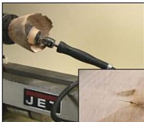
Photo 1.53. A flexible shaft with sanding material attached can provide "deeper" reach inside a bowl and a more comfortable grip.
