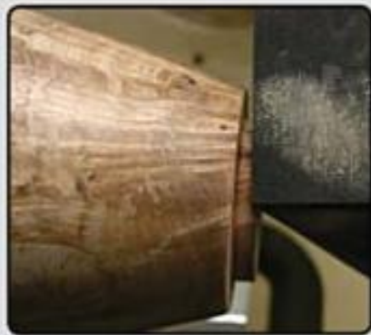
Photo 1.63. A sanding pad, such as this Abralon one, works to remove microscratches after the workpiece has been sanded up to 600 to 800 grit.
