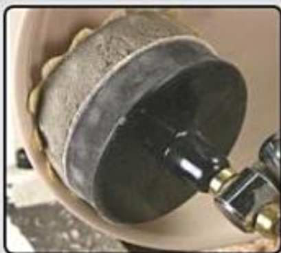
Photo 1.58. Notice how the wavy edges conform to the shape of the bowl, leaving a smoother finish.
