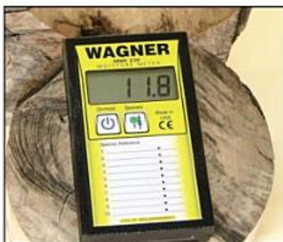
Photo 1.38. The moisture meter shows a low moisture content from only the top portion of the maple burl. Each manufacturer will supply a reference chart listing each individual wood and its relative moisture content.
