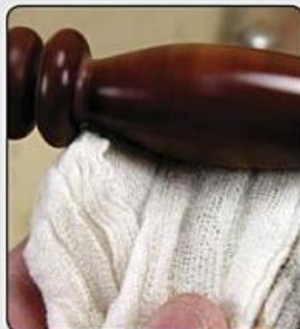
Photo 1.79. Use cheese cloth to remove the excess EEE polish while allowing the heat to seal the polish into the wood.
