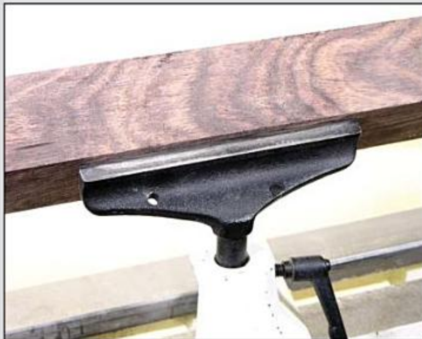
Photo 1.13. Notice that the wood is hitting the tool rest. Do not allow this to happen! Your workpiece will be mangled and the spindle could be set loose in your workshop.
