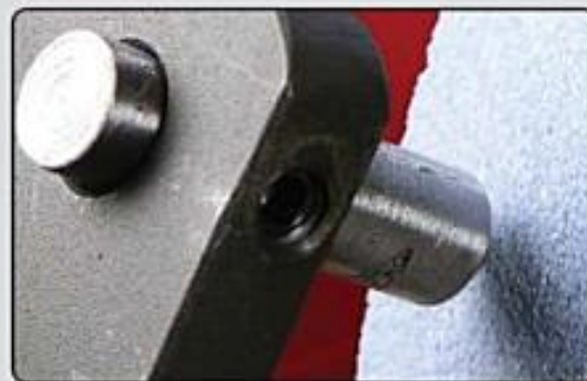
Photo 1.44. In this close-up, you can see that the diamond dressing tip is removing small amounts of the grinding wheel.
