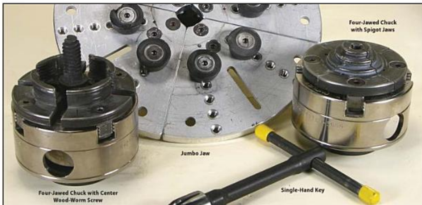
Photo 1.26. Assorted chucks and jaws used to hold faceplate work. The single-hand key operates all three chucks.
