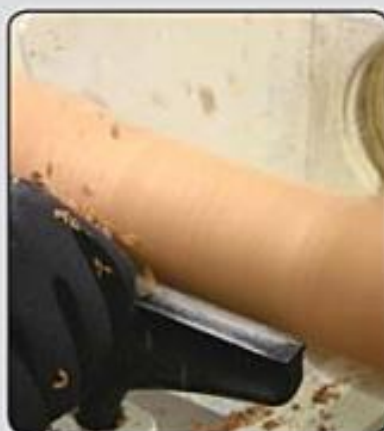
Photo 2.16. The gouge lightly removes the sharp edges of the blank.
