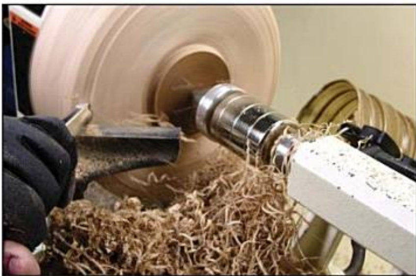
Photo 2.2. In faceplate turning, the grain runs perpendicular to the lathe bed.
