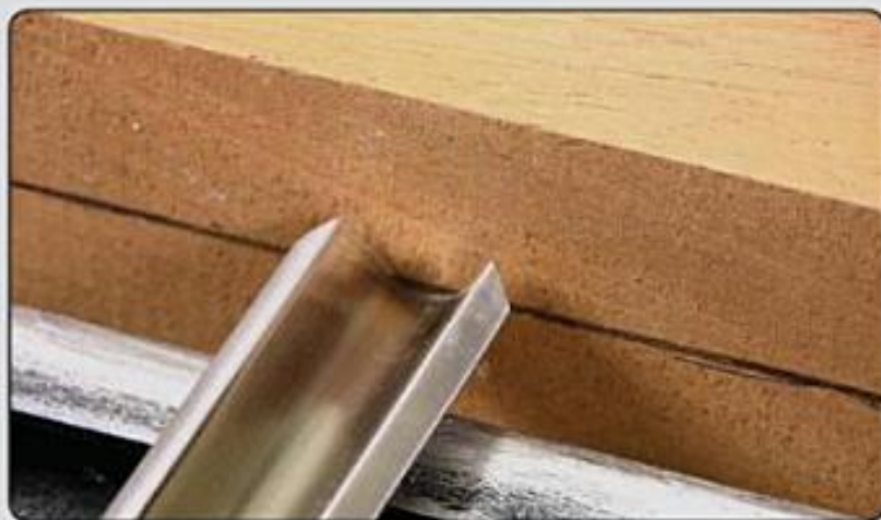
Photo 2.15. The tool rest height should be approximately in the center of the spindle.
