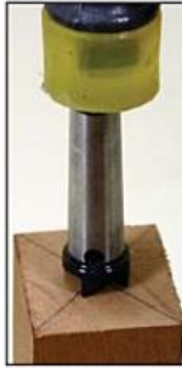
Photo 2.3. Find the center of the spindle by drawing a line from one corner to the other corner.
