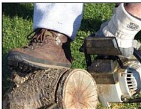
Photo 1.17. Wear protective boots and gloves whenever you are using a chainsaw to prepare wood for turning.
