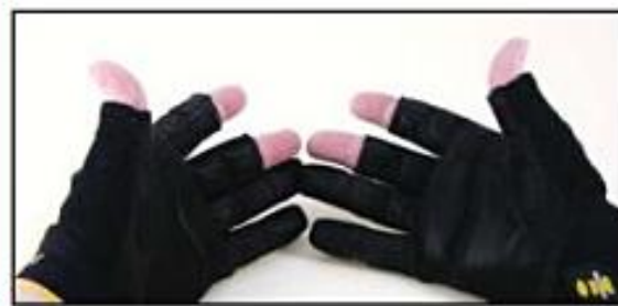
Photo 1.19. Use turning gloves with padded grips to reduce vibration and to protect your hands from overheated, flying chips.
