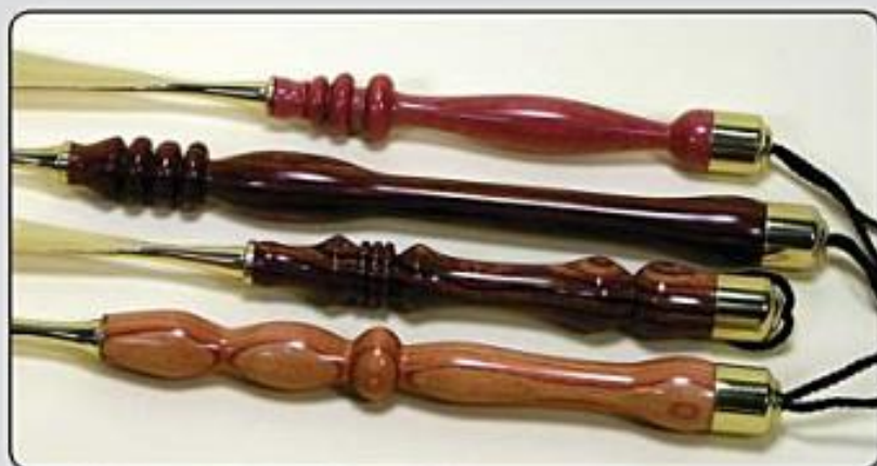
Photo 1.84. This spindle work was finished with either the woodturner's finish and EEE polish or the buffing system—can you tell the difference?
