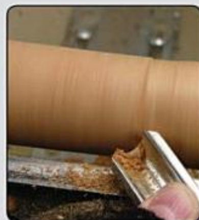
Photo 2.17. Ride the bevel of the roughing gouge to smooth the cutting action of the tool.
