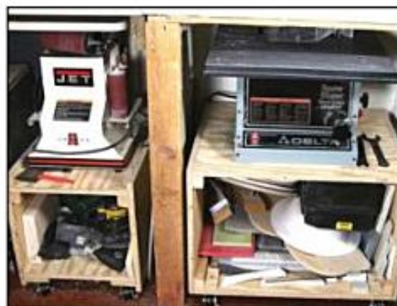
Photo 1.20. At the left is an oscillating spindle sander and at the right a router/shaper. To save valuable space in the shop, mount tools on rolling stands so that they can be rolled out and used when needed and placed back under the workbench when they're not in use.
