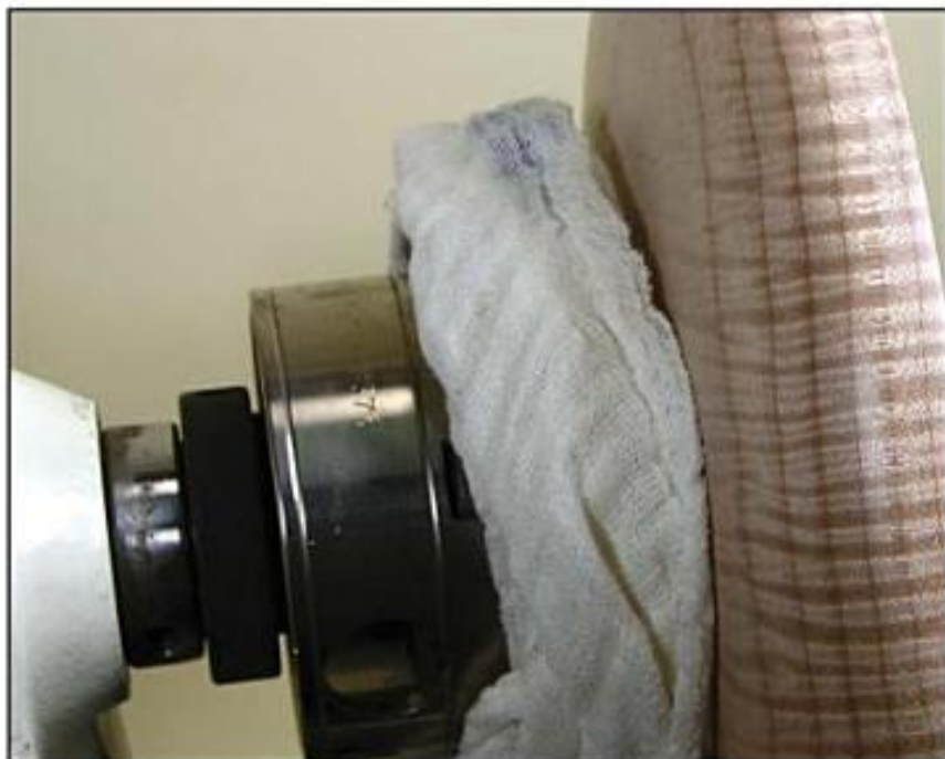
Photo 1.16. A finishing rag that "got away" from me and wrapped around the workpiece.
