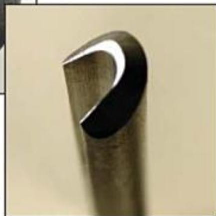
Photo 1.49. A shiny edge like this one is a tell-tale sign that this tool needs to be sharpened.
