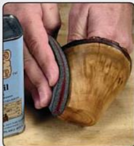
Photo 1.72. Lightly sand between coats of tung oil with a 4000-grit sanding pad, like the Abralon one I'm using here.
