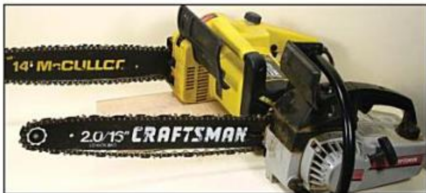
Photo 1.30. Chainsaws, either electric (top) or gas (bottom), can reduce logs to smaller, more manageable pieces of wood.
