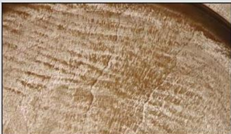
Photo 1.66. Now, look at the same bowl with a single coat of salad bowl finish rubbed on it. Notice all of the scratches and end-grain tear-out. If the bowl were left as is, this would be a horrible finish.
