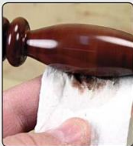
Photo 1.81. Apply a small amount of woodturner's finish with a paper towel and allow friction to seal the lacquer finish to the workpiece.
