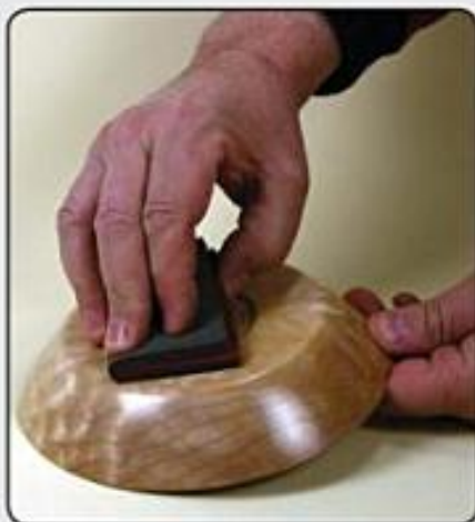
Photo 1.75. In between coats of sanding sealer and final finish, use a 4000-grit sanding pad, like this Abralon one, to remove any "wood fuzz" that might pop up.
