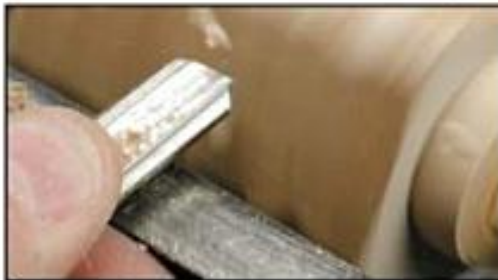
Photo 2.7. Make sure the tool is resting securely on the tool rest.
