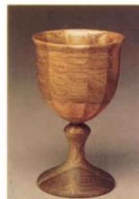
Oak and cherry goblet finished with Danish oil which dries to a hard finish. Popular easy finish. Apply more coats for a harder finish
