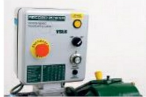
Photo 21. Modern electronic control offers infinite variation of speed
