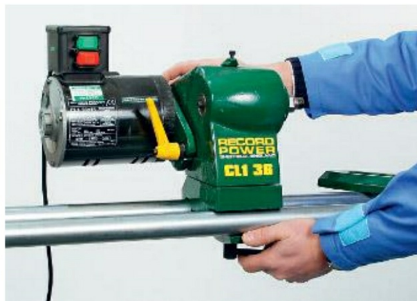
Photo 15. A headstock you can move along the bed is a big advantage
