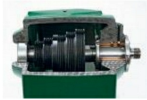
Photo 11. Tapered bronze-sleeved bearings give greater support than ball races
