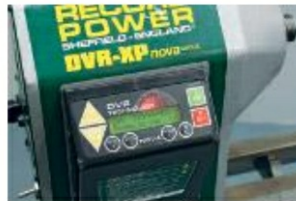
Photo 22. Memory functions can remember your favourite speed settings
