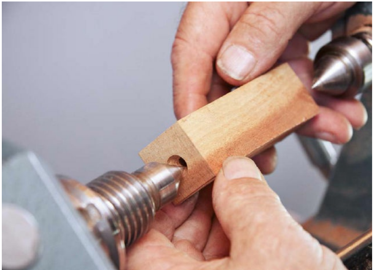
The predrilled blank is mounted between conical centers.
