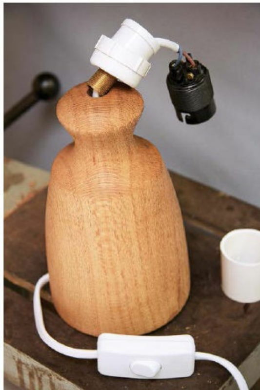
Fitting the lampholder. First widen the center hole for the connector. Then pass the power cord through the bottom and center holes and connector before connecting the wires to the bulb
