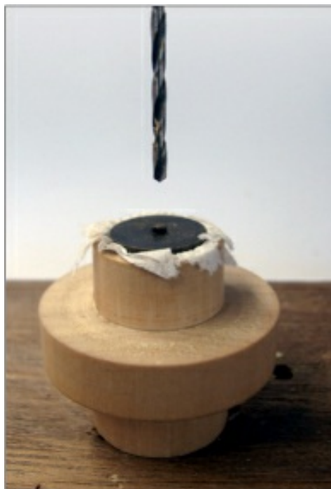
Insert inside the first jig waiting to be drilled. The kitchen paper (paper towel) removes the slack between
