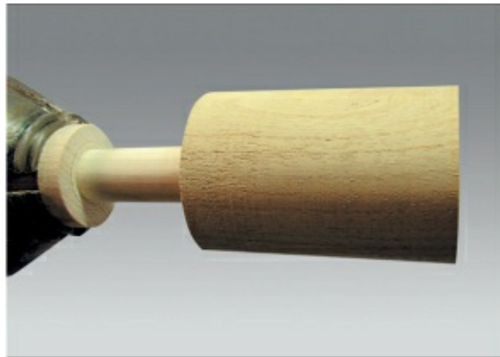
A being placed on the drive plug which will support the shaker while B is glued in place and its outside turned.
