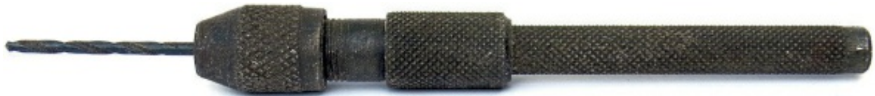
Fig A8-9 Pin chuck holding a 1/16 in (2 mm) twist drill.
