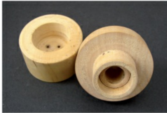
The two jigs for drilling the exit holes in the insert at the top of the shaker shown in Fig A8-8 on Page 22 .
