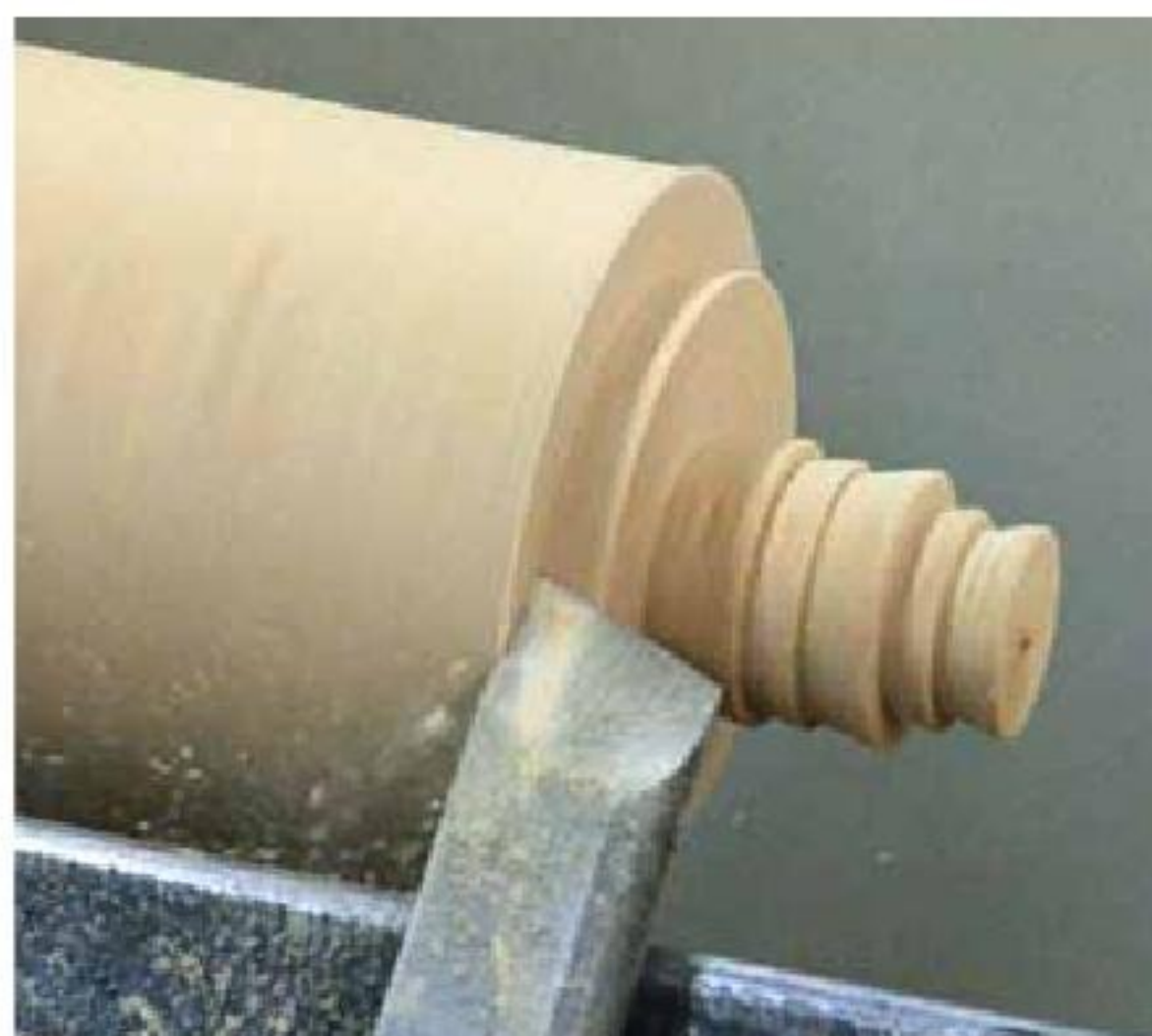
17. Use the skew chisel to peel cut the finger top.
