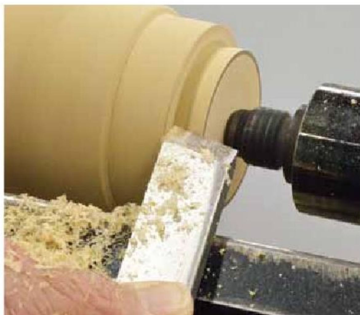
6. Cutting a dovetail tenon can be easily done with a skew chisel and a peeling cut.
