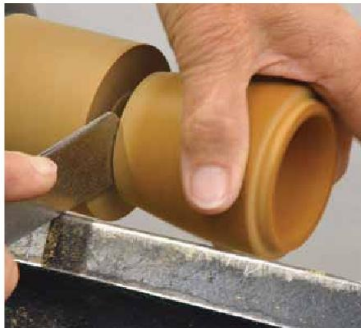
13. Part the base from the remaining jam chuck material.
