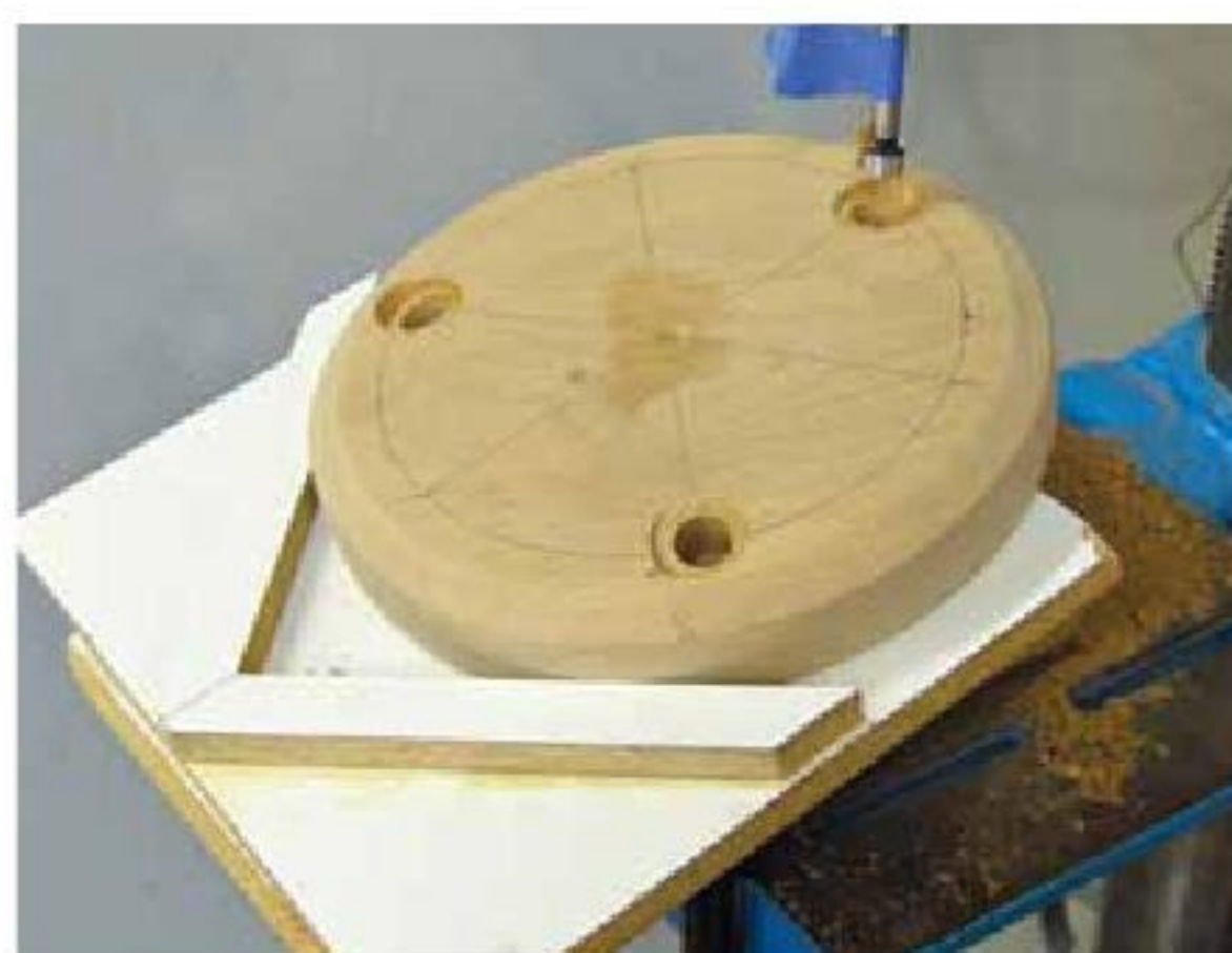
9. Drilling the smaller leg hole centered on the larger shoulder, using the alignment line to be sure of squareness.
