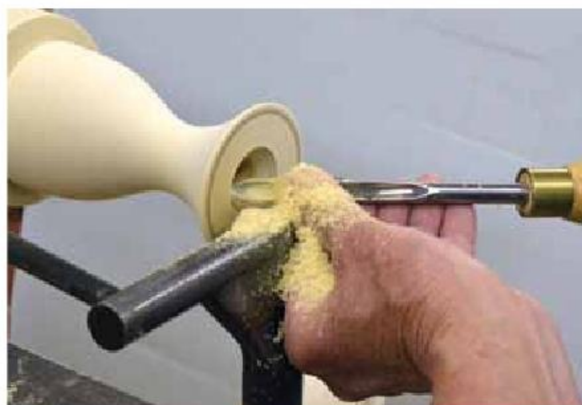
37. Flair out the neck with a shallow fluted gouge from the center outward.
