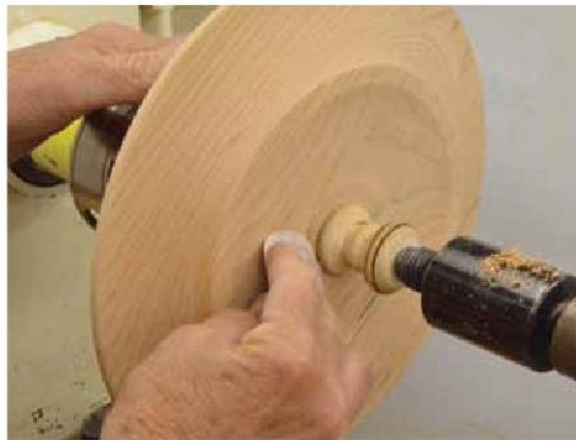
15. Remove additional wood from between the foot and the center and sand.
