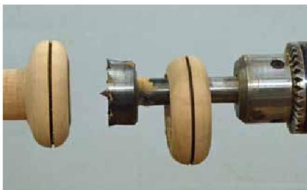
29. After the first ring is cut off, stop the lathe and retrieve it.
