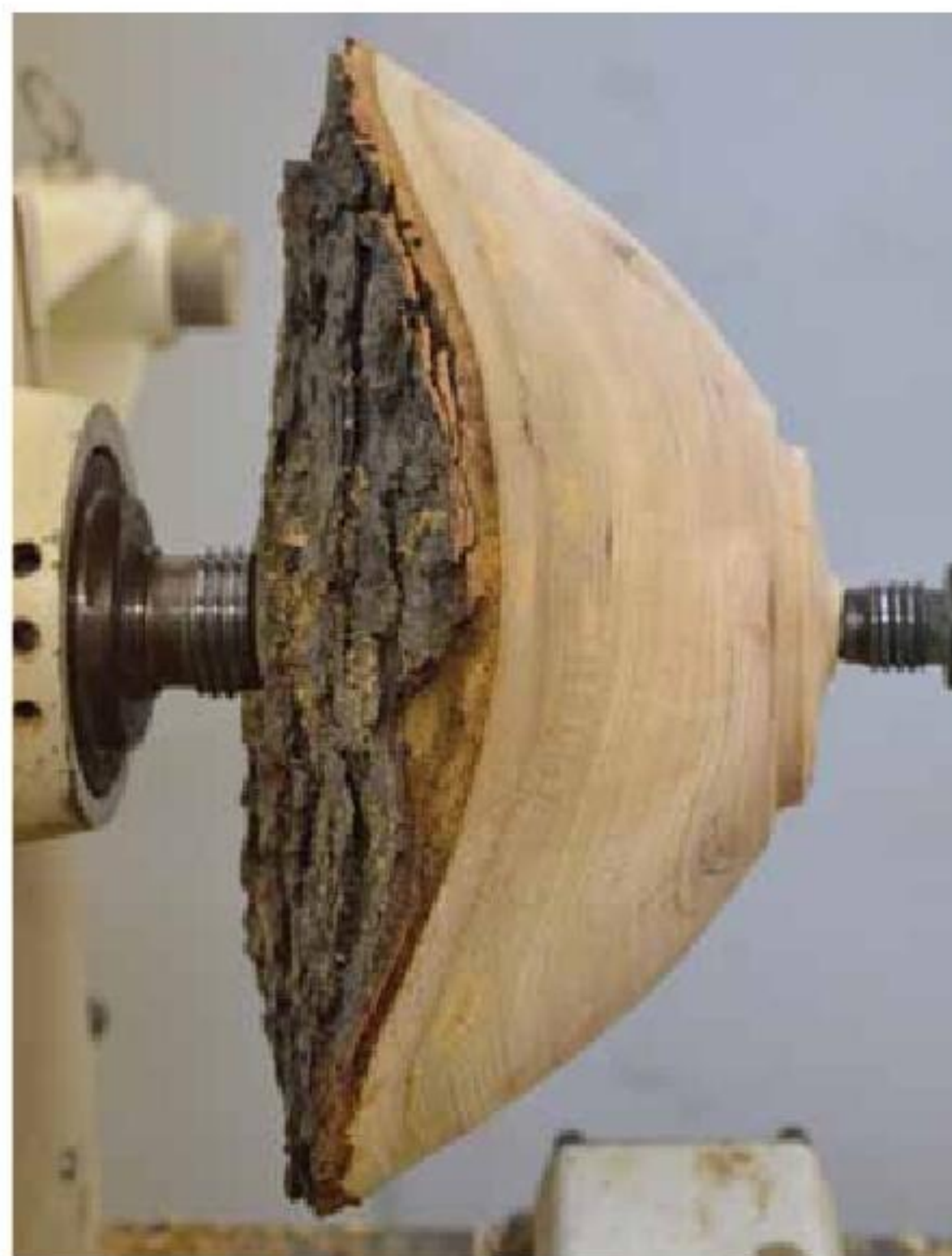
5. Completing the exterior reveals the balanced upper and lower wings.
