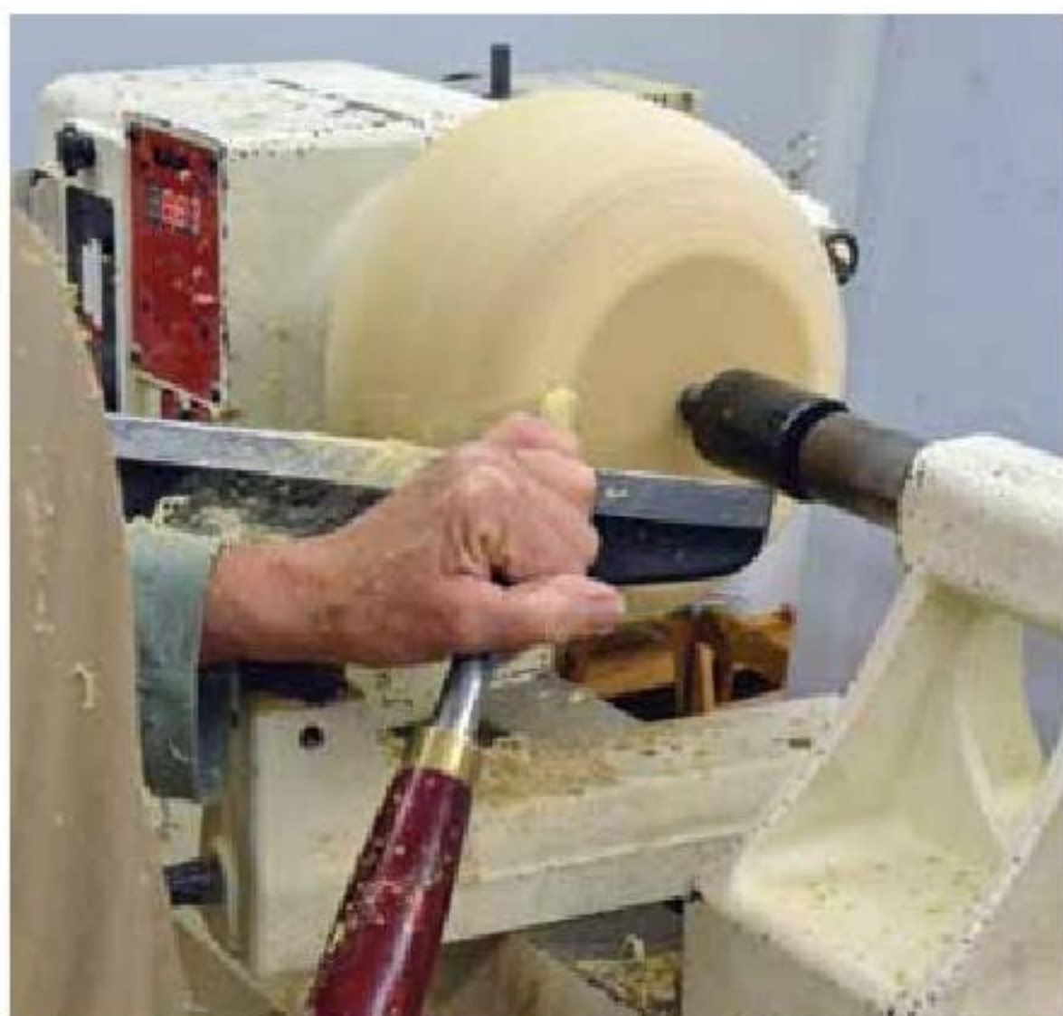
4. Begin to shape the exterior with the tailstock added for support.
