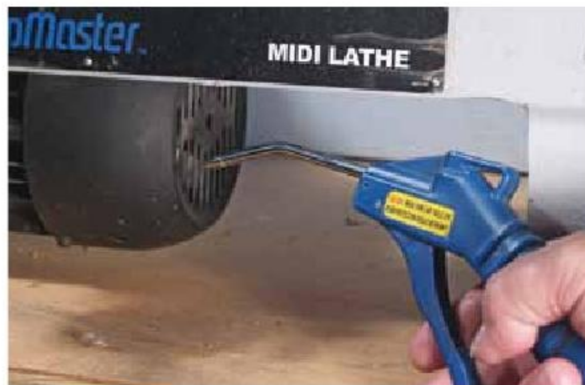
7. Cleaning out the motor's cooling vent will allow it to last much longer.
