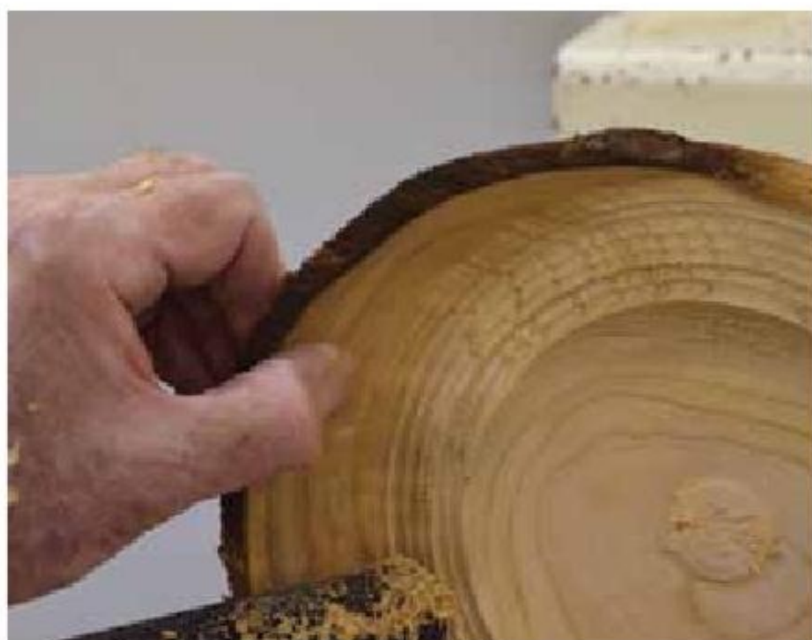
7. Complete the first inch to final wall thickness.
