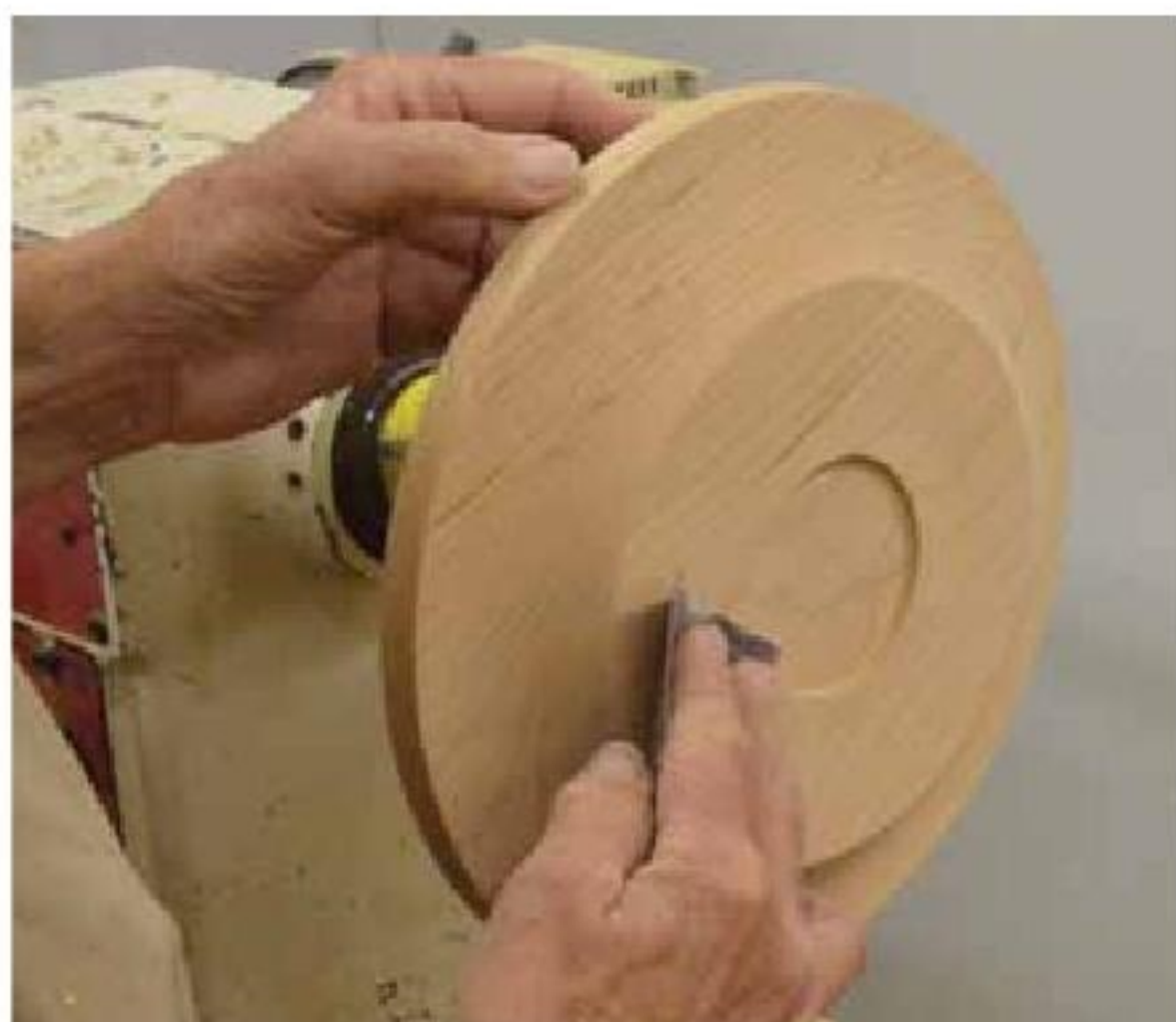
7. The back side of the rim is shaped and sanded first.
