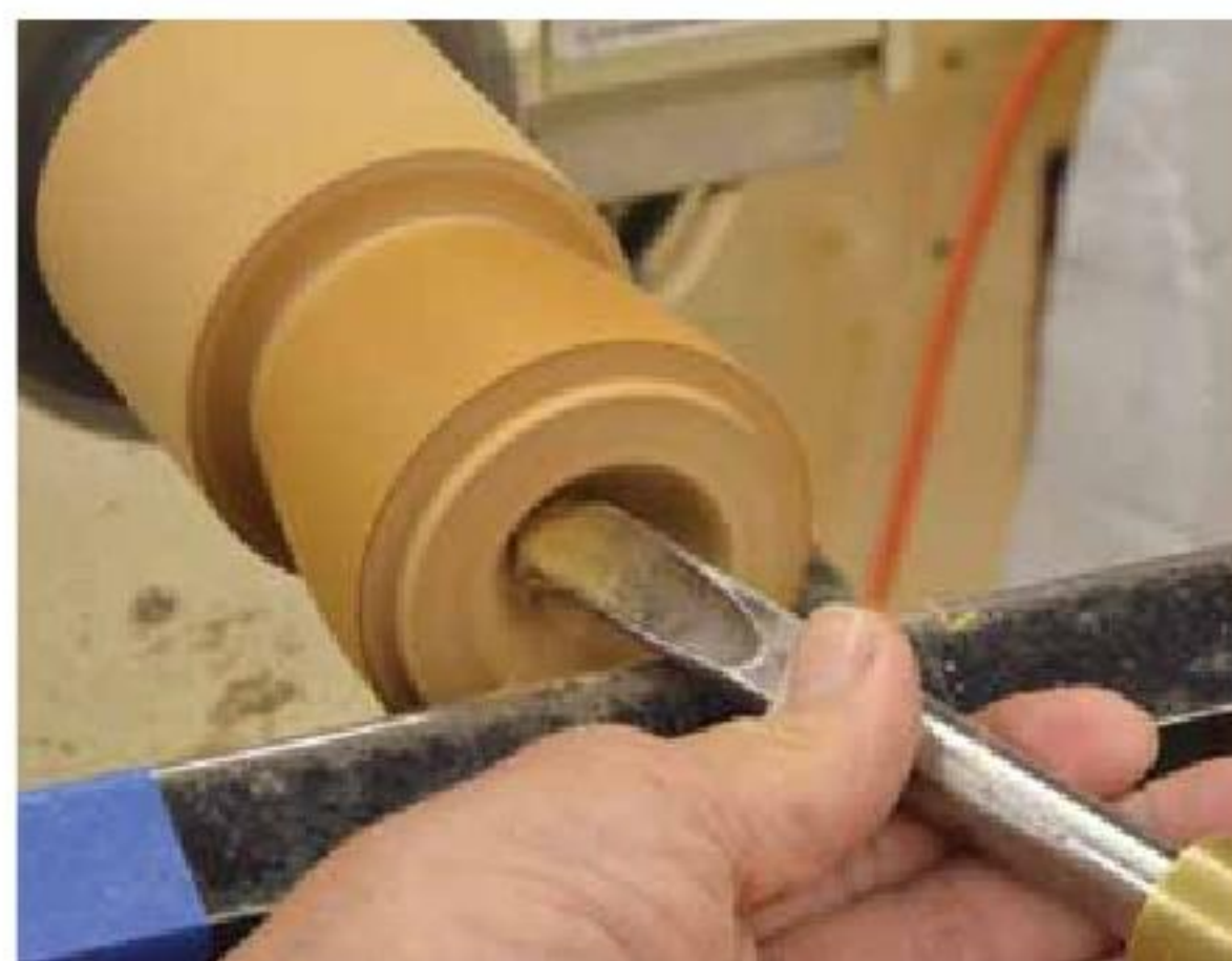
11. Hollow the box with a gouge or a round nosed scraper.
