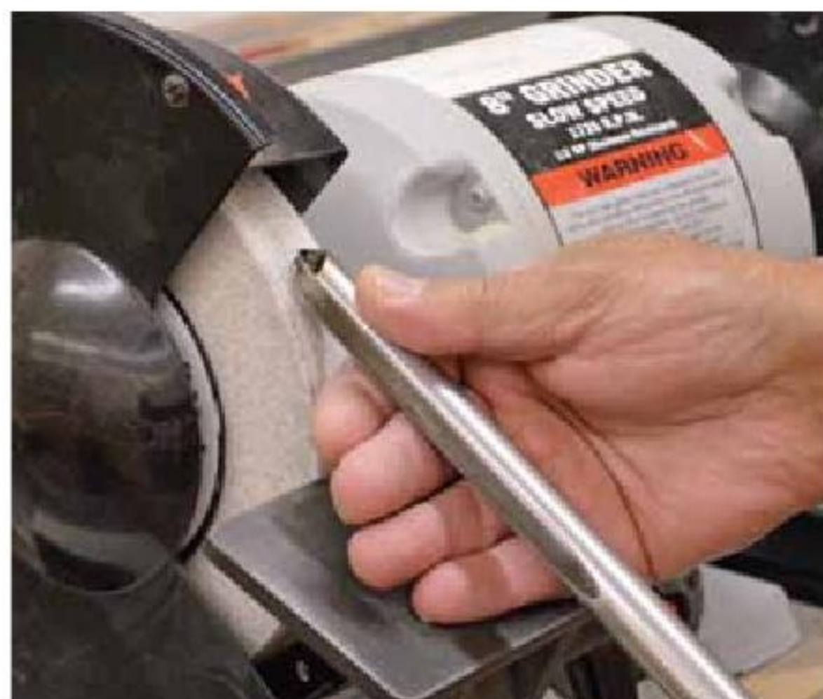
17. Free hand sharpening can also be done by pushing the tool upward while rotating.
