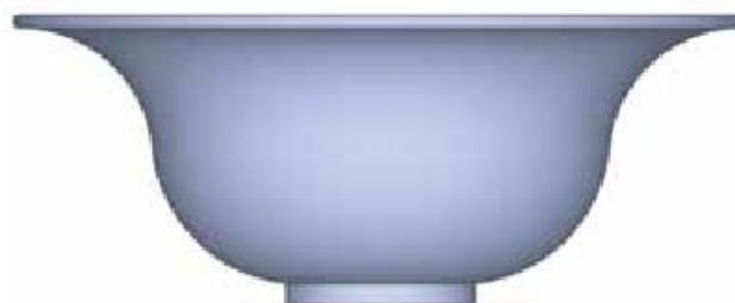
13. An ogee shaped bowl has one curve reversal near the top or foot.
