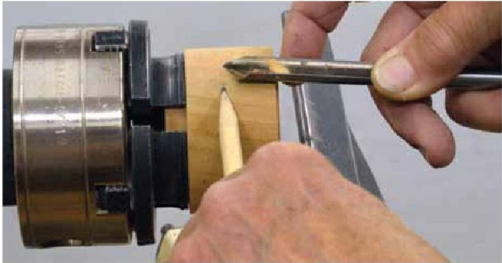
5. Drill out the depth of the lid and mark its depth.
