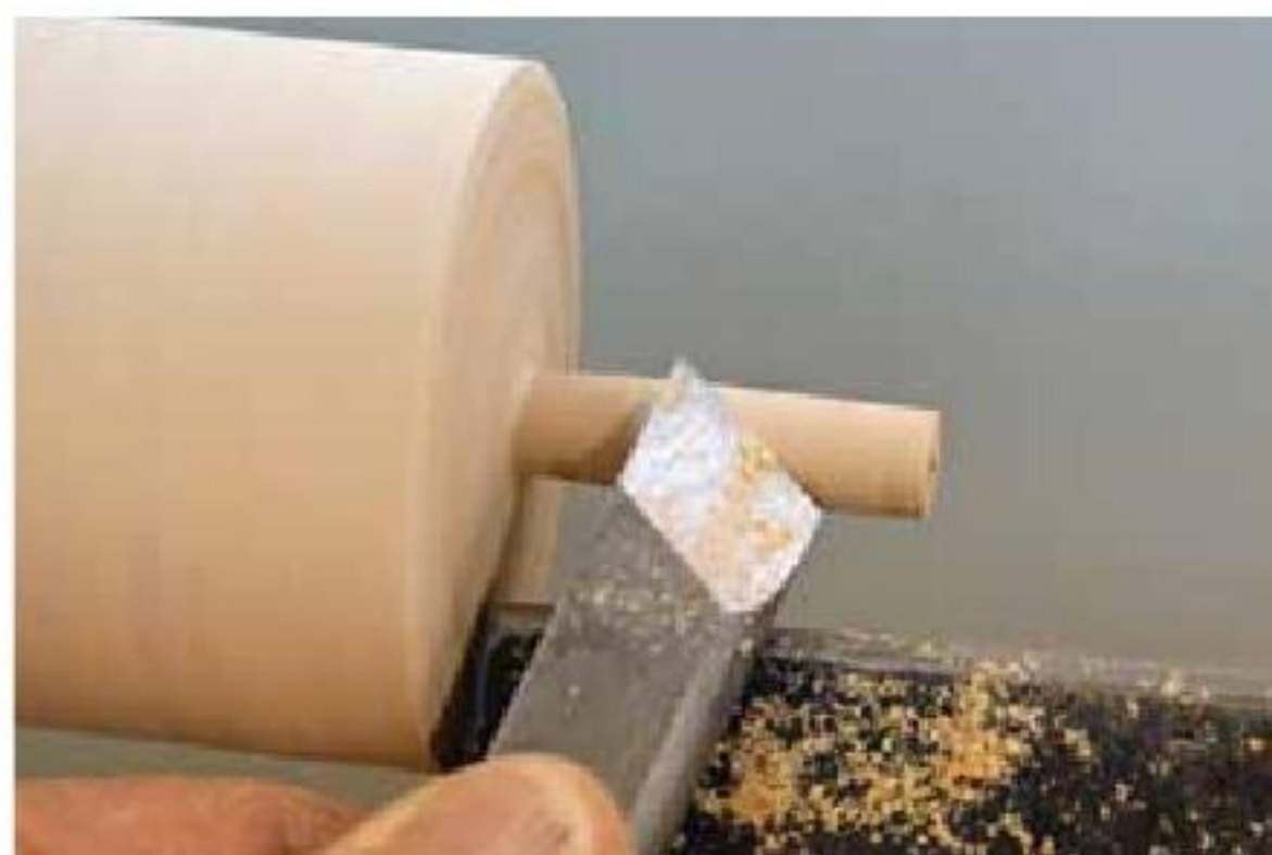
18. Use a planing cut to smooth the finger top.
