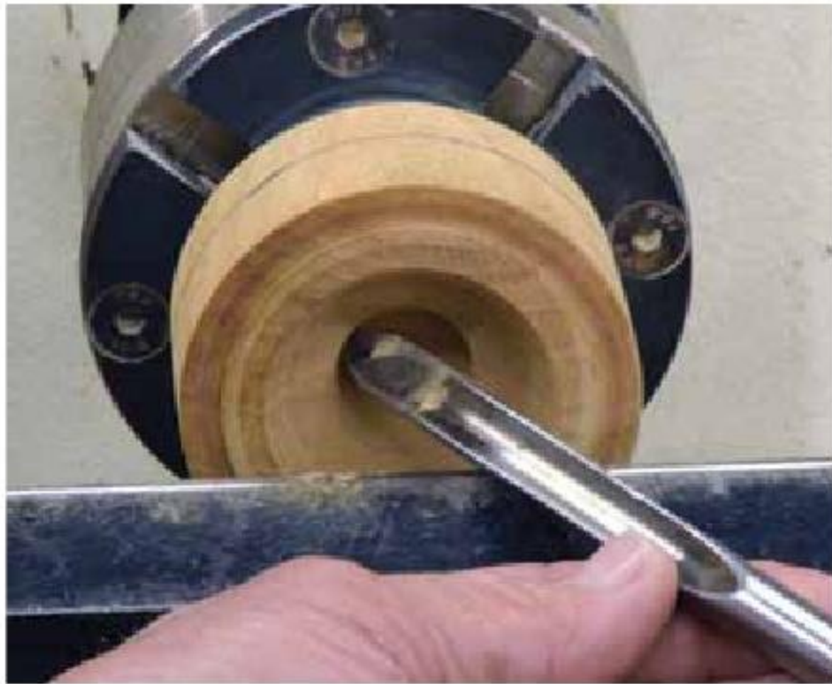
6. Hollow out the lid with a gouge.
