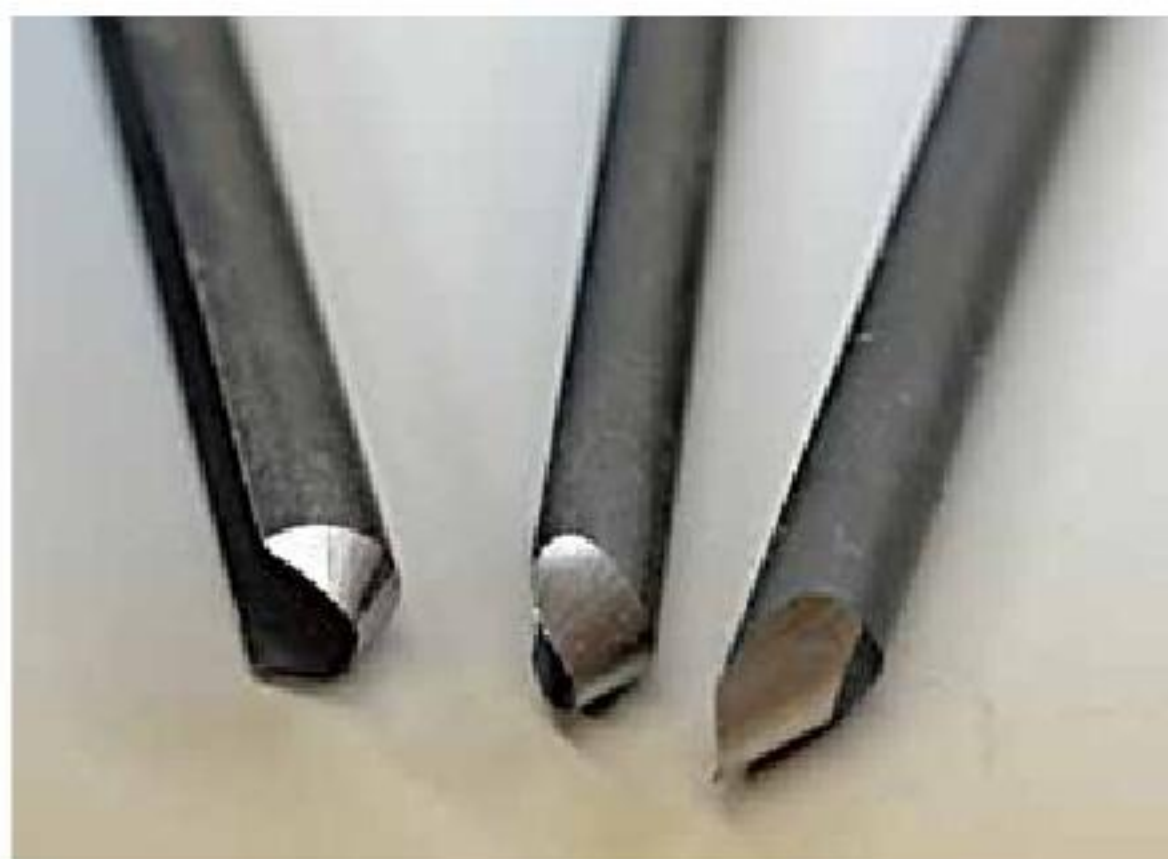
10. Three shallow-fluted spindle gouges are the traditional, swept back, and detail grinds.
