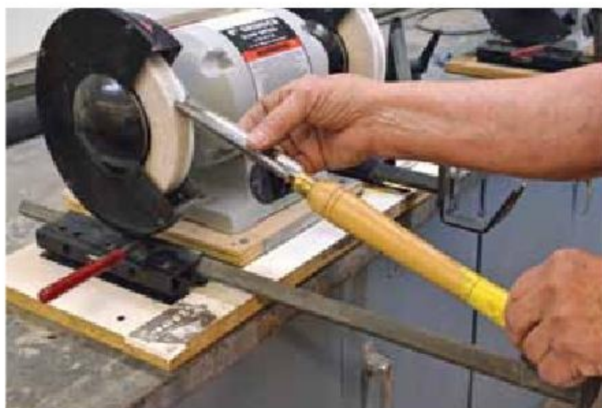
5. To sharpen the SRG in a long arm fixture, use very light downward pressure.
