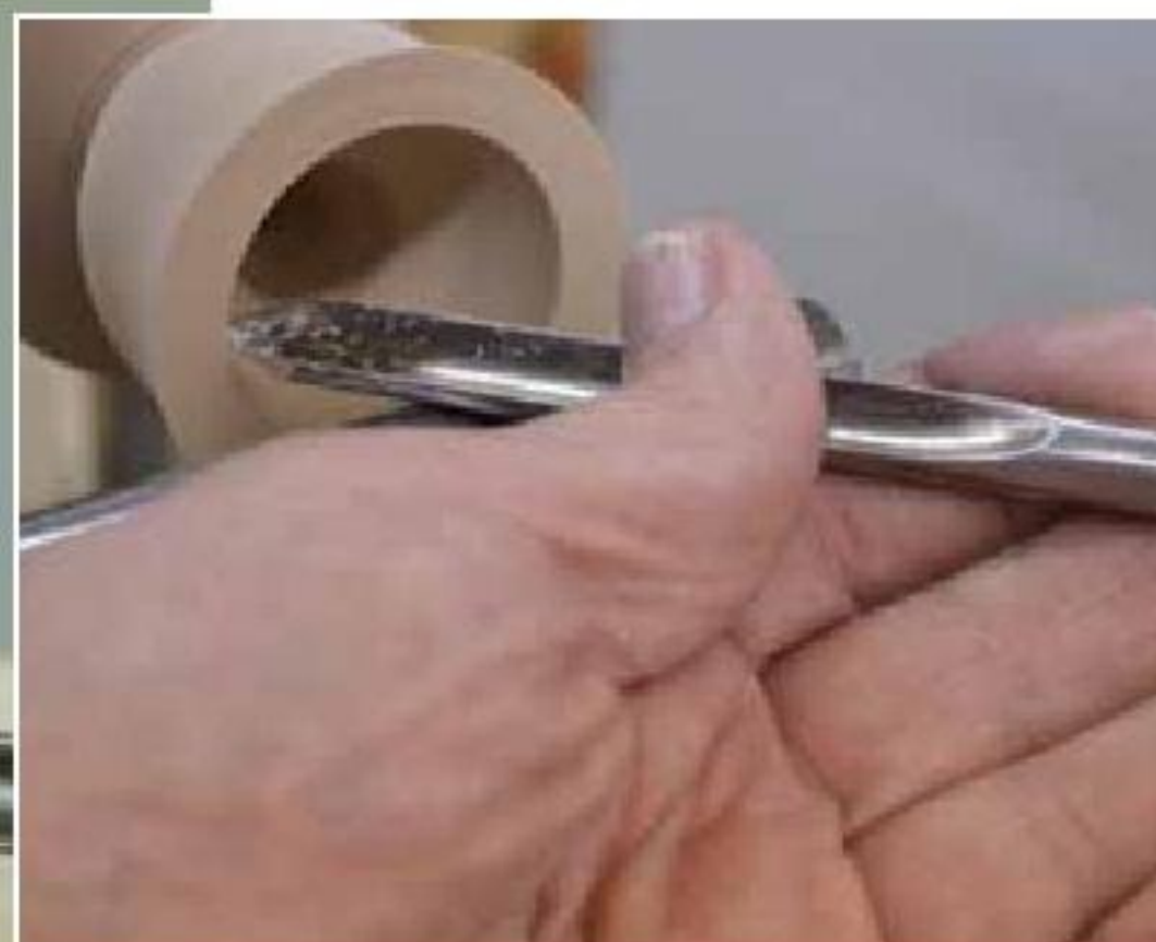
6. Position the gouge at 45 degrees to hollow out the cup. Hollow by pushing the handle backward and pivoting around the left thumb.
