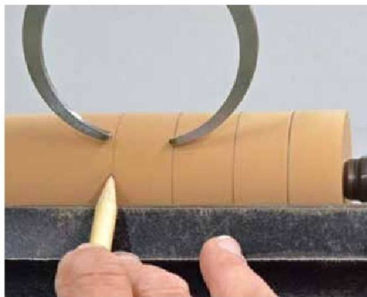
24. Lay out the dimensions with calipers and a pencil.
