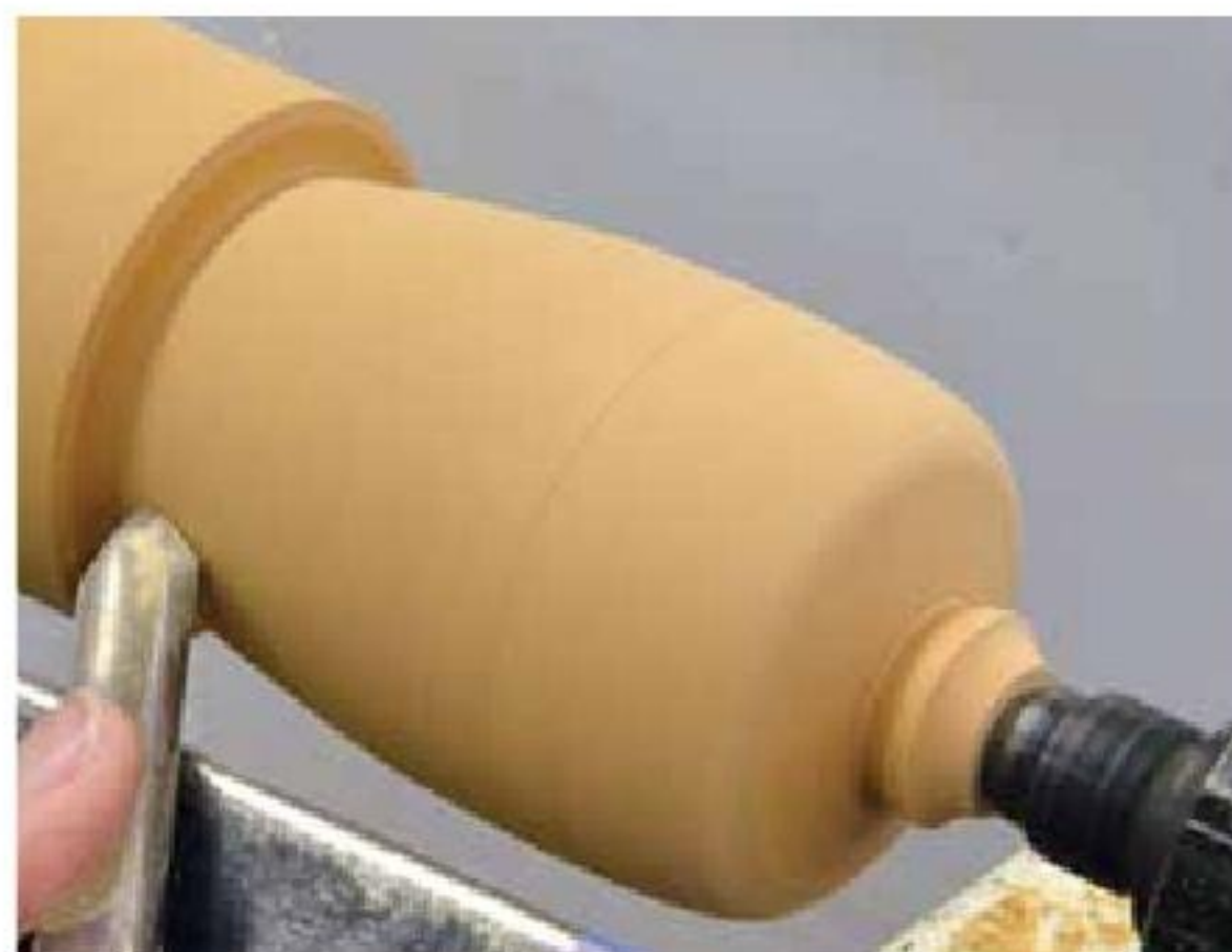
9. Mount the base in the chuck, attach the lid and shape the exterior.
