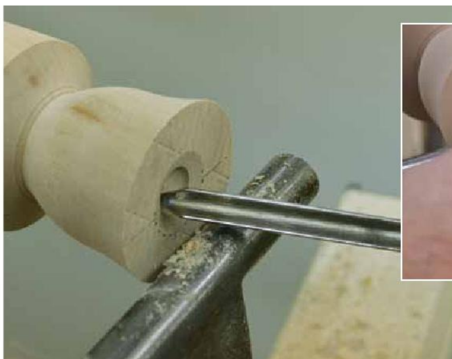
4. Drill a depth hole to about 90% of the cup's depth.
