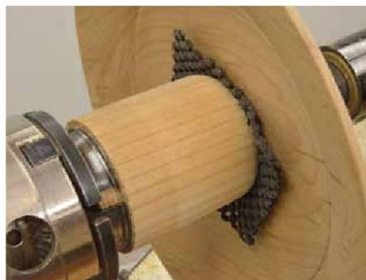
13. Set up the jam chuck to hold the platter without marring the completed center.
