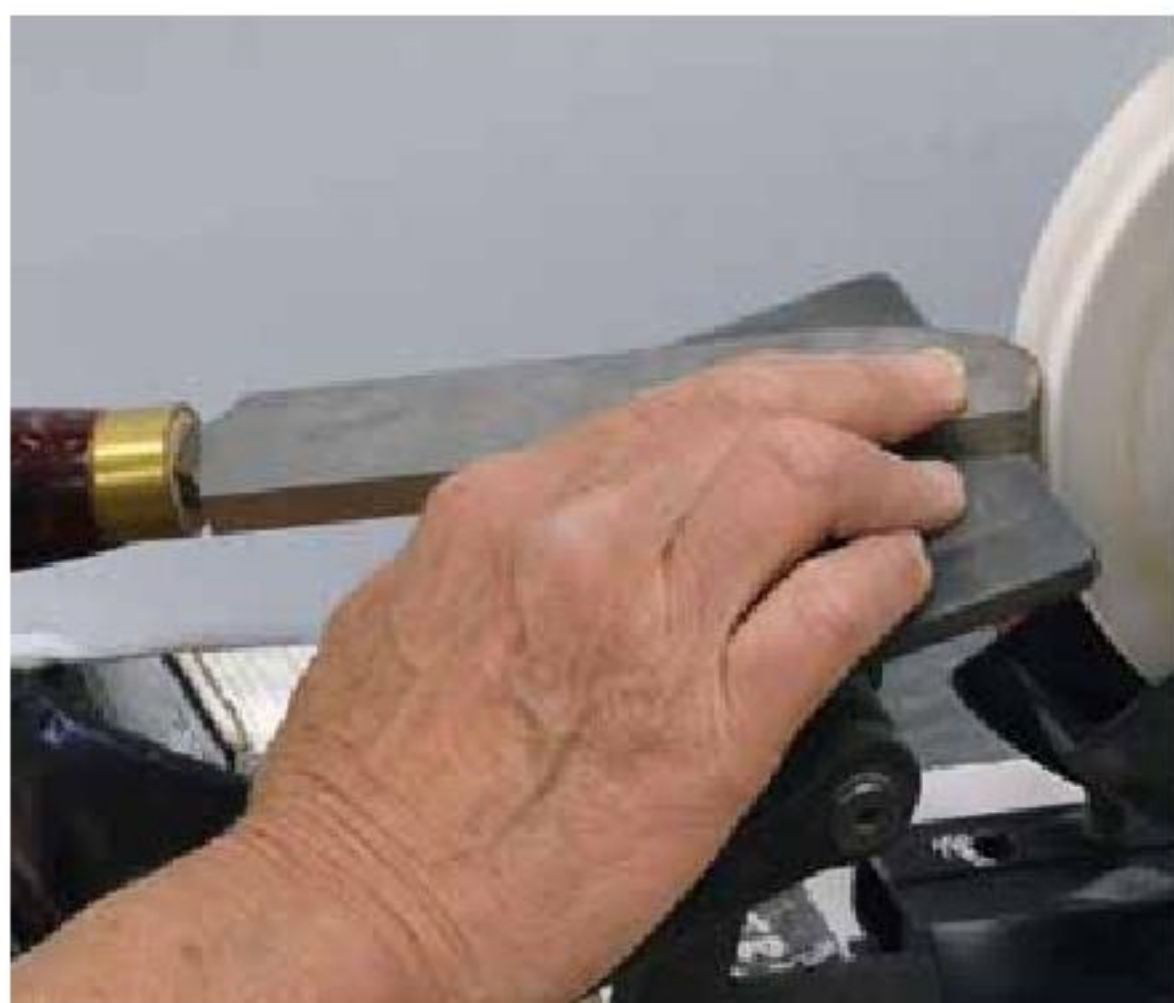
18. Sharpen a scraper by laying it on the platform and rotating it.
