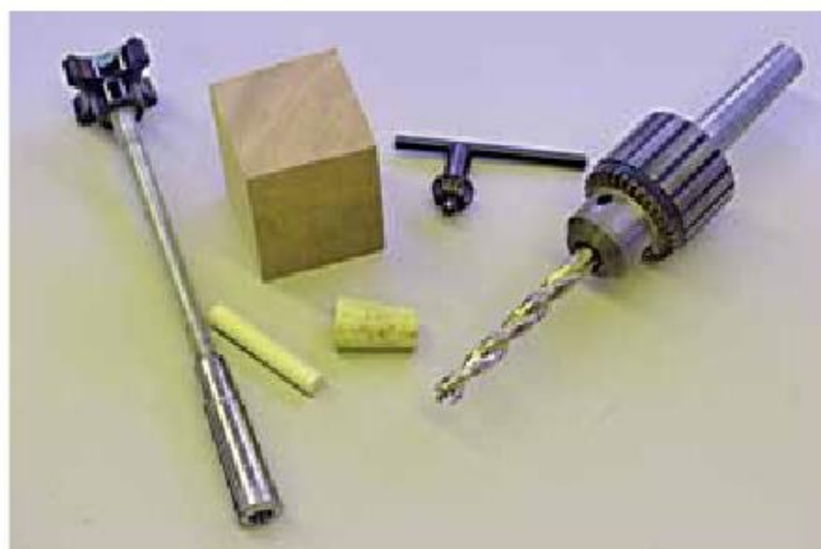
18. A ⅜" drill, dowel, and collet chuck are ready to start a stopper project.
