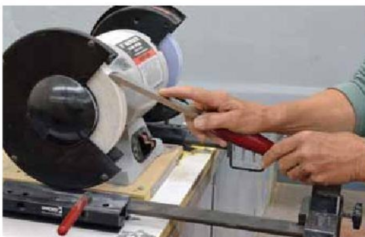
7a. Set the right face of a skew chisel using a "T" fixture.
