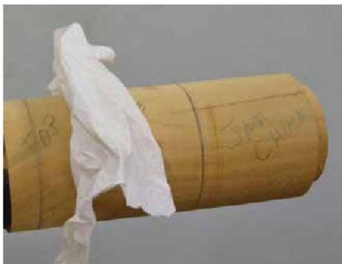
8. If the lid is too a loose, use a paper shim.
