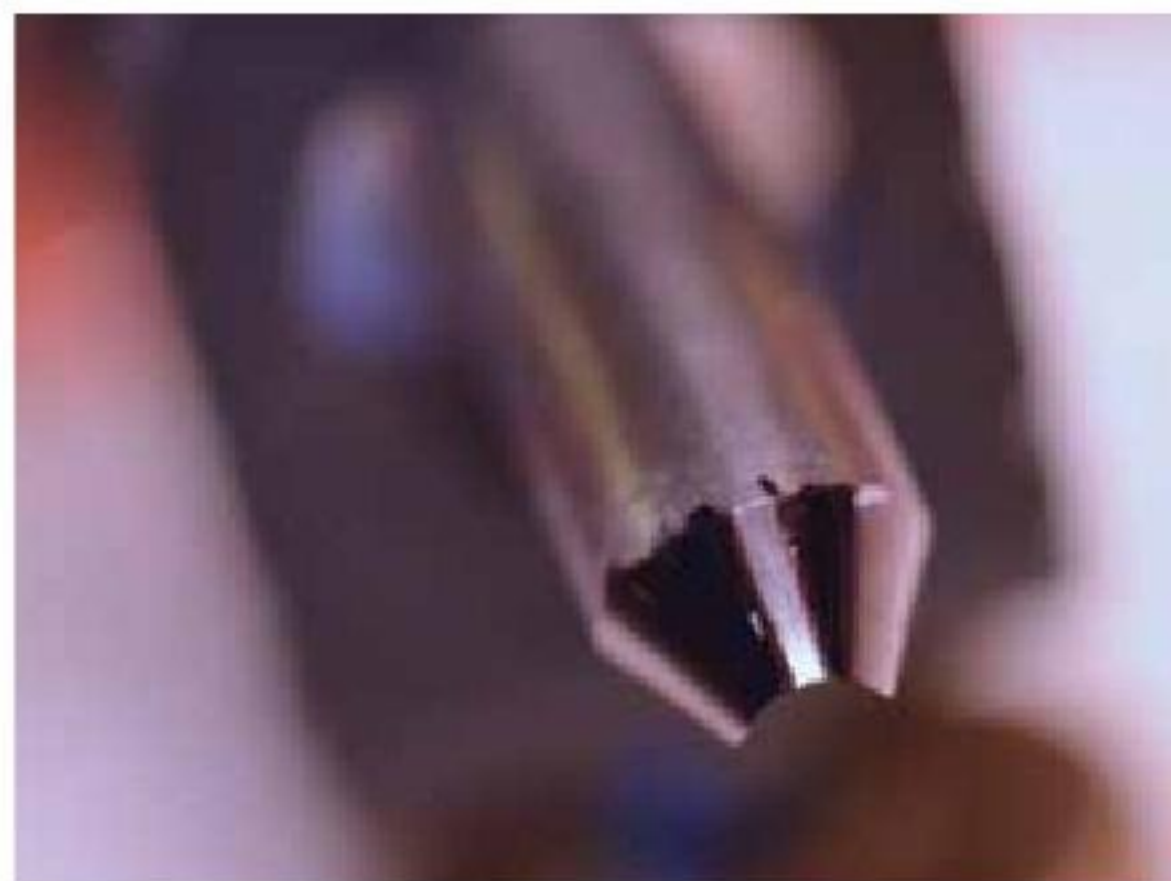
4. The fixture is properly adjusted to fully align with the tool bevel.
