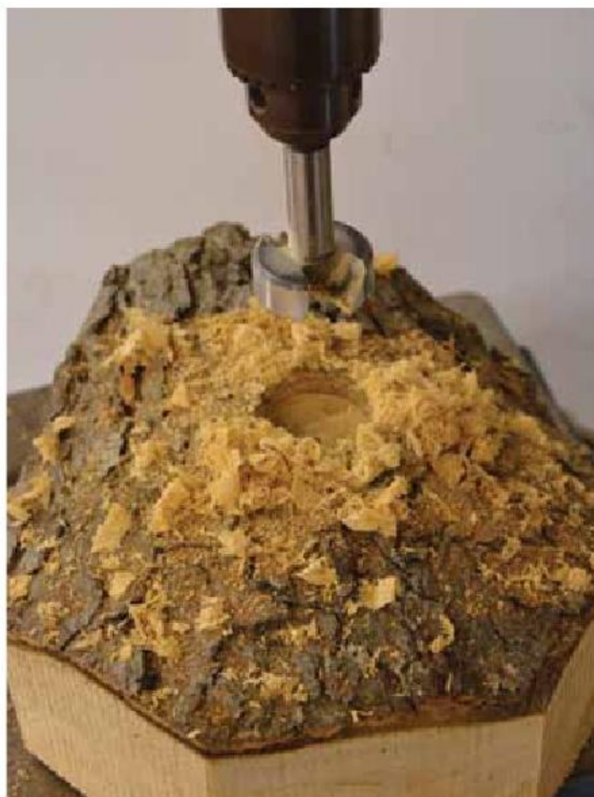
2. Drill out the bark to give the live center a solid bite into the hard wood.
