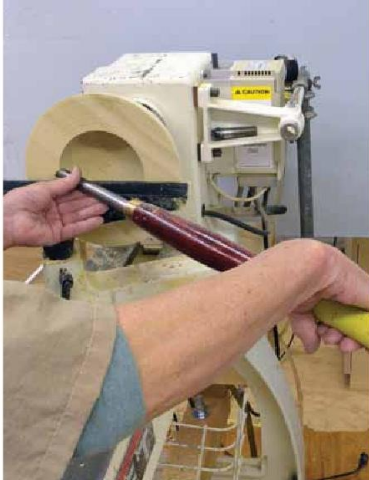
9. Phase I—Right Hand Push: The starting position is with the wrist over-rotated and the cutting edge vertical.
