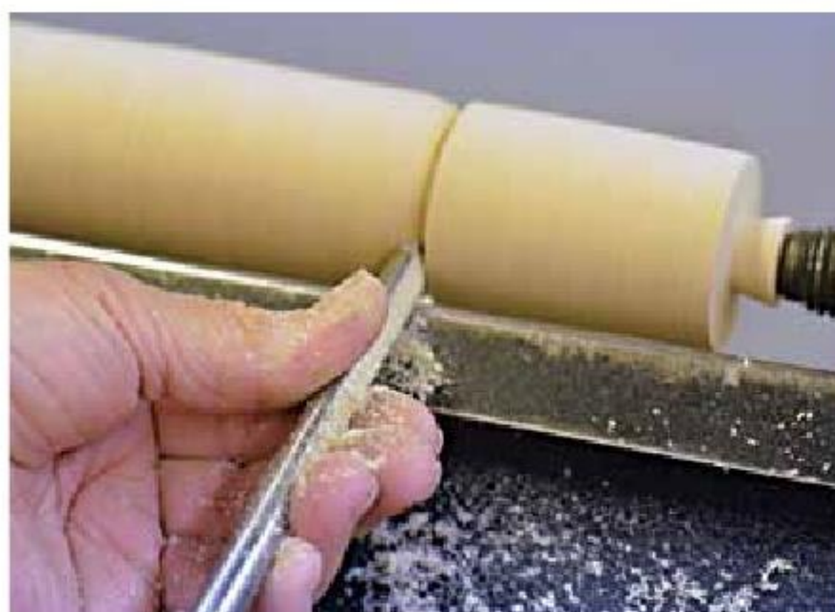
14. Completing the bead, the gouge is almost vertical to keep the edge cutting.
