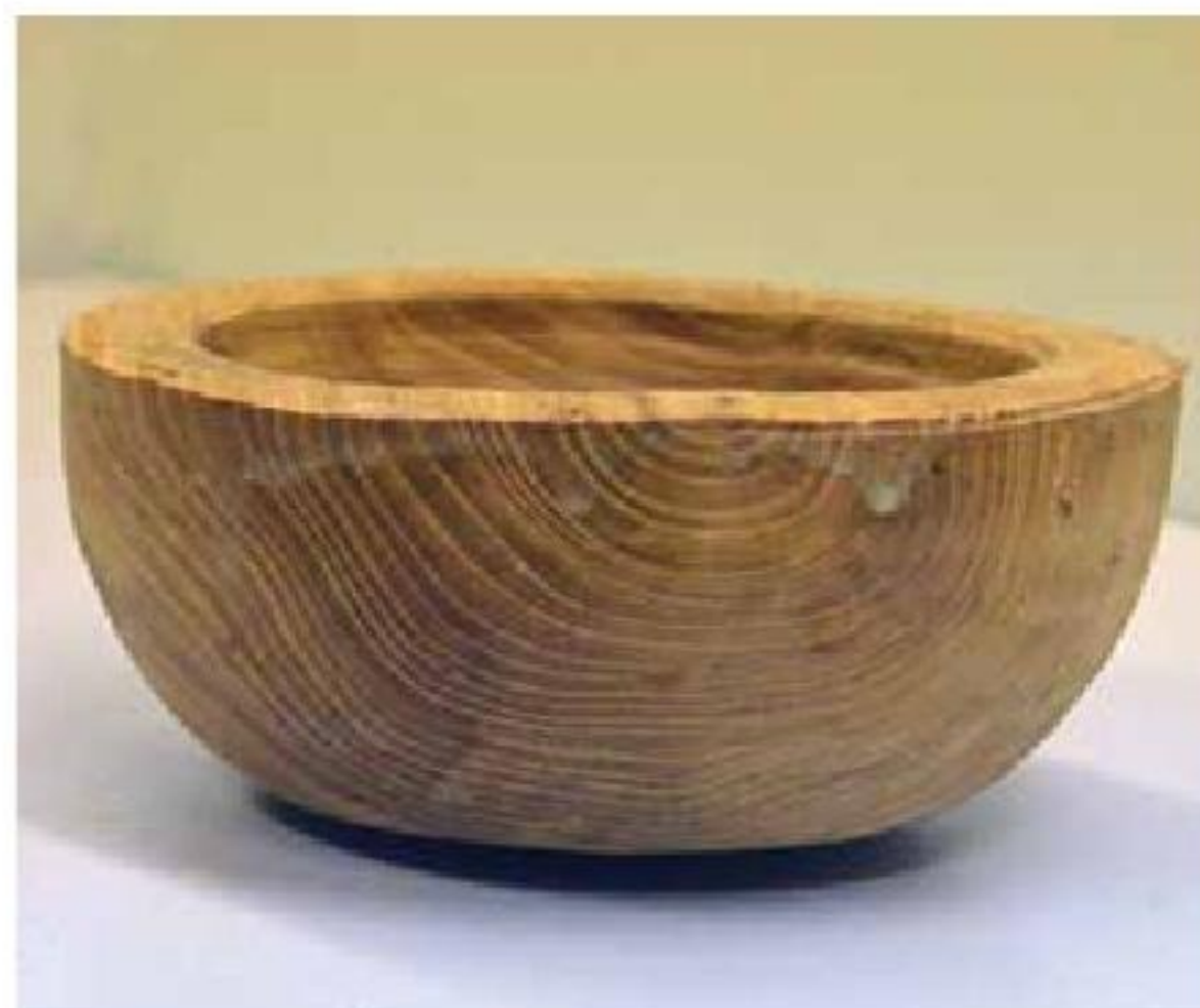
10. Blanks distort more in the direction of the growth rings as they dry.
