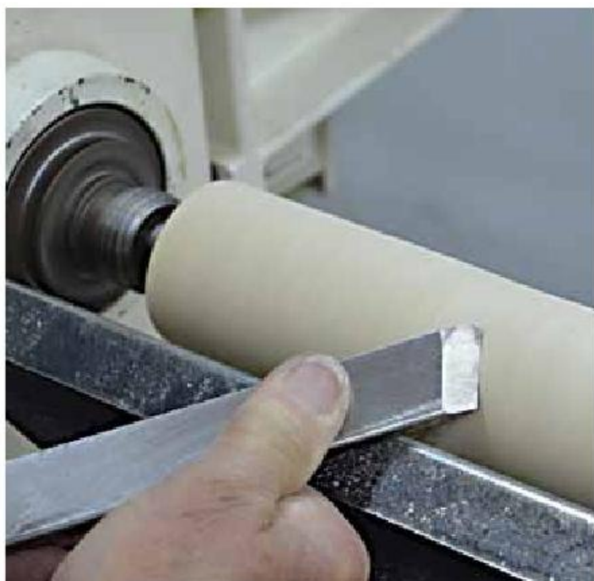
4. Start the planing cut with the skew in this position, cutting toward the right.
