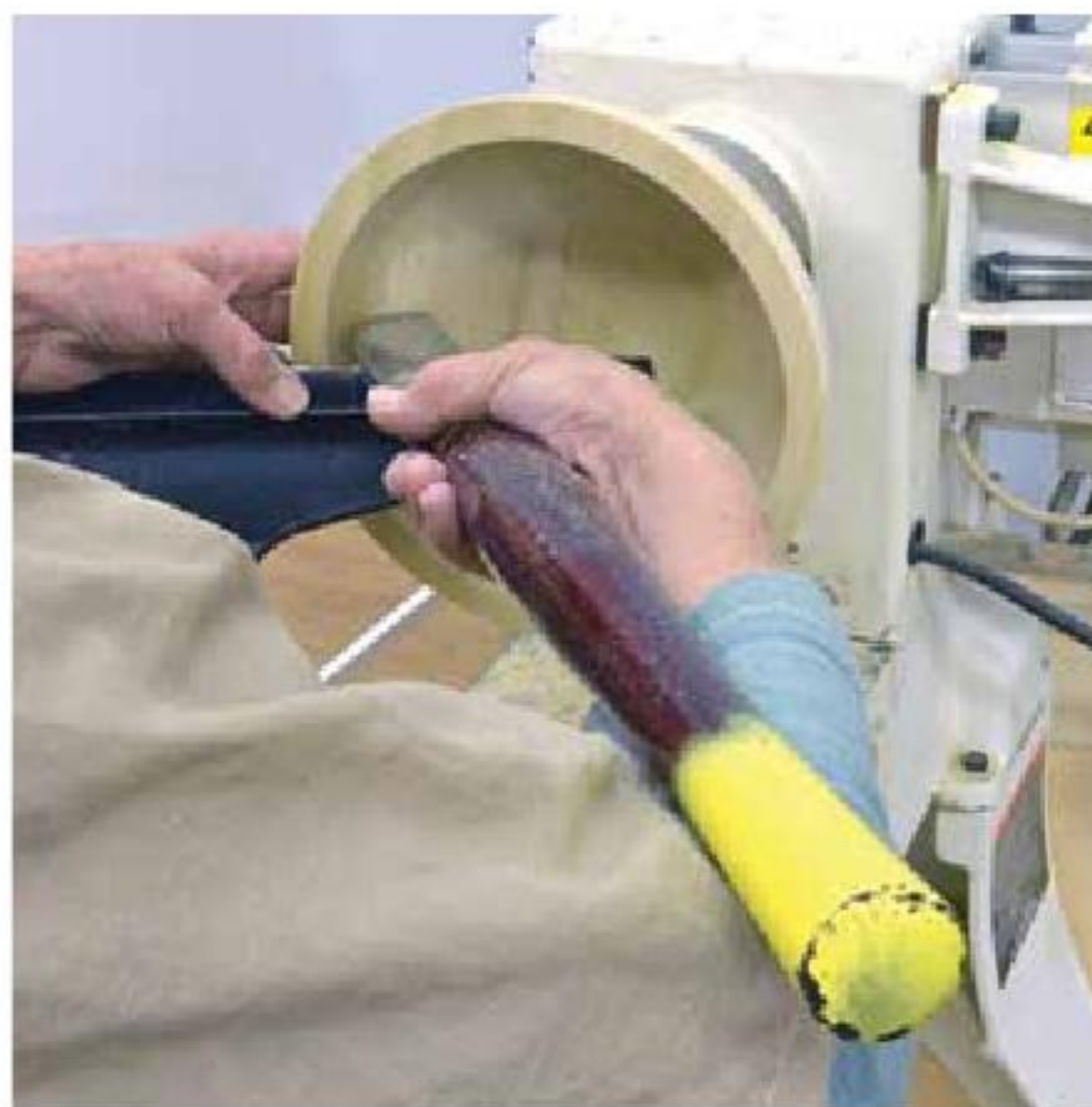
10. Use a bowl scraper to perfect the interior; be sure the cutting edge is trailing down to the center.
