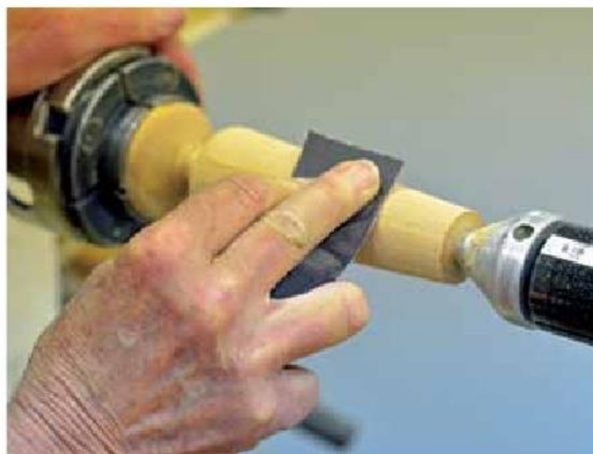
12. Completing the sanding on the lathe saves time and effort.
