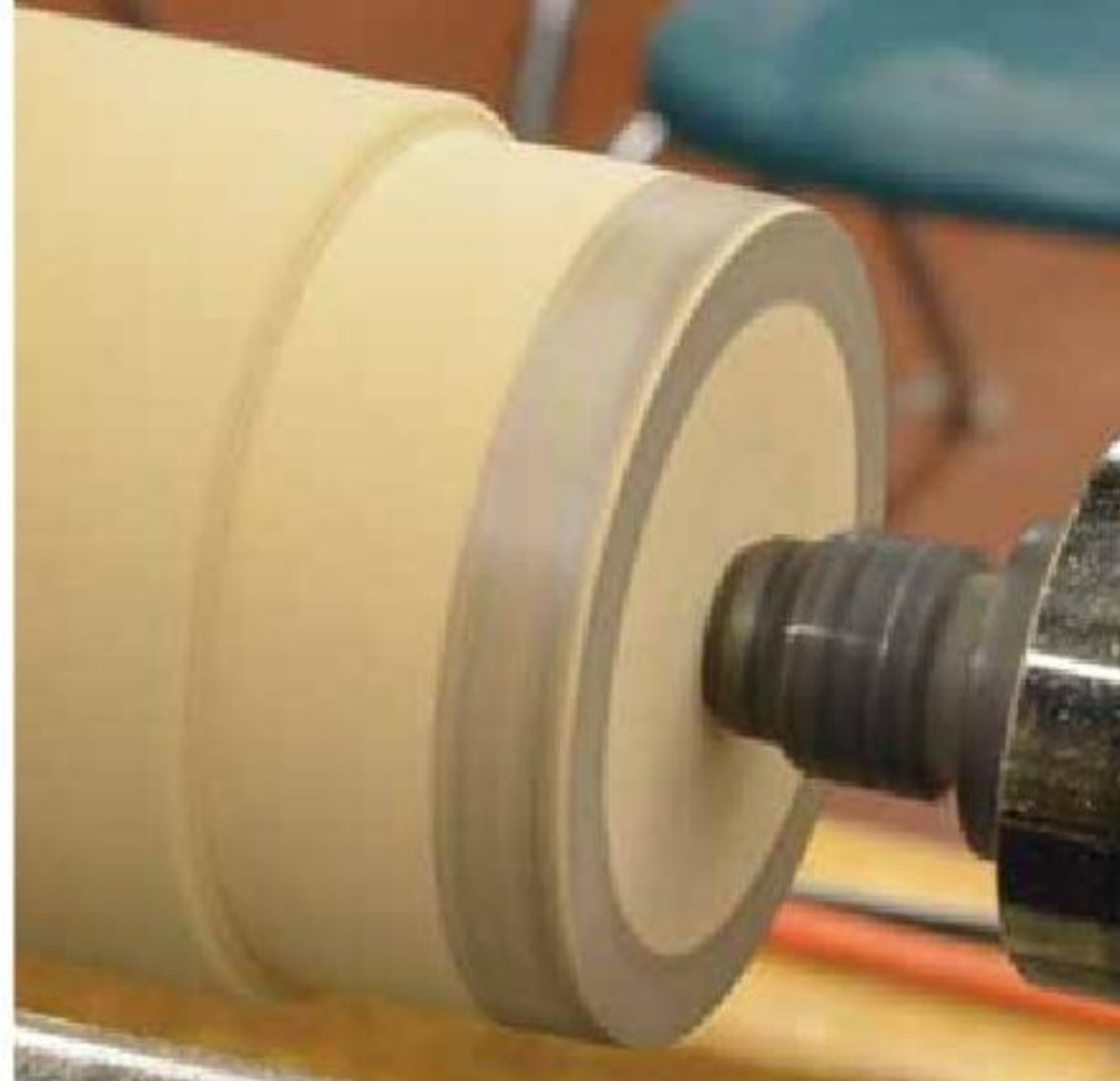
2. After transferring the measurements, this tenon is ready to be cut.
