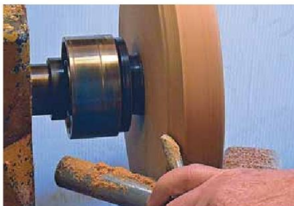
6. Complete the seat profile by chamfering the back edge, ready to sand.
