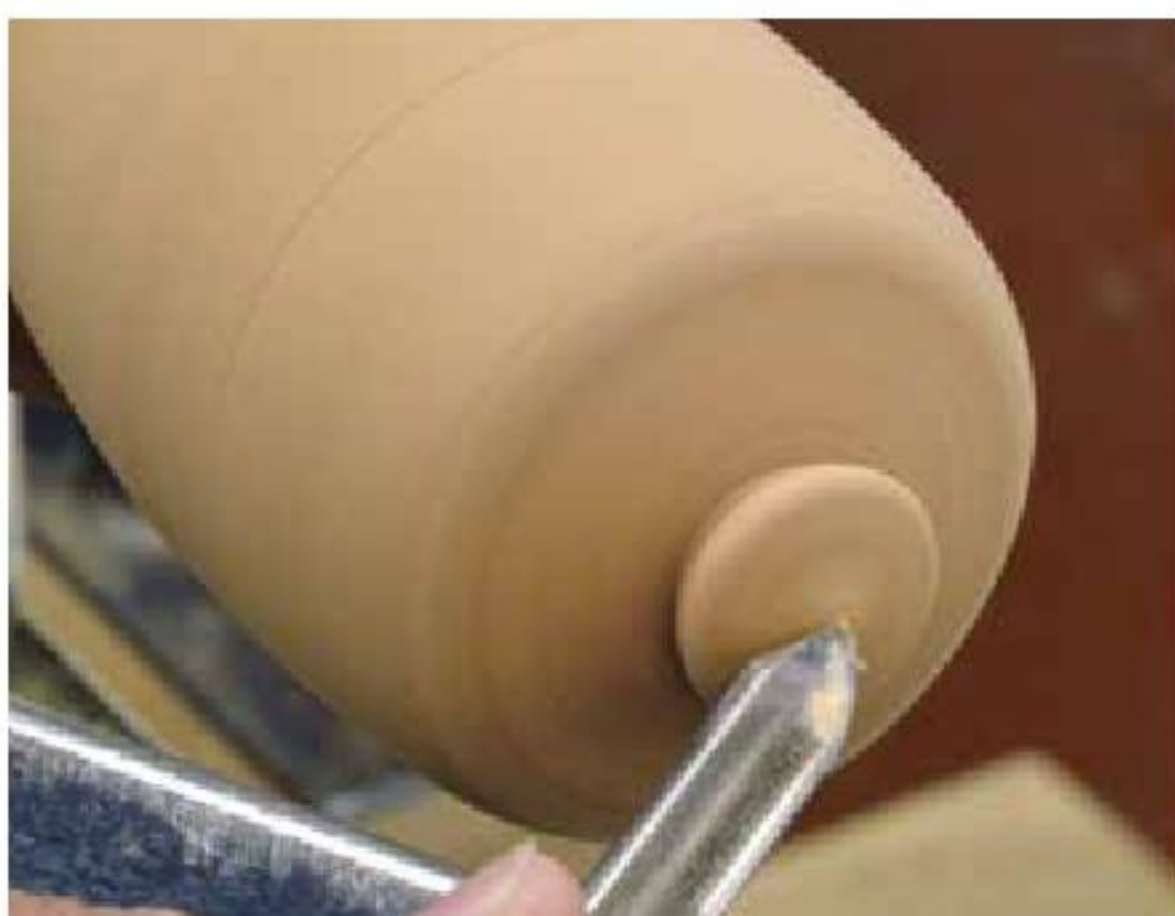
10. Complete the top of the lid carefully, pushing toward the base only.
