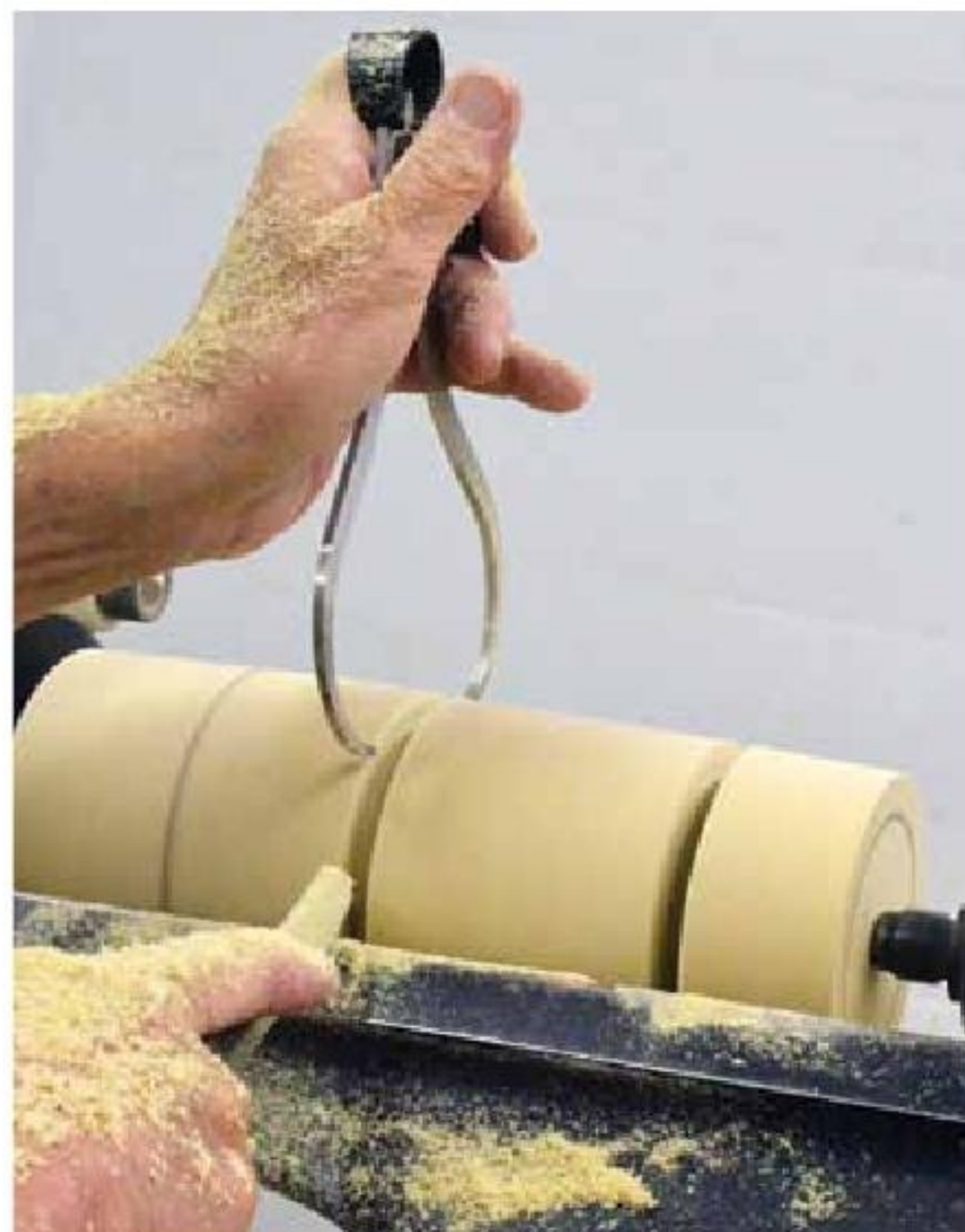
34. Lay out the vase diameters with your parting tool and calipers.
