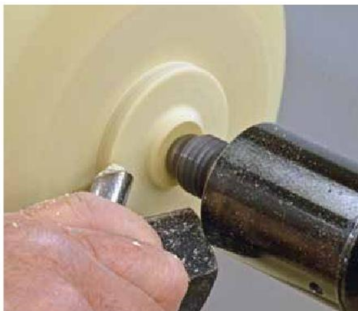
13. Reduce the tenon and complete the foot.
