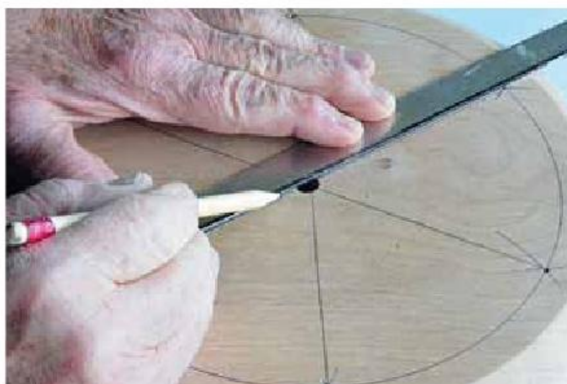
7. Laying out the alignment lines for drilling the leg holes.
