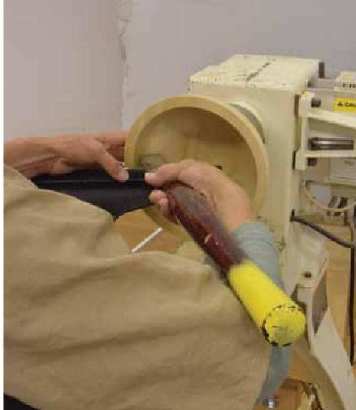
7. Support the scrapers on top of your arm to assure the safest cutting angle.
