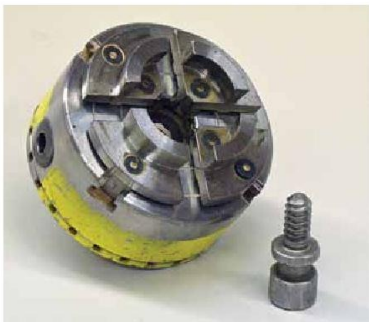
5. Some brands of chucks require a dovetail shape to match their jaws.
