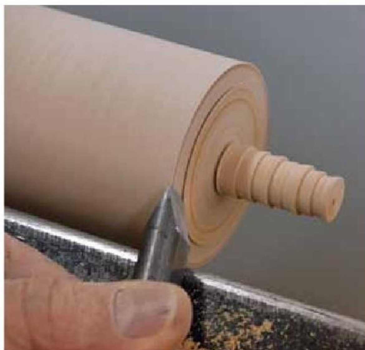
19. A “V” cut will clean up the top face.
