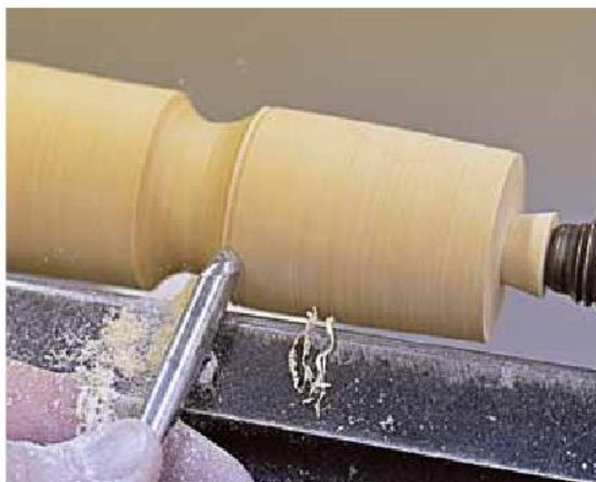
15. Start a cove cut to the left with the tool engaging the left cutting edge.
