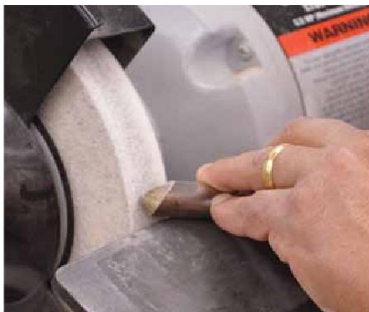
16. This is the finishing position for the right hand side.
