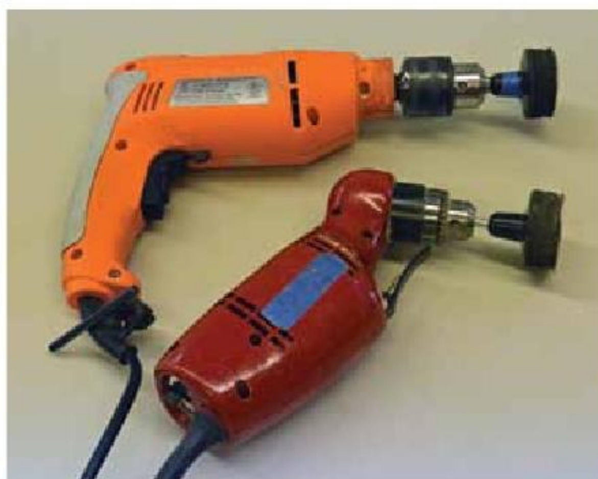
2. Power drills with sanding disks attached can be more aggressive.
