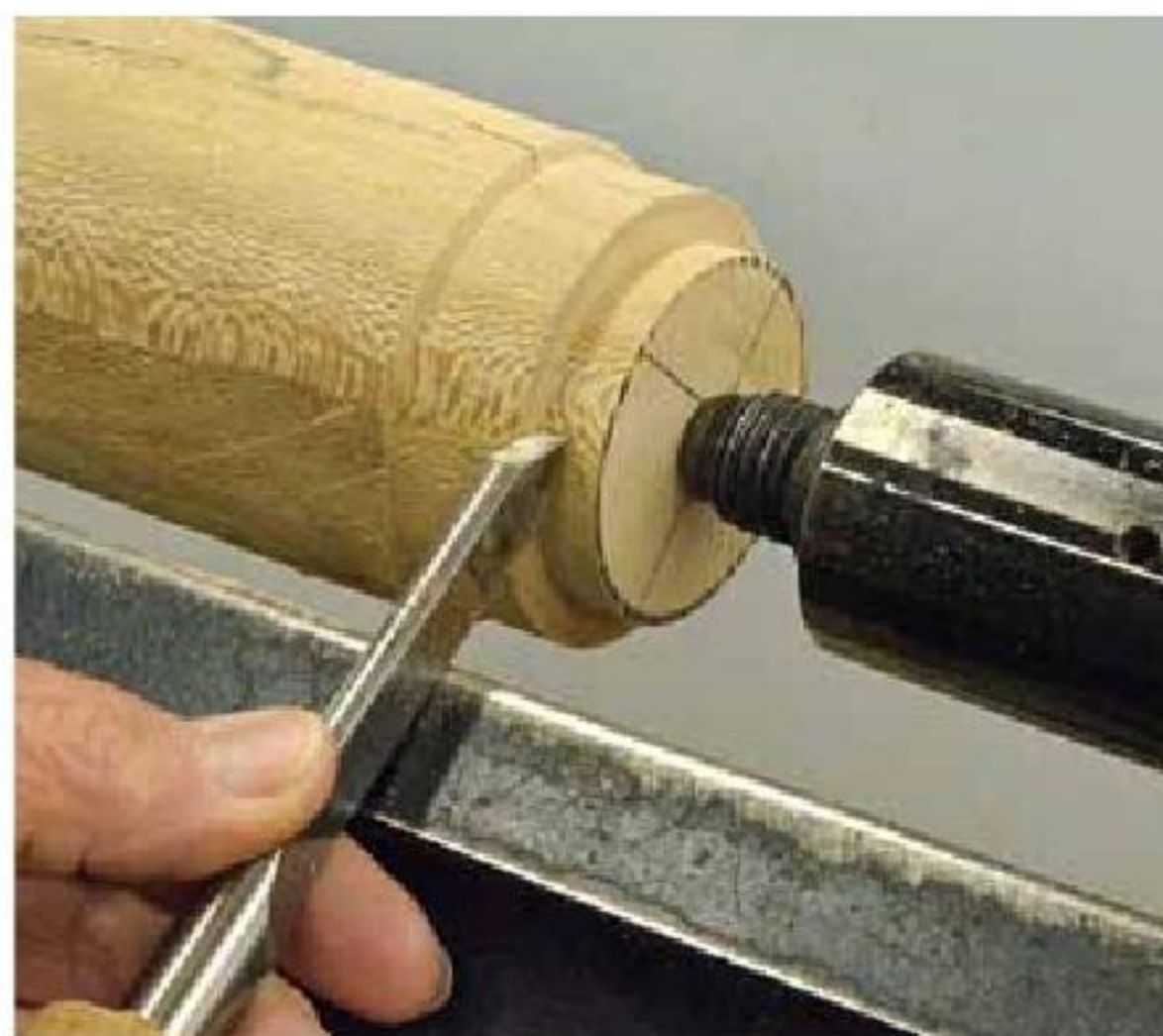
3. A square shoulder is important for a good, tight hold. Keep it straight.
