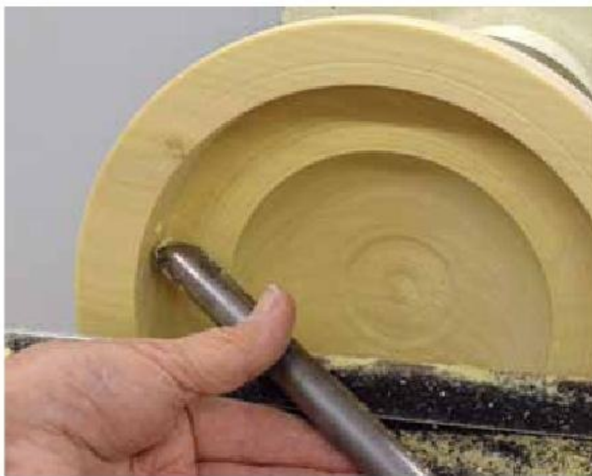
8. Hollowing the interior in 1" increments.
