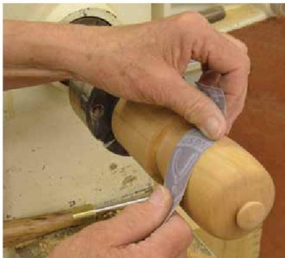
12. Sand and complete the exterior.
