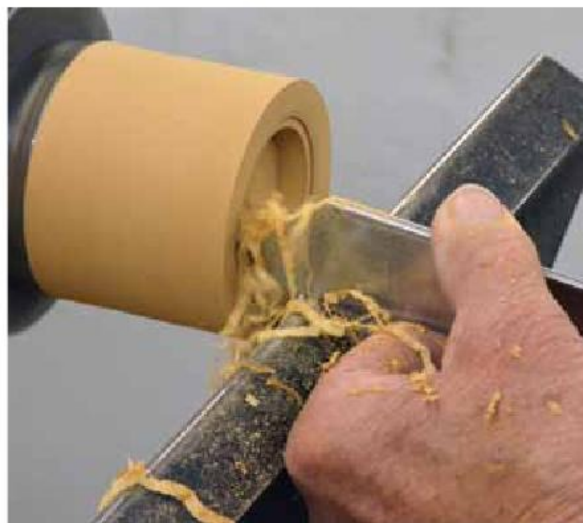
14. Make the final jam chuck to fit the box body.
