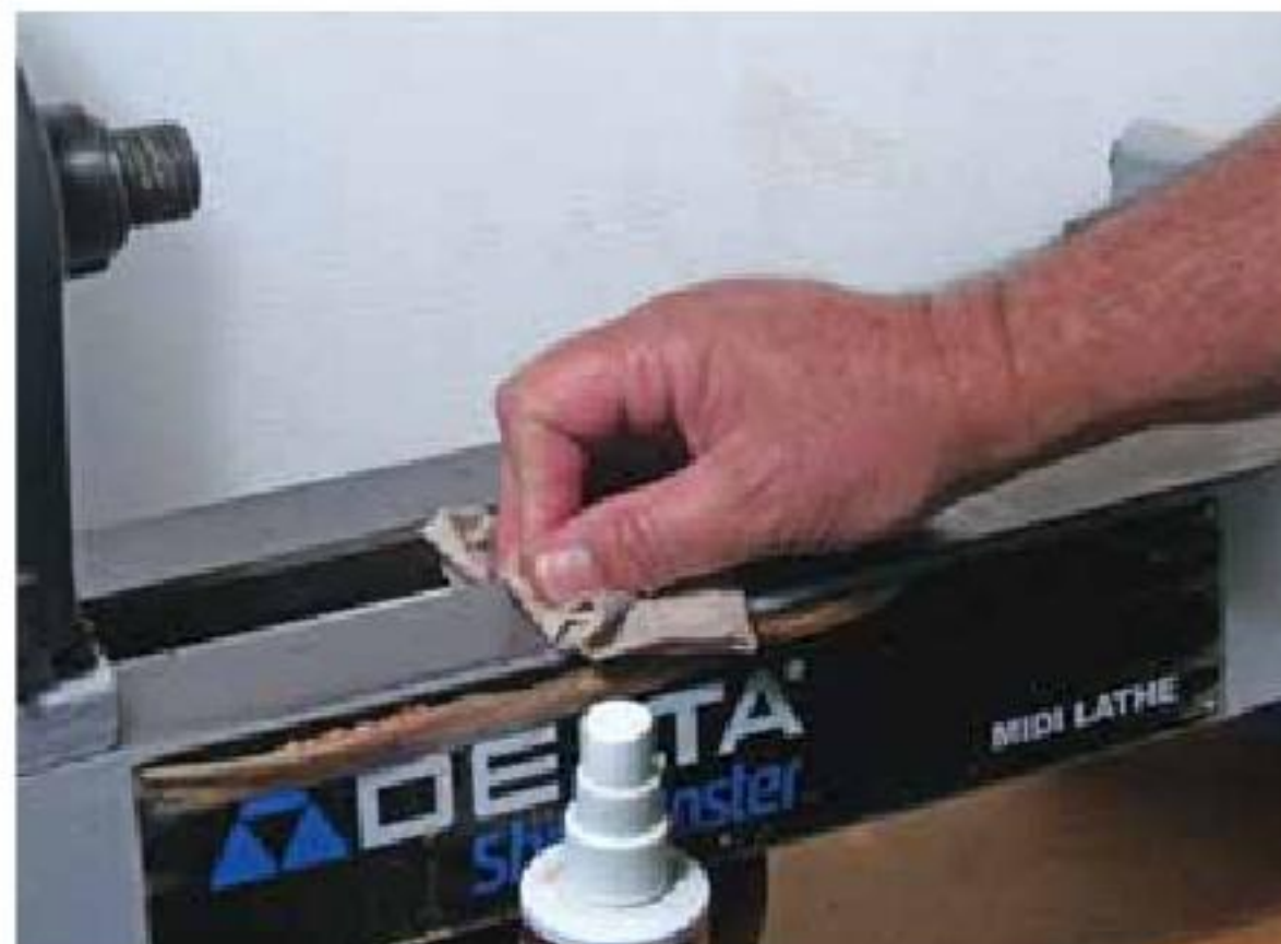
2. Clean the ways and only use silicon spray to lubricate.
