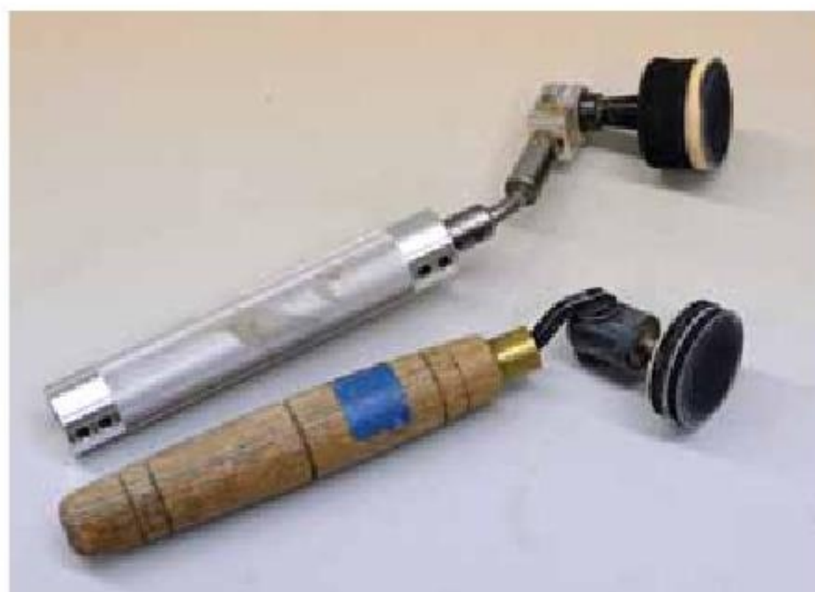
1. Inertial sanders operate with the lathe's rotating motion.
