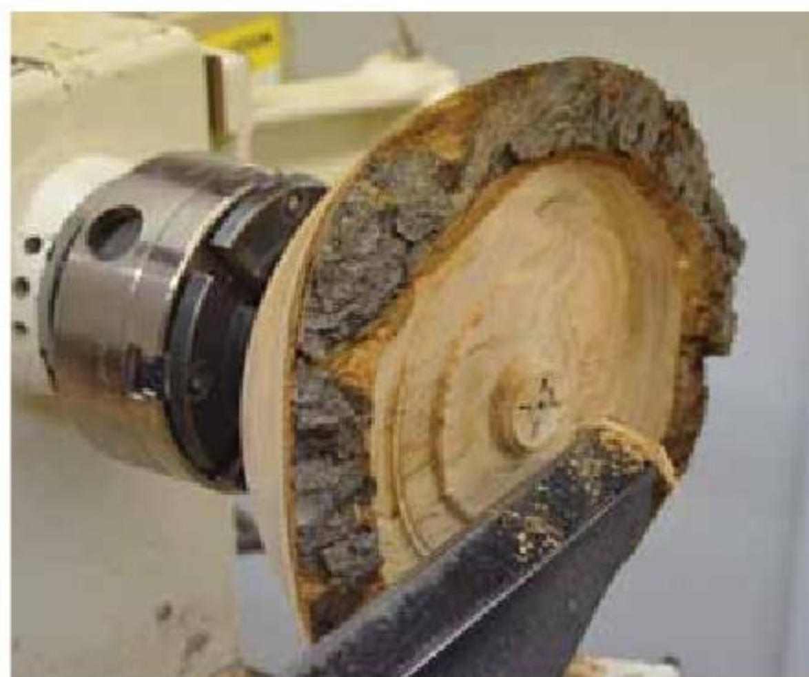
6. Start to cut the interior down to solid wood.
