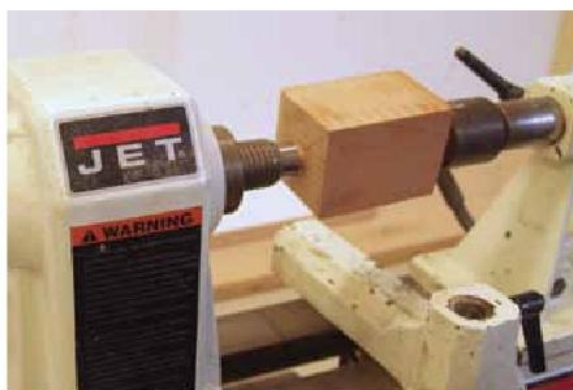
20. Mount the blank on the lathe by tightening the collet chuck into the headstock taper.
