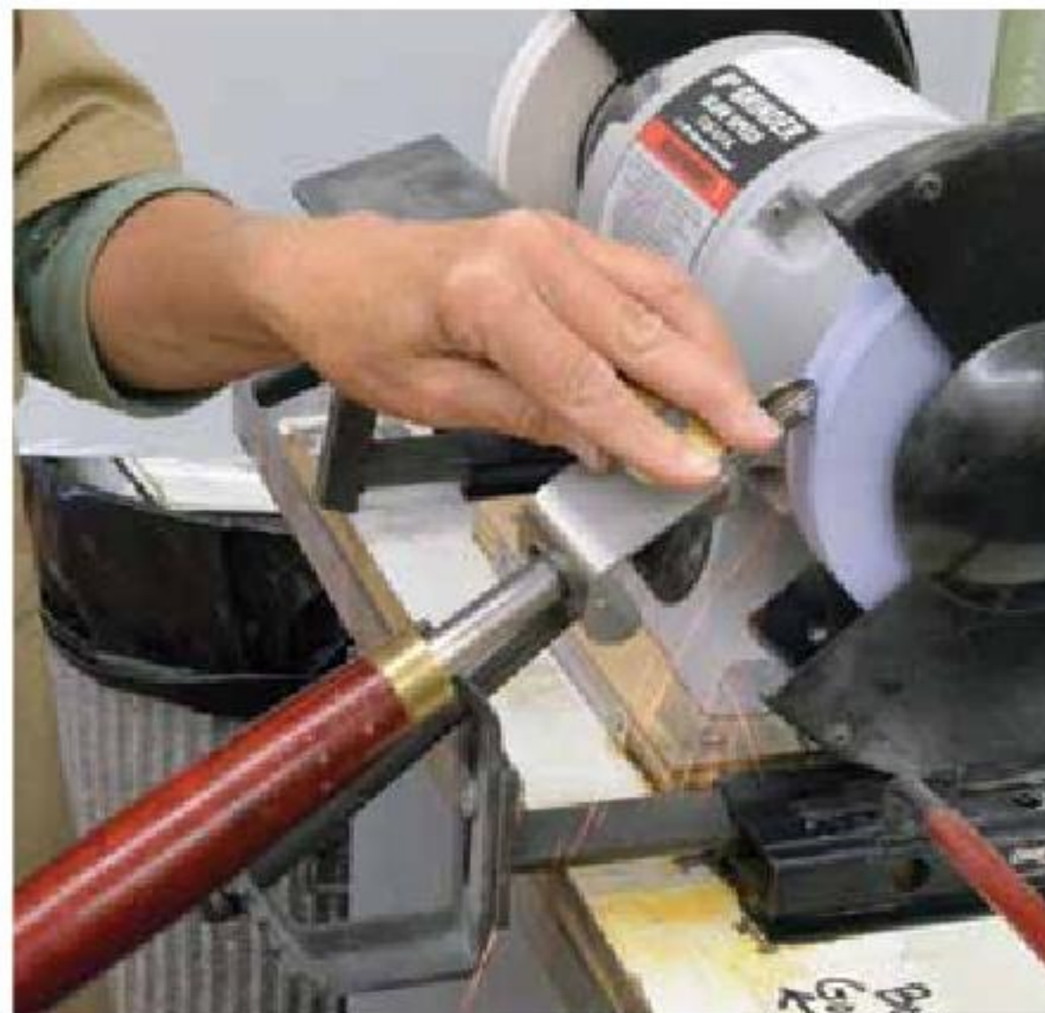
12. Sharpen one side by sweeping the fixture to the right side.
