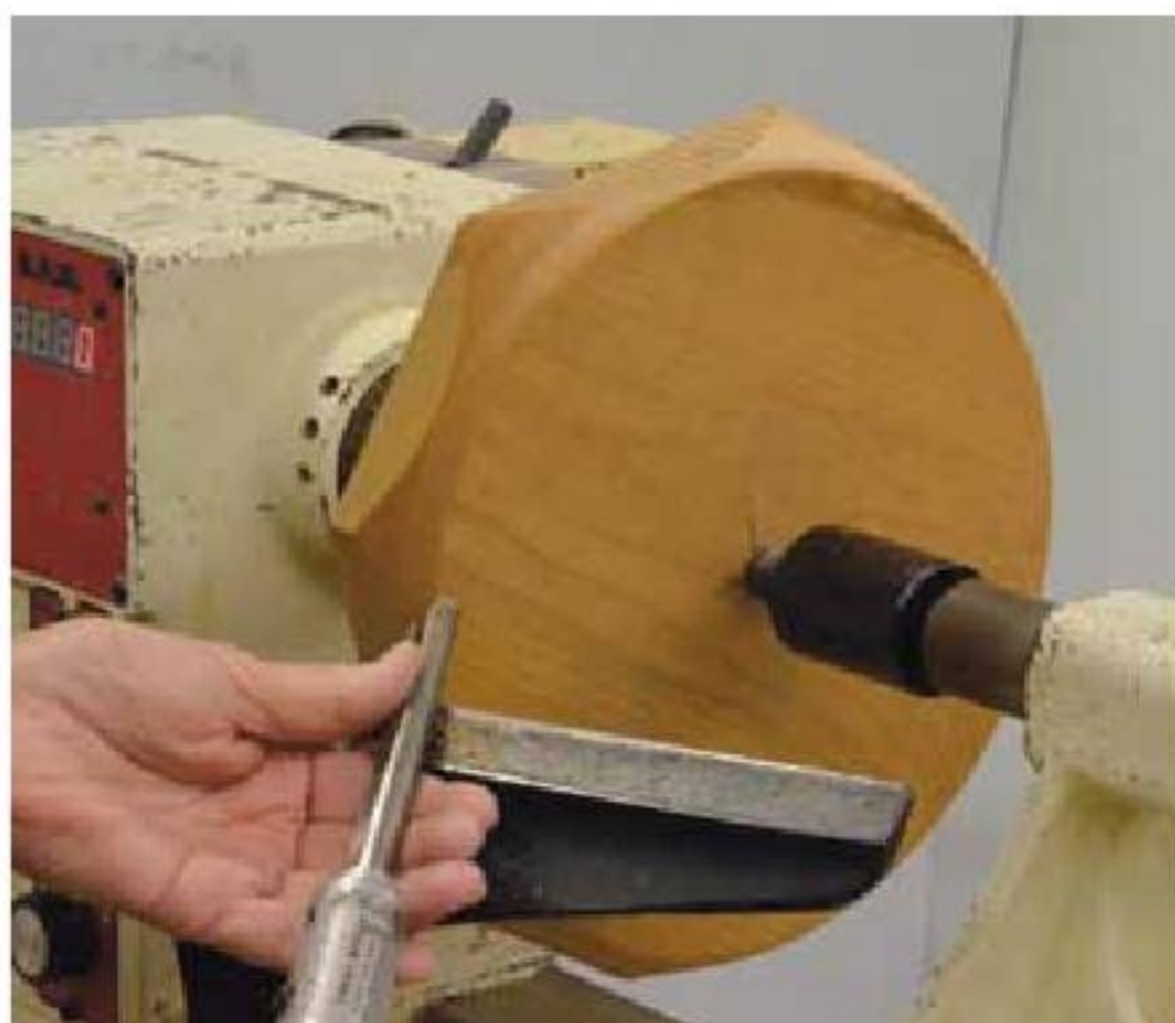
3. Round the edges of the blank from the face sides, maintaining the rule of 45's.
