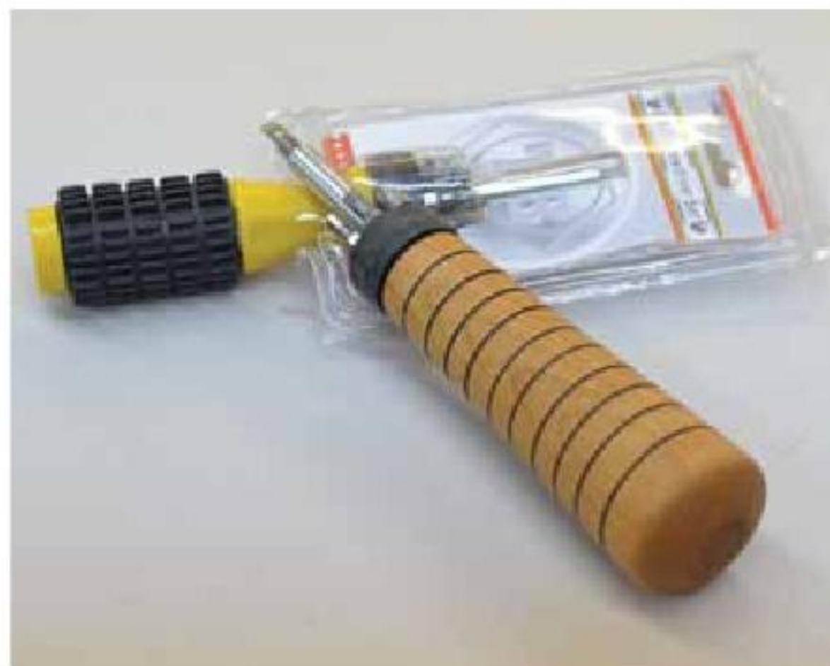
8. An inexpensive screwdriver can easily be dressed up with a custom handle.
