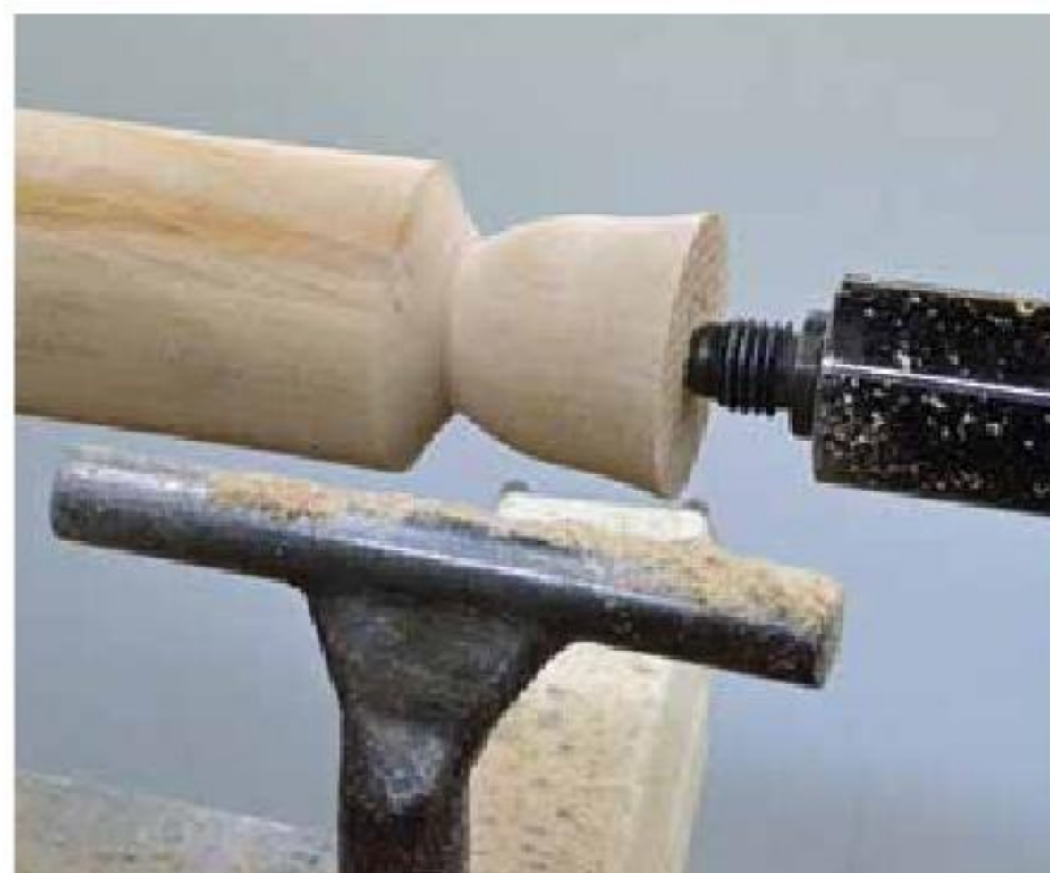
2. Begin by shaping the cup exterior.
