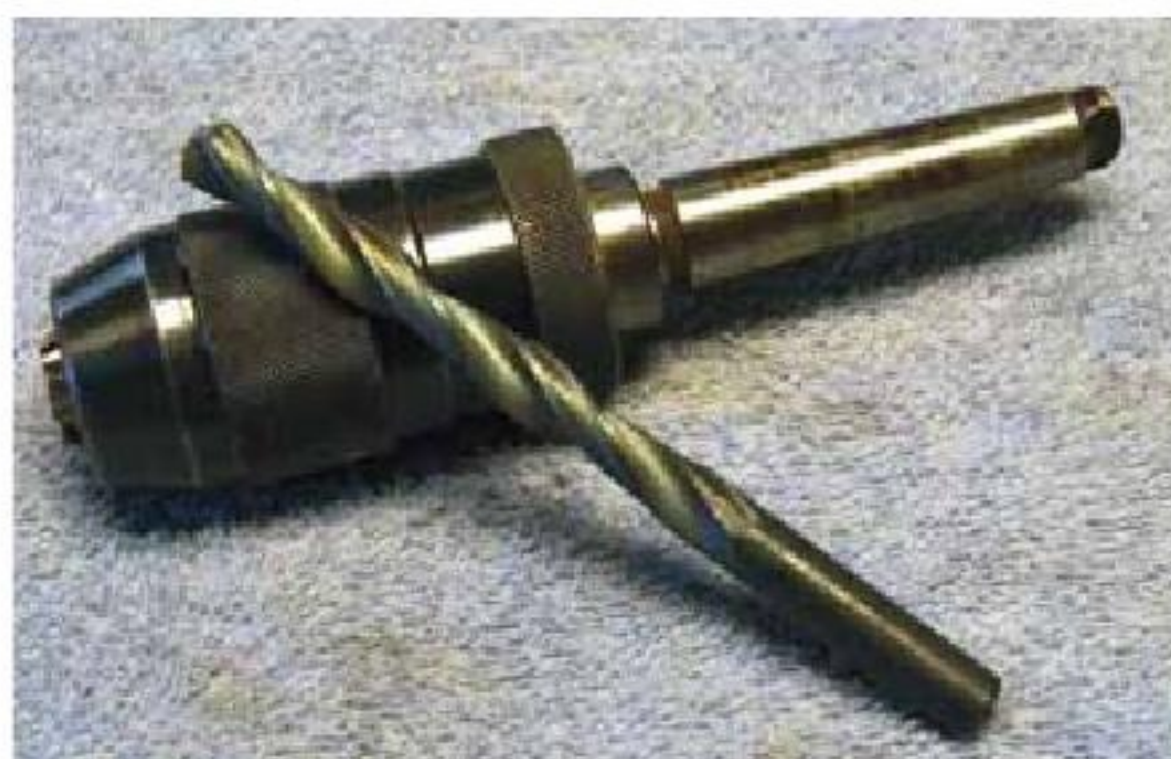
7. A Jacob's chuck mounted to a Morris taper is a major accessory for drilling on the lathe.
