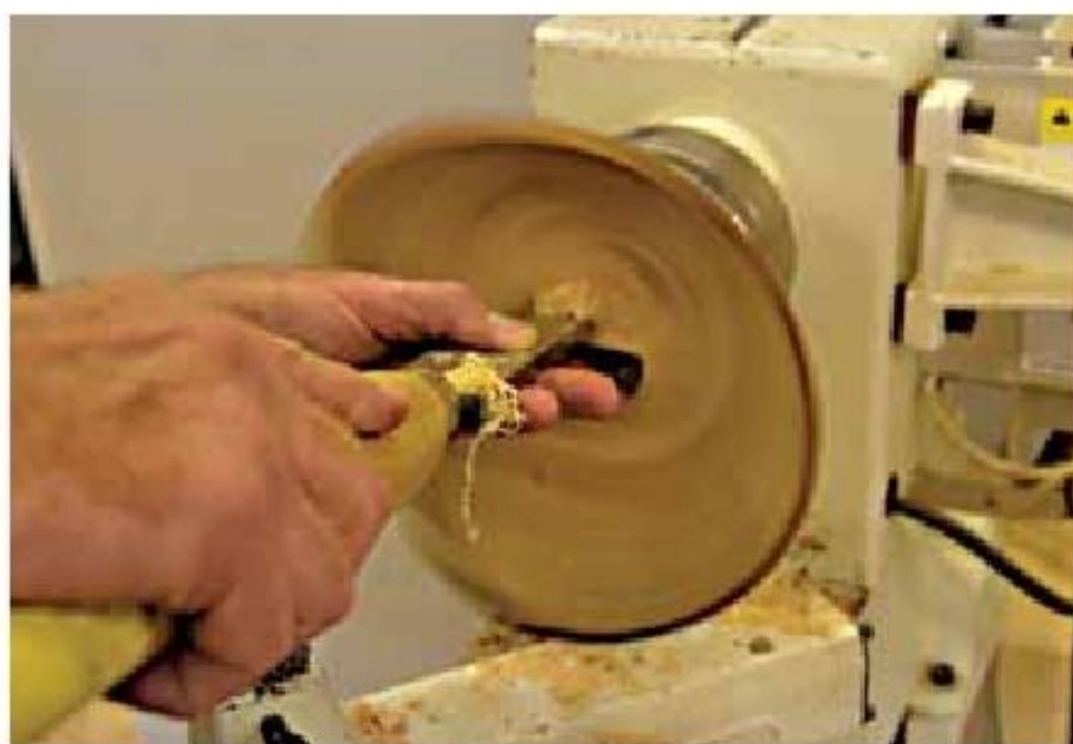
9. Continue cutting 1" at a time all the way to the bottom.
