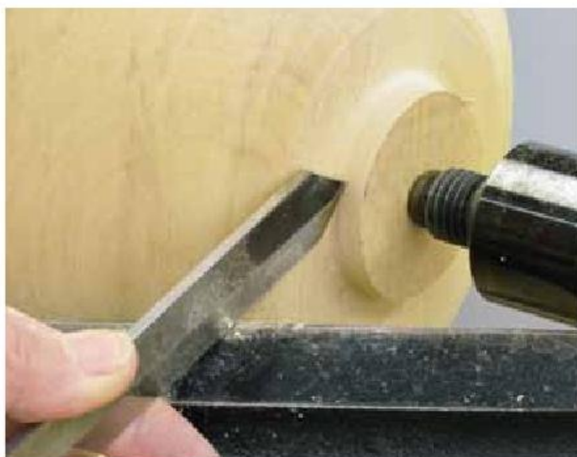
5. Square up a tenon with the parting tool.
