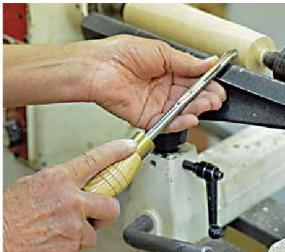
11. The starting position for a right hand bead places the index finger on top of the tool.
