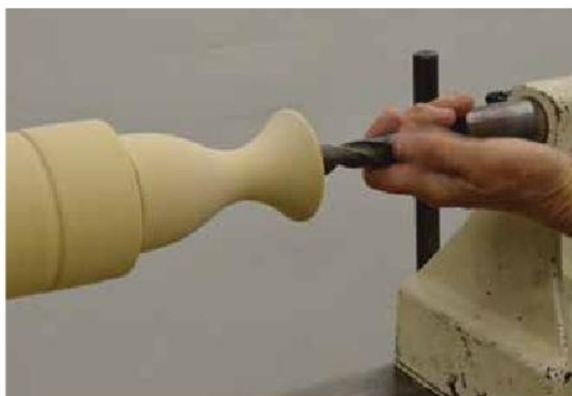
36. Drill the interior hole by slowing the lathe speed first.
