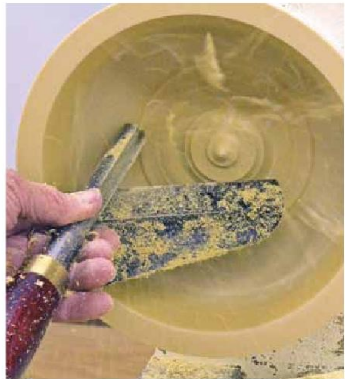
9. Complete cutting the interior with the bowl gouge.
