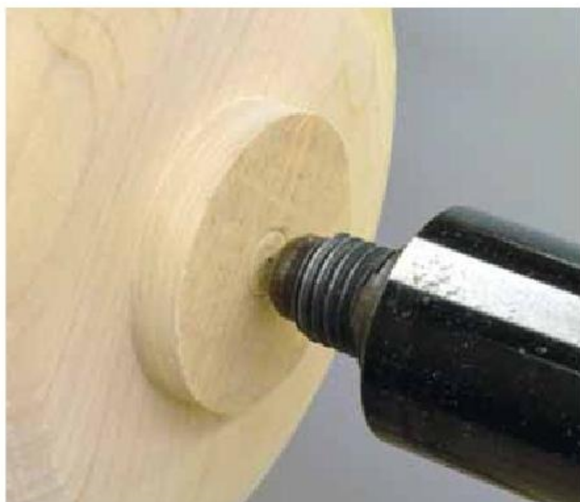
12. To get the alignment, place the live center into the pinhole at the base of the tenon.
