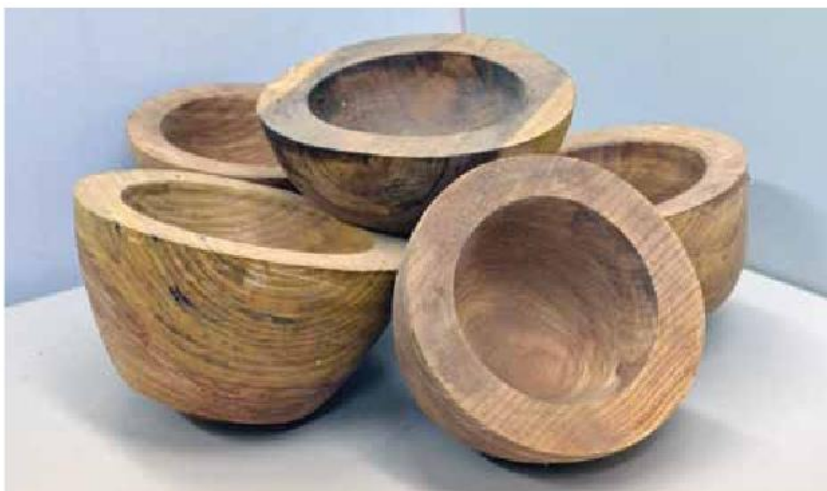
8. Rough out the bowl blanks to a wall thickness of about 10% of the diameter.
