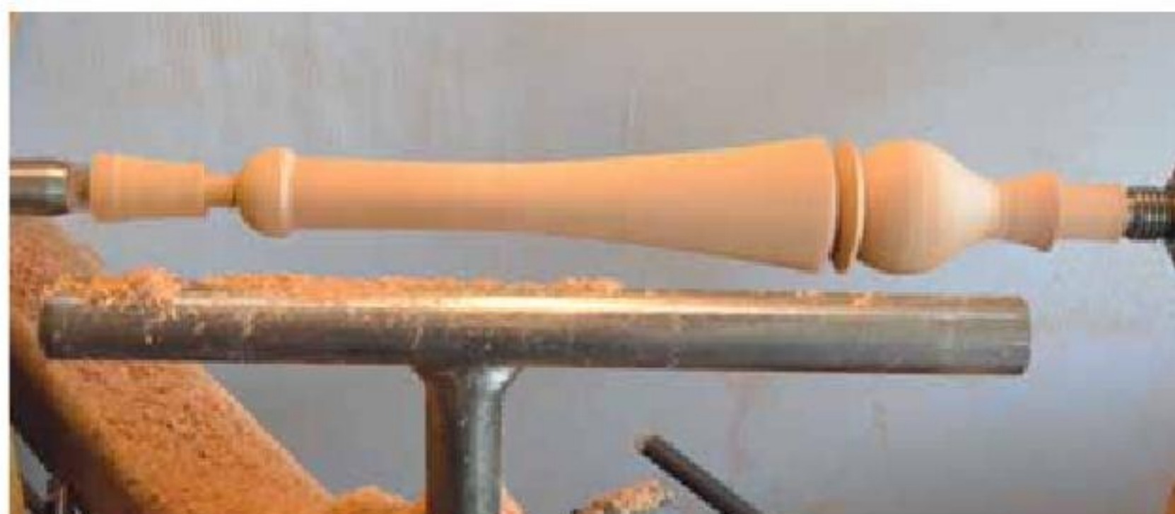
14. A leg turned to the drawing dimensions and ready for sanding.
