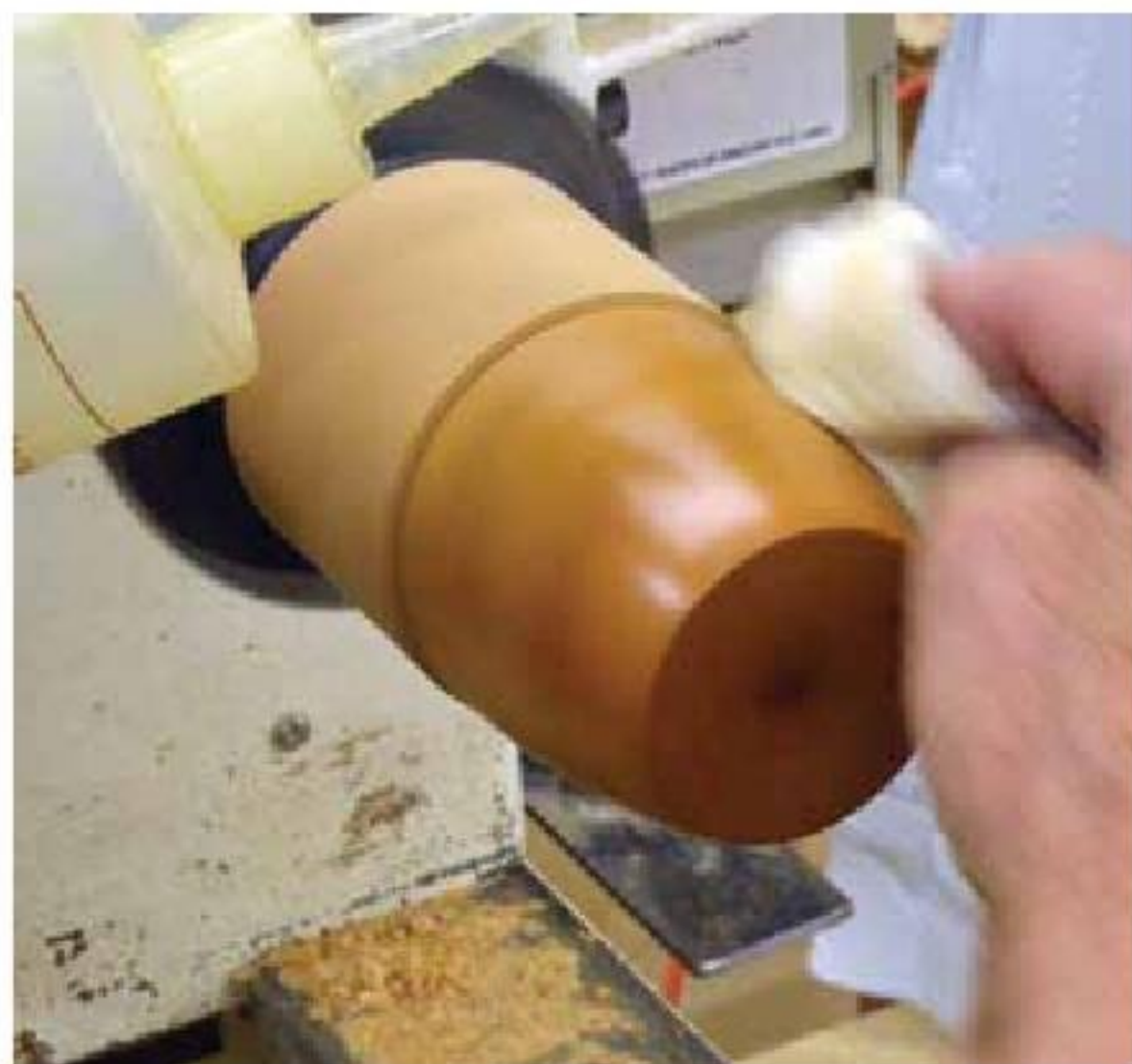
16. Add a coat of finish to complete.
