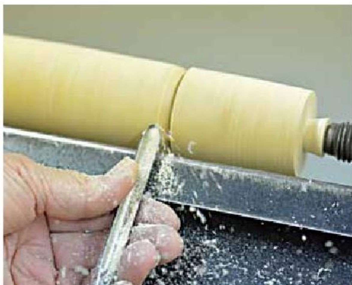
12. See that the lower side of the tool is doing the cut.
