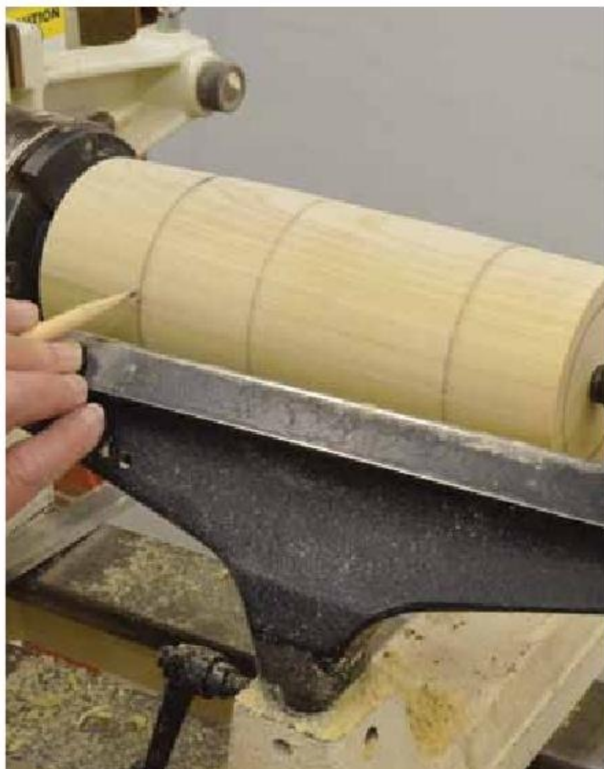
33. Lay out the vase lengths from the tailstock end.
