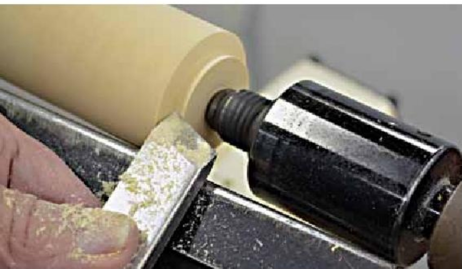
5. Skew chisel flat on the rest, long point facing the wood, ready to make a peel cut.
