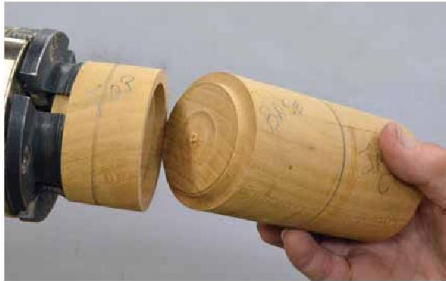
7. After cutting a square internal shoulder, test fit the base.
