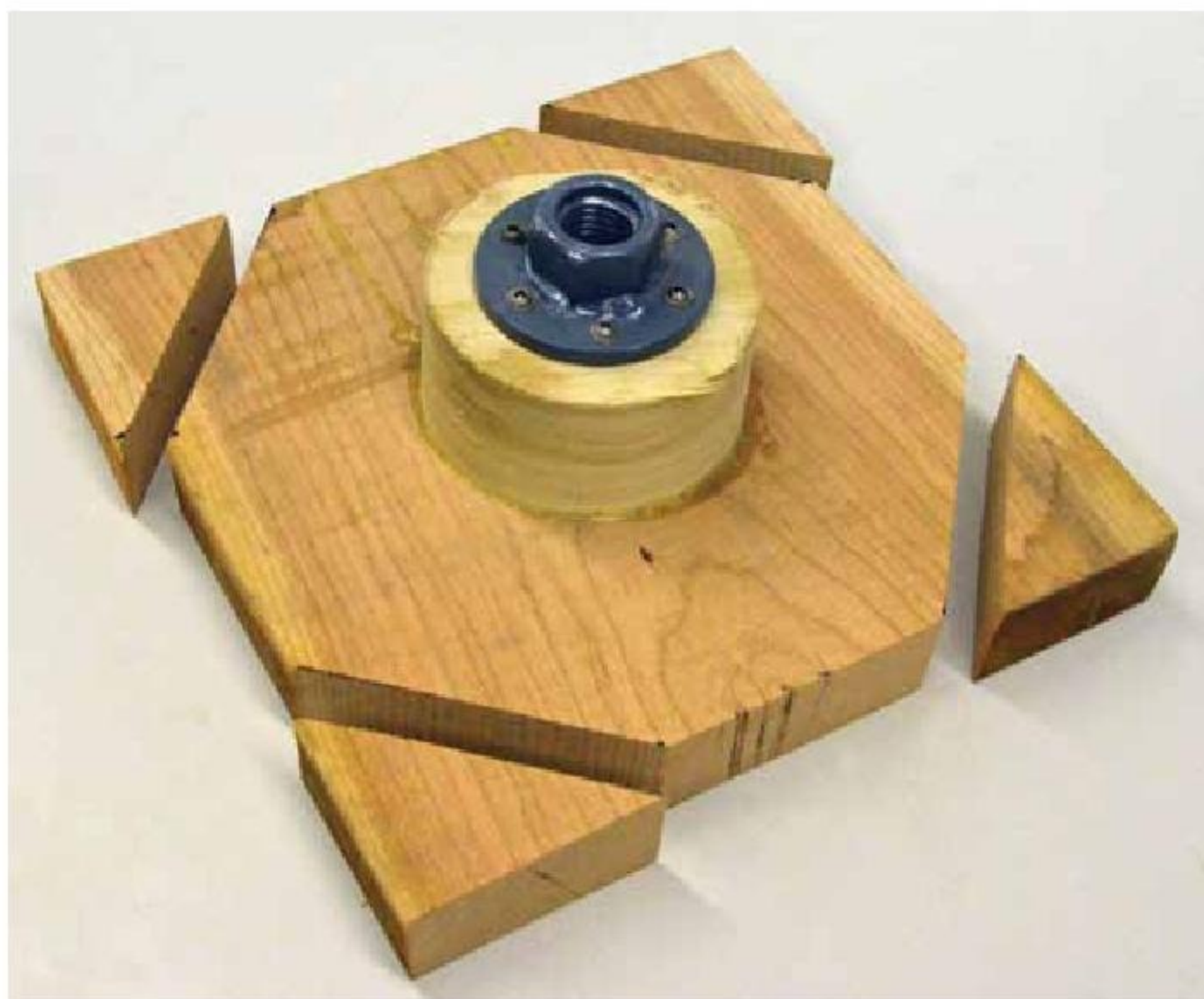
2. The blank is mounted onto a faceplate and glue block assembly and the corners removed.
