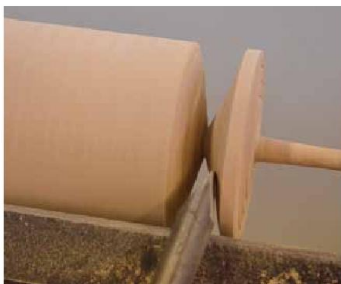
20. Parting off with a skew creates the spin point at the same time.
