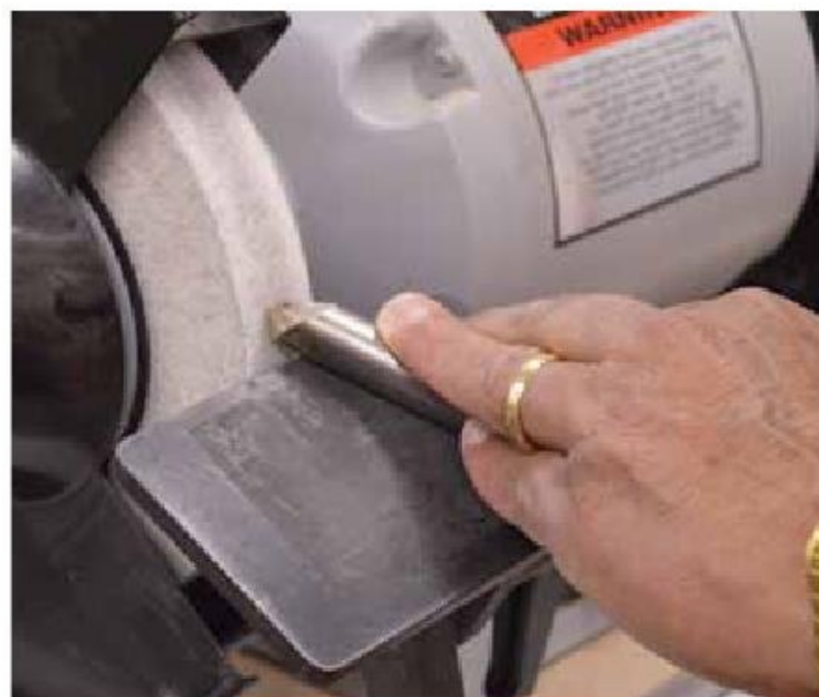
15. Start the sharpening by rotating the tool and sweeping to the right.
