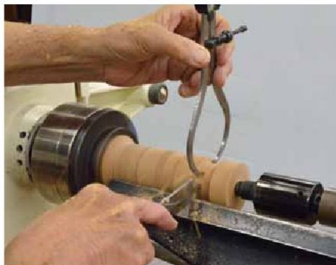
25. Reduce the waste wood between the rings to one inch.
