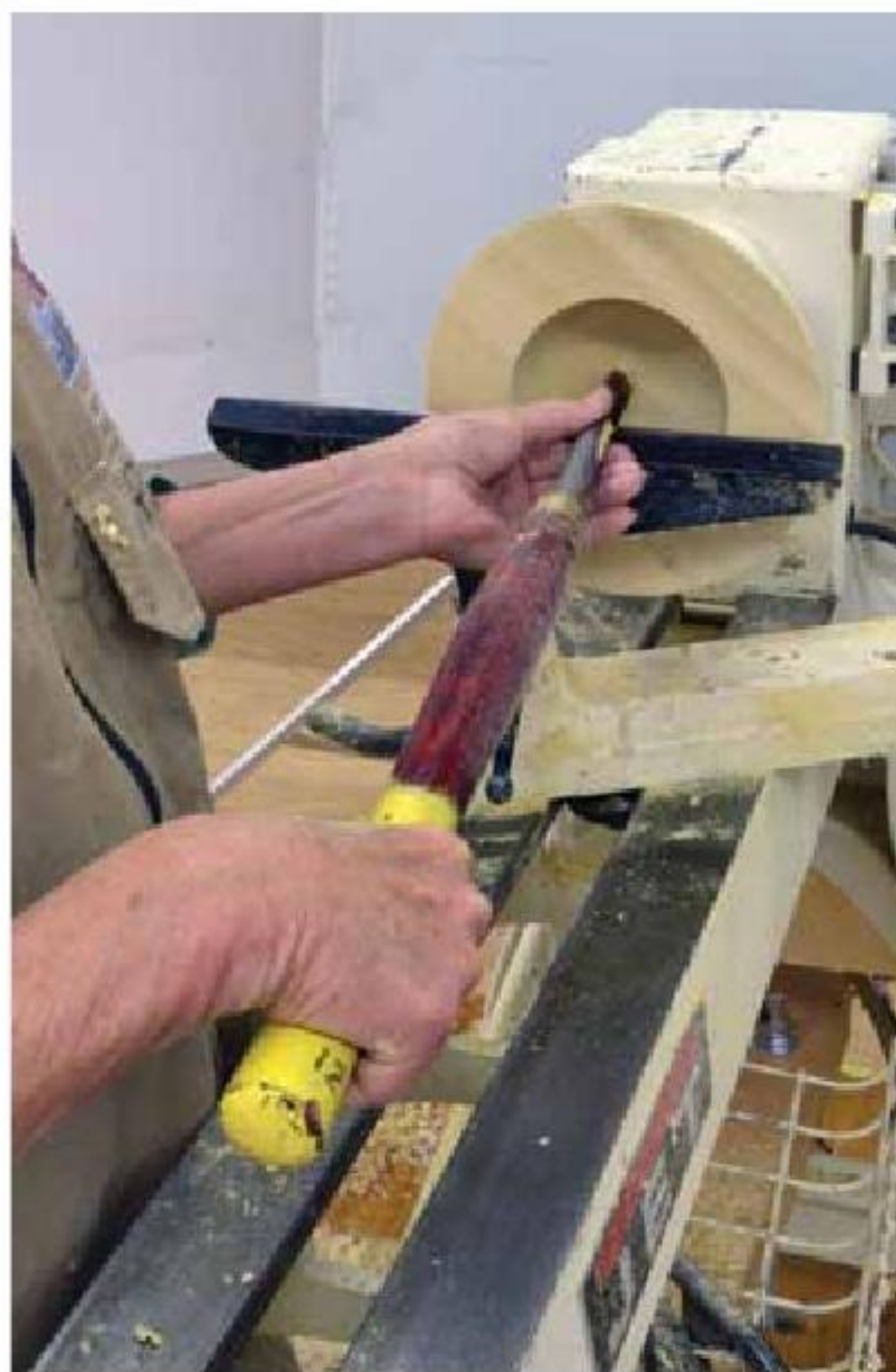
11. Phase III—Left Hand Push: With the right hand parallel to the lathe, the left hand pushes forward.
