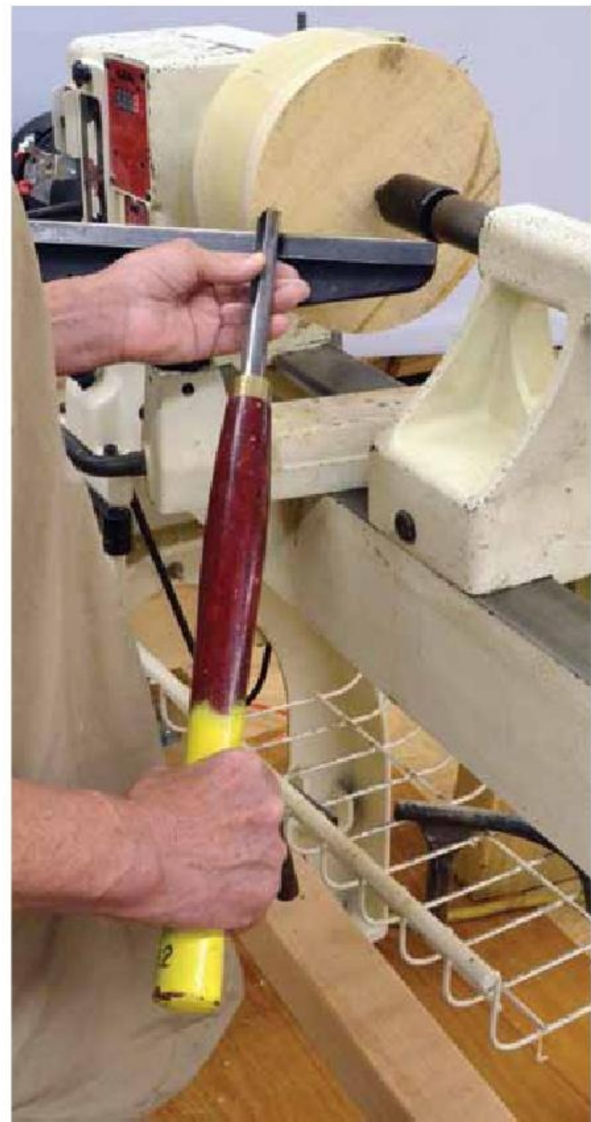
2. Mounting the blank on a screw chuck is a good starting position.
