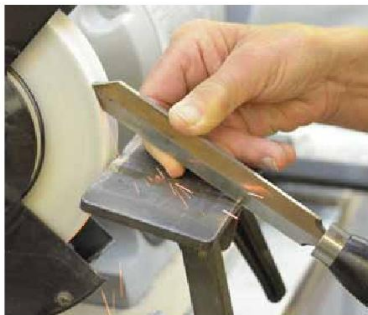
19. Parting tools start with the heel of the bevel against the wheel then raise the handle.
