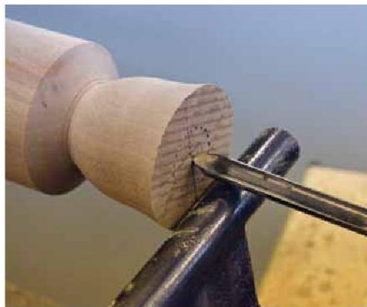
3. You are ready to drill with the shallow fluted gouge exactly at the center line.
