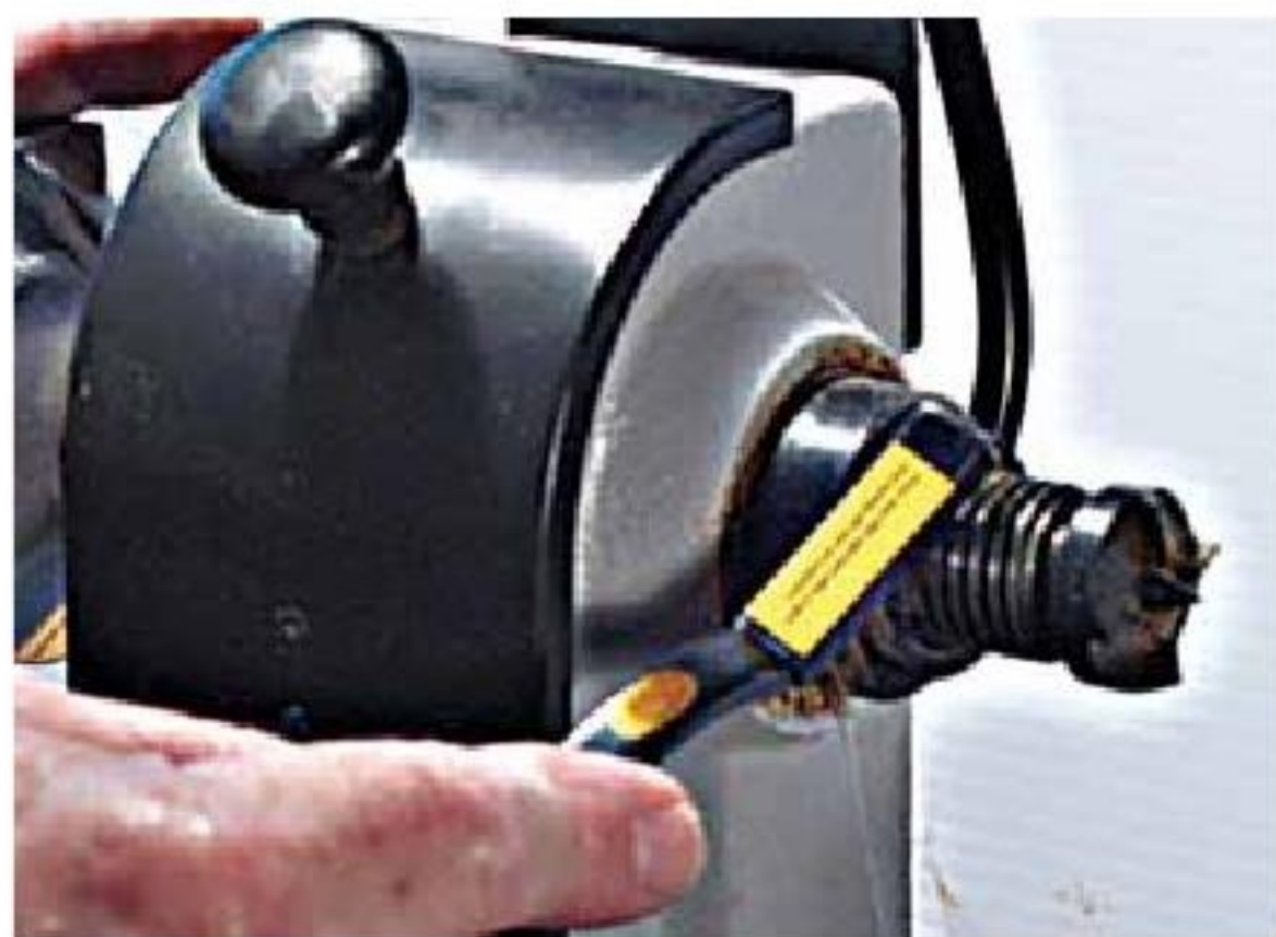
3. The headstock threads should be cleaned with a soft brush.
