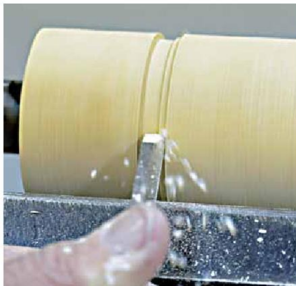
9. Parting tool cuts always overlap for safety.
