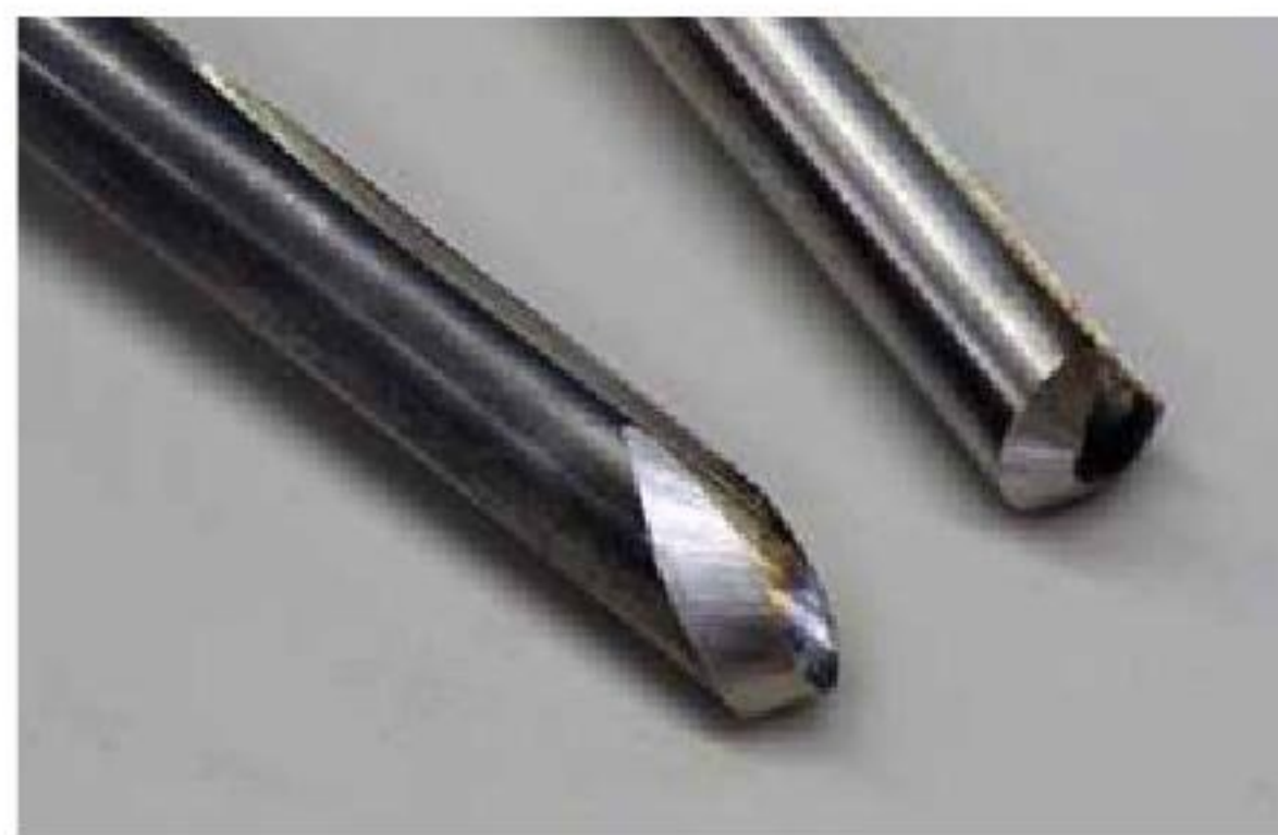
2. Sweptback and traditional grind bowl gouges are both useful in bowl turning.
