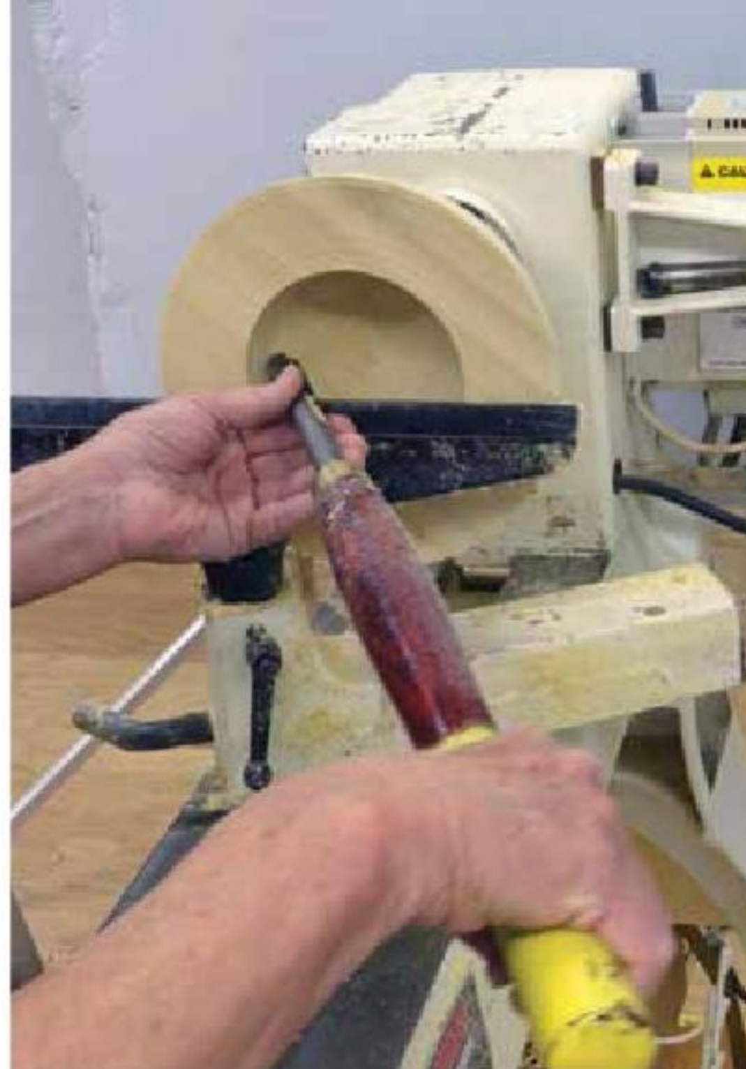
10. Phase II—Right Hand Pivot: The right hand comes forward while the wrist unrolls.
