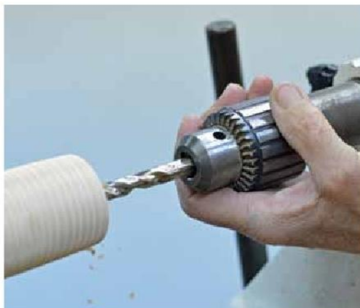
11. A Jacob’s chuck with the correct drill easily centers the hole for the screwdriver shaft.
