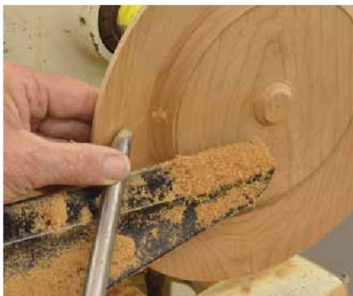
10. Shape the interior of the rim and slightly start to cut the bowl.
