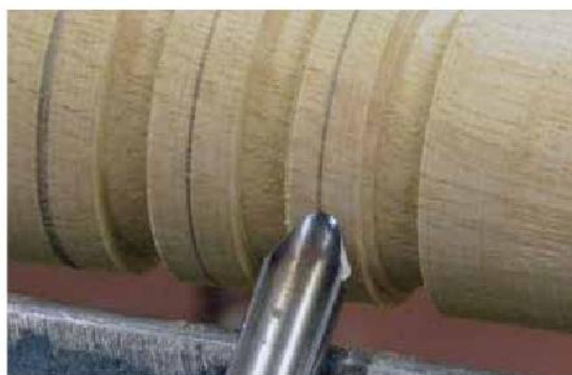
17. Practice cutting beads, trying not to eliminate the pencil line until the last cut.
