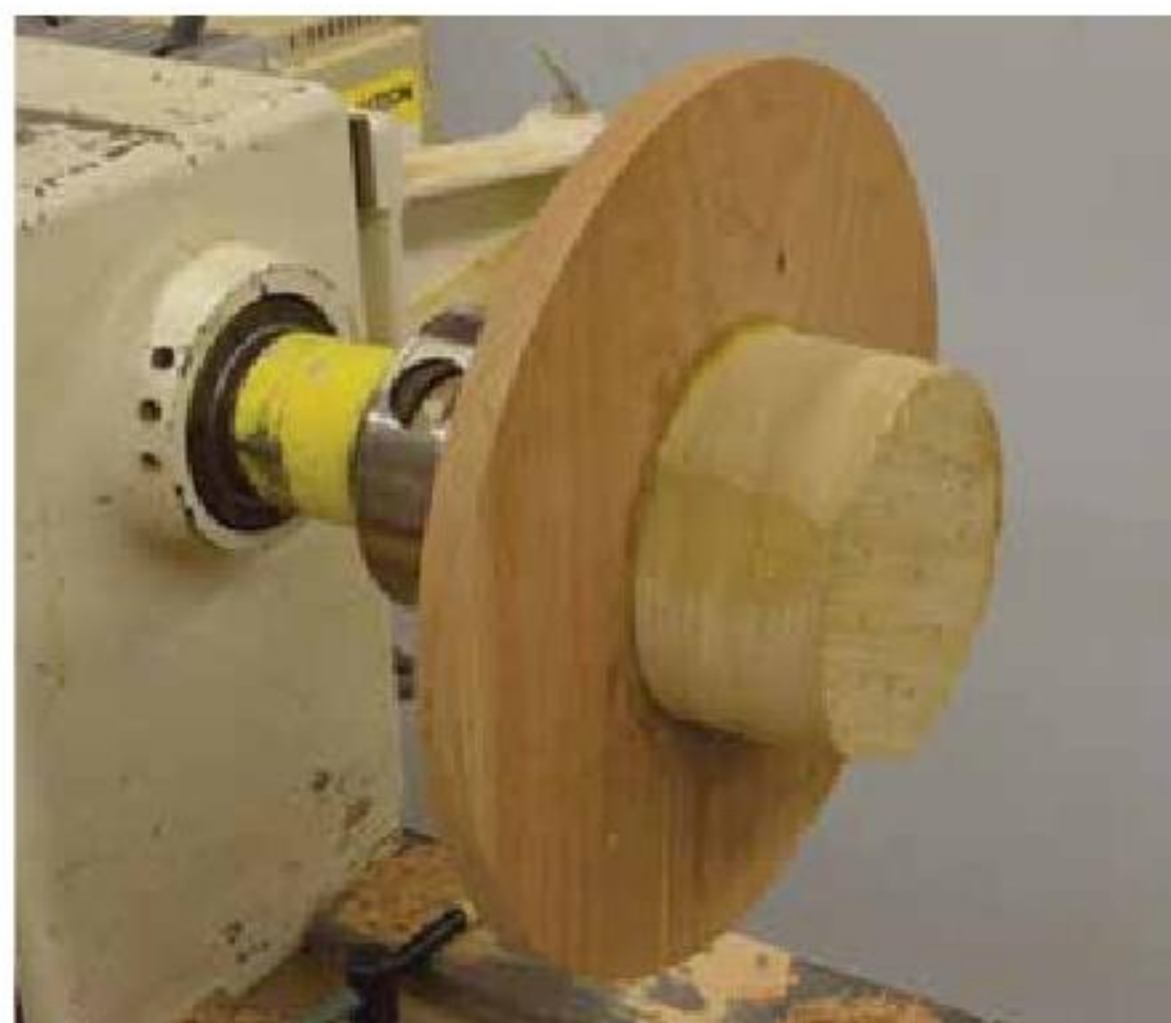
8. Chuck the platter in the expanding jaws after removing the faceplate.
