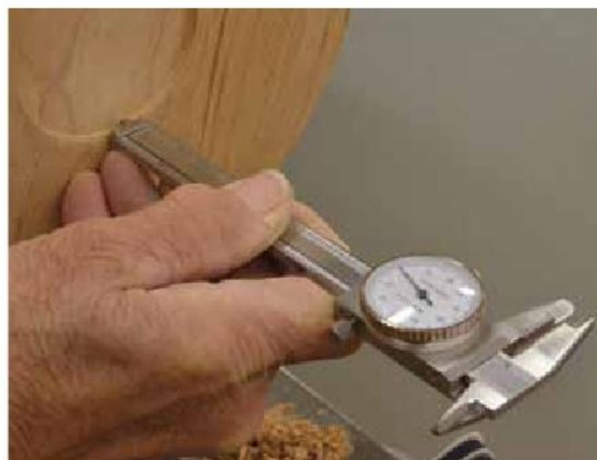
6. Be sure to have an exact depth measurement of the recess for the expanding jaws.
