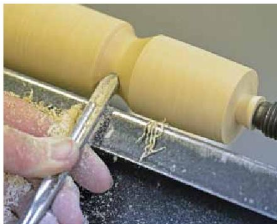
16. Complete the cove with the gouge facing upward.
