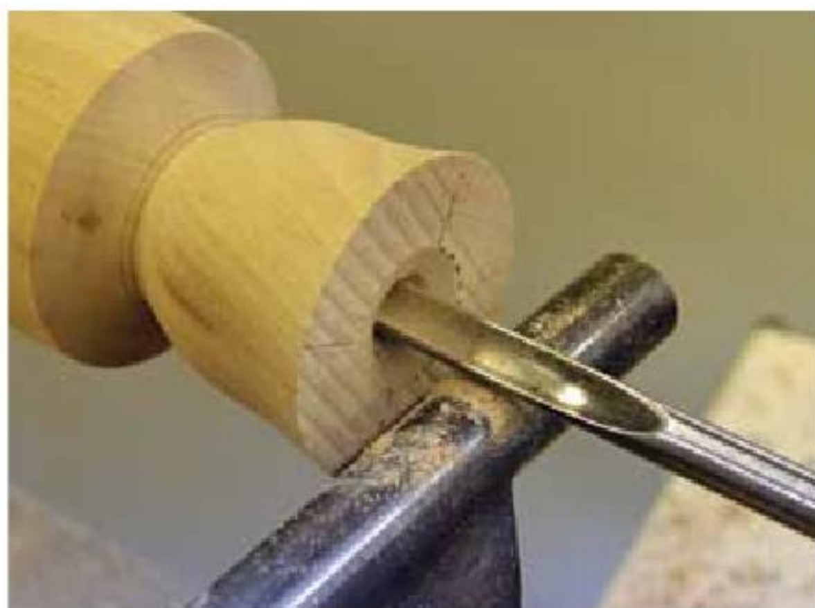
4. Drill a depth hole to about 90% of the cup's depth.
