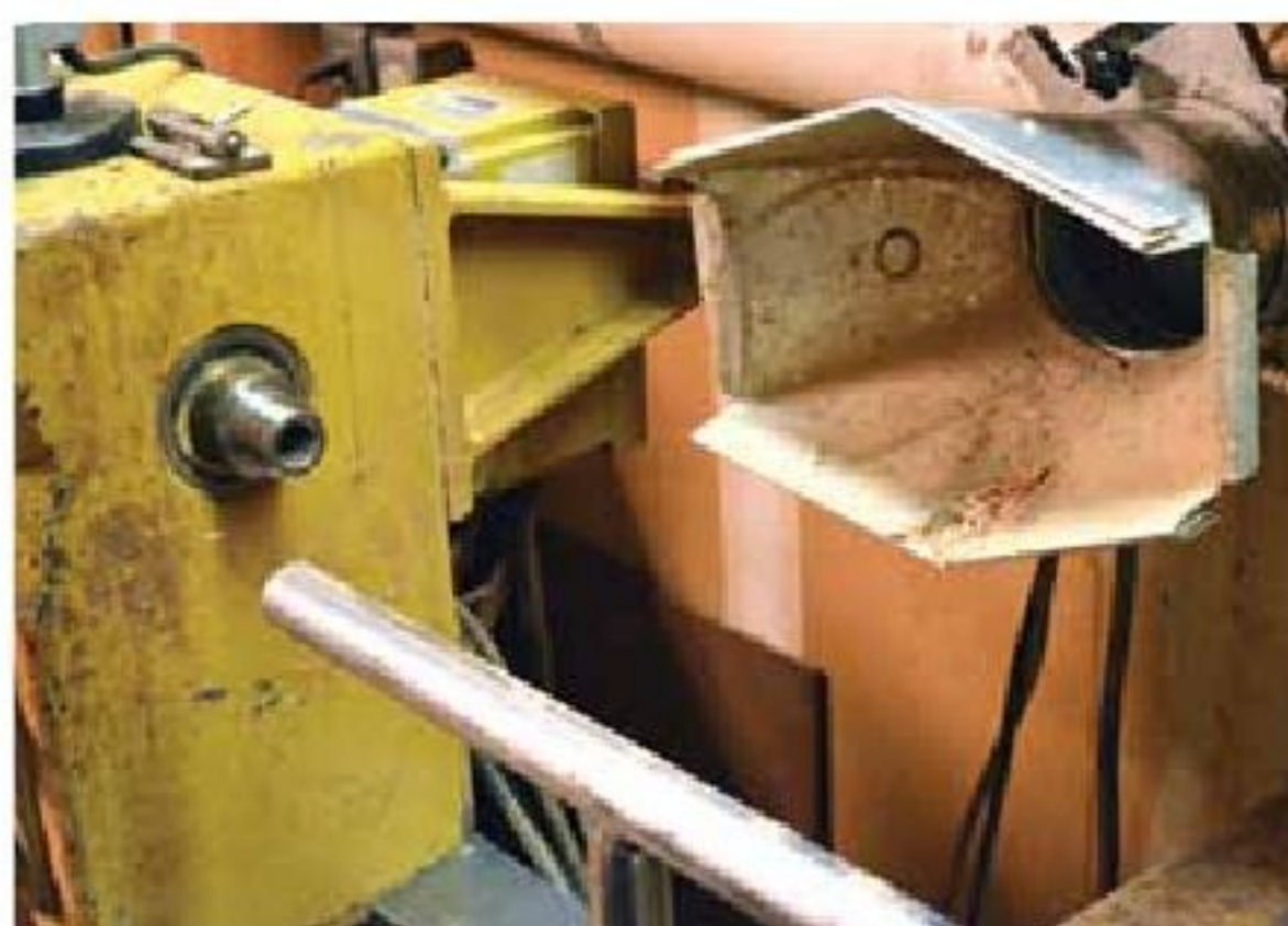
3. Set up a dust collection system at your lathe.
