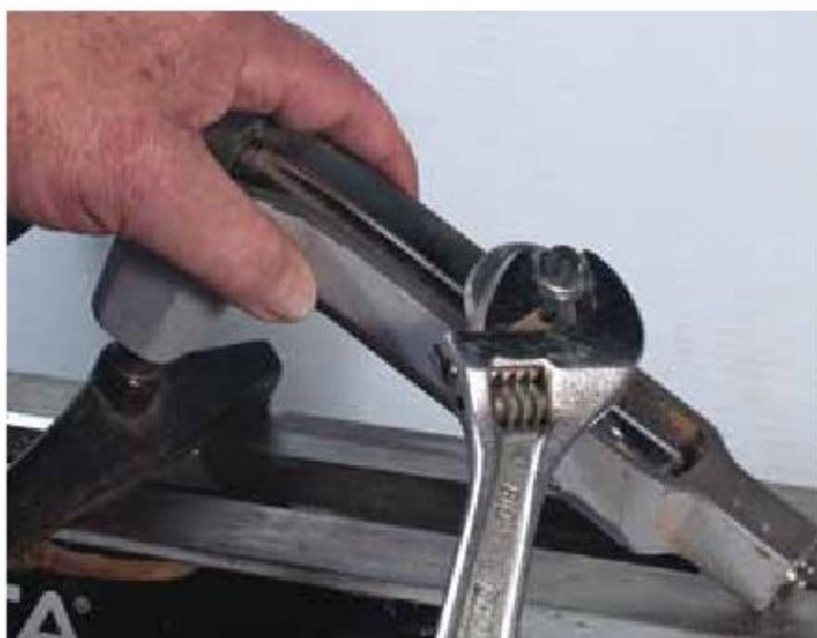
5. Adjusting the banjo may be needed periodically.
