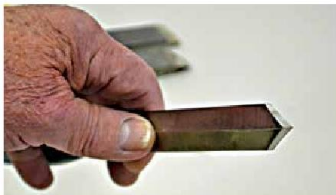
8. The diamond parting tool must keep the cutting edge in the center.
