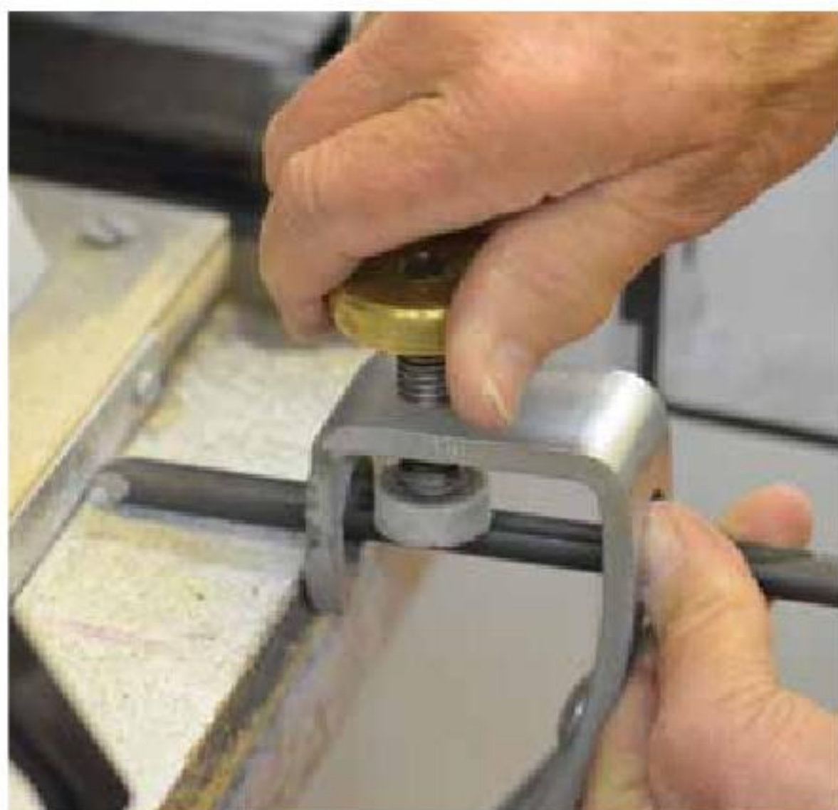
11. With a commercial fixture, set the tool projection.
