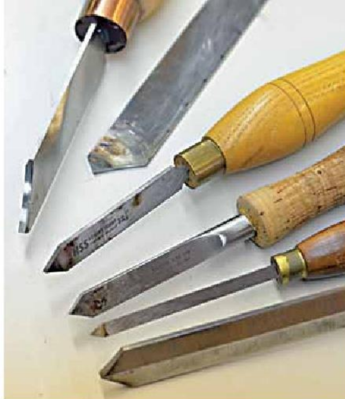
7. Parting tools come in many sizes and shapes.
