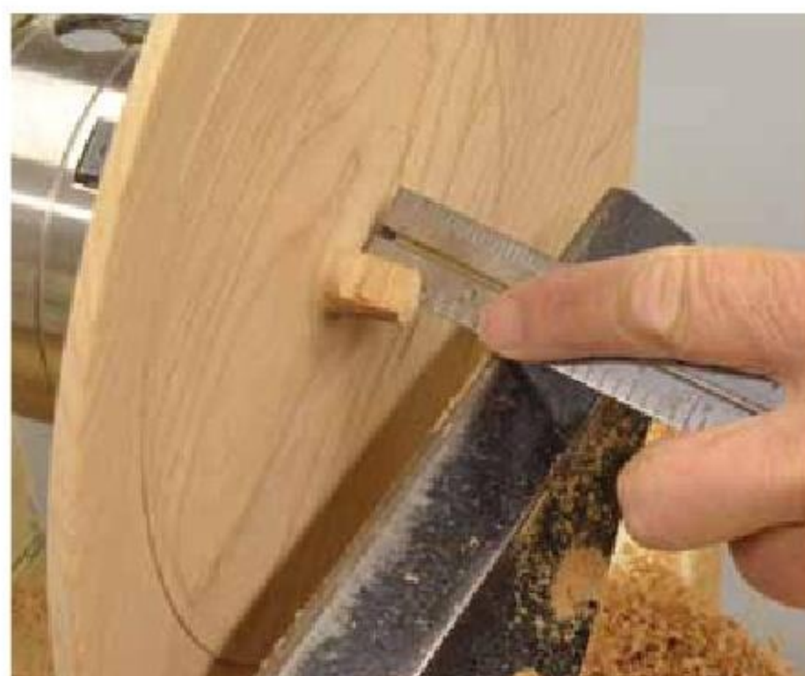
11. Shape the bowl area carefully, retaining the center for depth measurement.
