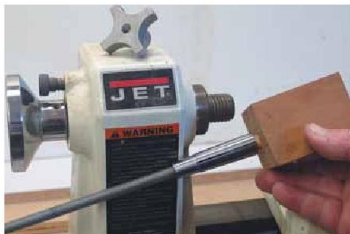
19. A blank with a dowel glued in is being inserted into the collet chuck.
