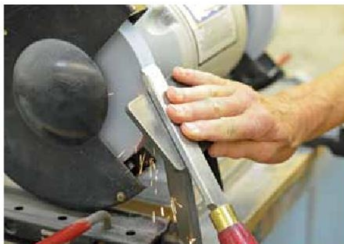
8. Hand sharpening a skew using a platform is safer.
