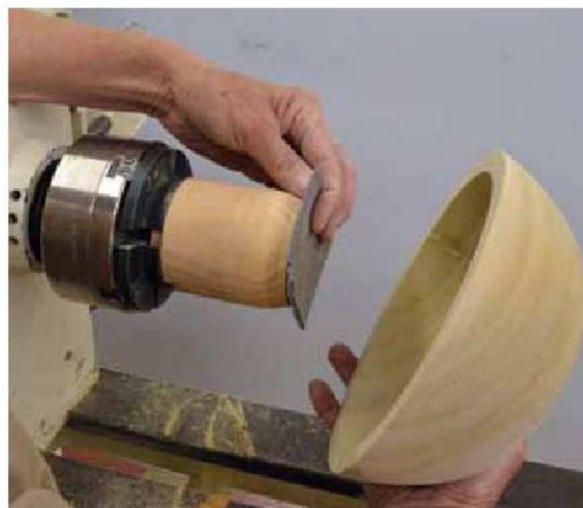
11. Set the bowl onto the jam chuck with a protecting pad.
