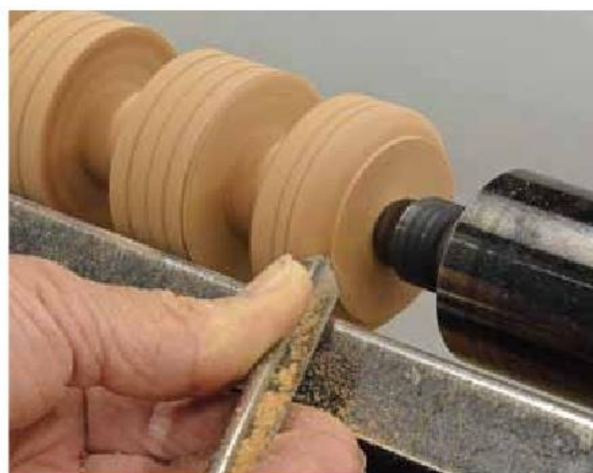
26. Note the layout lines added before beginning to shape the first ring.
