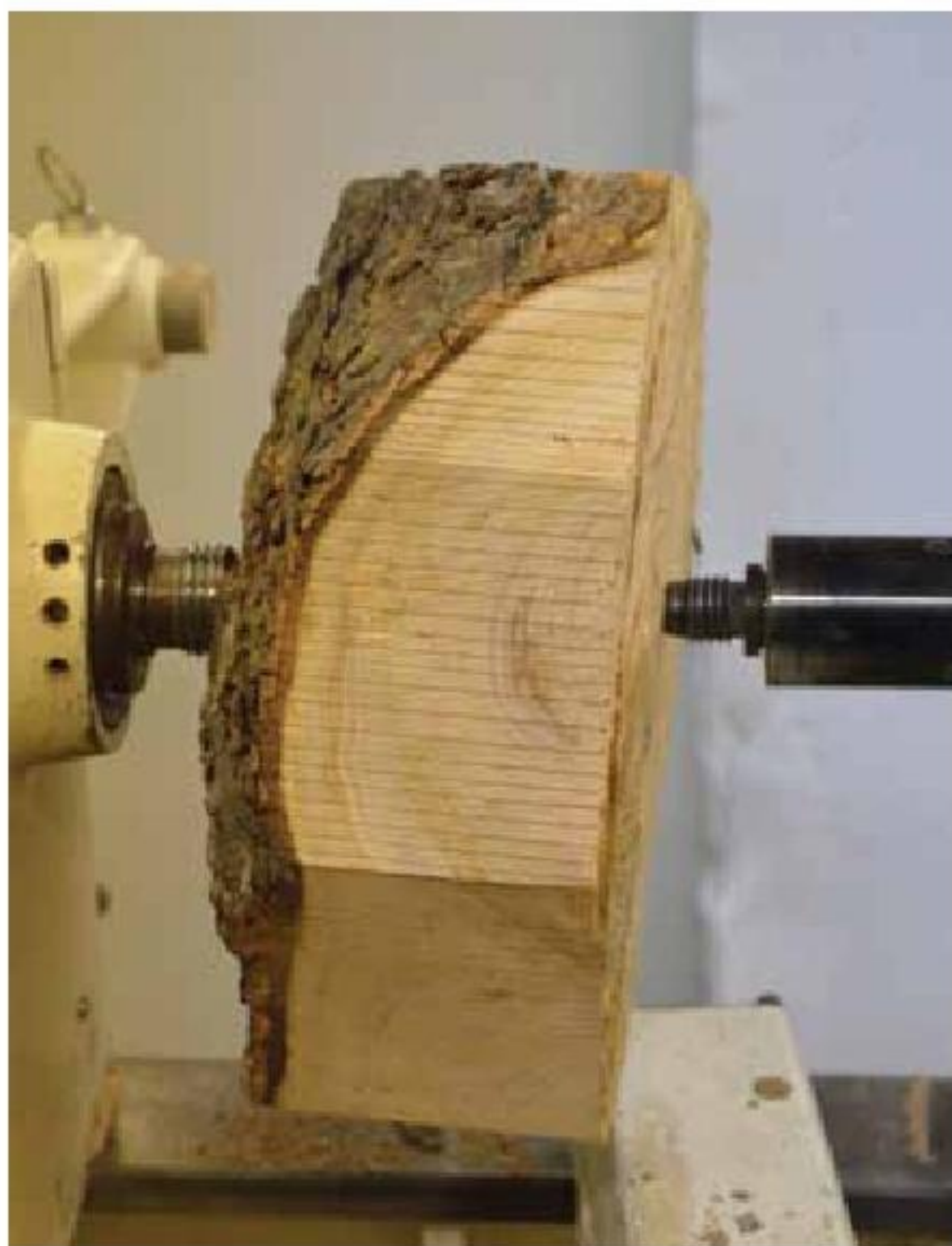
4. You may need to adjust the blank alignment to get the wings balanced.
