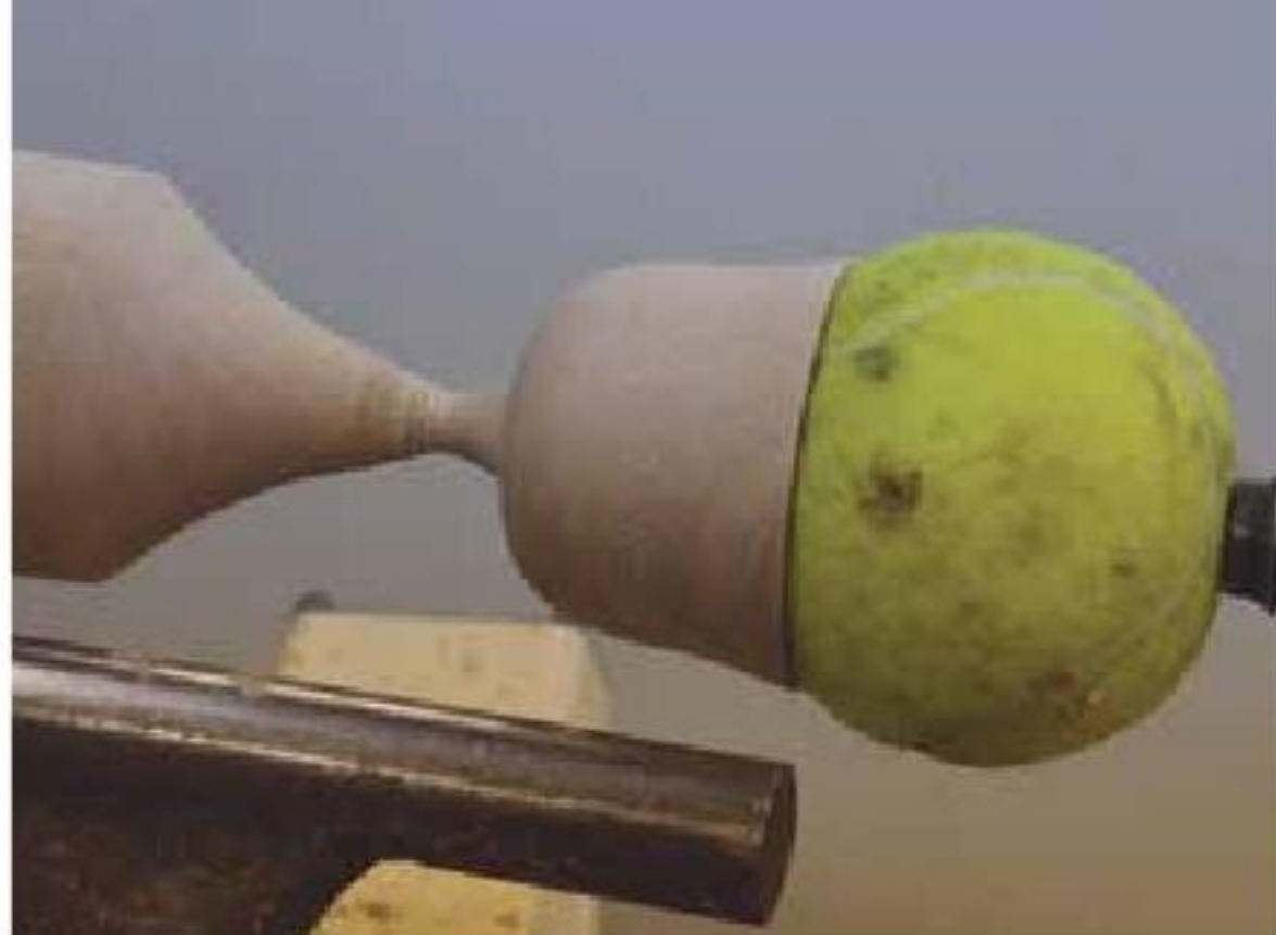
7. Support the goblet with a tennis ball.
