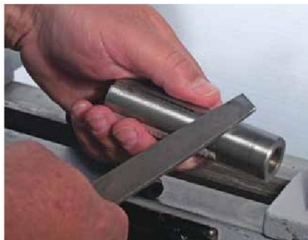
6. Filing the quill is necessary when it has been abused by improper locking.
