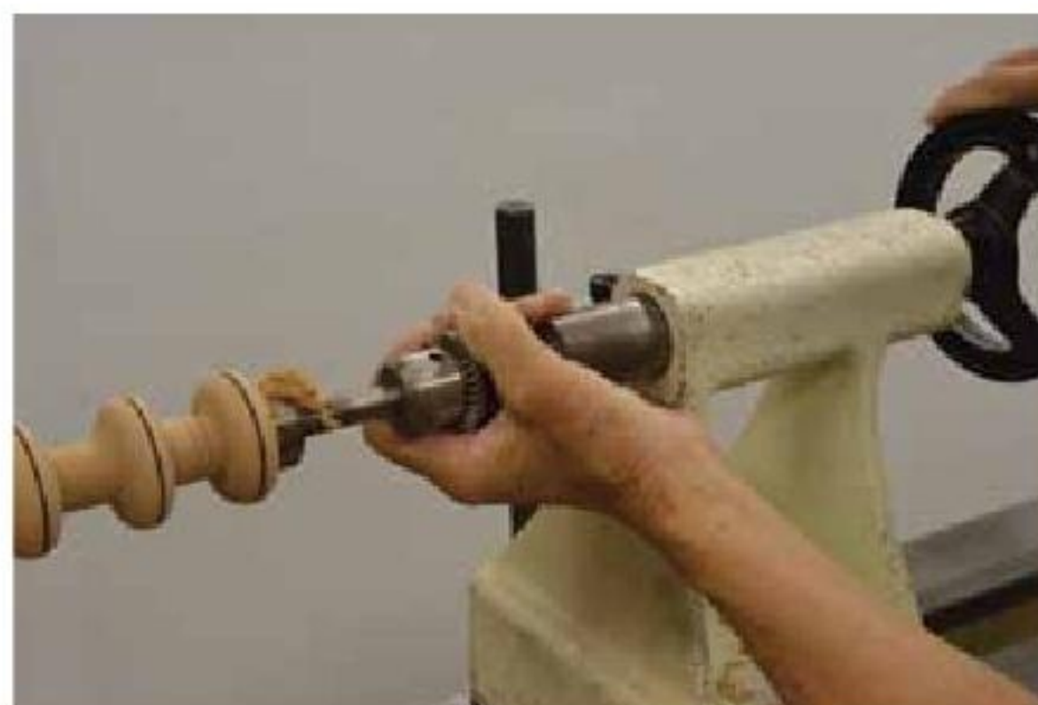
28. When drilling off the rings one at a time, use slower drilling speeds.
