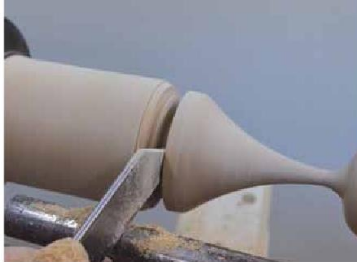
8. After completing the stem, undercut the base.
