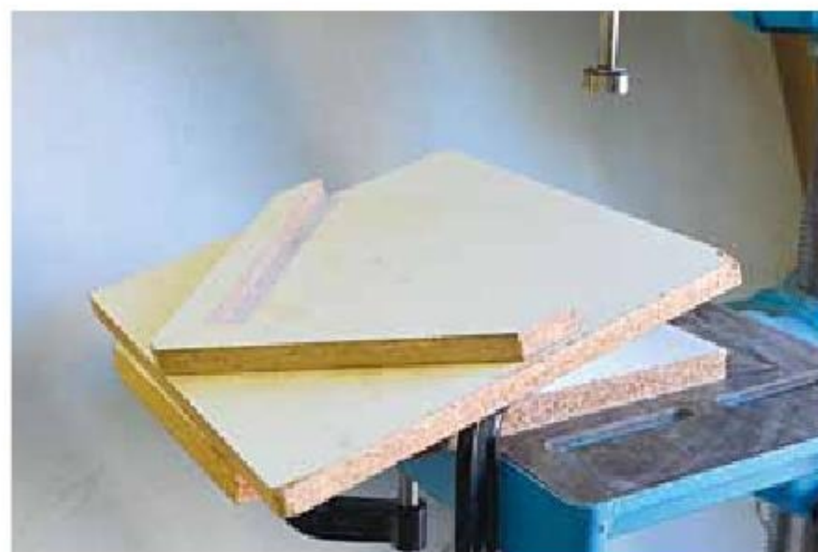
8. A leg hole drilling fixture with a table angle of 15 degrees clamped to the drill press.
