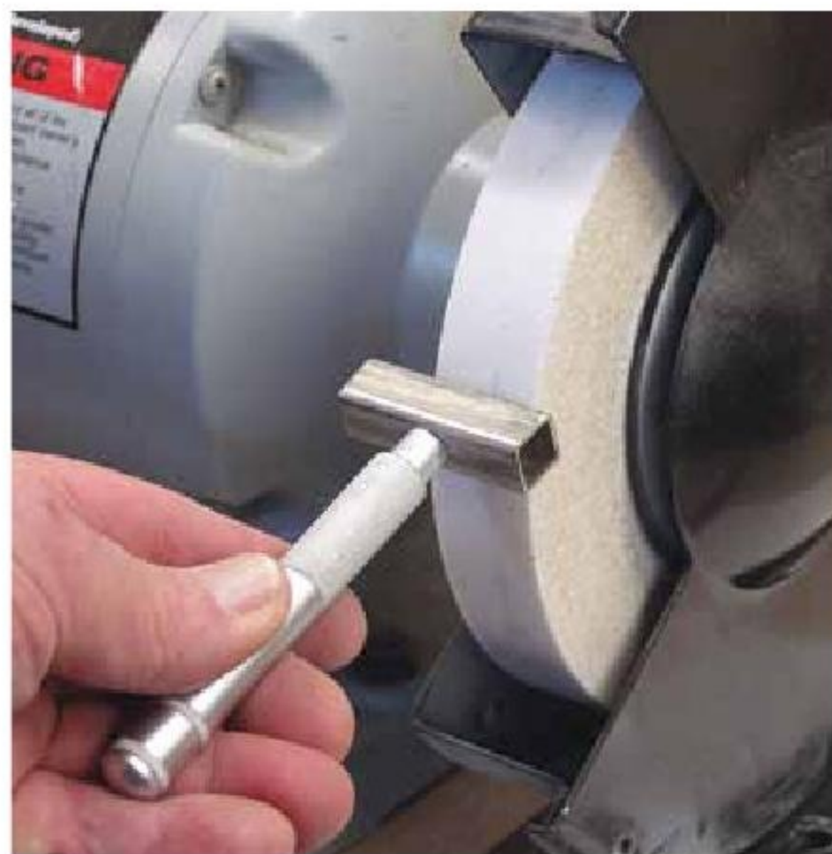
1. An inexpensive diamond wheel dresser is necessary to keep the wheels clean.
