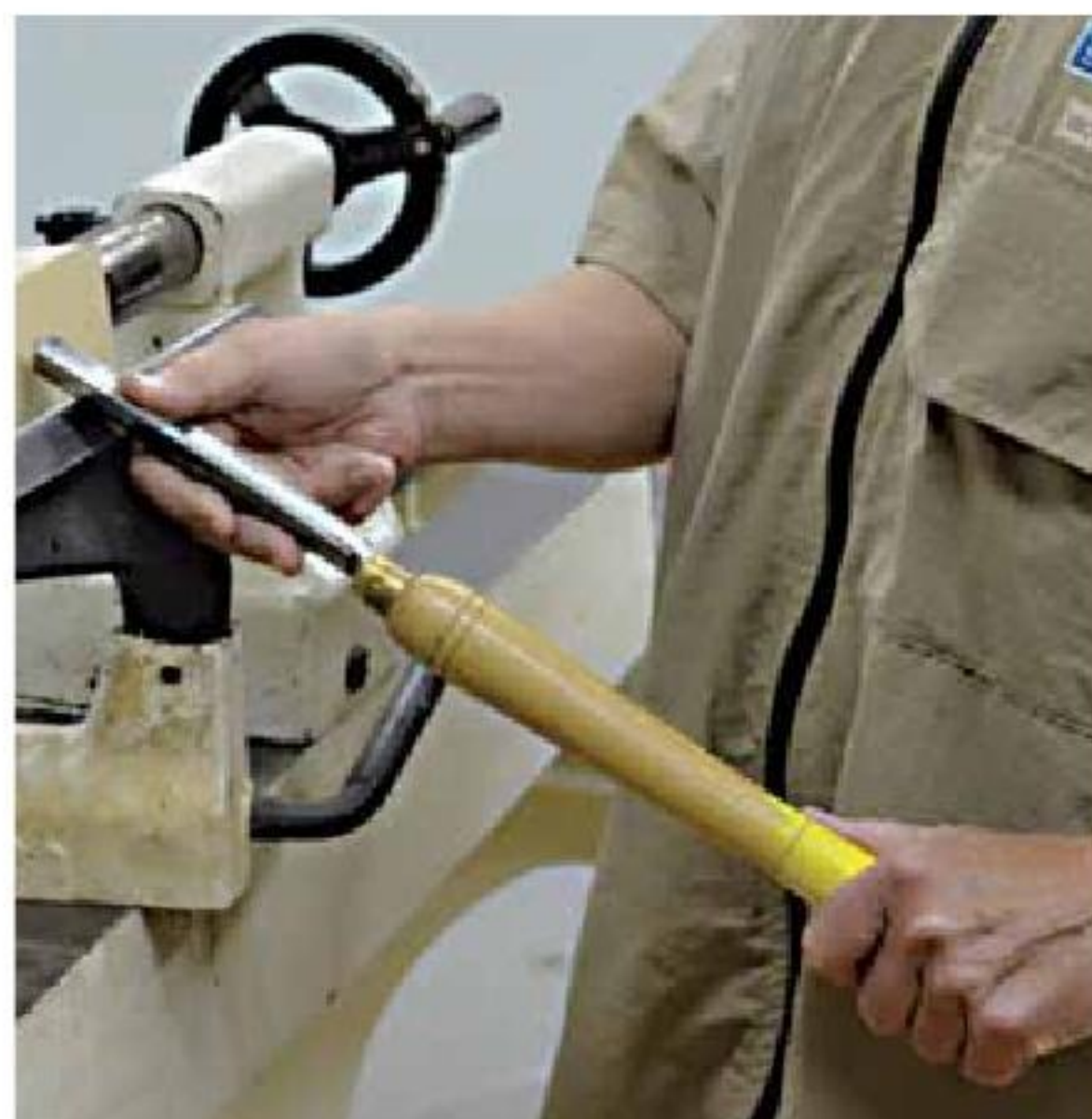
2. The SRG is ready to make a cut with the handle down and anchored.
