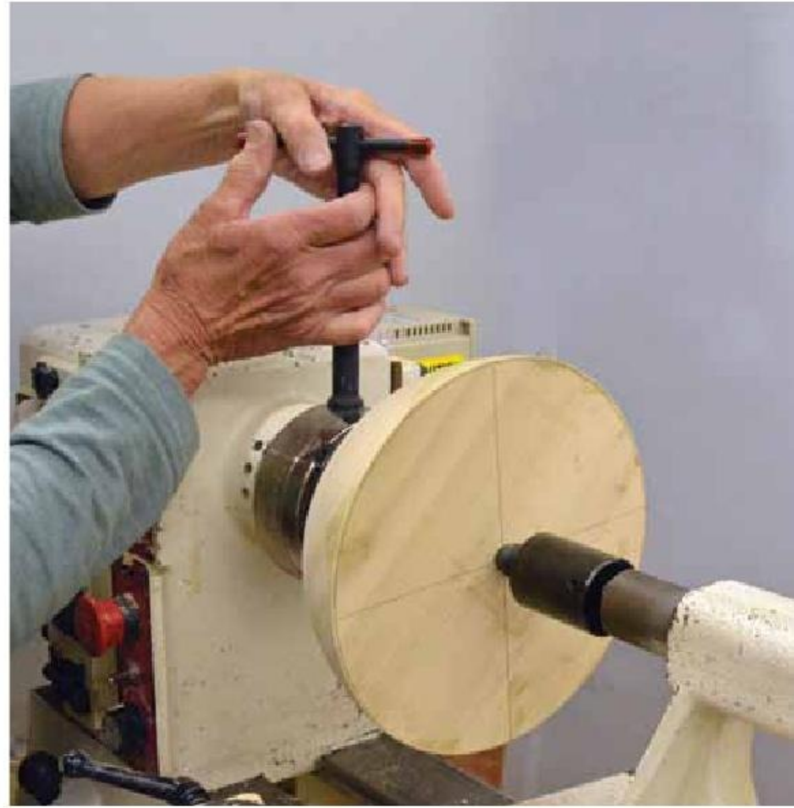
7. Mount into the chuck using the tailstock for alignment and support.
