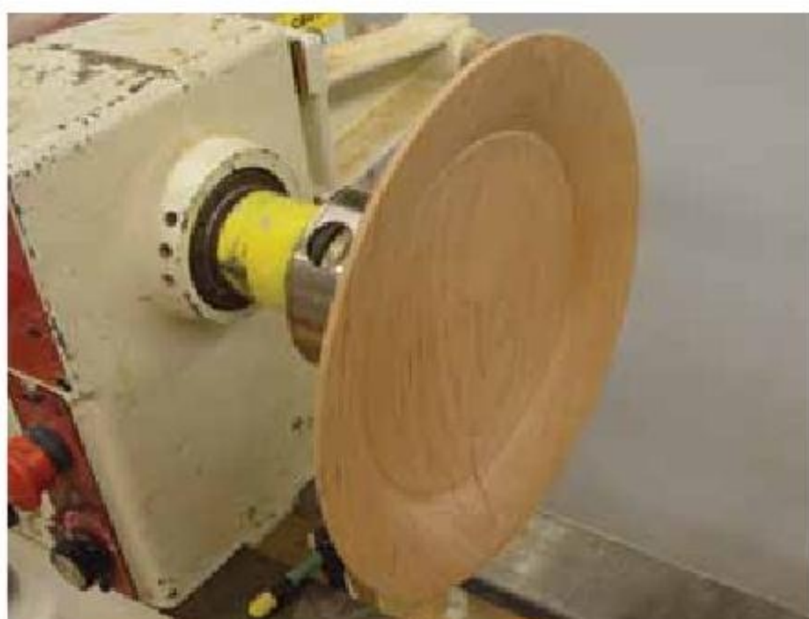
12. Complete the interior by removing any remaining ridges and sanding.
