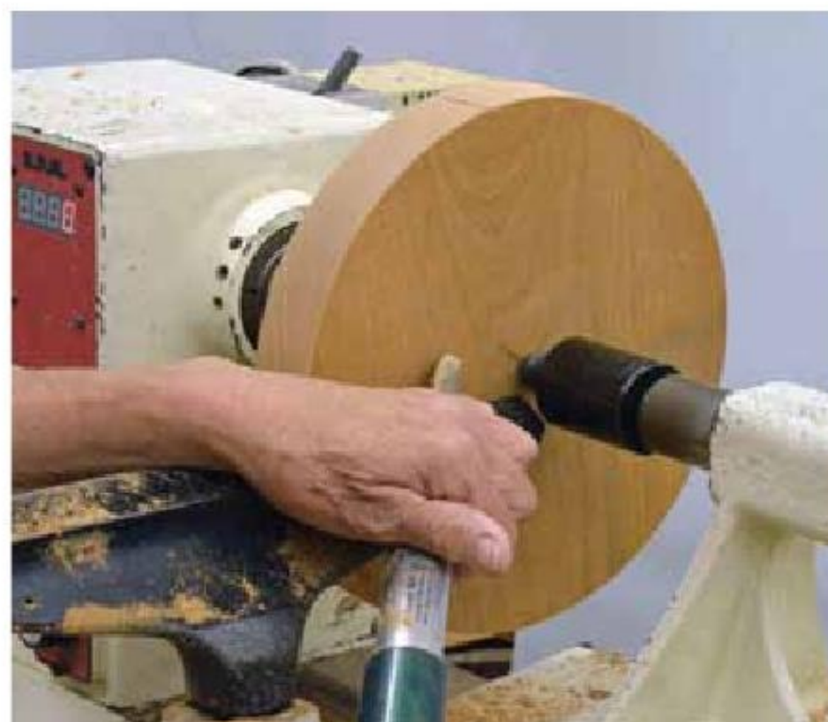
4. Flatten the face by using pull cuts, with the flute facing the turner at 45 degrees.
