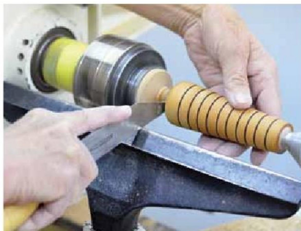
13. After completing the handle, part off carefully with a parting tool.
