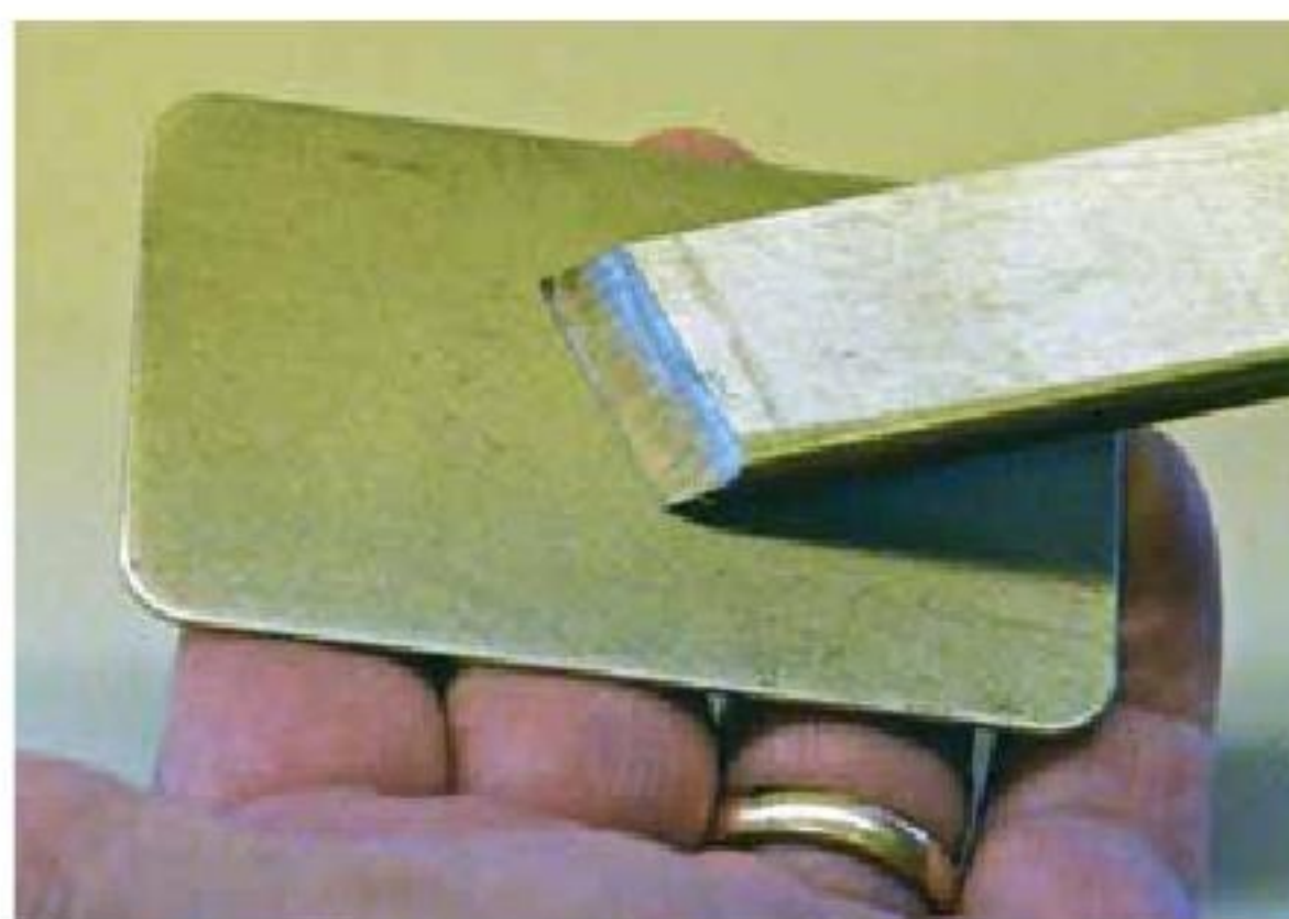
9. Honing a skew chisel after sharpening will improve the edge.
