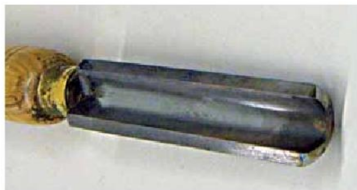
1. The spindle roughing gouge (SRG) is just for getting the spindle round.
