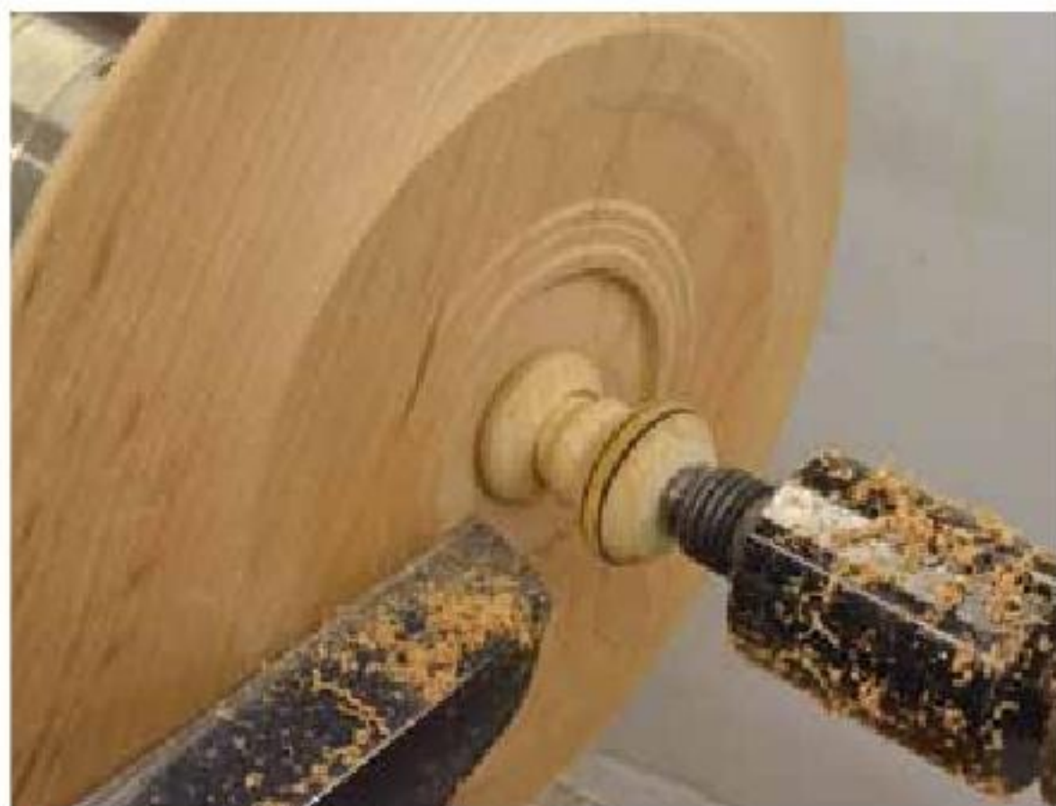
14. Support the base with a protector on the live center point.
