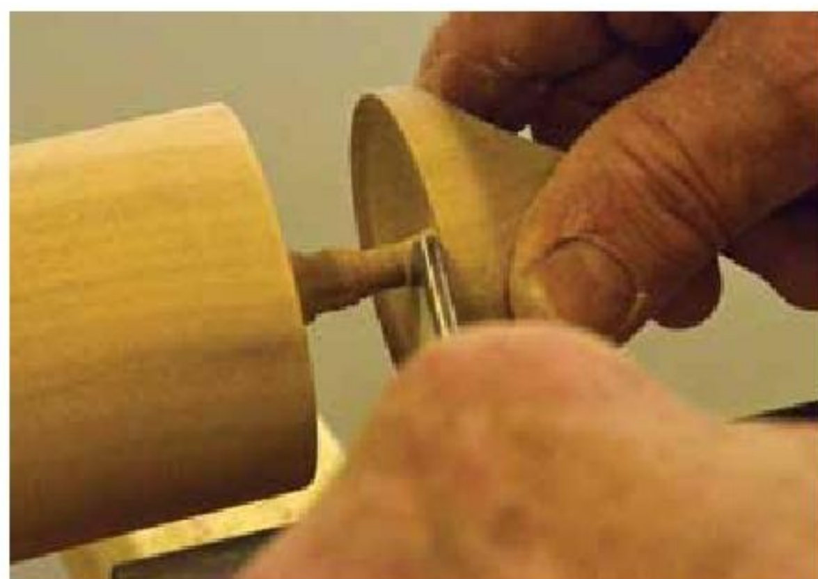
9. Part off with a smooth cut to reduce the amount of sanding.
