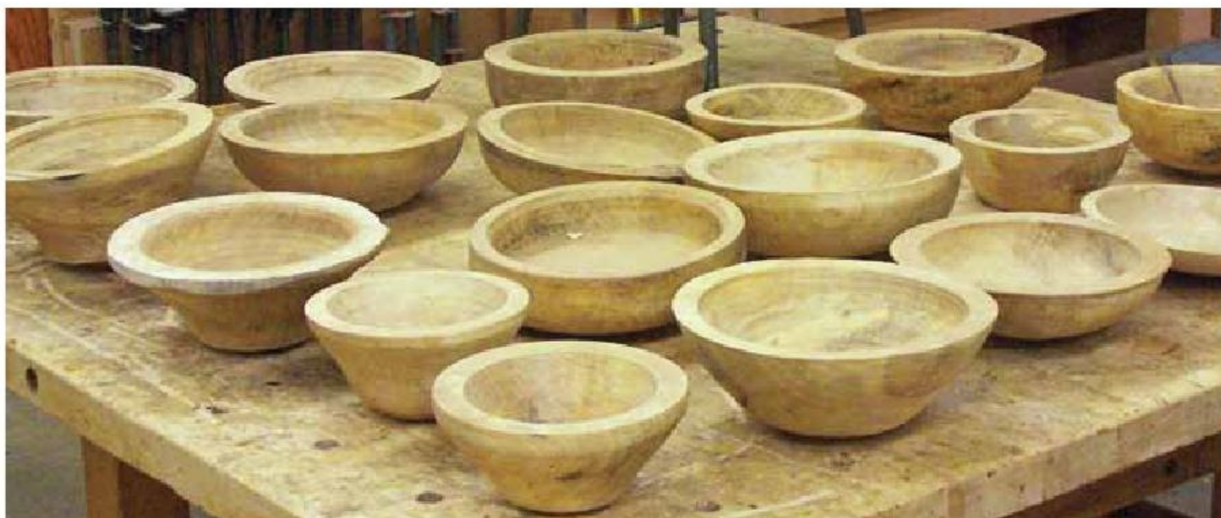
9. Seal and store rough bowl blanks until dry.
