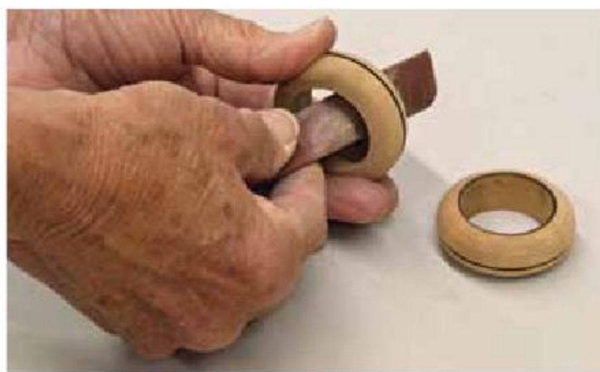
30. Clean up the interior by hand sanding.
