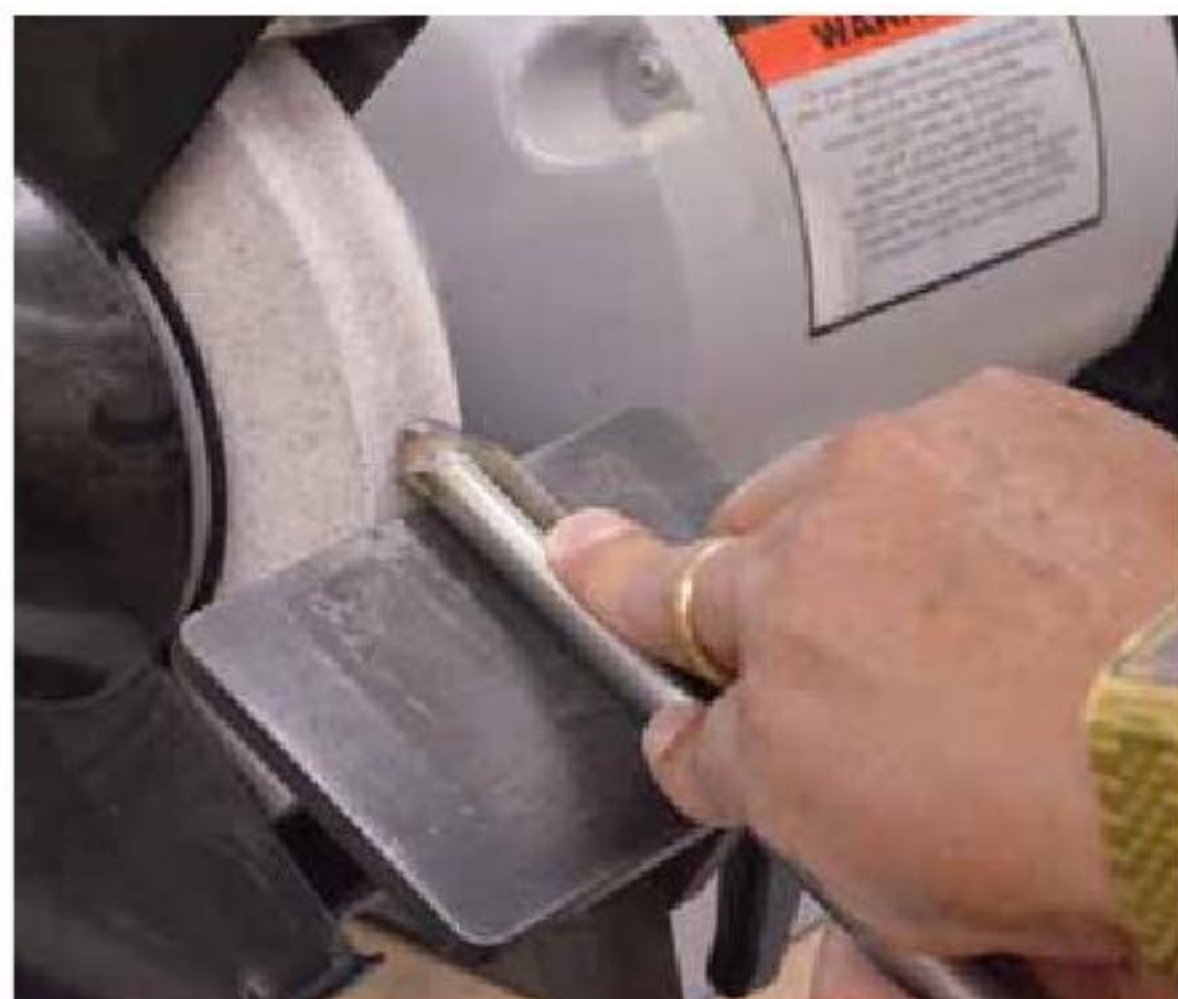
14. Adjust the platform to match the gouge bevel angle.
