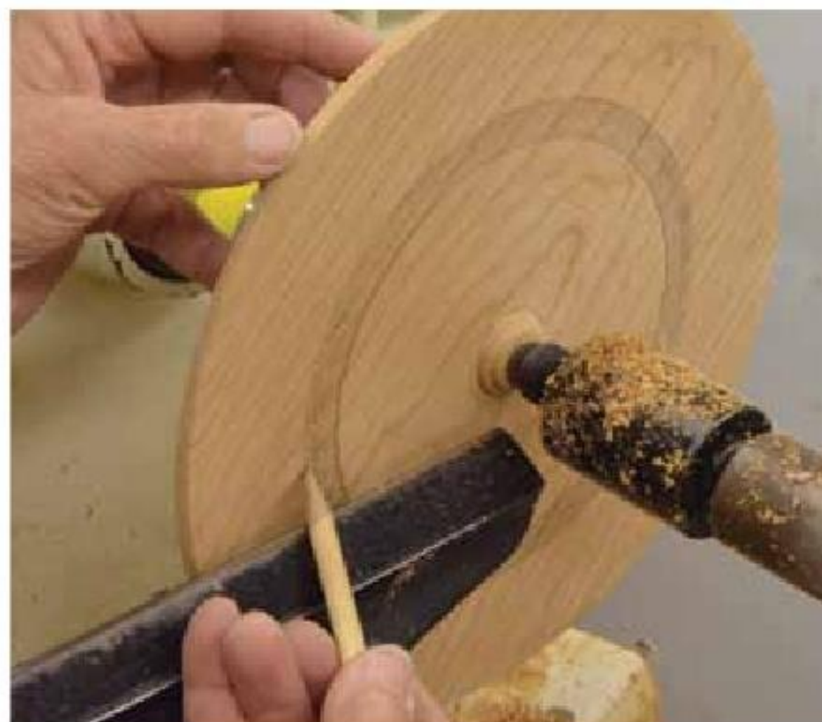
9. Layout the platter rim on the face to align with the backside.
