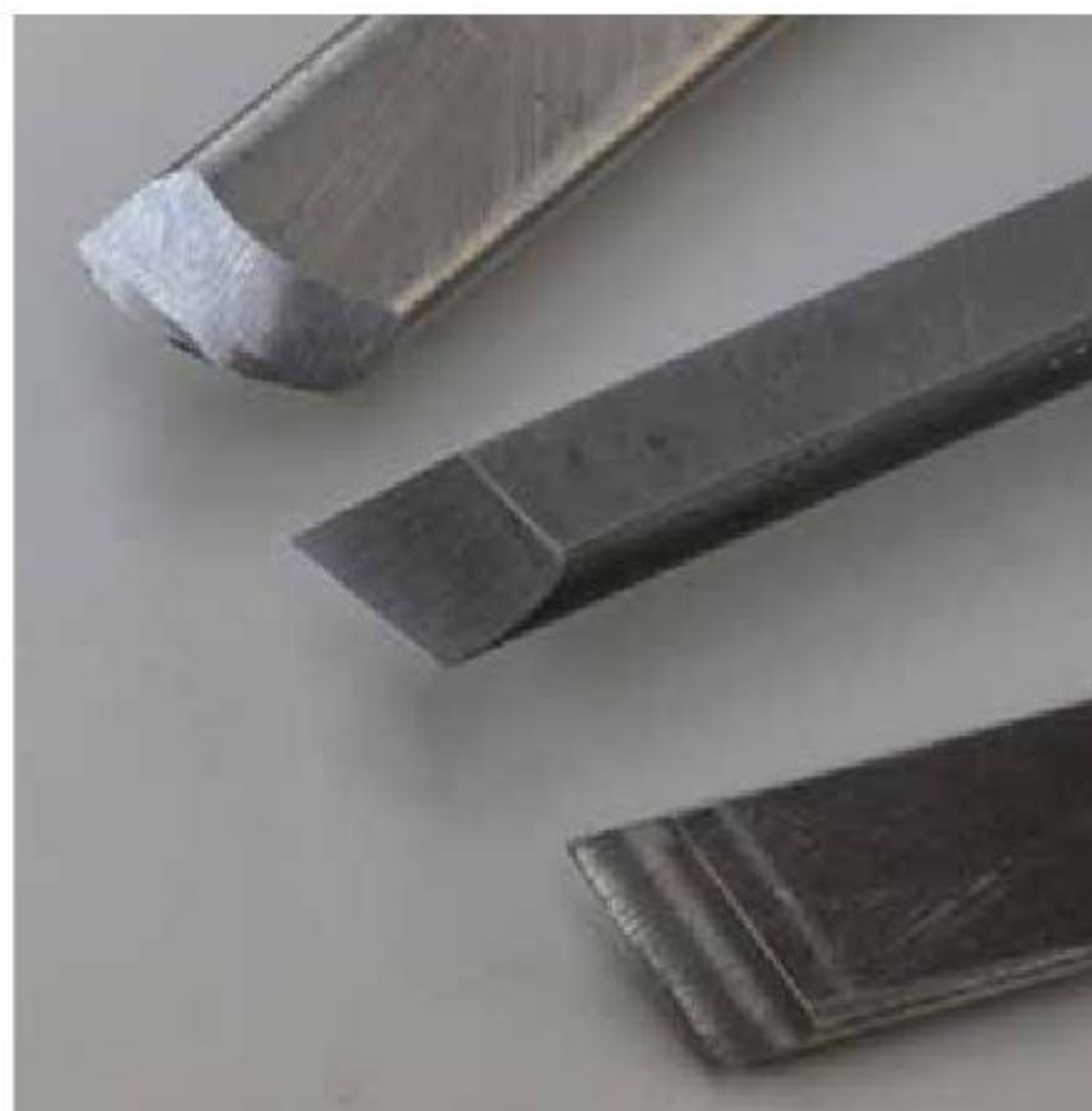
3. Here are three typical skew chisels, one with a radiused edge.
