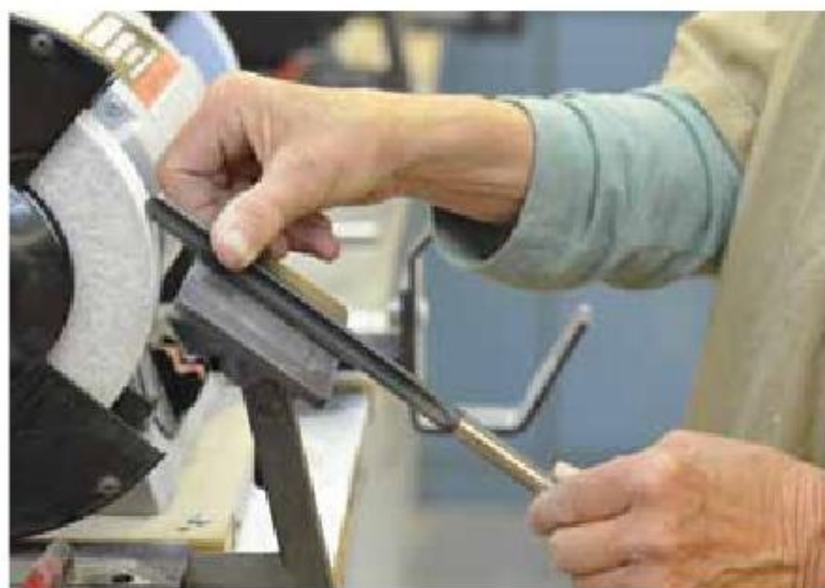
10. Sharpen a conventional grind gouge by rotating it against the wheel.
