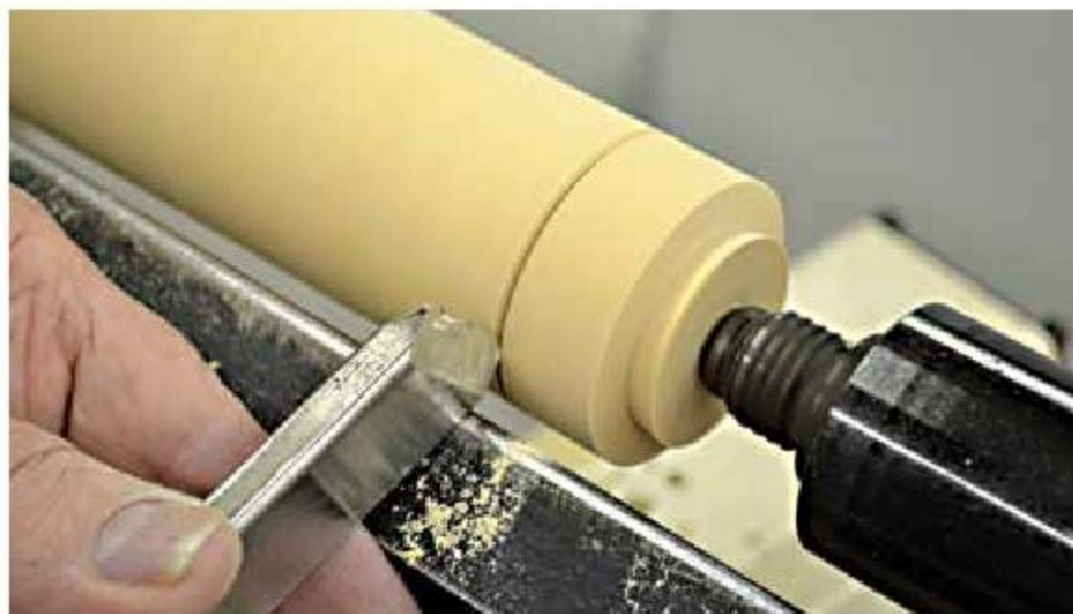
6. “V” cuts start with the long point down and the skew standing on its flat edge.
