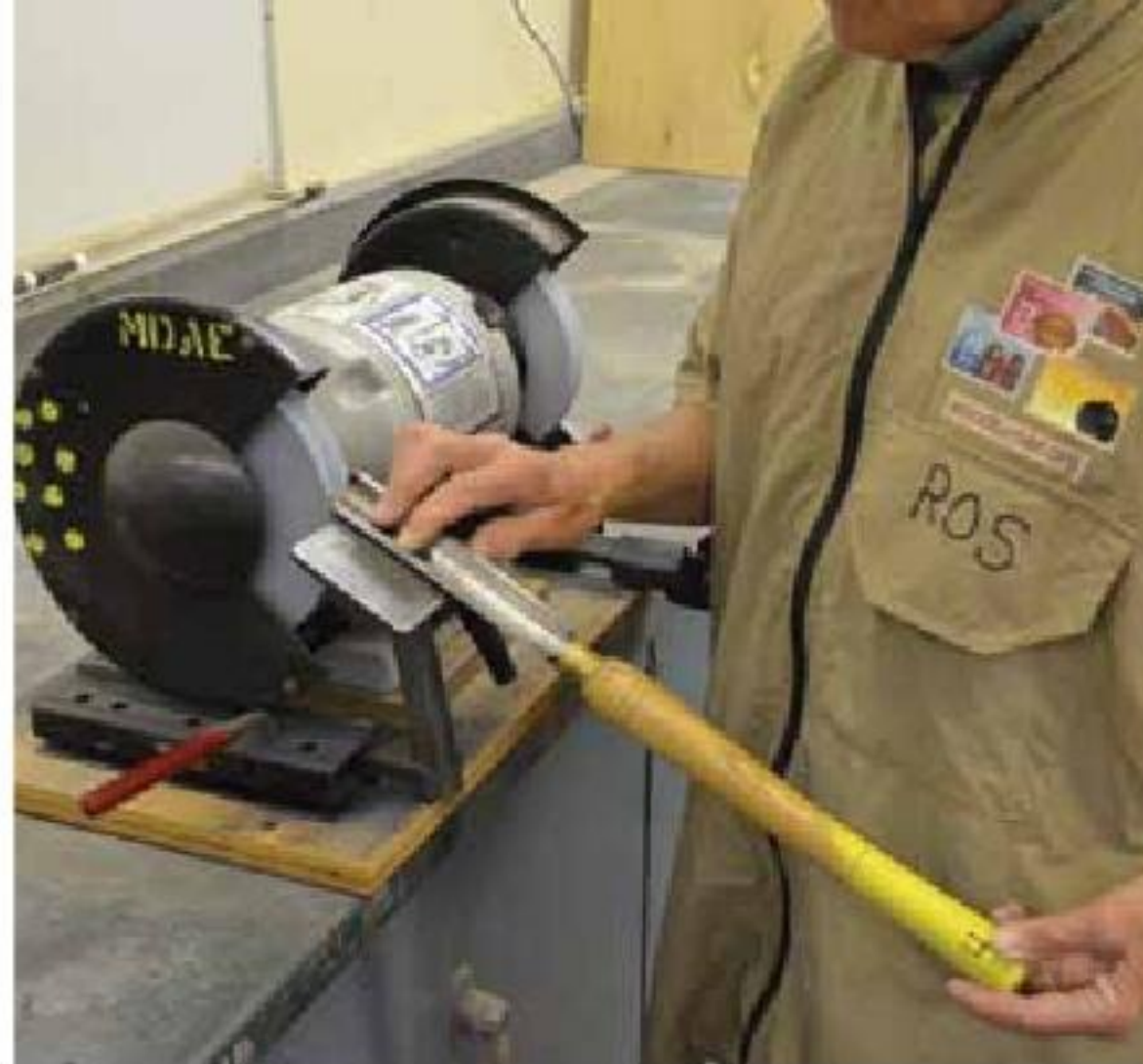
6. A safer method is to hand sharpen the SRG.
