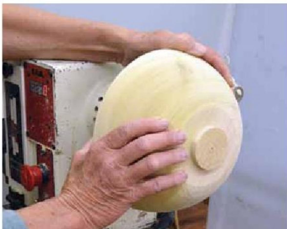
5. Square up a tenon with the parting tool.
