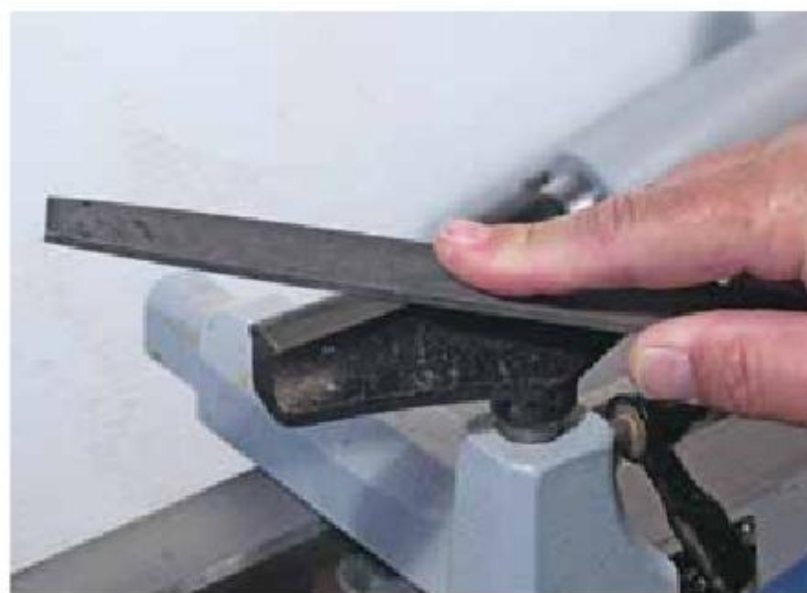
4. Filing the tool rest removes accumulated nicks and gouges.
