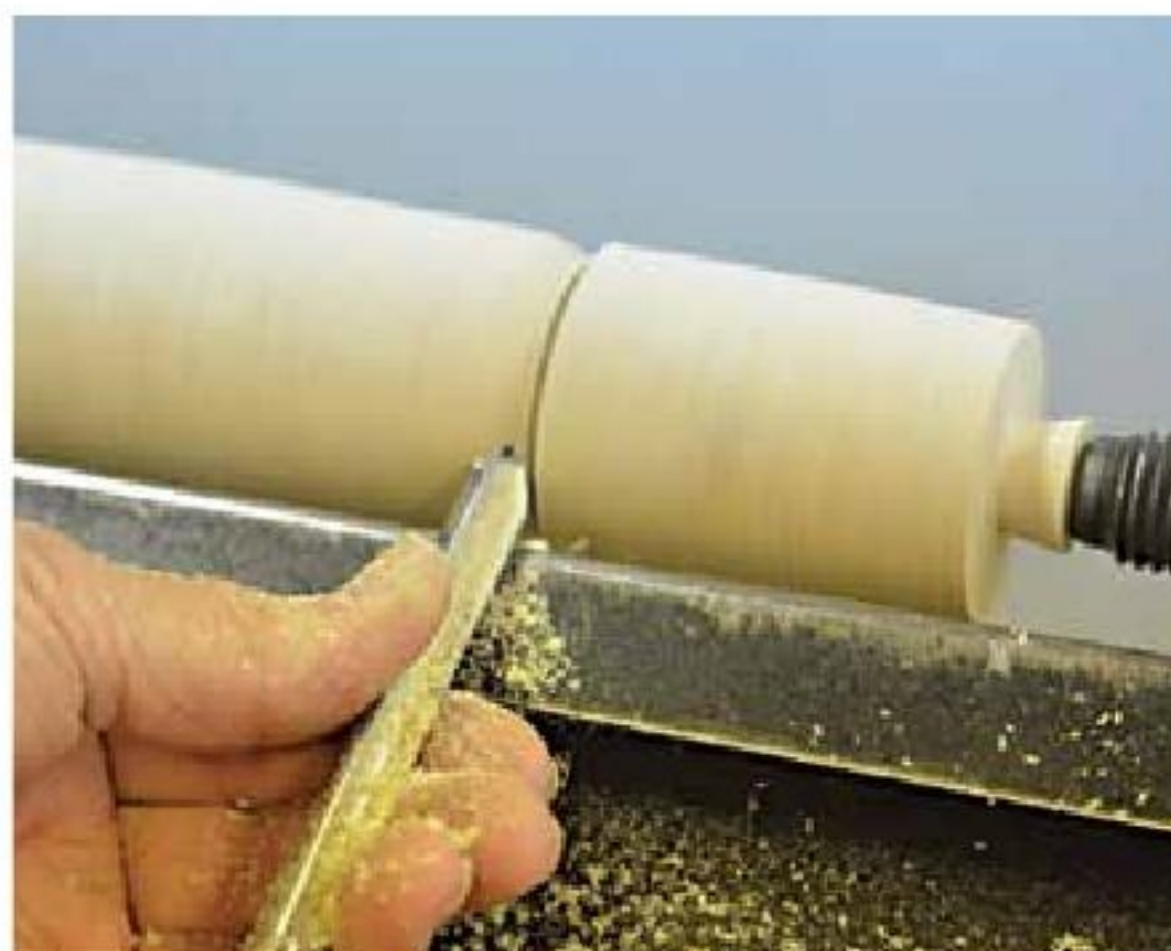
13. As the right hand bead continues, the tool rolls over to the right.
