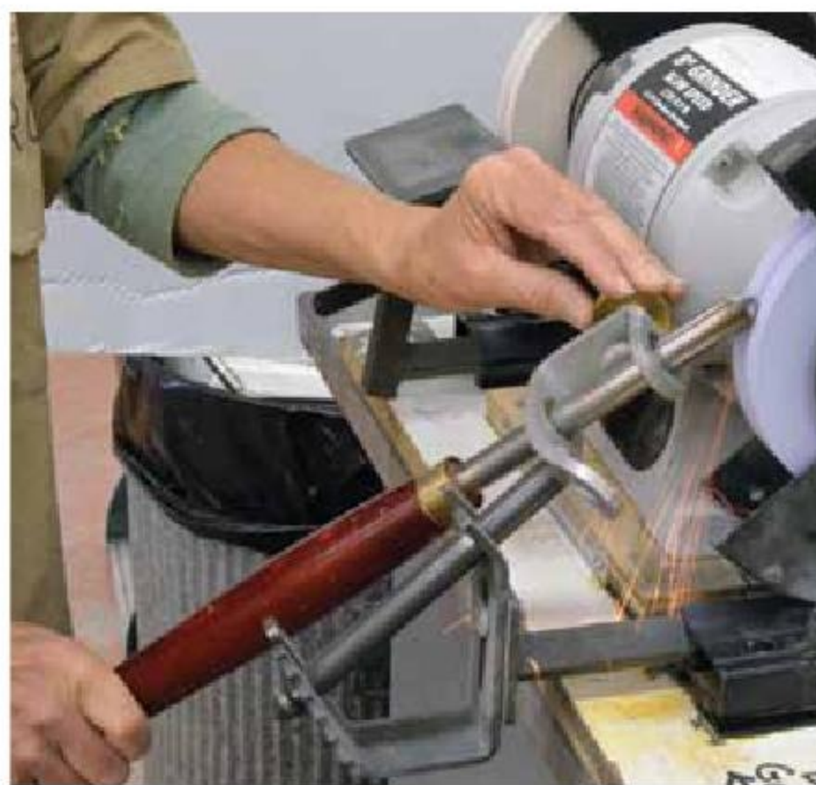
13. Sharpen the opposite side by sweeping in the opposite direction with the hand is on top.
