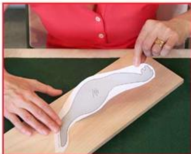
4. Attaching the pattern to the wood.
