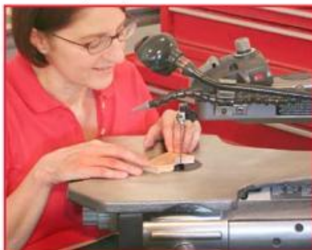
5. Sawing out parts following pattern lines.
