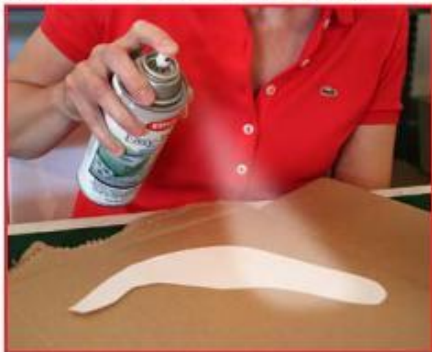
3. Applying spray adhesive to the pattern.
