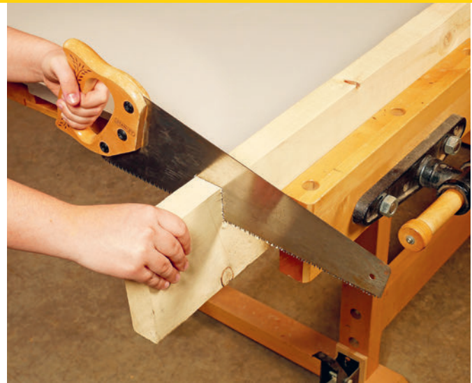
Notice that the jaws of this steel vise are lined with wood, which prevents wood damage.
