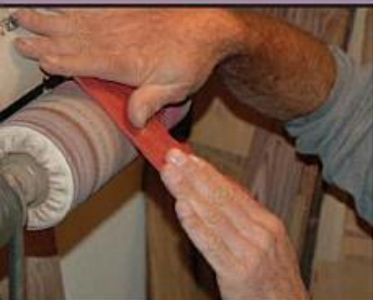
Using a pneumatic drum sander, sand the edges of the sections of your choice down to create a relief effect.
