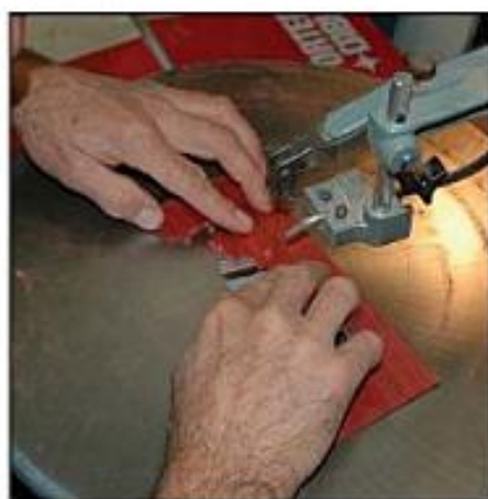
Using a very fine blade, cut out each of the puzzle pieces leaving a lobe or a socket on each side of the piece.
