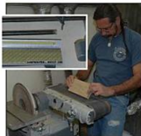
Sand the puzzle first with a belt sander and then with a pneumatic drum sander to soften the edges.
