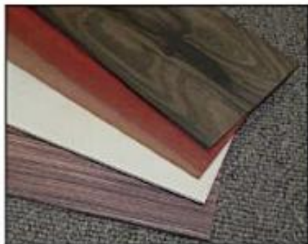
Re-saw and sand the four pieces of wood to \frac{5}{32} "-thick.
