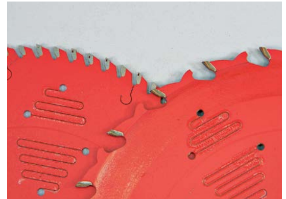
The author's go-to blades for puzzle making are an 80-TPI crosscut blade (left) and a 24-TPI rip blade (right).
