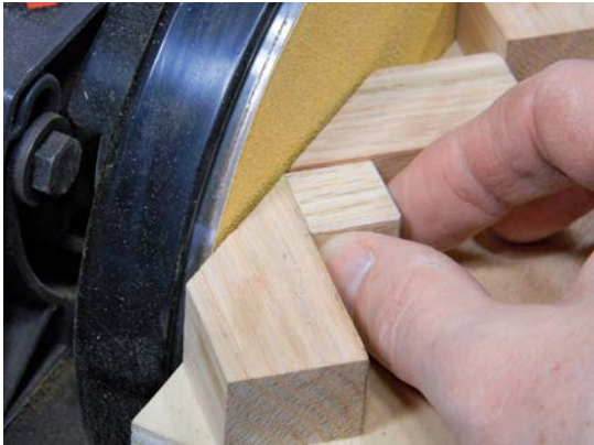
Bevel all 12 edges of the cube, applying consistent pressure so that the bevel is a consistent width from the top to the bottom of each edge (below).
