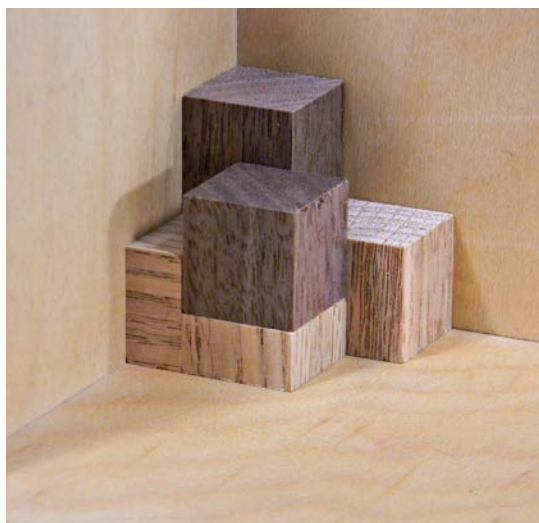
You will be adding either full or half-spacers with each successive piece to raise them up and shift them over. Substitute a full spacer for two half-spacers when necessary.
