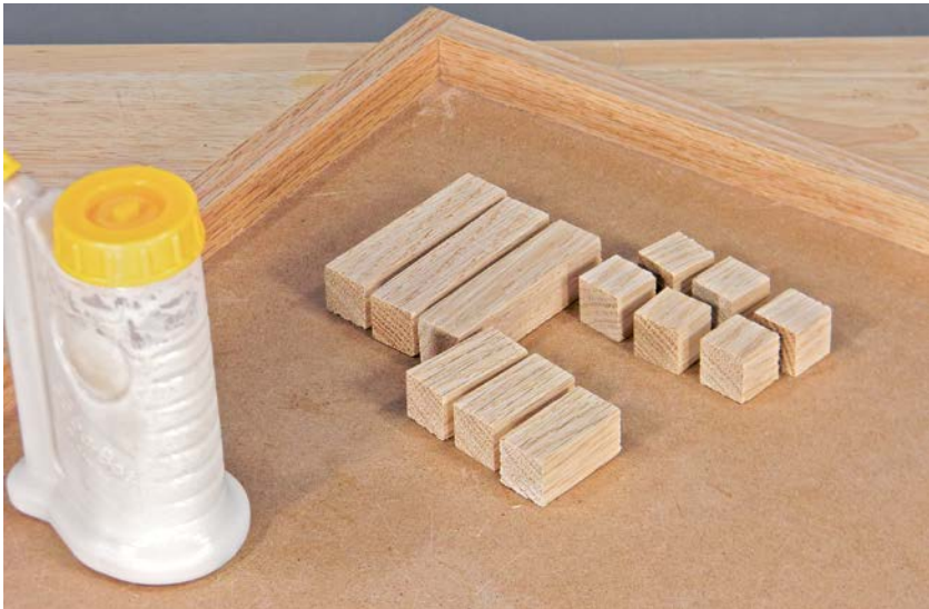
With all 12 pieces cut, you are ready to begin construction on the large flat-gluing jig.
