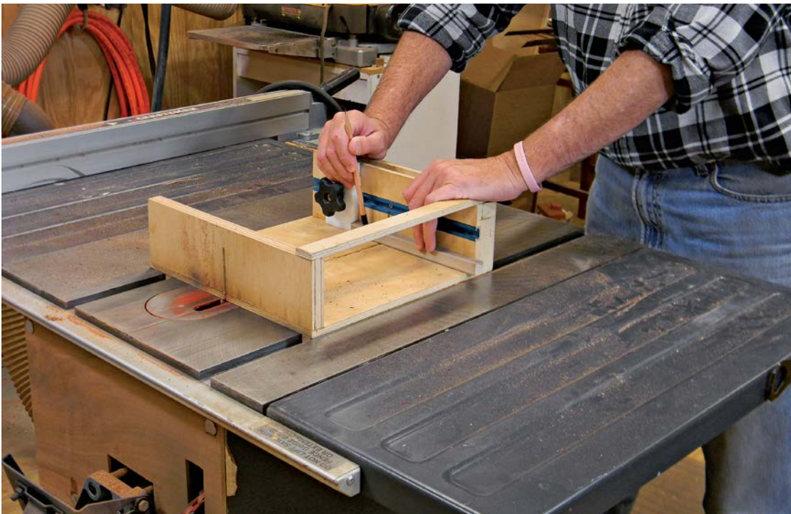
A tablesaw (shown here with a crosscutting jig) is an essential tool for puzzle making.
