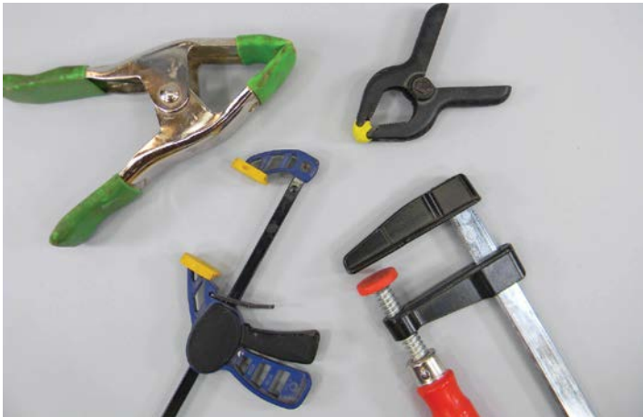
Spring clamps (top) and the blue quick-grip mini-bar clamps (bottom left) see a lot of use in puzzle making. A larger bar clamp (bottom right) also comes in handy for jig making.
