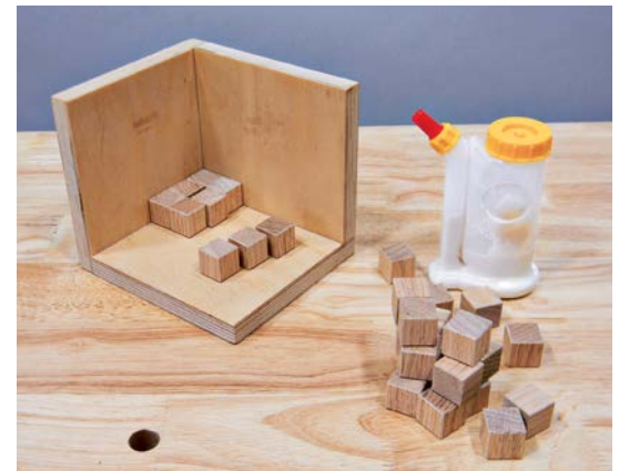
Use the corner-gluing jig (see p. 23) for gluing up the cubes.
