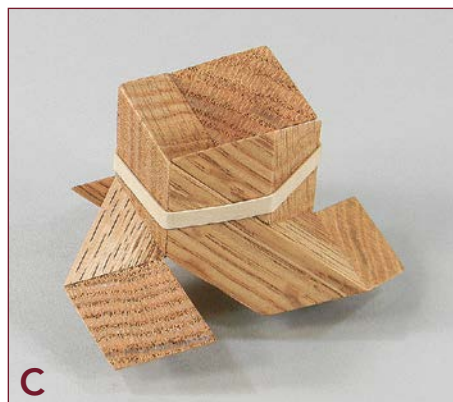
Here is where the rubber band or tape comes into play. Wrapping a rubber band around the trunk of your first assembly will enable you to make the second assembly more easily.
