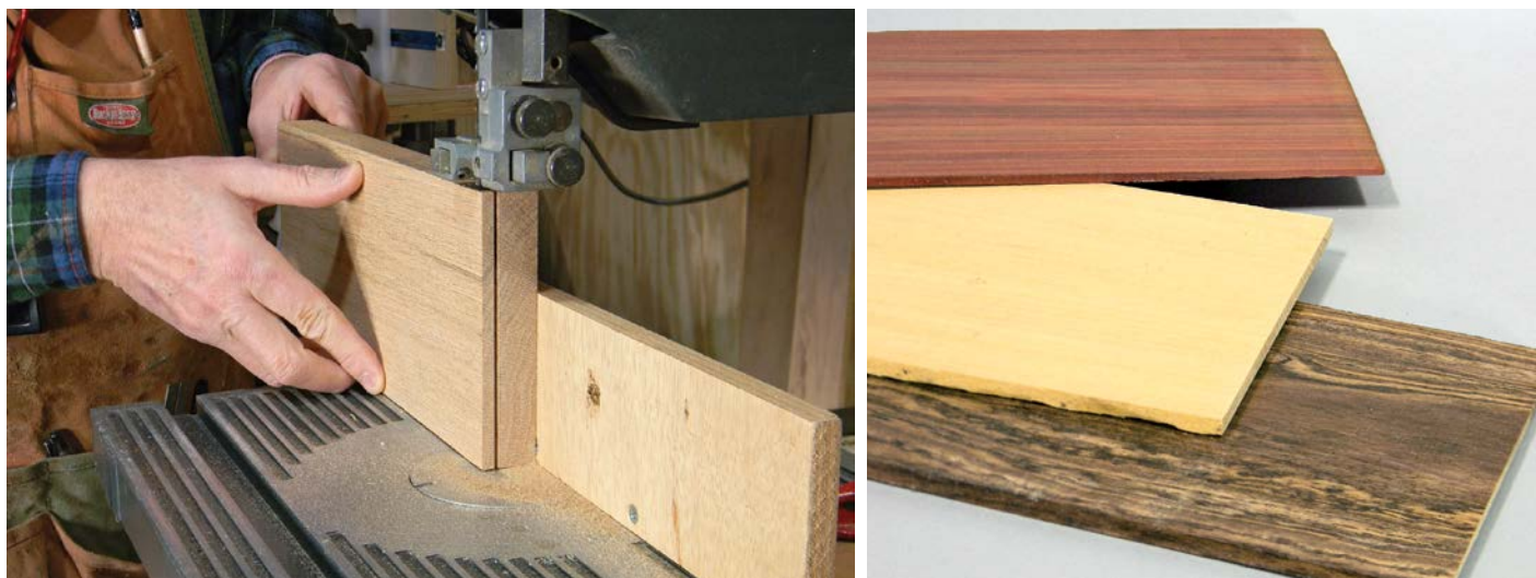
Resawing 4/4 or 5/4 stock on a bandsaw allows you to double your yield from a board. Pieces as thin as 1/4 in. (right) can be used for some puzzles in this book.
