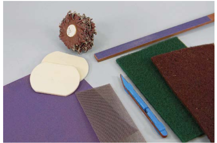
A variety of sanding options are available. The author keeps several sanding mops, abrasive pads, and sanding sticks close at hand. Shop-made sanding sticks, like the one in the upper right, also come in handy.
