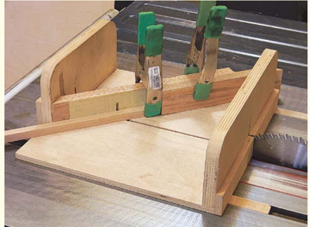
Use a stop block with the miter sled to cut the frame pieces to a consistent length.
