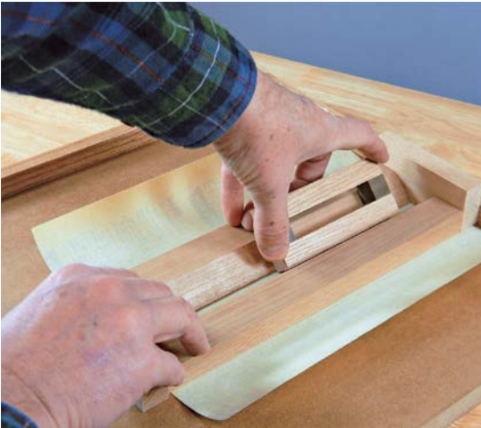
Use the long edge-beveling jig over a sheet of 180-grit sandpaper to bevel the edges of the finished parts.
