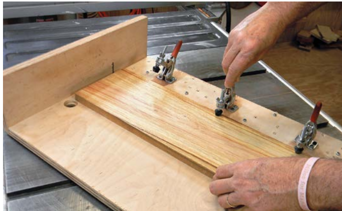
To use the ripping jig, place the stock flush against the stock and hold it in place with the three clamps.
