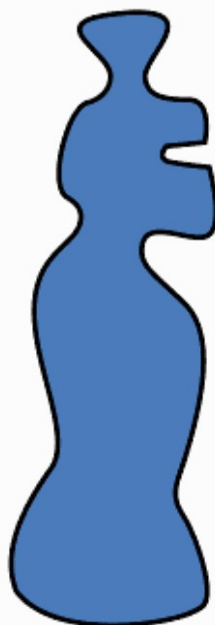
BODY ACTUAL SIZE MAKE 1 7/8" thick wood cut from 2 x 4
