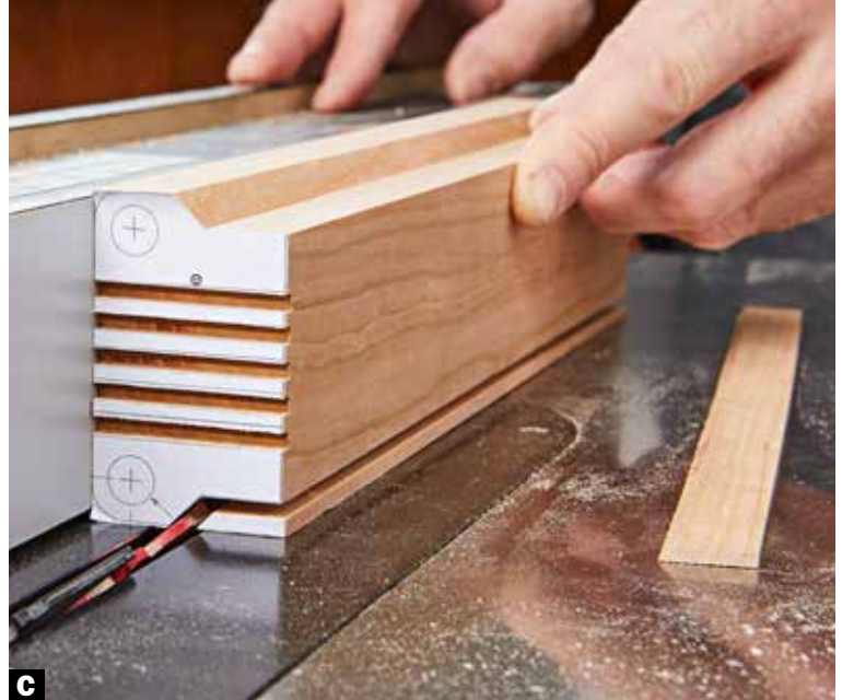
C Two cuts create the fender wells. Make the first cut with the blade at 90^\circ ; for the second cut, angle the blade to 45^\circ .
