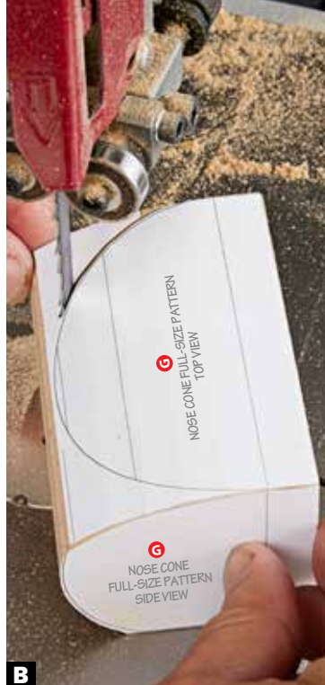
B Bandsaw just outside the line, then sand the blanks smooth.
