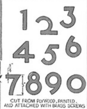
SCROLL-SAWED FROM \frac{1}{4} " PLYWOOD
