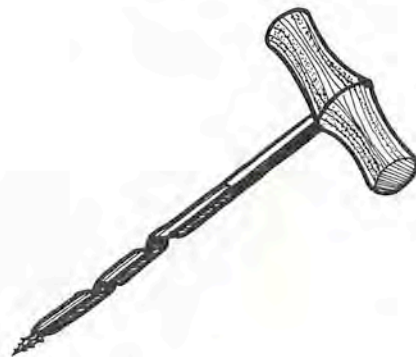
Figure II-23. The gimlet is used to make shallow holes in lumber.
