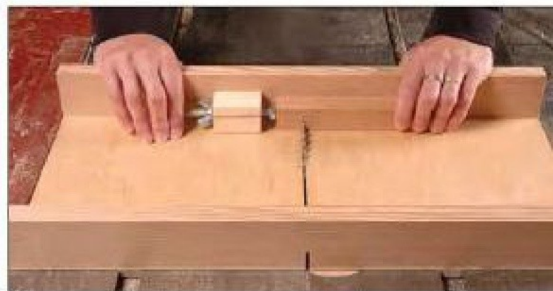
Figure 81—Saw the first cut using the notching jig. Note that if a jig of this type were to be used for through cut-offs, a device to hold the cut-offs in place would be required.
