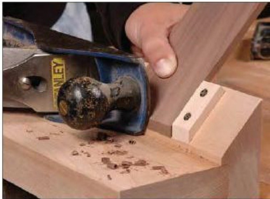
Figure 26—As an alternative to the table saw method, you can miter the box sides using a hand plane and a miter shooting board, also called a "donkey."
