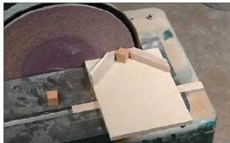
Figure 76—This fixture was designed to hold cubes and limit the depth of cut when making chamfers on the disk sander.
