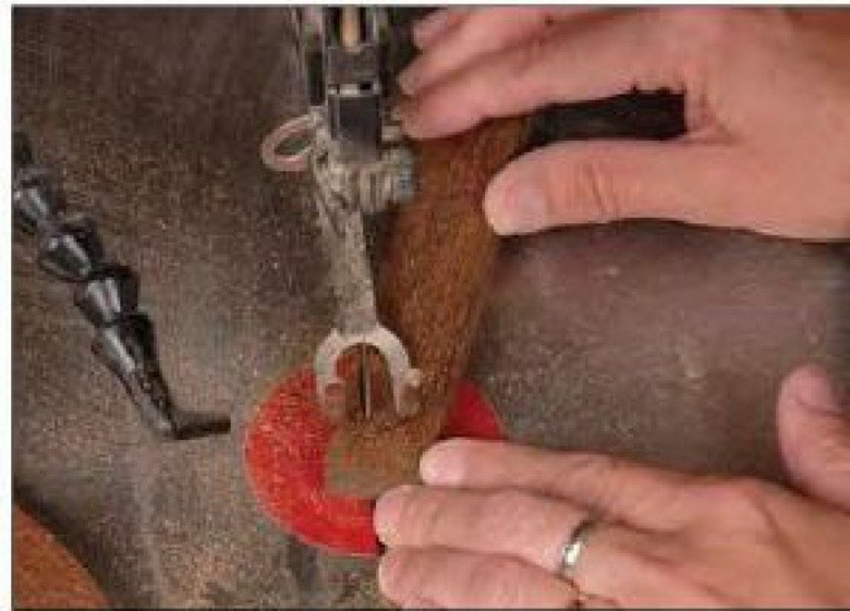
Figure 106—Cut the body of the Celt using a scroll saw or band saw.
