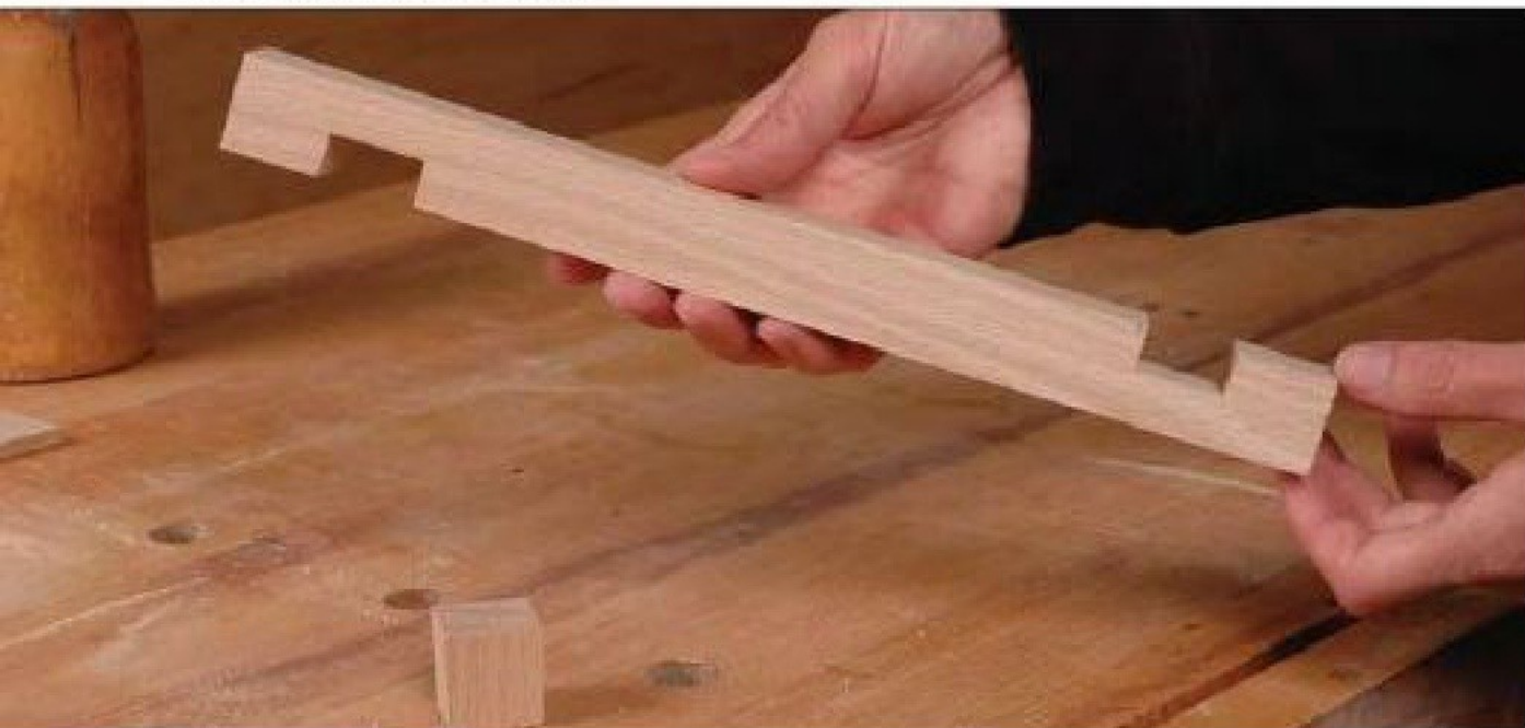
Figure 5—Here is the 12-inch stick with the notches cut and the gage block (left foreground) sawn off one end.
