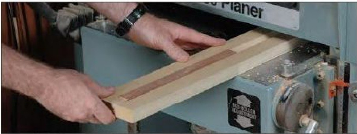
Figure 16—The long prismatic stick sits in the shop made cradle, ready to be pushed into the thickness planer.
