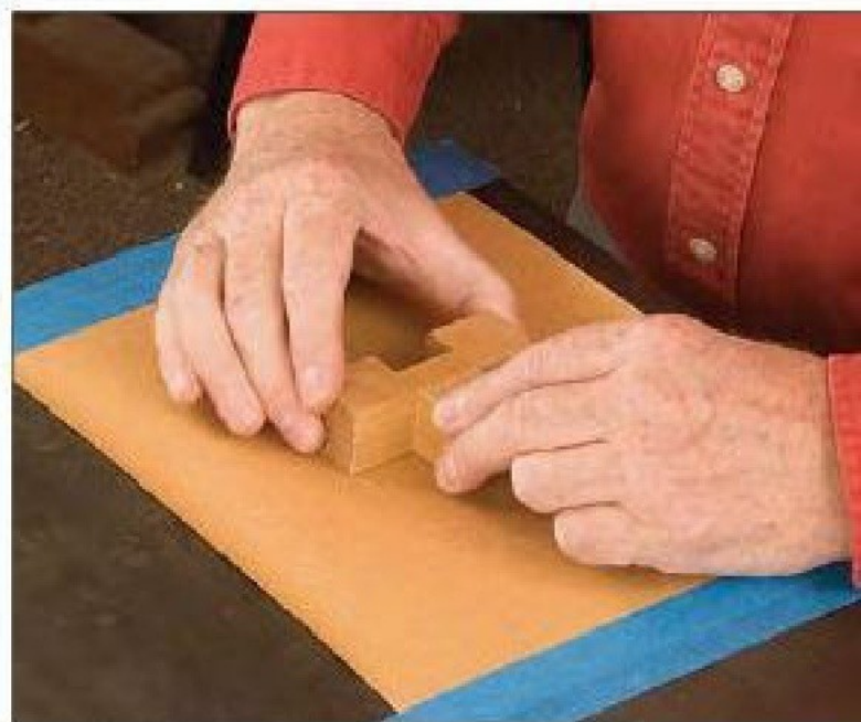
Figure 8—Size the puzzle pieces by rubbing on 280-grit sandpaper that has been taped to a flat surface such as a machine table.
