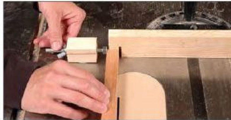
Figure 74—On the table saw, cut the cubes to length using an offset stop attached to the table surface with cyanoacrylate glue
