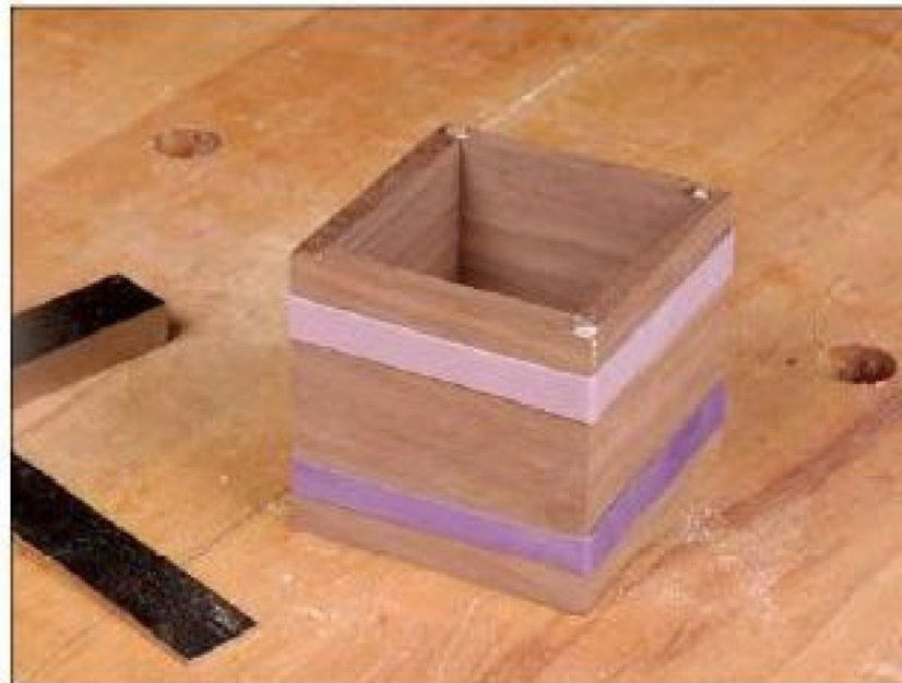
Figure 29—Use heavy rubber bands to clamp the assembled box while the glue dries.
