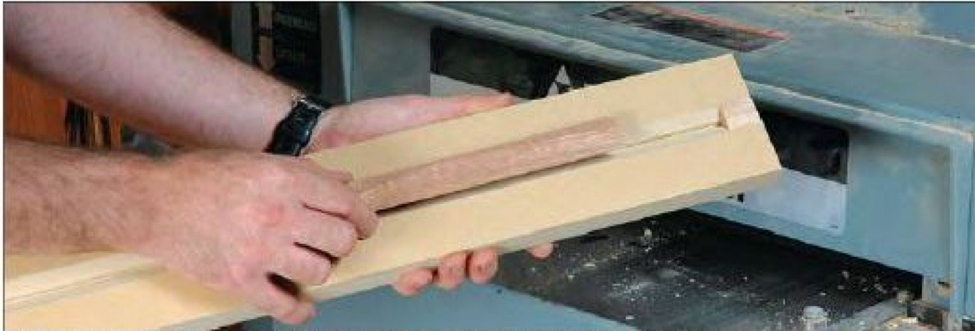
Figure 15—The shop-made cradle, with a stop at one end, is being used with a thickness planer.
