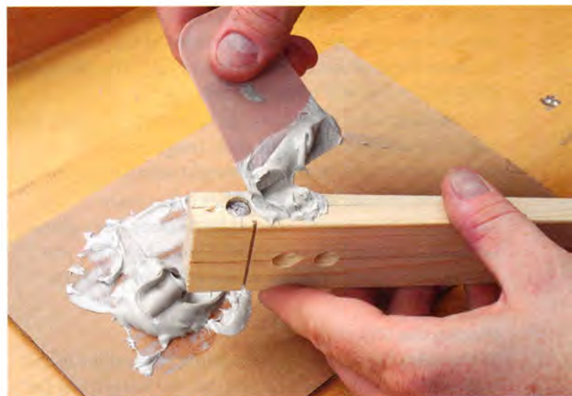
To seal the weights into the car, fill the holes with putty. This is also a good time to fill any nicks or scratches in the car body. Once the filler has dried, sand it flush with the car.
