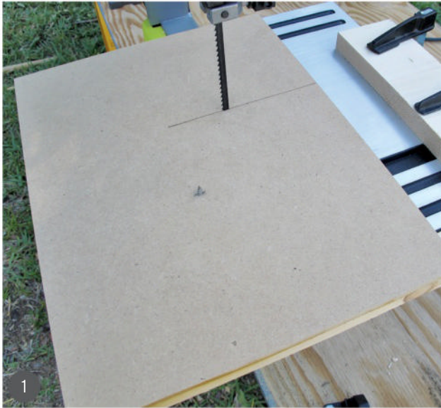
1 Use a simple jig to make cutting the circular checkers an easy task on the bandsaw.
