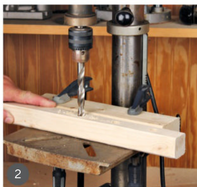
2 Drill the holes for the pegs, aiming for a snug fit.
