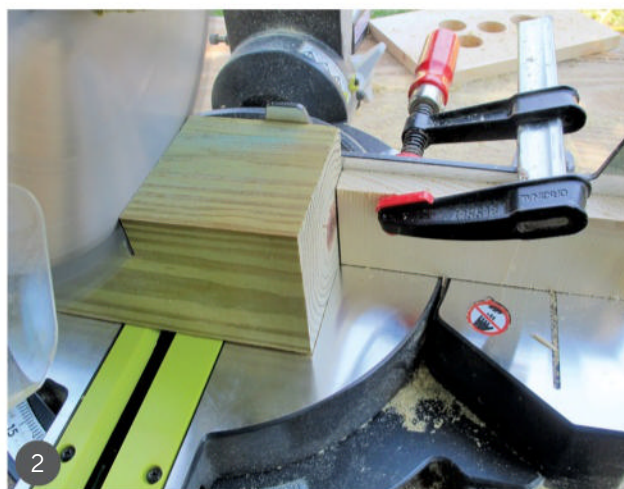
2 The stop ensures consistent cuts to form identical cubes.
