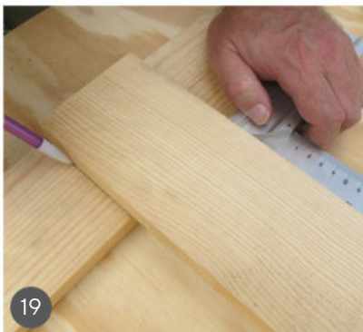
19 Center and square the leg upright on the outer face of the foot, then mark its location.
