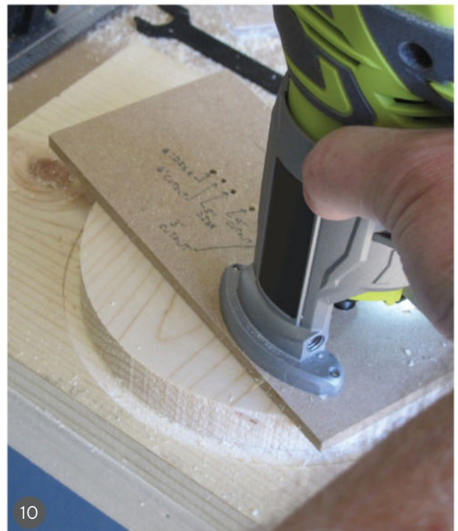
10 Rout the inside diameter in the same way. Finish by sanding all the faces and rough edges.
