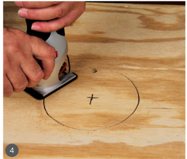
4 Mark and cut the hole in the top, then sand the rough edges.
