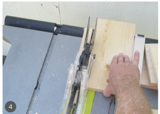
4 With one of the long edges of the tile tight against the rip fence, rip each tile to final width.
