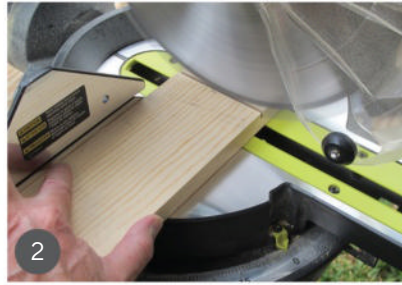
2 Cut the table sides and ends to length.
