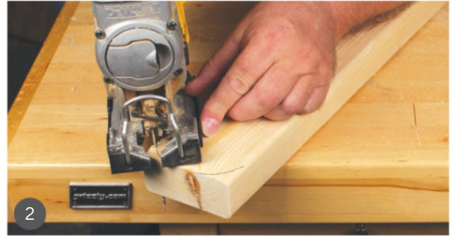
2 Saw the radius on the end of each arm.
