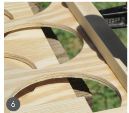
6 Glue and clamp the remaining frame pieces in place.
