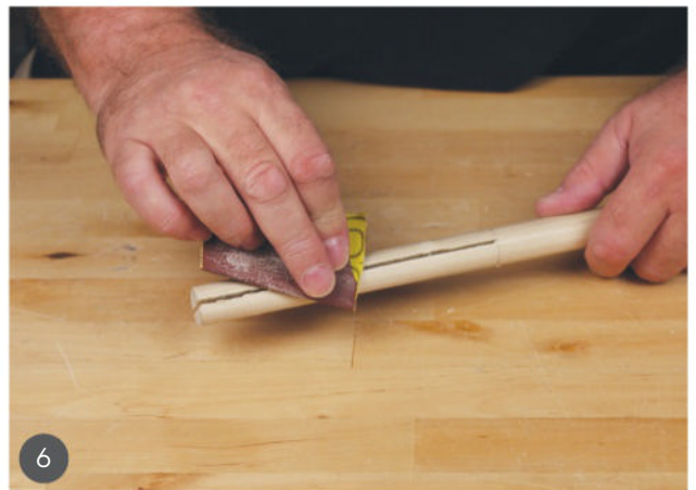
6 Sand the shaft ready for the flights.
