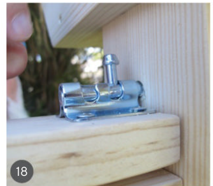
18 The barrel bolt aligns with the hole in the leg assembly.
