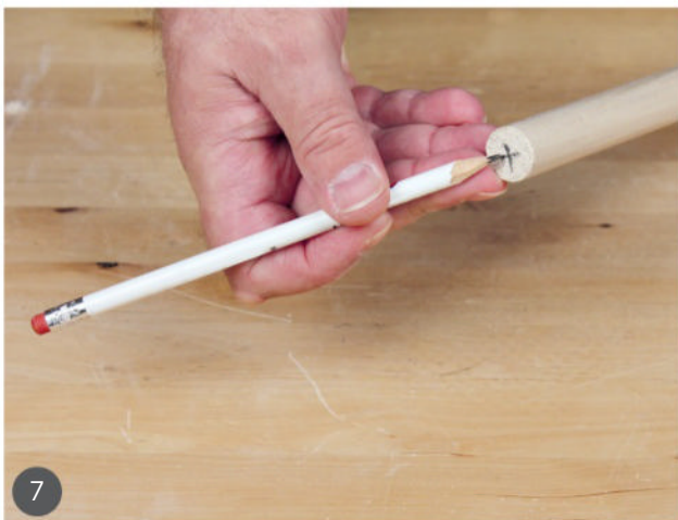
7 On the other end, mark the center of the shaft ready for the screw.
