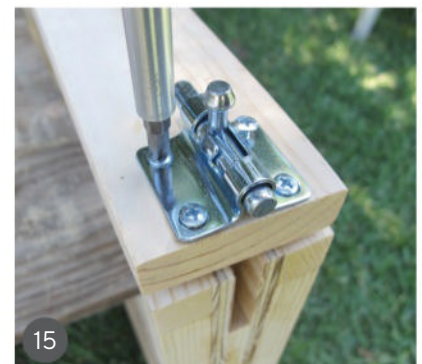
15 Attach the barrel bolt at one end of the disc-release door.
