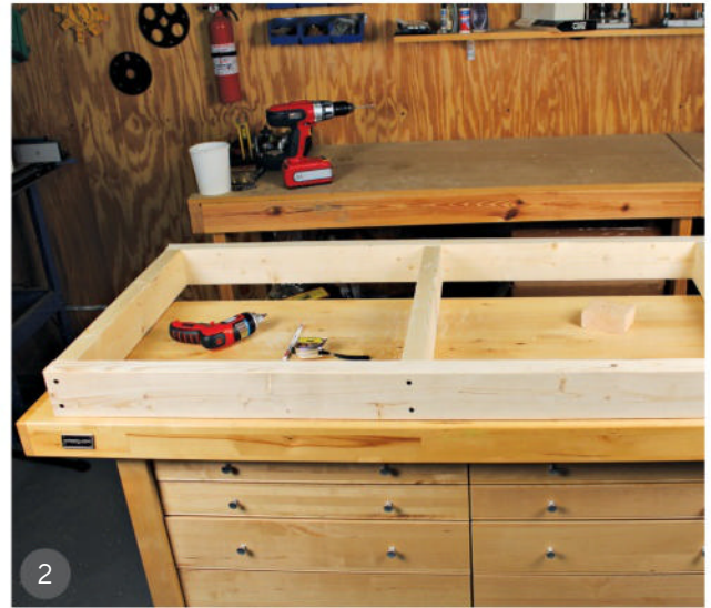
2 Screw all the frame parts together.
