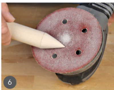
6 Sand the point smooth—though it won't remain this way after it has been hammered into the ground a few times!
