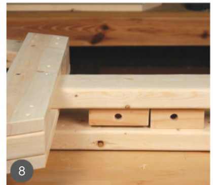
8 Be sure to stagger the brace mounts so they clear one another when the catapult is folded.
