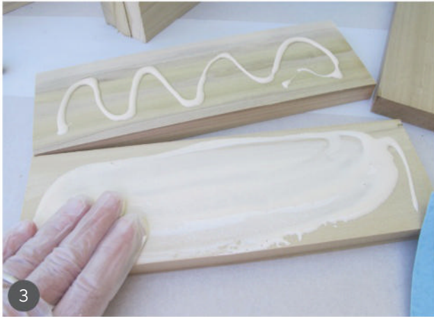
3 Apply an even coat of glue.
