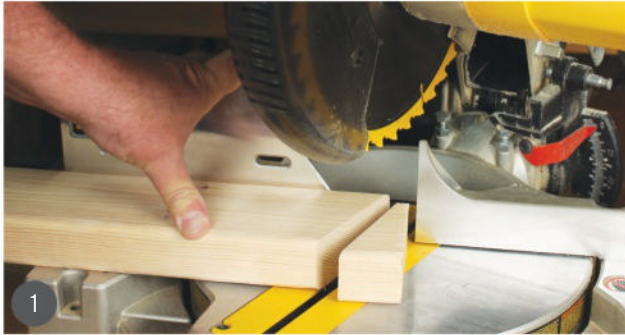
1 Cut the angled ends on the crossbars.
