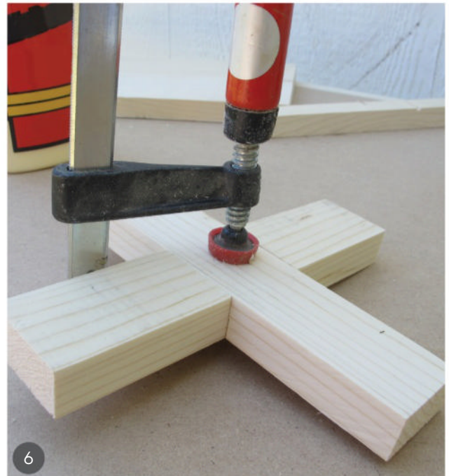
6 Clamp the parts together until the glue has set.
