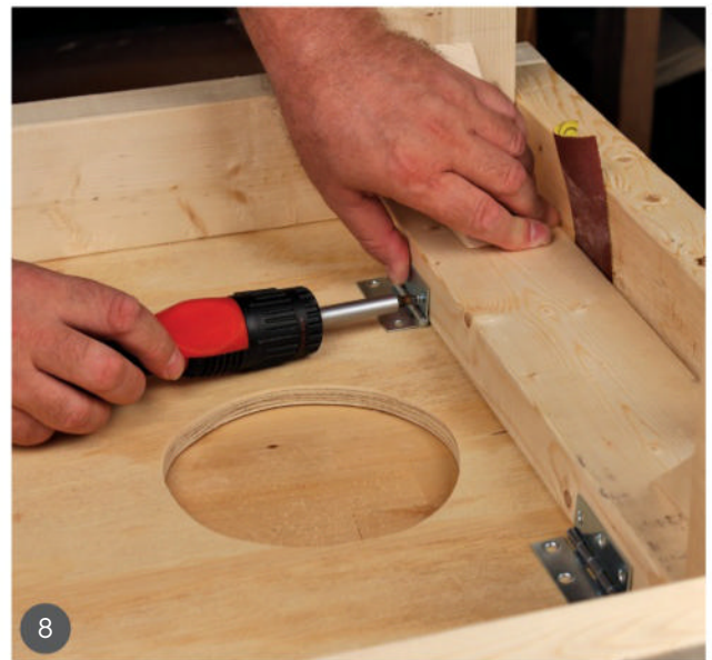
8 Place the leg assembly in the underside of the frame and attach the hinges. Repeat to make a second table.
