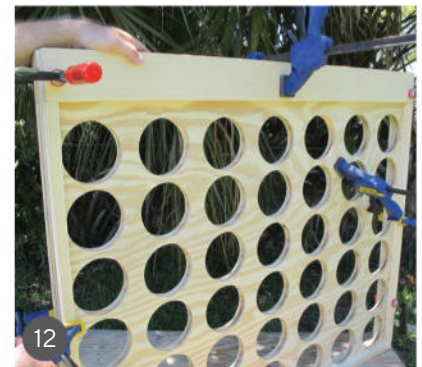
12 Clamp the panels together, ensuring the edges are flush.
