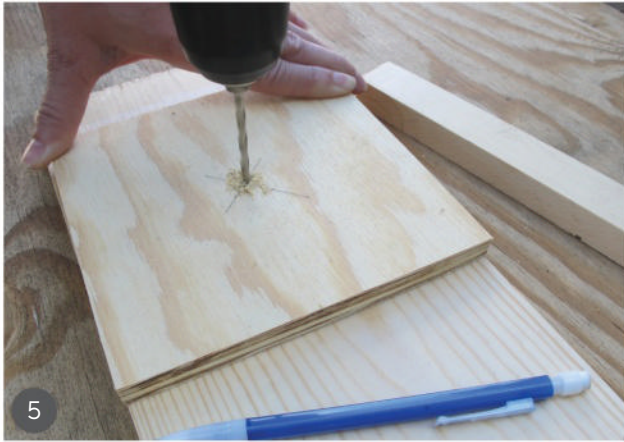
5 Drill a pivot hole in each blank to fit over the pivot pin in the jig.
