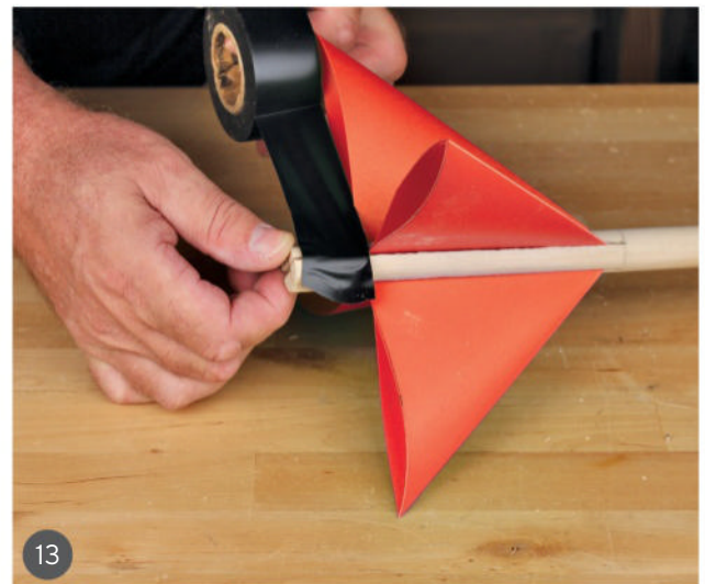
13 Use electrical tape to hold the flight in and close the cross on the end of the shaft.
