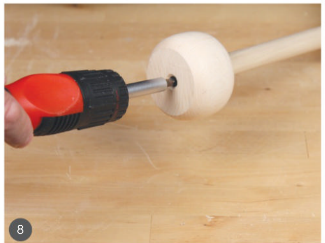
8 Drill into the end of the shaft, then screw the head of the dart to the shaft.
