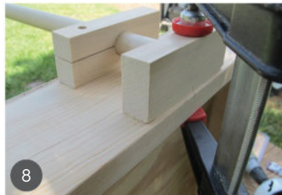
8 Glue and clamp the brackets in the center of one of the table sides, then insert screws. Use the long dowel to check alignment.
