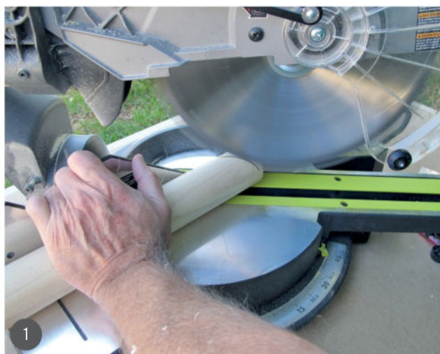
1 Set the saw to make a 45° cut, then trim the end of the first dowel blank.
