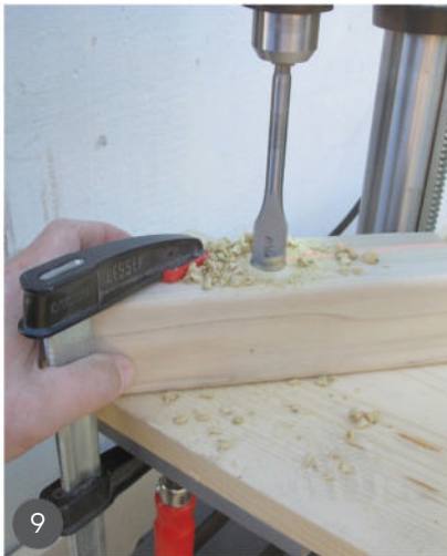
9 Drill the hole for the handle in the mallet head.
