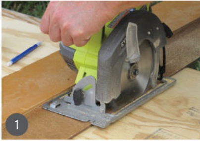
1 Use a circular saw and straightedge guide to cut the plywood for the table top into a 24in (610mm) square.
