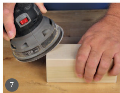
7 Sand all the pieces and round over the corners.
