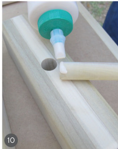
10 Apply glue and tap the handle into the mallet head.
