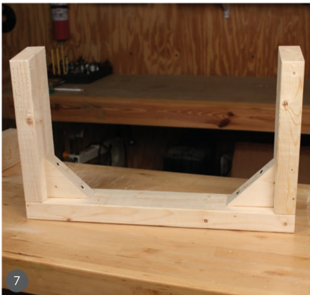
7 Screw the leg assemblies together.
