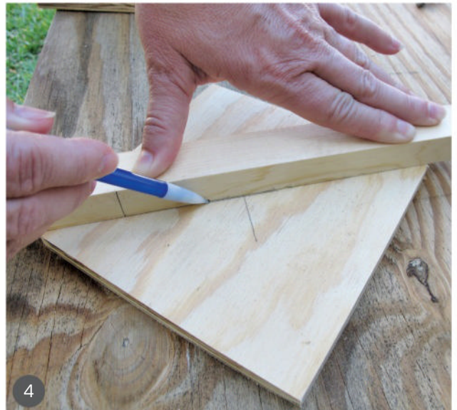
4 For a quick way to locate the center, mark the diagonals of the square blanks.
