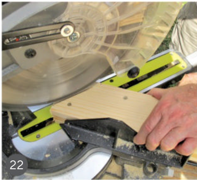
22 Lay out and cut the angled corners of the feet.
