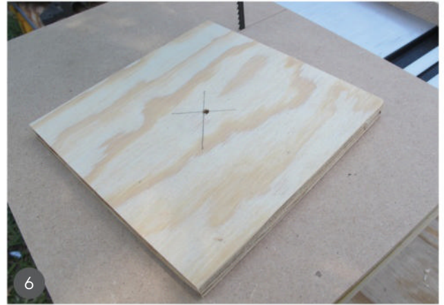
6 Position the blank over the pivot pin before switching on the saw.
