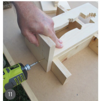
11 Use a pair of screws to attach the base to each chess piece.
