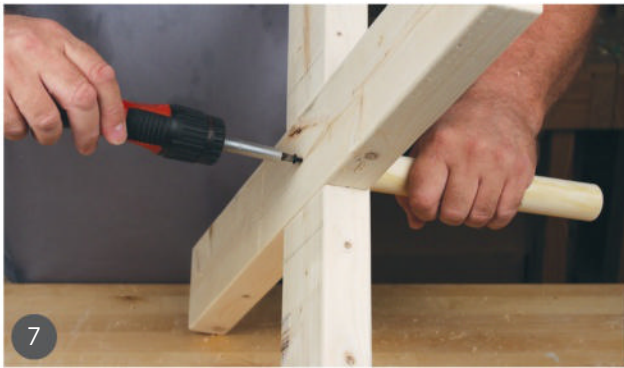
7 Screw into the pegs from the underside; the central screw will hold the joint together.
