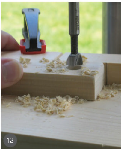
12 After cutting the hoop crossbars to length, drill holes for the uprights.
