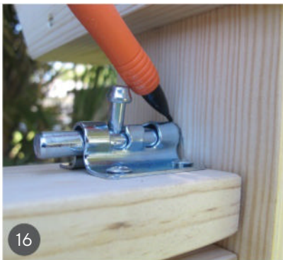
16 Mark the bolt location on the leg assembly.
