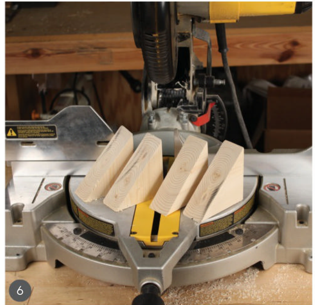
6 Cut four corner blocks to brace the leg assembly.
