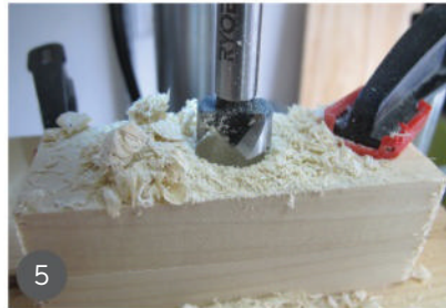
5 Drill the hole for the post into both brackets.
