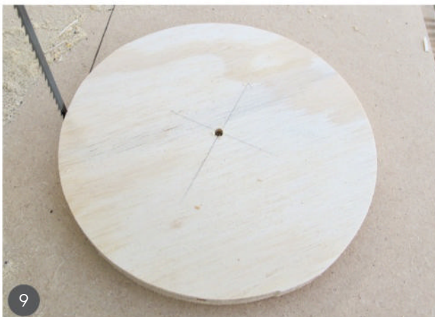
9 Remove the disc from the jig and repeat the process for the other blanks. Finish by sanding the edges and staining half the discs a dark color.
