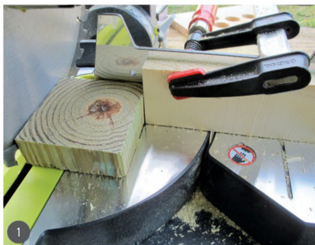
1 Cut a scrap piece from the end of the post and, using this as a guide, clamp a piece of wood to your miter saw to act as a stop.
