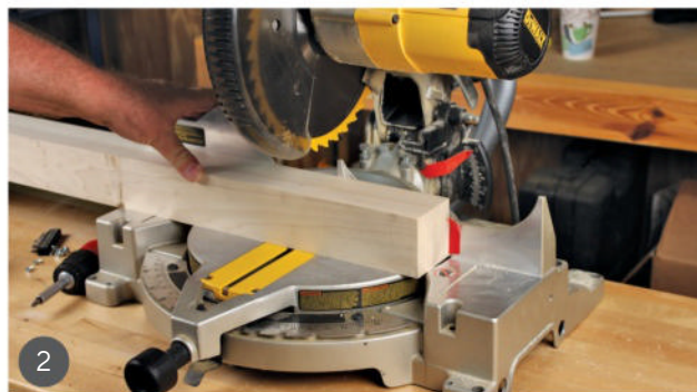
2 Cut the ten kubbs to 6in (150mm) long from timber 3in (75mm) square.
