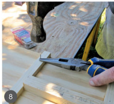
8 Glue and tack the dividers in place, using temporary spacers to position them accurately.
