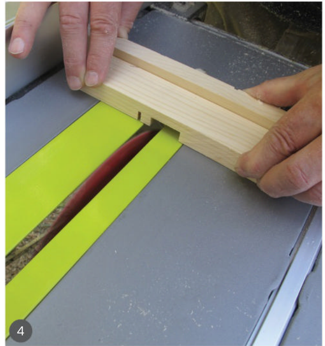
4 Remove the waste on the tablesaw. Make sure the blade guard is fitted; in the photo it has been removed for clarity.
