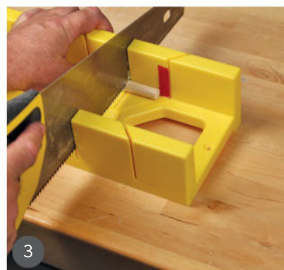
3 Cut the pegs to length; a miter box with a piece of tape to act as a length stop makes quick work of this.
