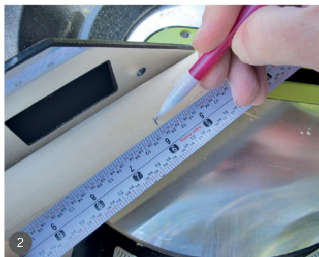
2 Make a mark 6in (150mm) from the tip of the angled end of the dowel.
