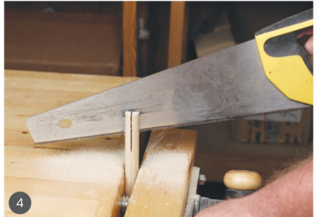
4 Make the saw cuts in easy stages.
