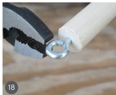
18 Install a screw eye into the end of the dowel and insert the dowel into the brackets.
