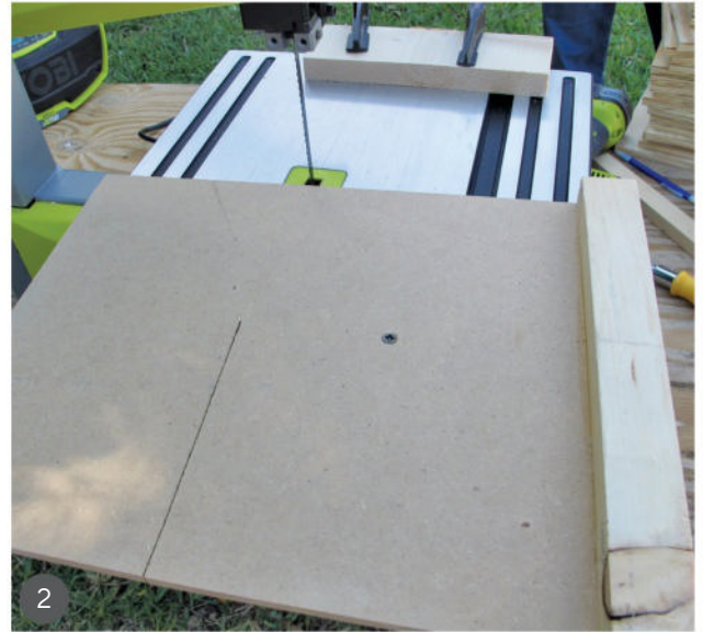
2 The underside of the jig features a cleat (shown at right) to register against the edge of the bandsaw table.
