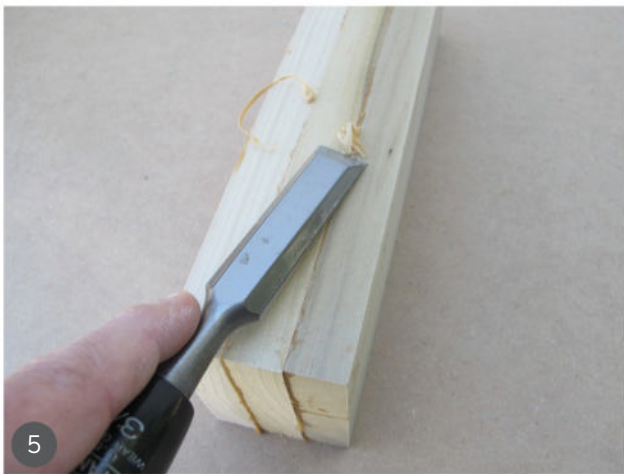
5 Use a chisel to remove dried, squeezed-out glue.
