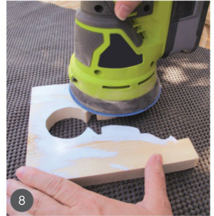
8 Sand the pieces to remove all traces of the pattern.
