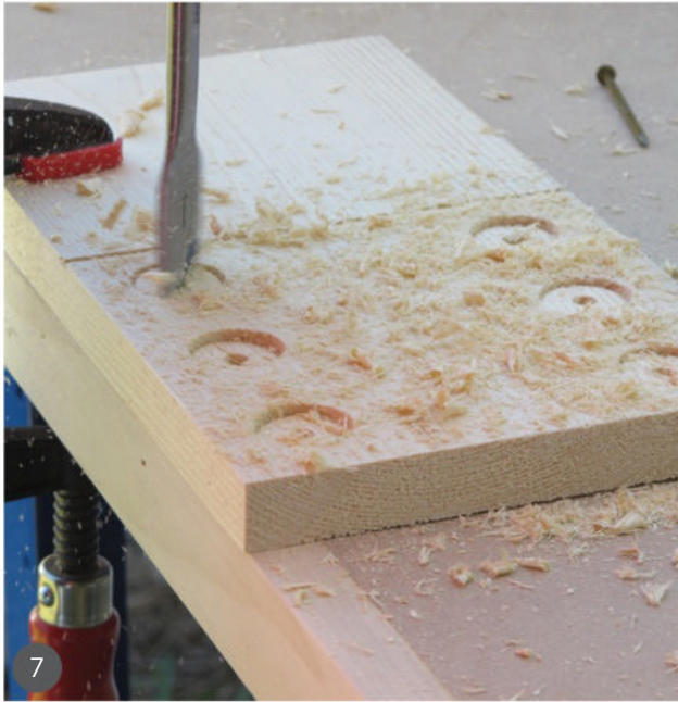
7 Drill a shallow hole to represent each of the pips. If you have a drill press, you can set the depth stop to ensure consistent depth.
