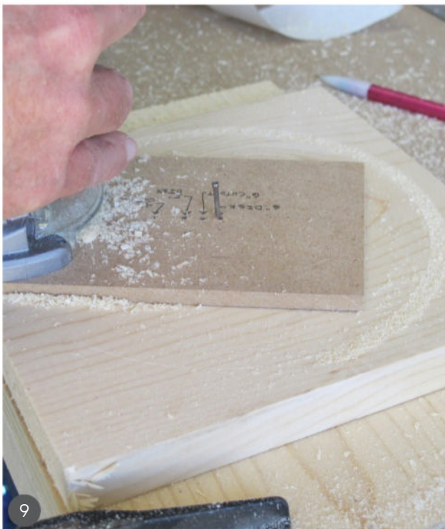
9 Rout the outside diameter, using this simple jig made from an offcut of MDF.
