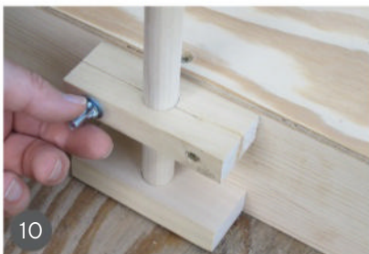
10 Insert the carriage bolt from the inside and install the washer and wing nut.
