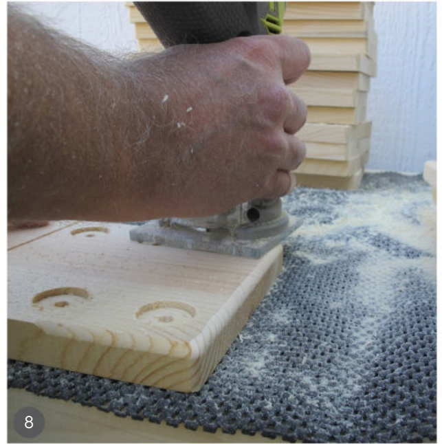
8 Use a roundover bit and sandpaper to smooth all the sharp edges on both faces of each tile.
