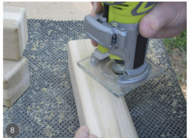
8 Round over all the edges with a router.
