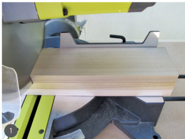
1 Stack up three boards and cut them to roughly 11in (280mm) lengths.
