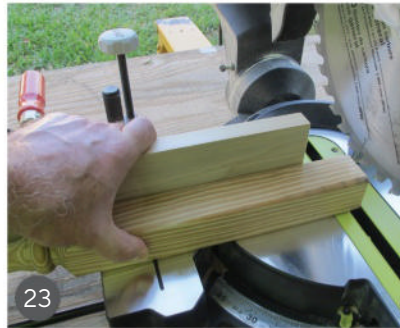
23 Trim the ends of the spindles square so they stand straight on the table.
