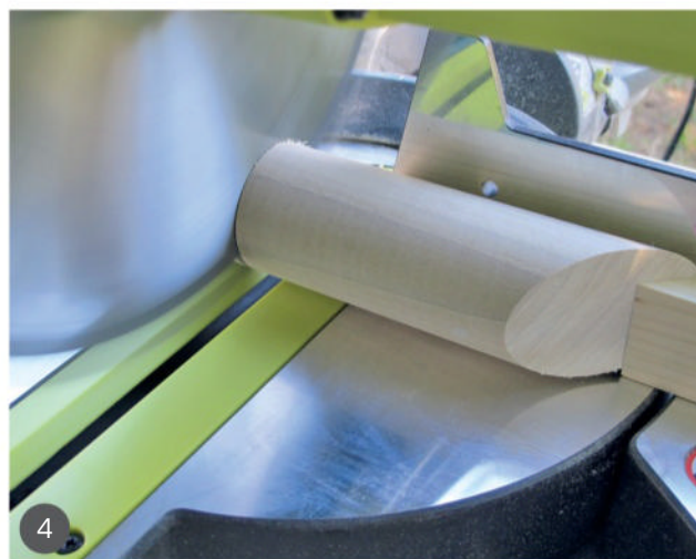
4 The stop block helps to secure the dowel and ensure consistent cuts.
