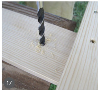
17 Drill a stopped hole 1/2in (12mm) deep in the leg assembly for the barrel bolt to engage.
