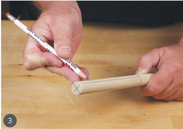
3 Mark the cuts for the flights. You can do this freehand, using your finger as a pencil gauge.
