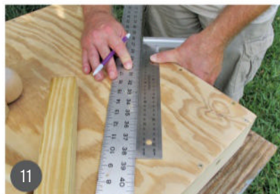
11 Lay out the squares on the table top using a straightedge and a miter square.
