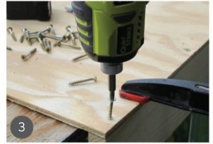
3 Screw the ends to the top.
