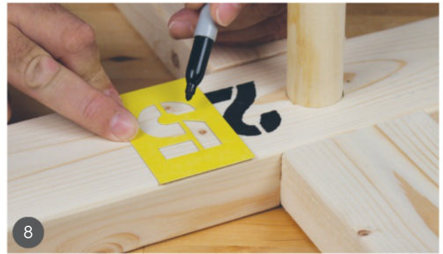
8 Use stencils to mark the scoring numbers.
