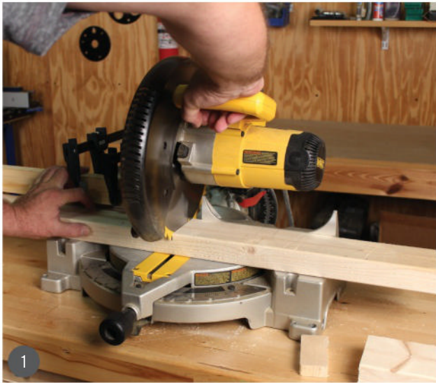
1 Cut all the frame parts to length.
