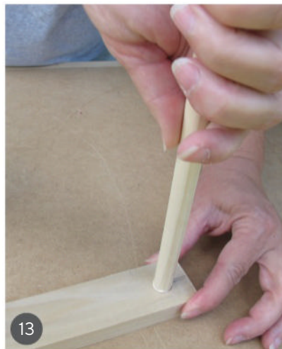
13 Glue the uprights into the crossbars and tap them home.
