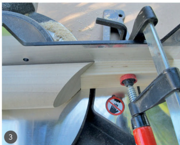
3 Make an angled stop block and locate this to make a cut 6in (150mm) from the tip of the dowel.
