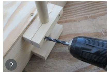
9 Use the 1/4in (6mm) hole in the bracket as a guide to drill through the table side.
