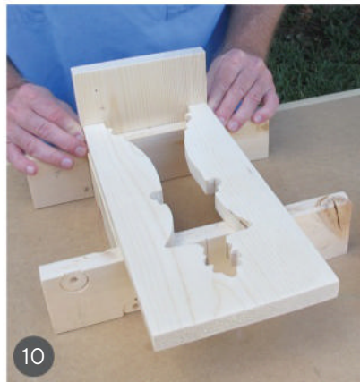
10 Place the chess piece on the alignment jig.
