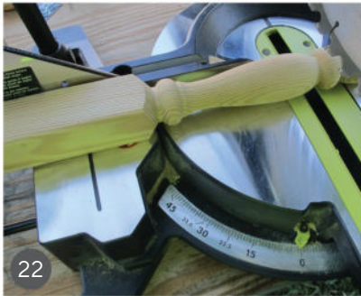
22 Use the chopsaw to cut the spindles to create a pair of pins.
