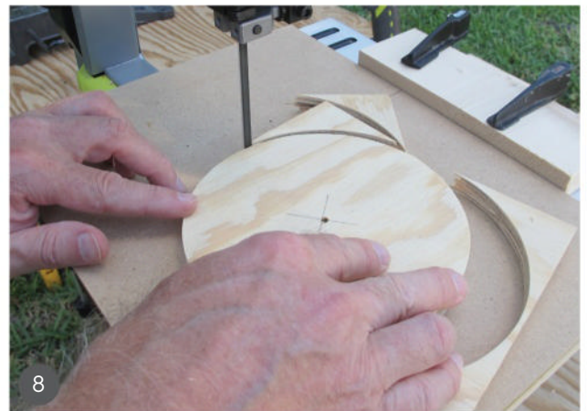
8 Continue turning the blank steadily to complete the cut.
