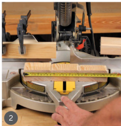
2 Measure the width of three blocks side by side.
