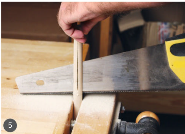
5 Hold the top of the shaft to reduce vibration as you approach the final depth.
