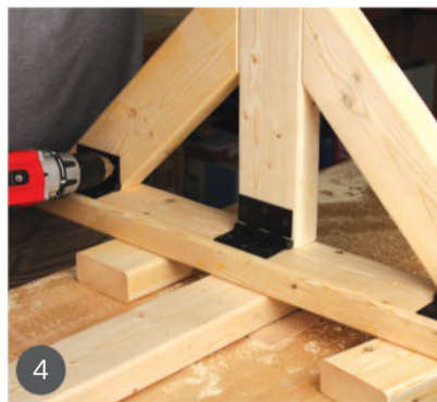
4 Attach the hinges to the upright and the diagonal braces.
