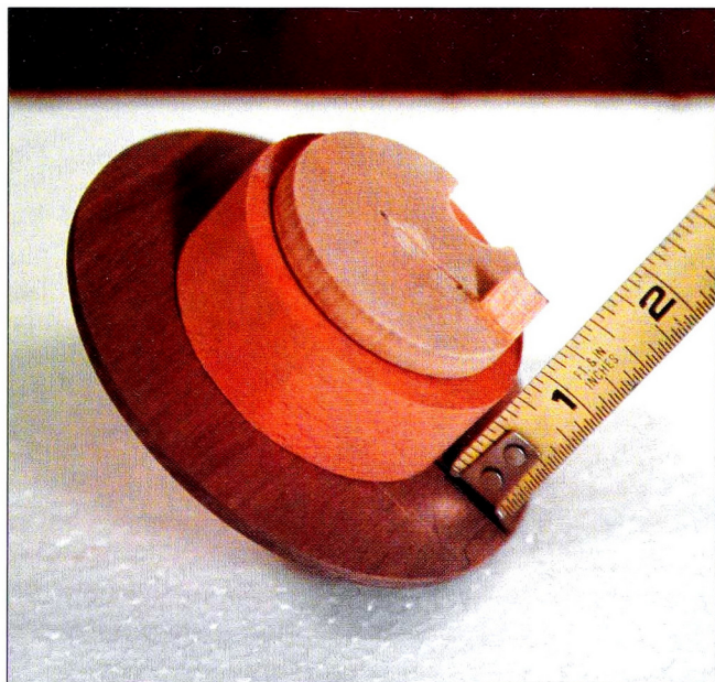
Photo 41: Measuring Length of Drive Pin from Dial Back
