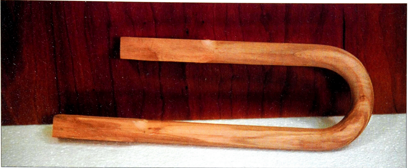
Photo 4: Shackle Rounded Over, Not Cut to Length
