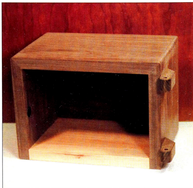
Photo 31: Safe Body Glued Together
