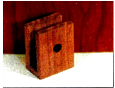
Photo 18: Completed Shackle Mounting Block
