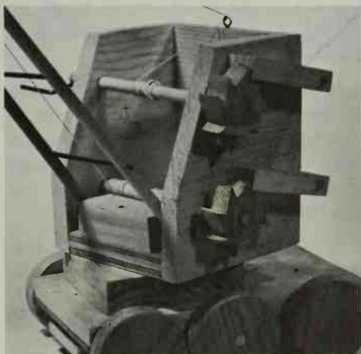
Here's a close-up view of the ratchet wheels and the pawls.
