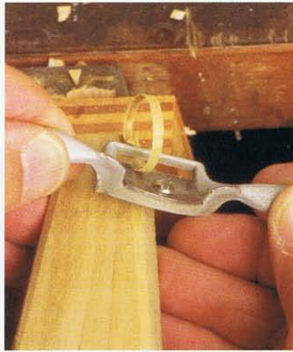
Photo J • To cut the radius on the hoods, a miniature spokeshave will also do the trick.
