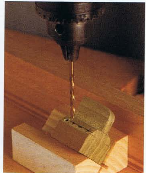
Photo AA • Aluminum or painted wooden pins inserted into \frac{1}{8} -in. holes drilled into the engine block provide the exhaust pipes.
