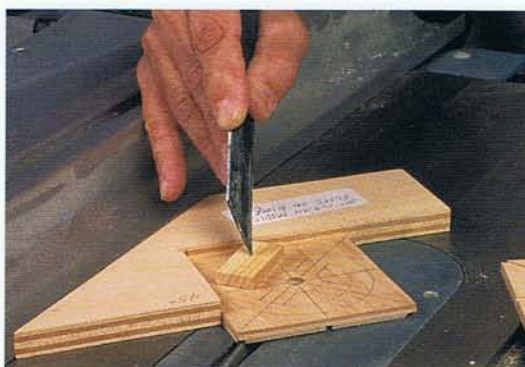
Photo BB • A simple jig provides the corner-to-corner slots in the wheel blanks.
