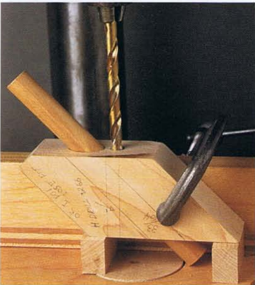
Photo K • Notoriously difficult to do, drilling angled holes in dowels is made easy with this jig. Here the crane post gets an accurately centered 45-degree angle hole to receive the arm.
