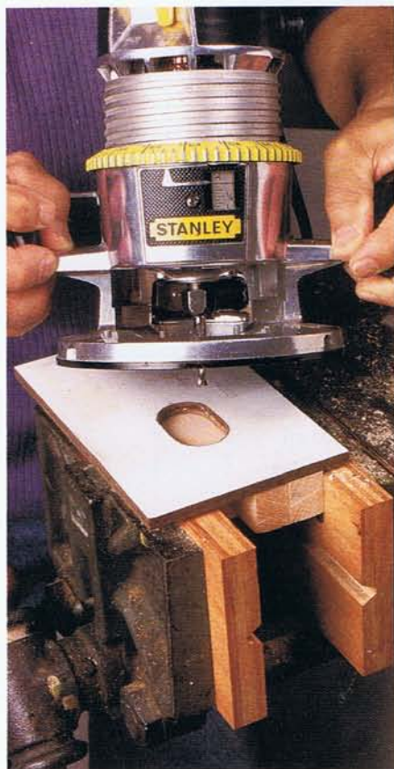
Photo C • Clamp the template and workpiece in a vice and rout the partial-depth windows.
