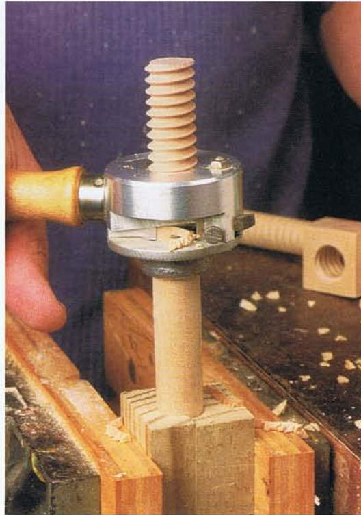
Photo 1 • While threading dowels, a bored-out block, cut in half, holds the dowel securely in the vise without marring its surface.
