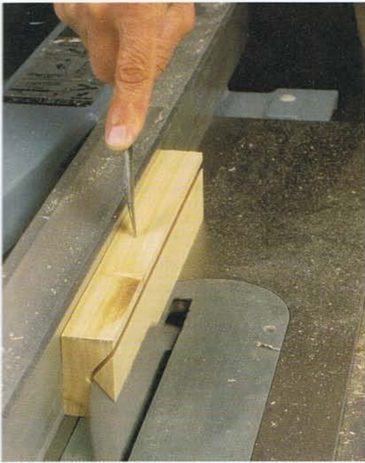
Photo G • With the blade set at 40 degrees, cut a V out of the center of the blank. Make the cut for the first side of the V in a couple of passes, bringing the blade up to the height of the apex.
