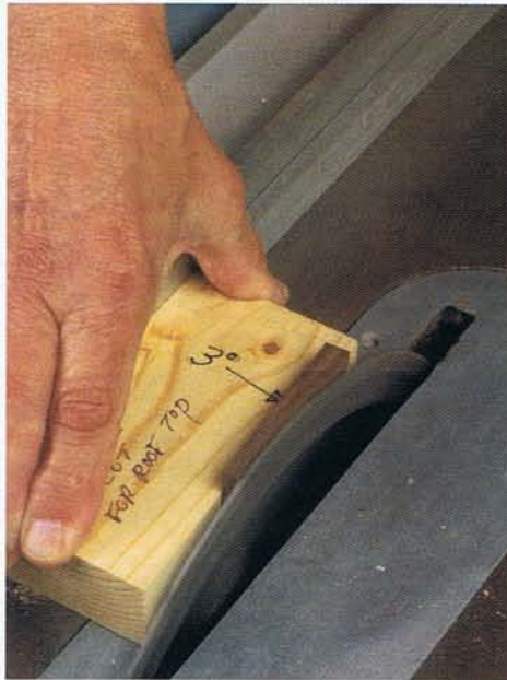
Photo L • The walnut roof cap for cab #5 is secured with double-sided tape to a slightly tapered block for the shallow angle cut.
