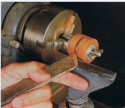
Photo K • Separate wheel blanks you're turning on the lathe with a couple of washers so that you can round the edges without cutting into another wheel.
