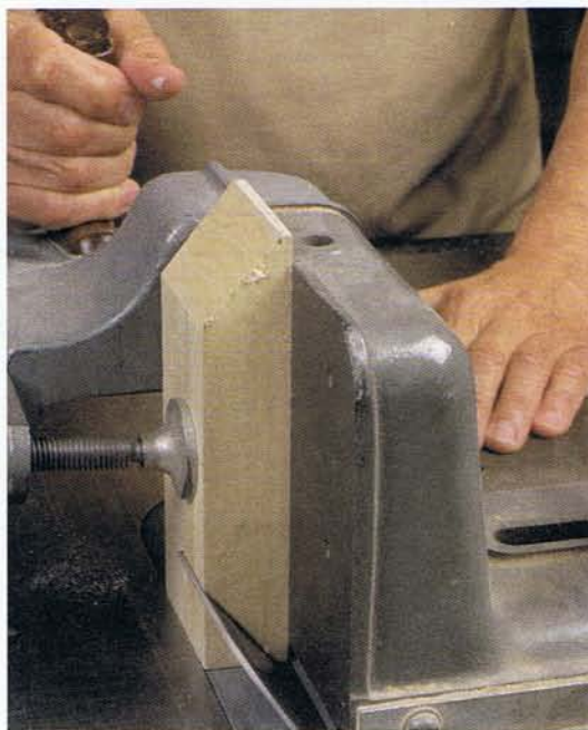
Photo C • A table-saw tenoning jig holds the roof blank securely in a vertical position to make the angled end cuts on the hip and half-gable roofs.
