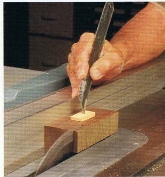
Photo F • An auxiliary block fastened to the top of a workpiece protects the surface from being marred by the tip of the push stick. Use a softwood block to give the stick something to bite into.
