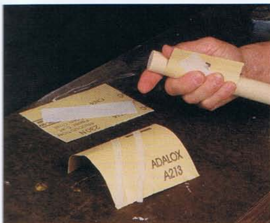
Photo N • For a firm grip when sanding dowels, apply rolled strips of masking tape (sticky side out) or double-sided tape to the back of the sandpaper.
