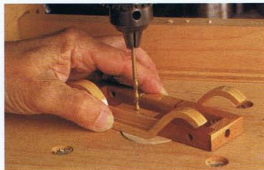
Photo G • Drilling the mounting pinhole through the fender flange into the chassis ensures the alignment of the components.
