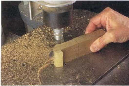
Photo O • Use a \frac{3}{16} -in. router bit to contour the trunk area of cab #10. This operation can also be performed on a router table.
