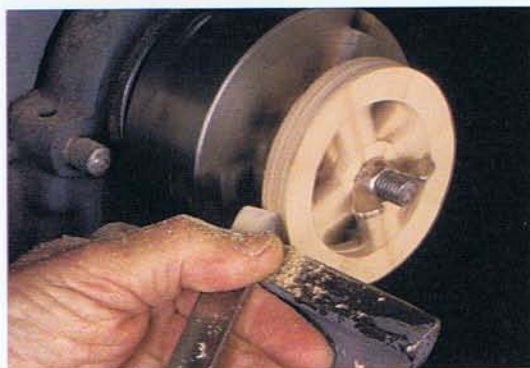
Photo EE • The two wheel blanks are trued together on the lathe.
