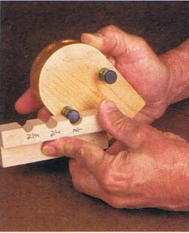
Photo C • Slide this jig up against a lug to make sure it's square to the component's surface before the glue sets.
