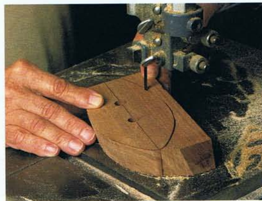
Photo B • The bandsaw's tilting table provides the 10-degree angle of the hull's curved perimeter.
