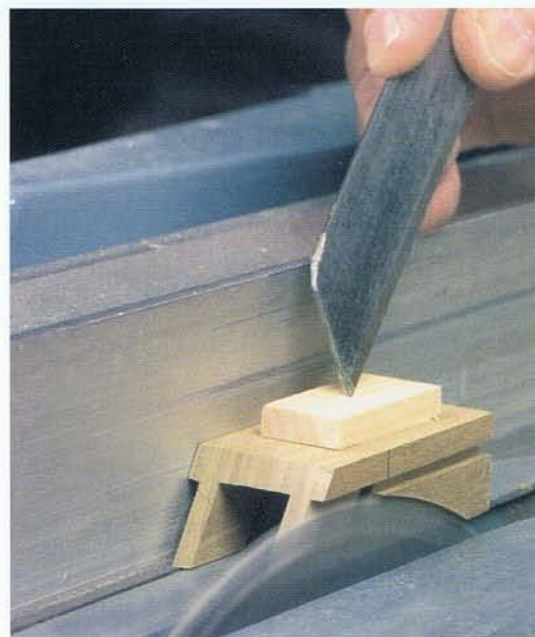
Photo JJ • Table saw cuts along the side complete the support block rabbets.
