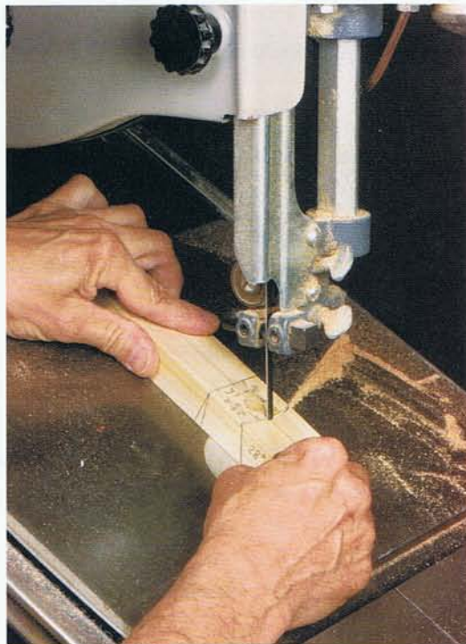
Photo F • For safe handling while shaping on the bandsaw, use a 6-in.- to 8-in.-long blank for the cruiser bridge.
