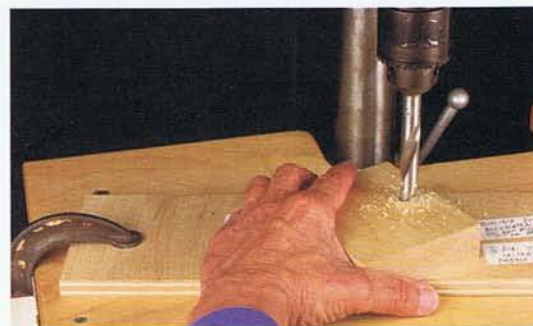
Photo B • To drill an aligned receiving hole, the lug cavity on the workpiece is seated over the lug in the jig.
