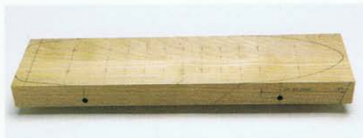
Photo E • Start with a hull blank slightly oversize in length to facilitate cutting the front curve.
