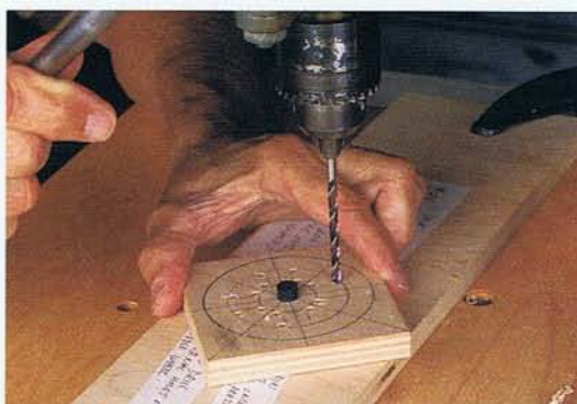
Photo CC • To drill the holes that define the cutout areas, the sandwiched wheel blanks are rotated on a plate with a protruding pin that is clamped to the drill-press table. The plate is set in one position for the outer ring of holes, another position for the inner one.
