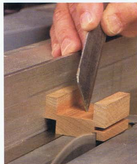
Photo GG • Vertical cuts complete the side rabbets after the channel is cut.
