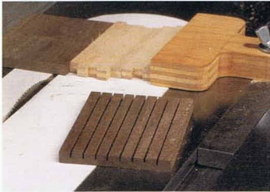
Photo T • To make the consistent parallel cuts that form the “slats” on the panels of beds #1 and #2, use a rip-fence stop and spacer blocks to align the work-piece for the cut. Note: This jig does not guide the workpiece through the cut.
