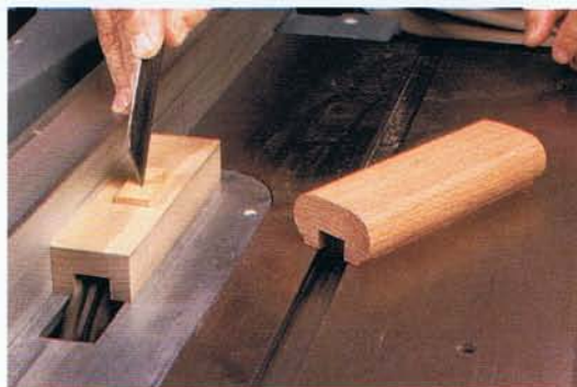
Photo E • Dado cuts in the chassis and tank of the oil tanker body form the channel that accommodates the threaded dowel.
