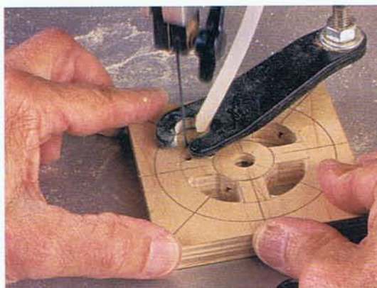
Photo DD • The scrollsaw blade is threaded through the holes to make the internal cutouts in the blanks.
