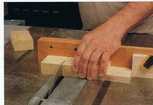
Photo H • To make repeat crosscuts on the table saw, place the stock against the stop block and make an initial cut to square it off flush with the sawblade. Add a spacer block for each subsequent cut.
