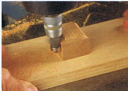
Photo K • Hood #5's recessed top edge curve, with its shallow lip, can be formed either on the overhead router or as a rabbet that is then rounded by hand. This can also be performed on a router table.
