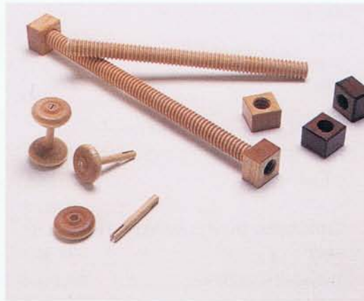
Photo G • The wheels are pressure-fitted to dowel axles. The body parts are aligned on threaded dowels, and secured with wooden nuts.
