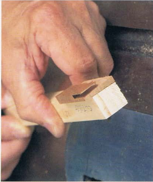
Photo KK • The rear foil's taper is cut with the workpiece fastened to a scrap block with double-sided tape.
