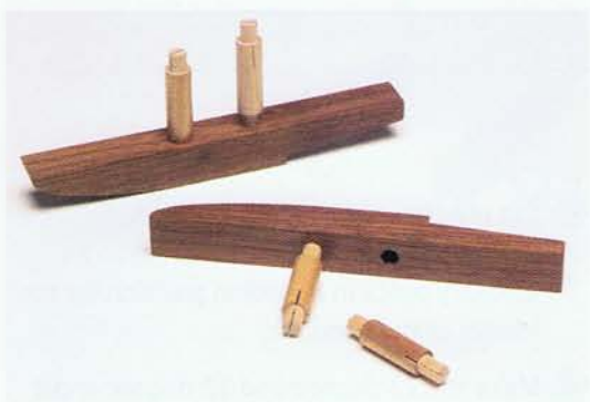
Photo N • Friction-fit struts fasten the pontoons to the undersides of wings.
