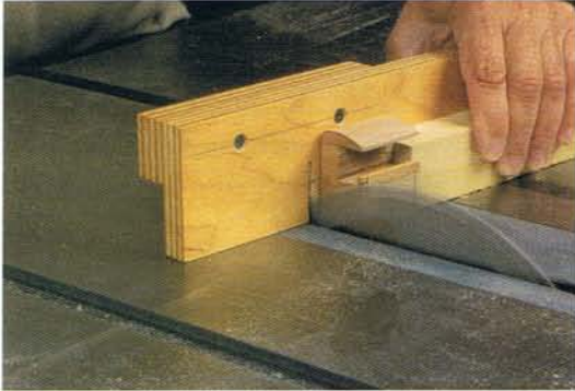
Photo M • To cut the angle on each side of the cab, set the miter gauge to 9 degrees.
