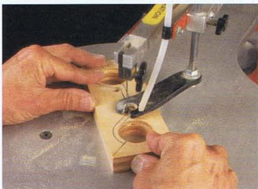
Photo E • Patience is the key to cutting the fender profile accurately and smoothly on the scrollsaw.
