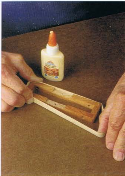
Photo B • A rubber band makes a fine clamp for gluing up the chassis, equalizing the pressure around the perimeter.
