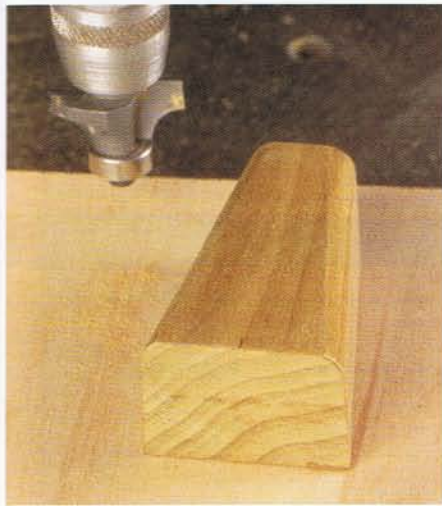
Photo I • The top-edge radius on hoods #1, #2, and #4 is most easily cut with an overhead arm router with a roundover bit.
