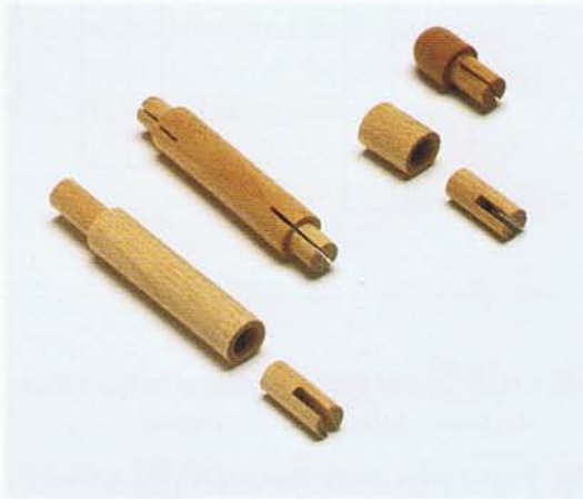
Photo R • Strut shoulders can be formed either on the lathe or by the insertion of a section of smaller diameter dowel.
