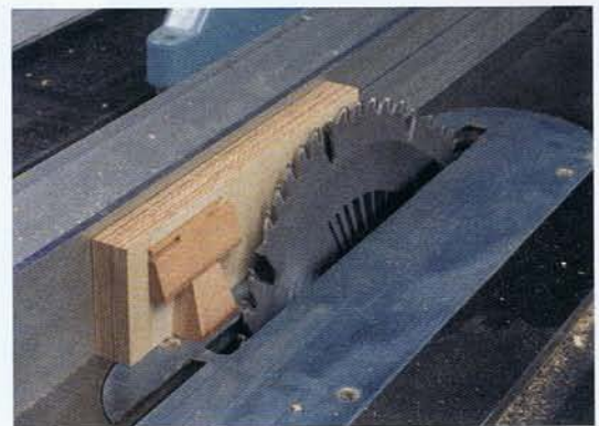
Photo CC • The wing and nose blanks are glued together before being mounted on an auxiliary block for the top angle cut.
