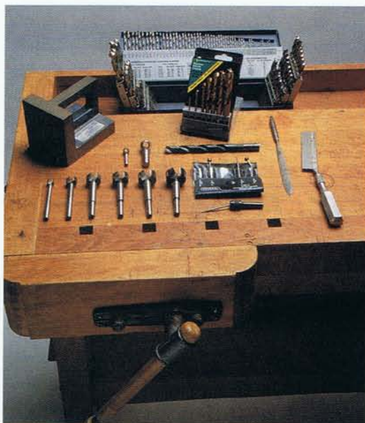
Photo B • Tools that come in handy in making these toys include a complete set of metal drill bits from \frac{1}{16} in. to \frac{1}{2} in., with number bits from 1 to 60 and letter bits from A to Z; a set of brad-point bits from \frac{1}{8} in. to \frac{3}{8} in.; selected Forstner bits; a \frac{3}{64} -in. high-speed steel drill bit; a set of metal-cutting countersinks; a center finder; a right-angle steel block; an X-Acto razor saw; and a letter opener.
