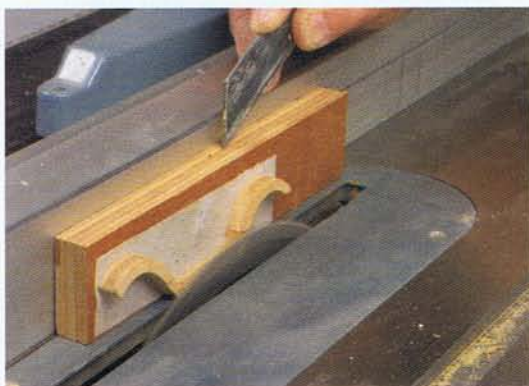
Photo F • An auxiliary block secures each workpiece for cutting the mirror-image fender rabbets. Use a thicker block if you're uncomfortable working this close to the blade.
