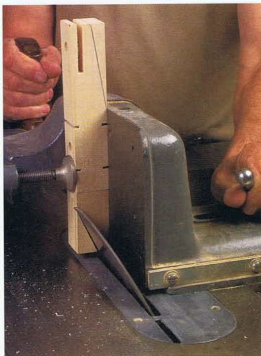
Photo E • The tenoning jig secures the workpiece for the top angle cut on the delta nose block.
