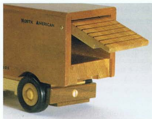
Photo V • The notched-out area in the underside of the van compartment's floor and the recess in the door enable swiveling the door open on its pin hinges with one finger.
