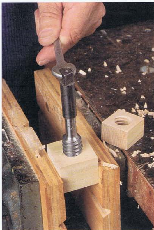
Photo J • Always tap an oversize nut blank, then cut it down to size to reduce the risk of splitting.
