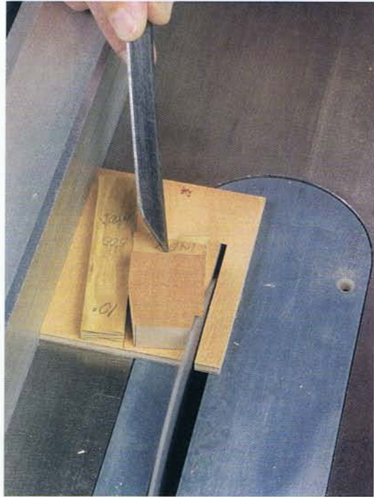
Photo DD • The Indy 500 hood blank has been flipped over in the simple jig for the second side angle cut.
