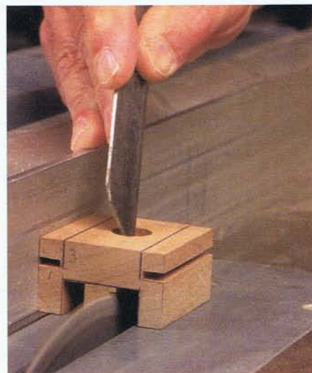
Photo FF • The channel on the underside of cab #9 is formed by a series of parallel cuts on the table saw after the horizontal cuts for the side rabbets have been made.
