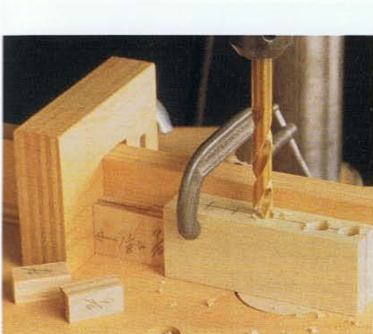
Photo G • Using the spacer-block technique ensures evenly spaced holes.
