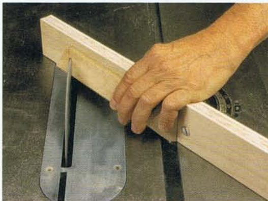
Photo I • Cut the completed dormers off the ends of the blank workpiece. Make sure the auxiliary fence is high enough to accommodate a through cut without jeopardizing its structural integrity.
