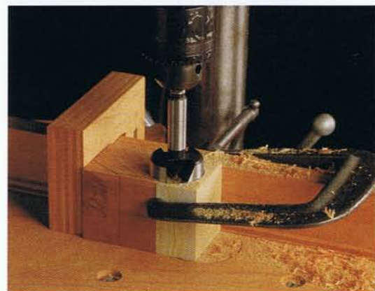
Photo M • When cutting wheel wells, clamp a scrap block to the bottom of the workpiece to give the bit's center some stock to drill into and to prevent tearout along the bottom edge of the vehicle.
