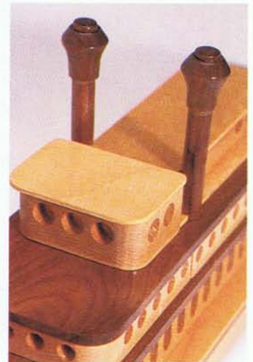
Photo X • The smokestacks pass through three separate components. The receiving holes are \frac{17}{32} in. in diameter to provide a little extra leeway for alignment.
