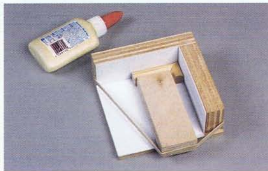
Photo I • A gluing jig for the dowel funnels has plastic strips to prevent the workpiece from adhering to the jig and a rubber band to hold the piece in place at 90 degrees.
