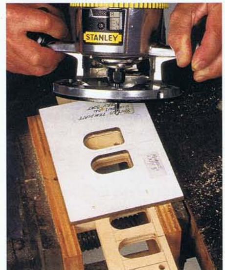
Photo KK • Routing the sidewall apertures is an alternative to the drill and scrollsaw method described in the text.
