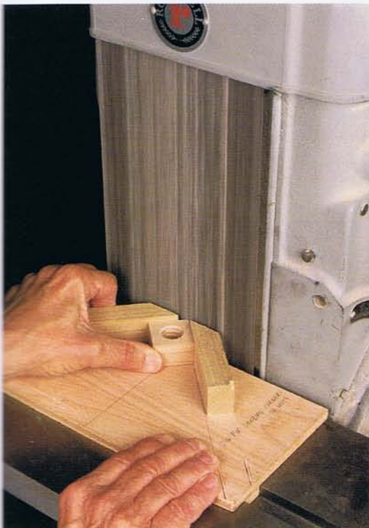
Photo K • A beveling jig for a stationary belt sander gives you a consistent cut on all 12 edges of a square nut.
