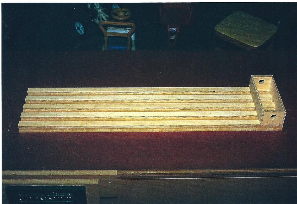
Fig 14.5 Slats secured to the base, with the winch box in position.
