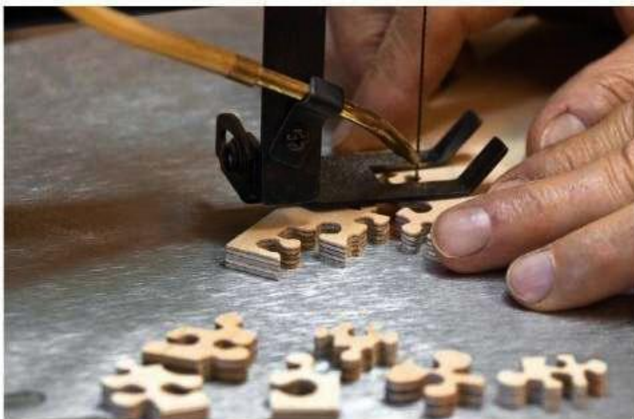
Test scroll saw blades by cutting pieces.
