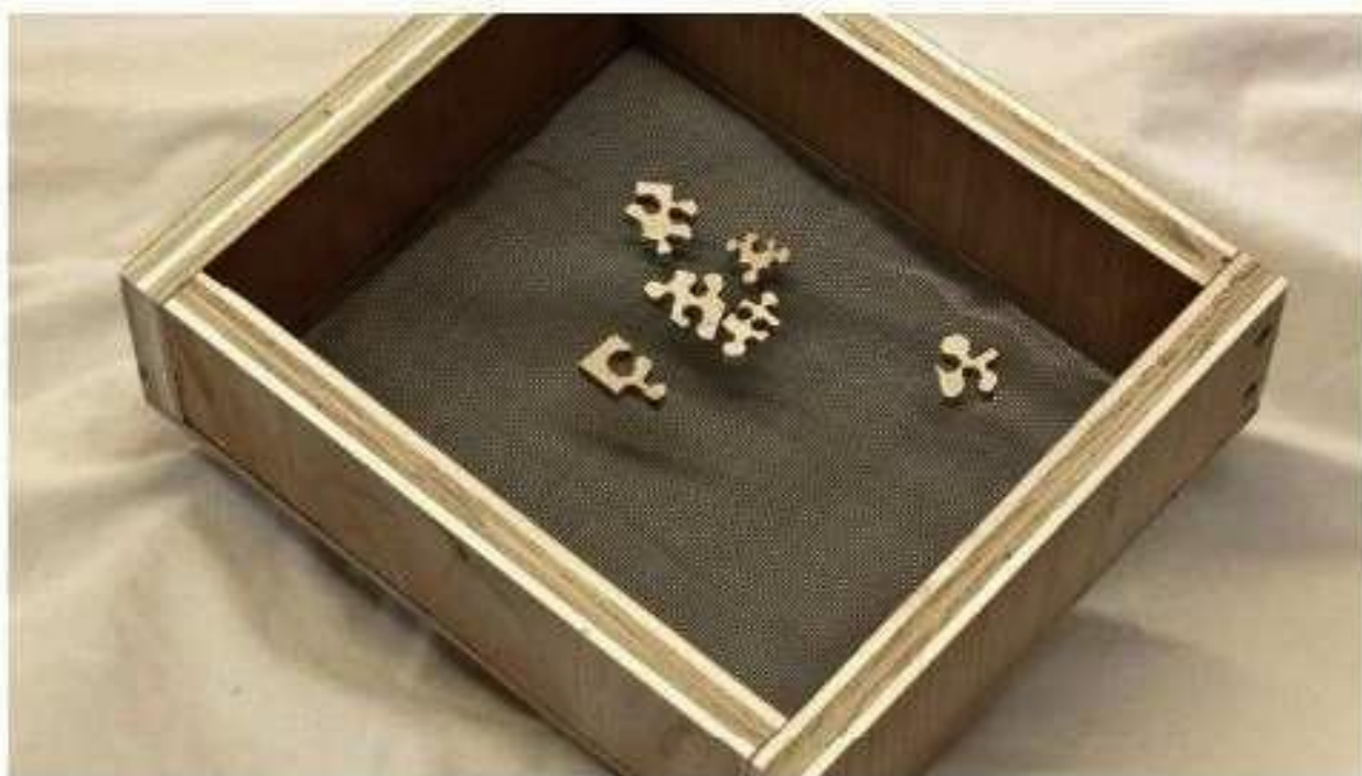
Make a sieve box to vacuum dust from the puzzle pieces.
