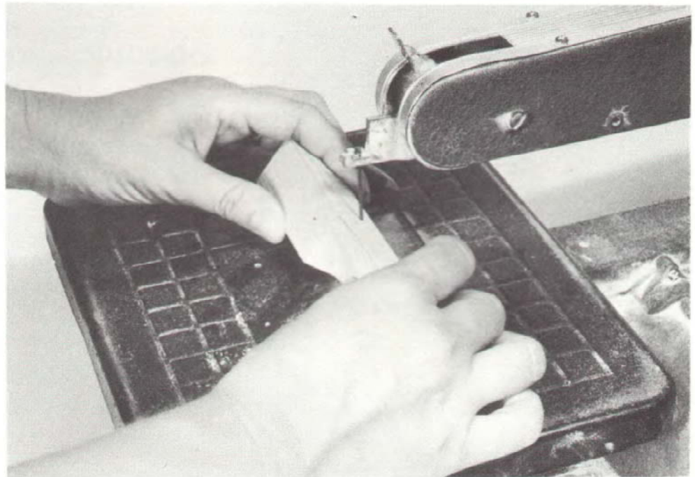
Illus. 12. Cutting off excess from first cut
