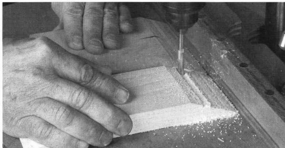
Cut the back-window louvers with a straight router bit on the drill press.
