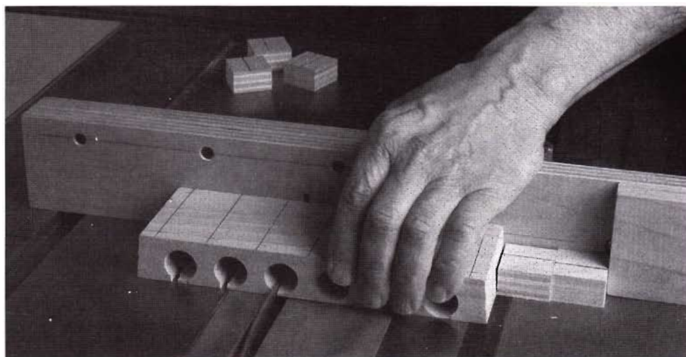
To cut the channels for the seats, make the first series of cuts with the blade slightly offset from the center of the holes (using the same spacer blocks as for drilling the holes).
