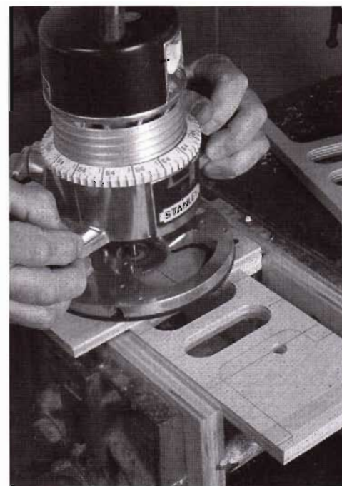
With the template clamped to the workpiece, rout the window opening.
