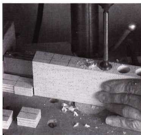
Using 1 1/8-in. spacer blocks, drill holes for the seats in the seating-platform blank.
