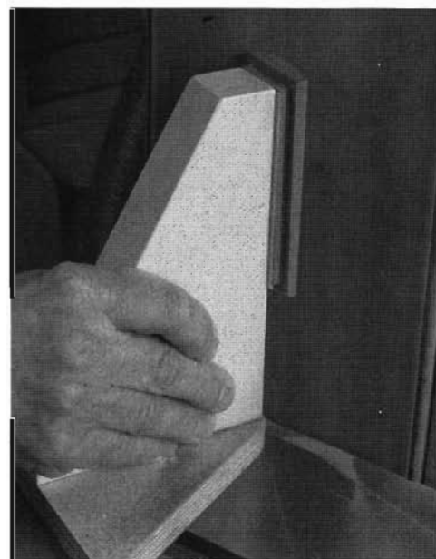
Sand the roof cap to a smooth radius, using a vertical jig for support.
