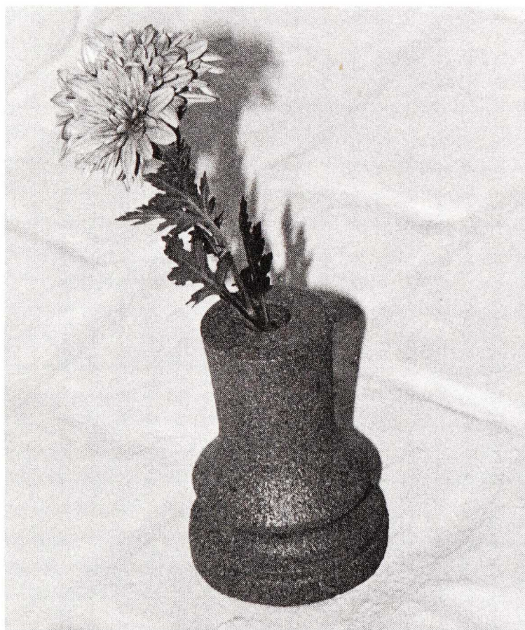
Fig. 10-32. The bud vase is a quick lathe-project. If you plan on showing live flowers, drill the hole to accommodate a small test tube.
