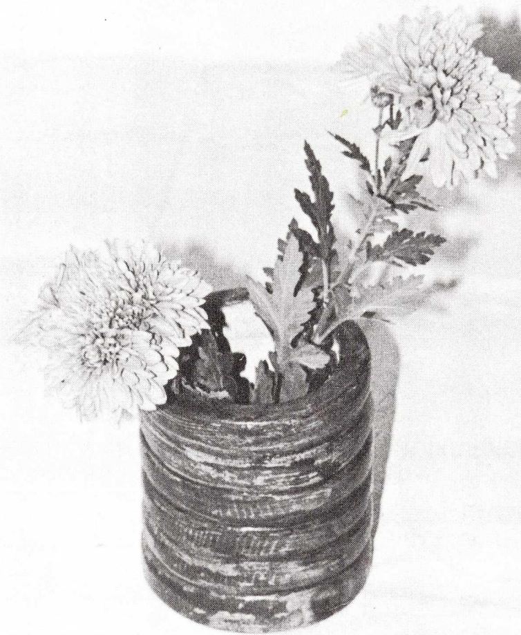
Fig. 10-18. The small vase looks like a lathe turning but is actually a set of wooden rings that were glued together.
