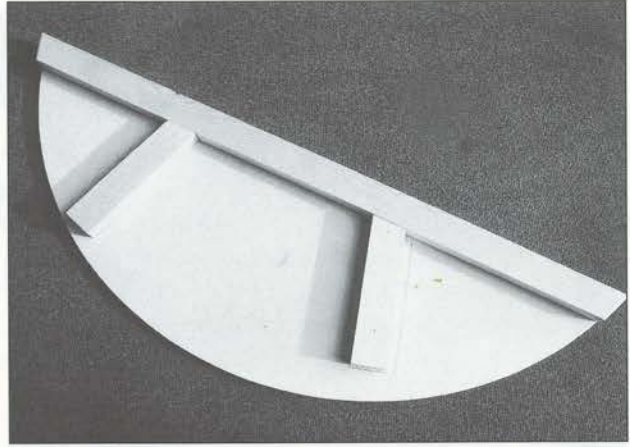
Fig 18.7 Part A with the battens (B and C) glued and screwed into place.
