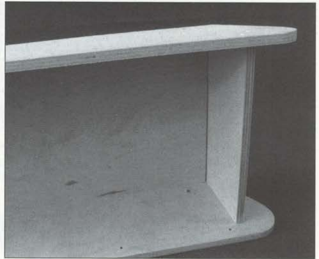
Fig 14.3 The hull sides, ends and base are fastened together.
