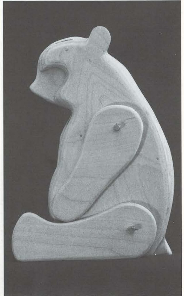
Fig 1.9 Assemble the parts before priming to check for fit.
