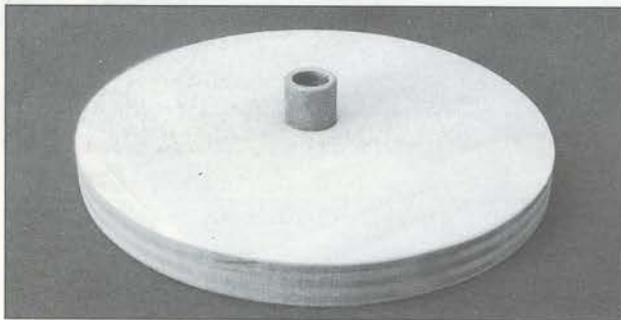
Fig 24.3 The bronze bearing protrudes from the disc.
