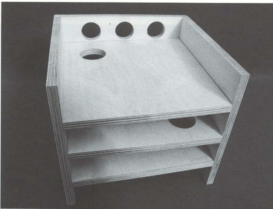
Fig 8.8 The three floors pinned and glued into position on the sides and back.
