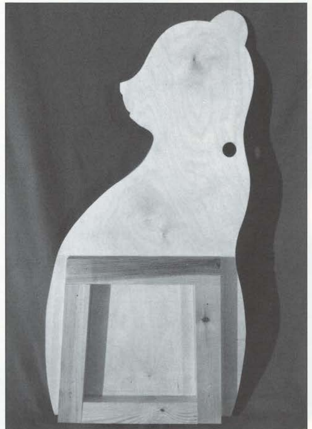
Fig 13.3 Glue and pin the battens to the inner sides.
