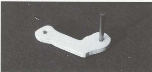
Fig 22.10 Epoxy glue is used to secure the wire into the hole in the arm.
