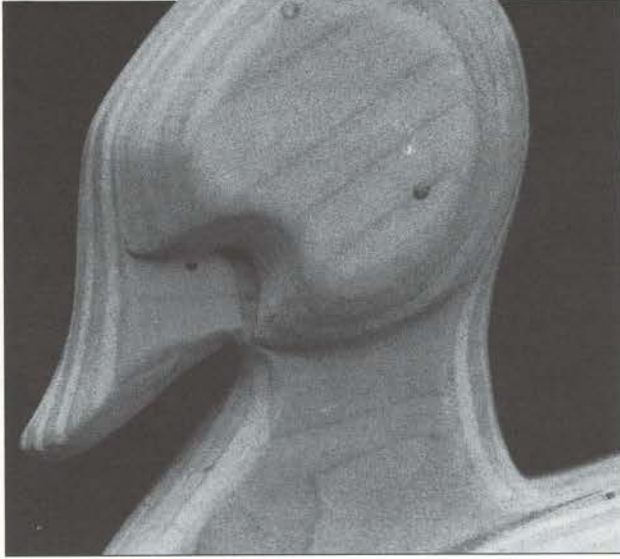
Fig 2.5 The contours of parts D and A have been blended nicely using the rasp and sandpaper.
