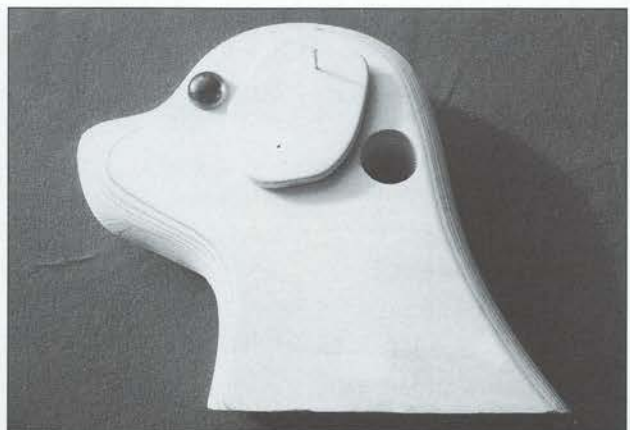
Fig 20.6 The contours of the head are rounded and smoothed with a rasp and sandpaper.
