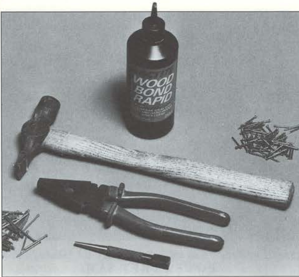
The requisites for securing plywood: a good wood glue, panel pins, a punch, pliers and a light hammer.
