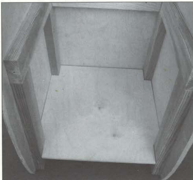
Fig 13.6 The notches in the base fit neatly round the battens.
