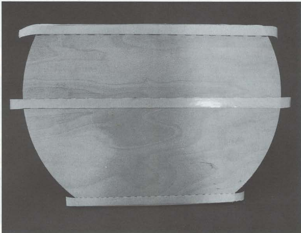
Fig 10.6 Masking tape prevents paint from covering surfaces that later become glue joints.
