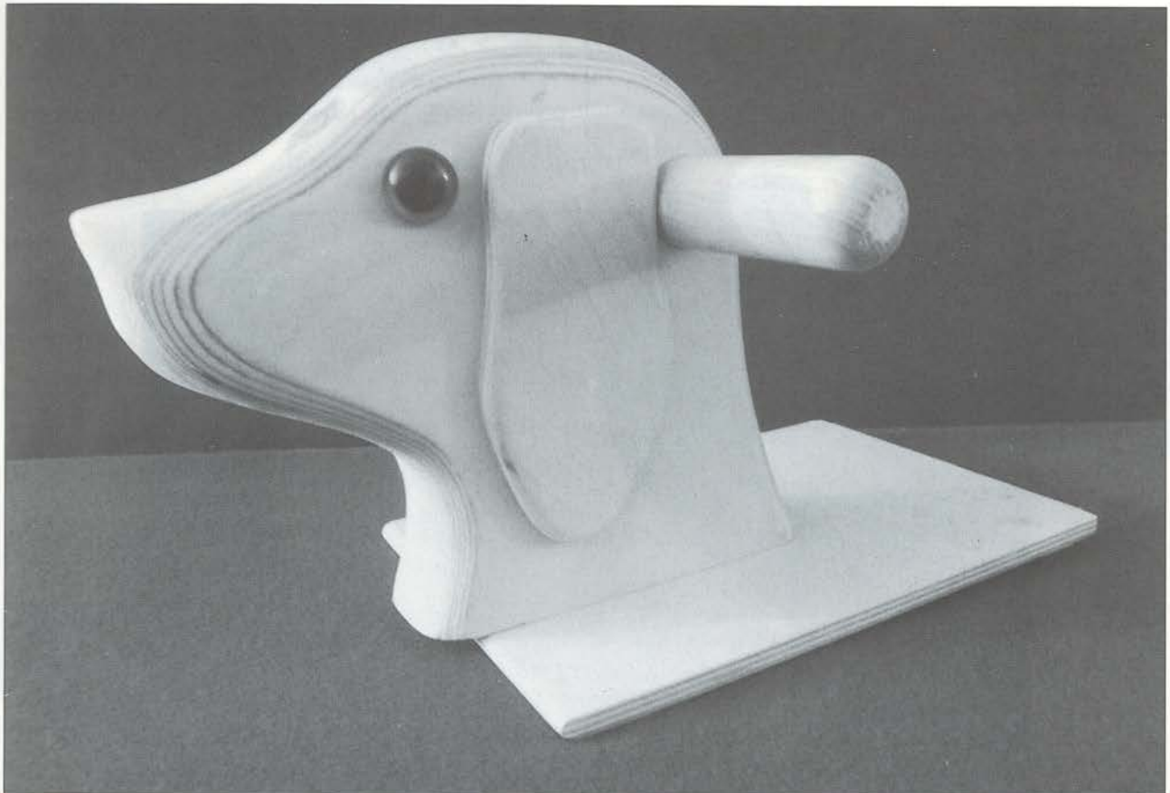
Fig 16.9 The contours of the head are shaped and rounded with a rasp, file and sandpaper.
