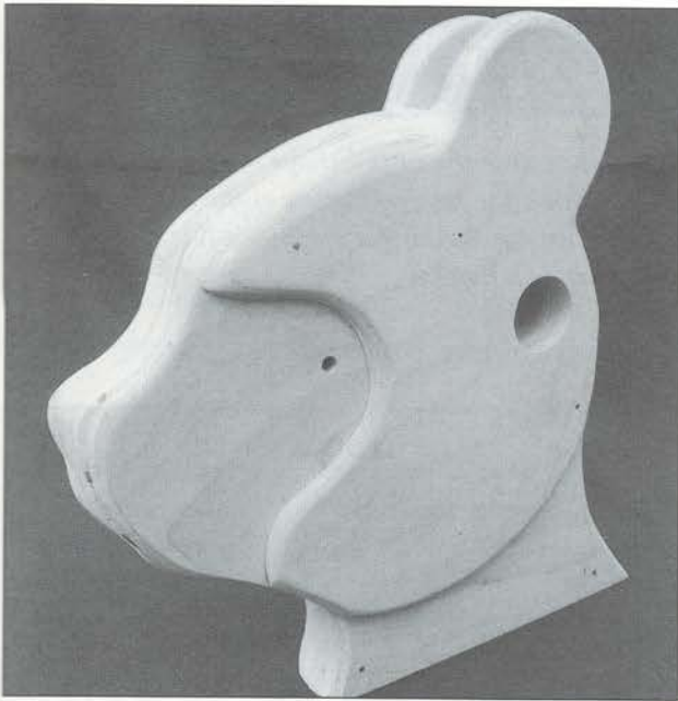
Fig 17.7 Parts E, F, and G form the head. Holes have been drilled for the plastic eyes and the handgrip. Edges have been rounded and smoothed with the file and sandpaper.
