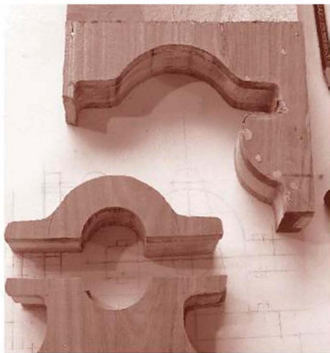
FIGURE 8-3 Secure the sandwich with pins and fret out the form on the scroll saw. Be careful at the end of the cut—when the layers are no longer pinned—that the layers don't slide out of kilter.
