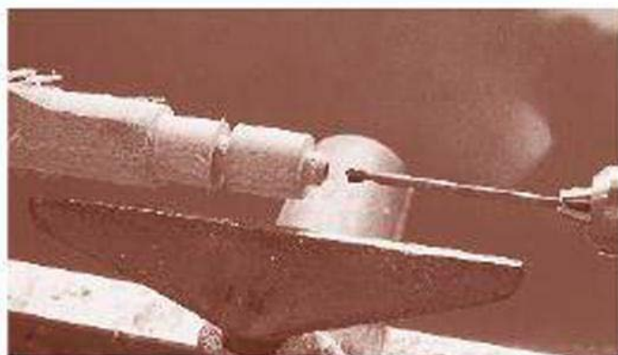
FIGURE 13-7 Fix the bit in the tailstock drill chuck, and run the pivot hole through the length of the turning.
