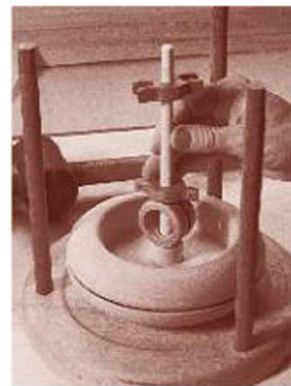
FIGURE 14-18 Slide the ring and the collars in place on the shaft. The top collar needs to be a tight fit.
