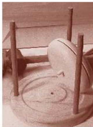
FIGURE 14-18 Ease the bearing hole and the end of the shaft so the whole component spins like a top.
