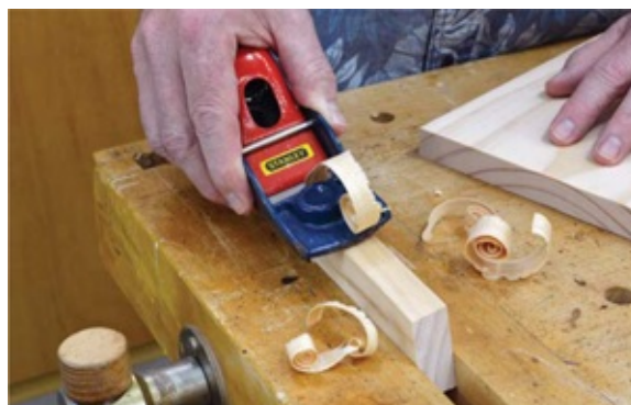
Photo 2 A block plane creates the bevel on the bookrack support foot.
