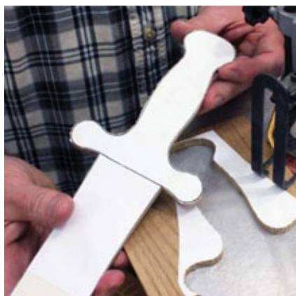
Photo 5 Saw just shy of the line; sanding will refine all the curves.
