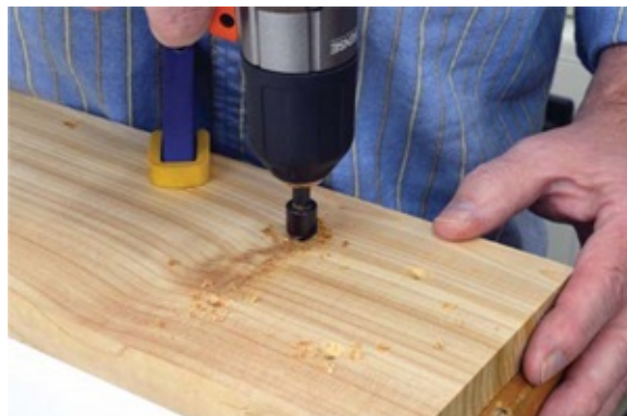
Photo 8 Flip the back piece over and countersink the pilot holes from the back.
