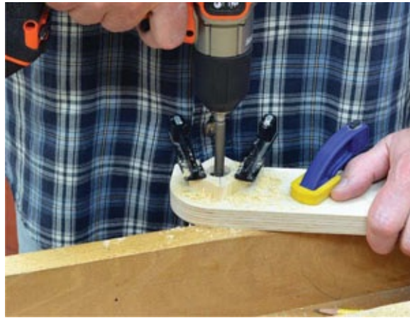
Photo 11 Drill a \frac{3}{4} " hole through the mouthpiece section.
