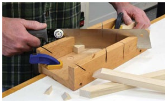
Photo 1 A miter box and fine-cut saw team up to create perfect 45° angles for the frame members.
