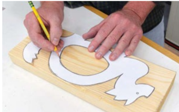
Photo 2 Copy and print out the pattern, and then attach or trace it onto one side of the workpiece.
