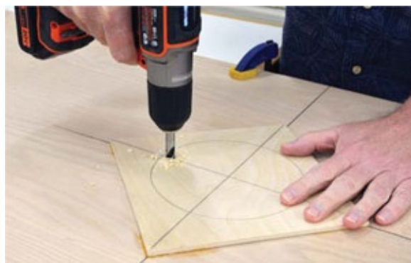
Photo 4 Drill a \frac{1}{2} " pilot hole as a starting point for cutting.
