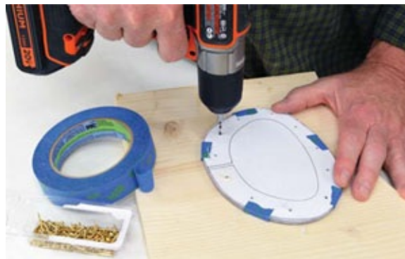
Photo 8 Stack the two clear side pieces and drill the pilot holes for the escutcheon pins.
