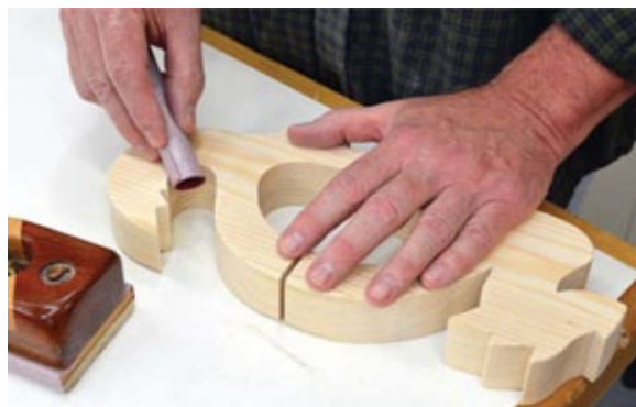
Photo 4 Give the workpiece a thorough sanding; a rolled-up piece of sandpaper reaches into the tight spots.
