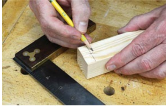
Photo 1 Mark the end of the workpiece with a cut line, plus a distinctive mark to make it easy to reattach the piece later.
