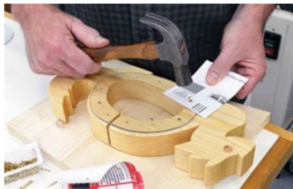
Photo 9 Hammer in the escutcheon pins to attach the clear sides.
