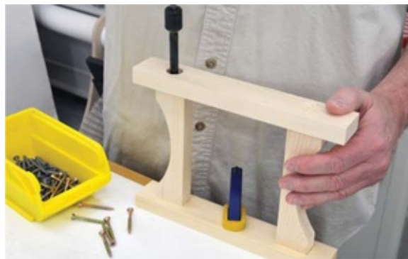
Photo 5 Countersink pilot holes for the screws. One of these will go right in the handle hole on each side.
