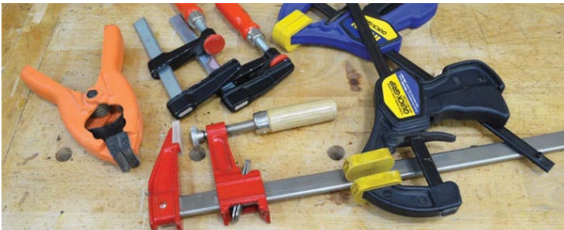
As the old woodworking adage goes, you can’t have enough clamps. (clockwise from left) Spring clamp, small F-style bar clamps, one-handed bar clamps, long F-style bar clamp.
