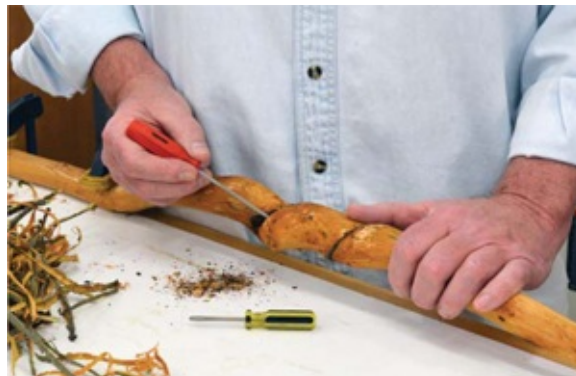
Photo 4 A narrow tool, like this small screwdriver, digs debris out of the fissures caused by the vine.
