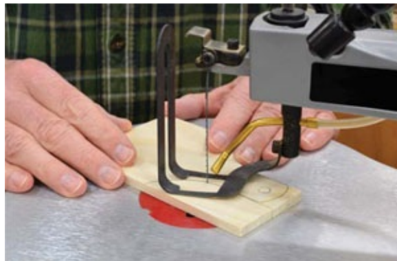
Photo 9 Cut out the counterweight box sides with a coping saw or, as here, a scroll saw.
