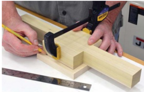
Photo 2 Using a piece of the same material as a spacer, trace the outline of where the sides will fit onto the bottom.
