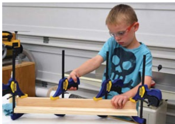
Photo 4 Assembling the leg components in an “L” shape makes for a sturdy workbench.
