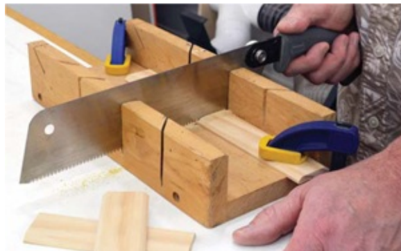
Photo 5 Cut the handle pieces squarely to length in a miter box. A fine-cut saw like this will ensure smooth, clean edges.
