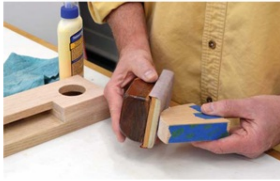
Photo 8 Tape the two supports together and sand both at the same time.
