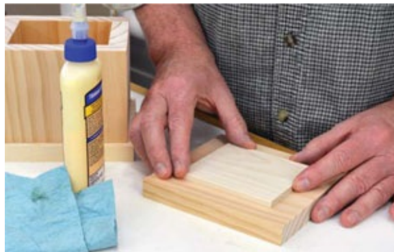
Photo 8 Center the lid keeper underneath the lid, and glue it into place.
