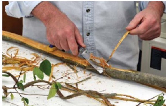
Photo 3 Remove the bark with a scraper or, as here, a putty knife.
