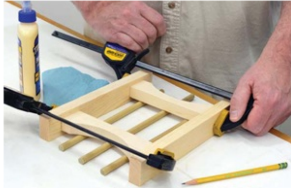
Photo 4 Some \frac{3}{8} " dowels help to center the spindles during assembly.
