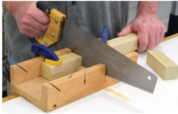
Photo 1 Cut the two side components squarely with a handsaw and miter box.
