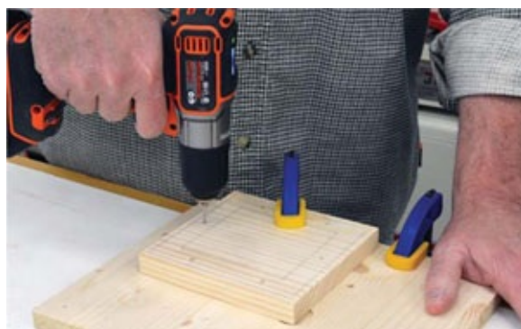
Photo 5 Use your penciled lines to place pilot holes in the center of the traced outline.
