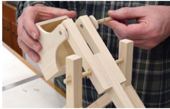
Photo 19 Hold the weight box in place and slide in the axle dowel.
