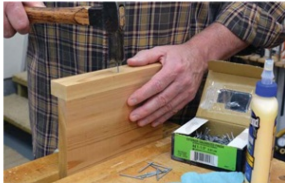
Photo 3 Nail on the shelf back. For outdoor structures like this always use water-resistant or waterproof glue and galvanized nails.
