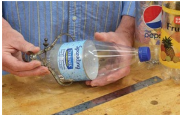
Photo 1 The bottle diameter is the most important dimension when sizing component parts.
