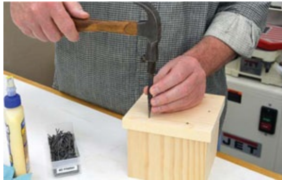
Photo 7 Use a nail set to drive the nail heads slightly below the wood's surface.
