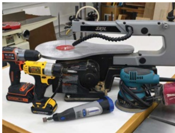
Kid-friendly power tools include (clockwise from top) a small scroll saw, sander, rotary tool, dedicated power screwdriver and a drill/driver.
