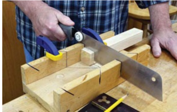
Photo 2 Cut off the end squarely to create the whistle mouthpiece. A fine-cut saw makes for a clean cut.
