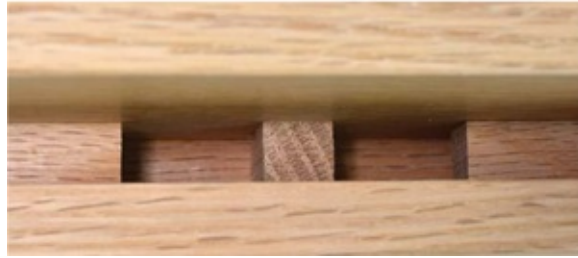
Photo 11 This inside view shows the sound channel openings.
