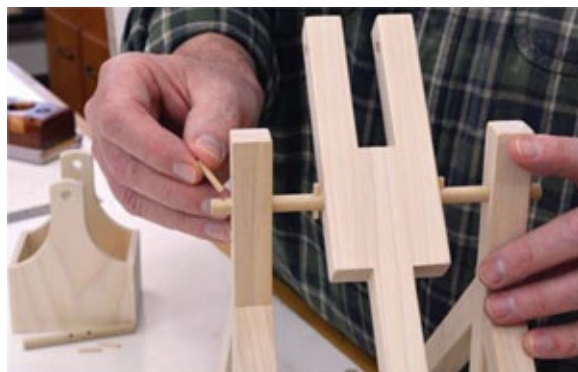
Photo 15 With the beam axle in place, secure it with \frac{3}{4}" lengths of \frac{1}{8}" -diameter dowel pins.
