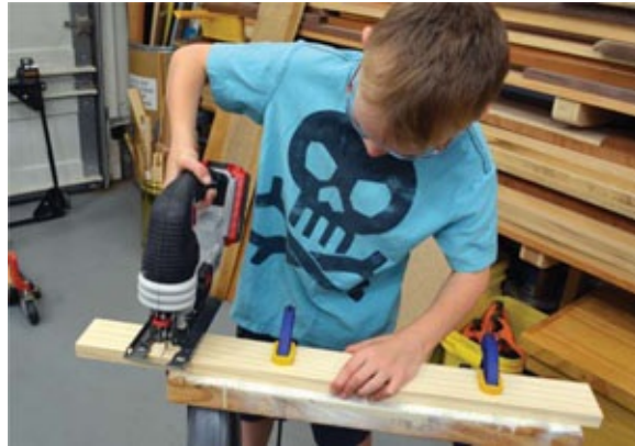
Photo 2 Whenever possible, clamp workpieces securely before cutting to make the task easier and safer.
