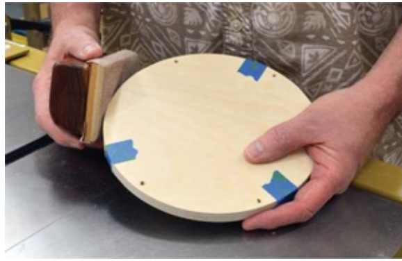
Photo 3 With the circles cut out, give the edges a good sanding, then untape and sand the faces.
