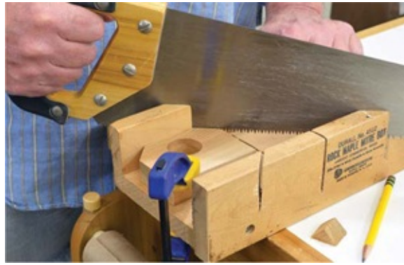
Photo 4 Clamp the work inside a miter box to trim the corners of the bottle support.
