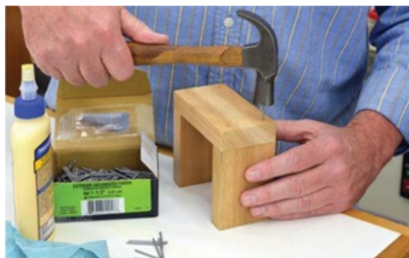
Photo 5 The upper bottle holder goes together with waterproof glue and nails.
