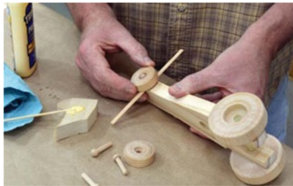
Photo 8 A spacer helps to get the front wheels installed the same distance on both sides of the racer.
