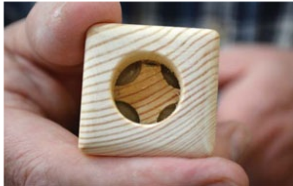
Photo 14 In this close-up, you can see how the air goes over the diverters.
