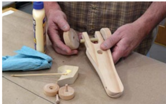
Photo 5 To prevent binding the axle, be sparing with the glue when attaching the rear wheels.
