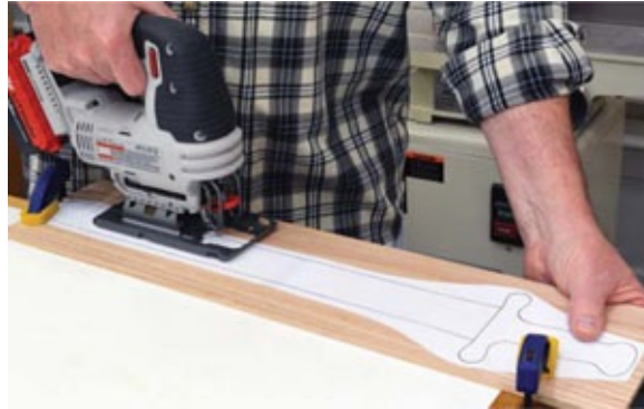
Photo 3 With the workpiece clamped securely, cut out the straightest portions of the pattern with a jigsaw.
