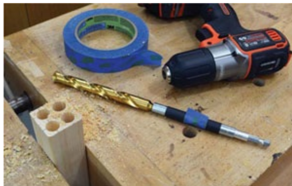
Photo 7 A drill extension allows you drill holes deeper than the drill’s actual length.
