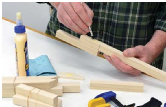
Photo 2 Apply glue to the side beams and clamp them to one end of the main beam.
