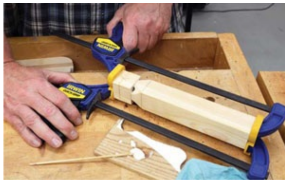
Photo 12 Line up your marks, then glue and clamp the mouthpiece back onto the workpiece.
