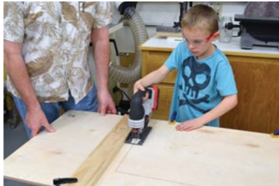
Photo 6 A clamped-on guide helps make perfectly straight cuts in the plywood workbench top.
