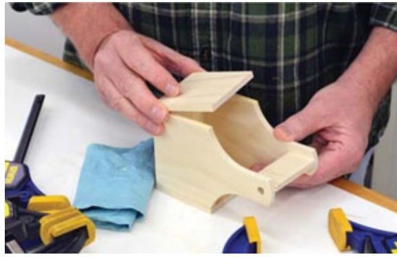
Photo 12 When the bottom has dried, glue and clamp the counterweight box ends in place.
