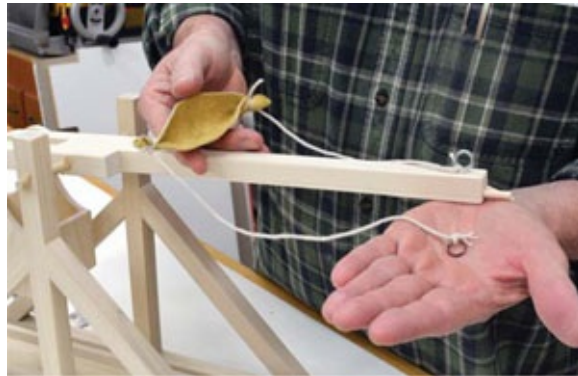
Photo 20 Tie one end of the sling to the screw eye on the beam. A ring or loop hooks onto one of the release pins on the end of the beam.
