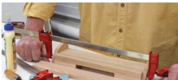
Photo 9 Line up the supports with the speaker top and front, then glue and clamp them into place.
