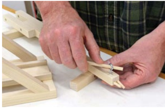
Photo 17 A dowel scrap – or even a pencil – makes a good tool to set screw eyes to the proper depth.
