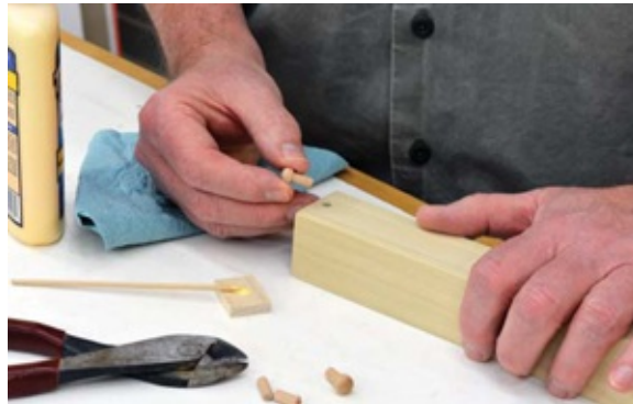
Photo 7 Trim a couple of toy axles and glue them in place to act as stops for the candy slide.
