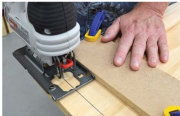
Photo 1 For a perfectly straight cut on the workpiece ends, a clamped-on guide ensures exact control of the jigsaw.
