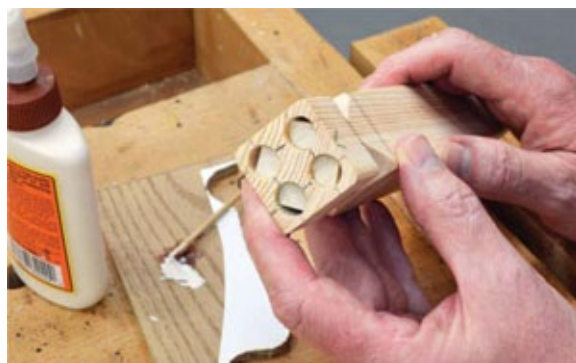
Photo 10 Glue the air diverters into the sound holes ⅛" from the top.
