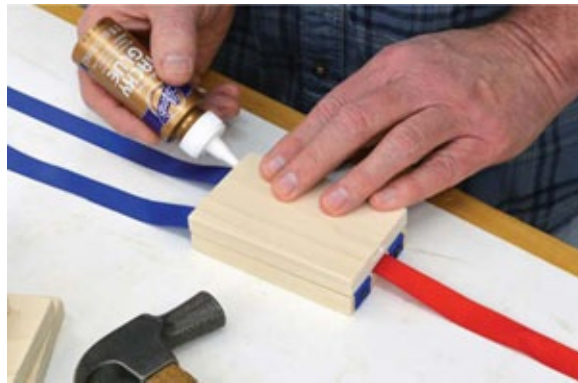
Photo 7 Lay the second block atop the first, and apply glue on the ends above the ribbons.
