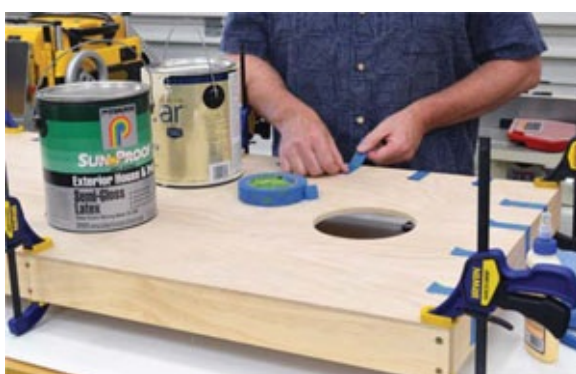
Photo 10 Never enough clamps! Tape stretched over the edges of the game board will hold everything in place until the glue dries.
