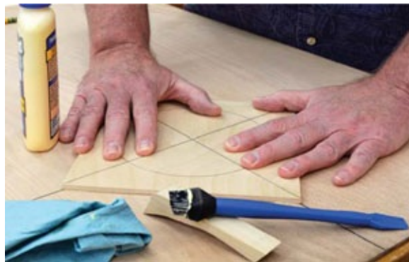
Photo 3 Match the guidelines on the board to those on the back of the reinforcement.
