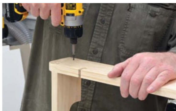
Photo 5 Reinforce the assembly by countersinking pilot holes and driving in 1- 5 / 8 ” screws.
