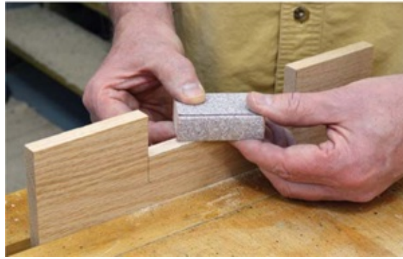
Photo 2 Sandpaper wrapped around a wood block quickly squares and smooths the cut opening.
