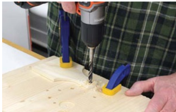
Photo 10 Drill the axle holes for the counterweight box sides with a \frac{5}{16} " bit.
