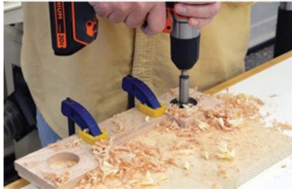
Photo 3 Clamp the speaker front to scrap and drill both speaker openings. A Forstner bit is perfect for this.
