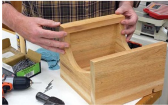
Photo 10 Line up and attach the shelf front with glue and nails, and the nesting shelf is complete.
