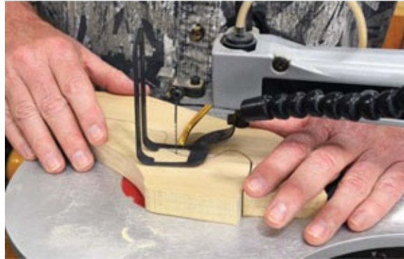
Photo 3 A scroll saw makes fast work of cutting out the shooter, but you could also use a coping saw.
