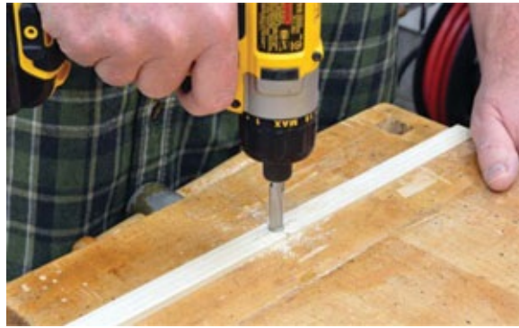
Photo 6 When the glue has thoroughly dried, countersink a pilot hole beneath the frame side and drive a 1- \frac{5}{8} " screw up into the vertical.
