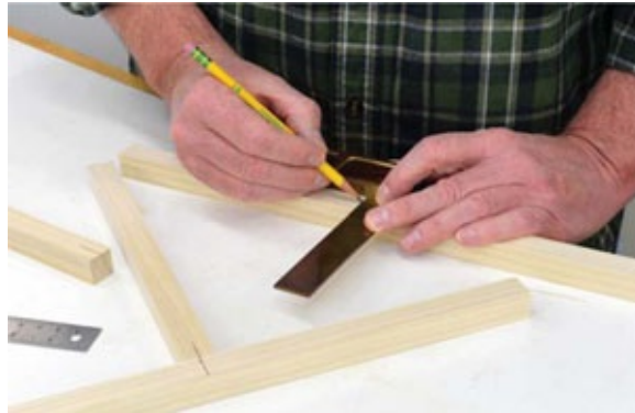
Photo 4 Begin frame assembly by marking the centers of the frame side pieces.
