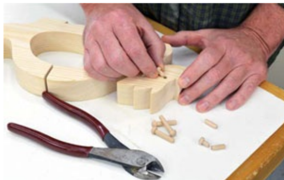
Photo 7 Trim the toy axles and glue them into the eye holes.
