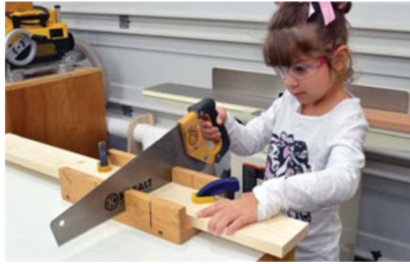
Photo 1 To make it easier for kids to saw, securely clamp the miter box and workpiece to a sturdy worksurface.
