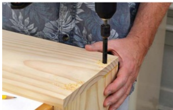
Photo 5 To keep the screws hidden in the finished bookrack, start by drilling countersunk pilot holes about \frac{1}{4} ” deeper than normal.
