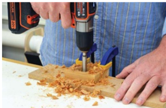
Photo 3 Drill the hole for the bottle support with a spade bit or, as shown here, a Forstner bit.
