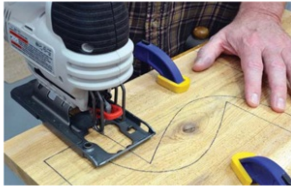
Photo 2 With the workpiece securely clamped, cut out the two sides of the nesting shelf.
