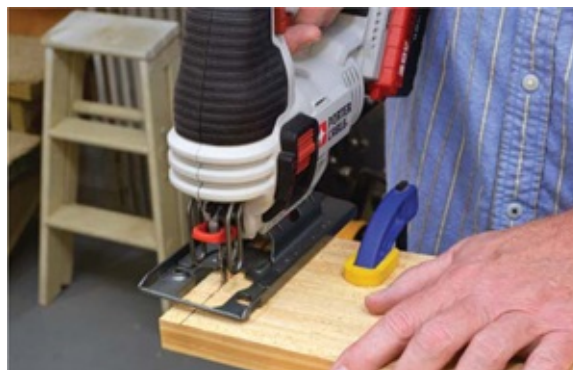
Photo 2 Clamp workpieces securely when cutting to length.
