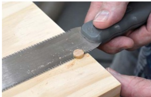
Photo 8 Trim off the excess plug, then sand everything smooth. Once painted, those plugs will disappear.
