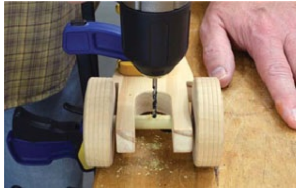
Photo 7 Drill a \frac{1}{8} " hole into the center of the rear axle for the rubber band's axle peg.
