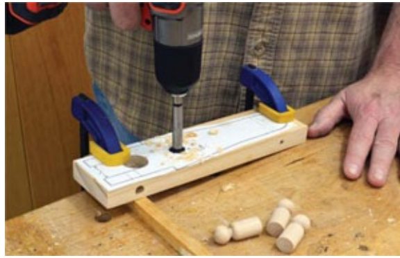
Photo 2 A \frac{5}{8} " Forstner bit or spade bit creates the hole for the driver. Tilting the workpiece makes it easier to drill the angled hole.
