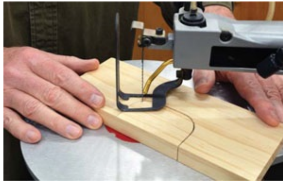
Photo 1 Cut out the goal opening with a coping saw or, as here, a scroll saw.
