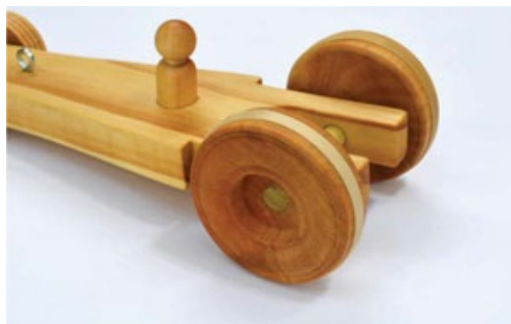
Photo 9 A wide rubber band stretched over the rear drive wheels provides traction on smooth floors.
