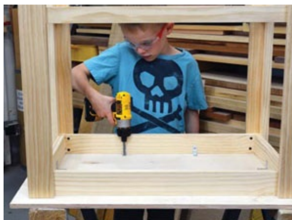
Photo 8 Simple metal brackets secure the leg set from underneath the plywood top. Be sure to use short screws that won't go all the way through the plywood.
