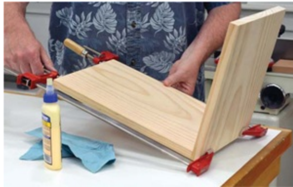
Photo 4 Clamp up the assembly until the glue dries.
