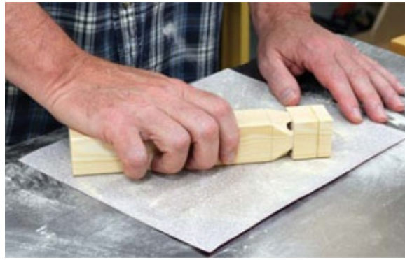
Photo 13 When the glue dries, give all four sides a good sanding.
