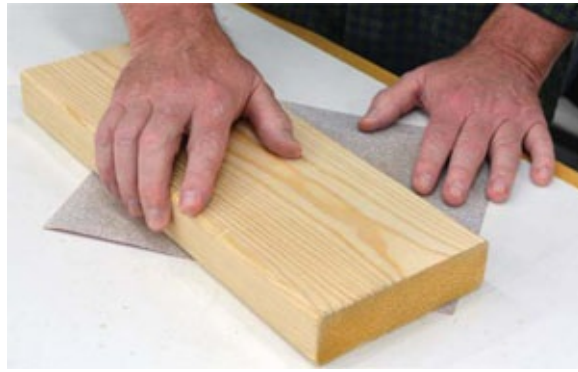
Photo 1 Flatten the workpiece by sliding it over a piece of sandpaper held on a flat surface.
