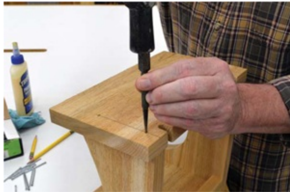
Photo 7 Use a nail set to drive the heads of the nails just below the surface.
