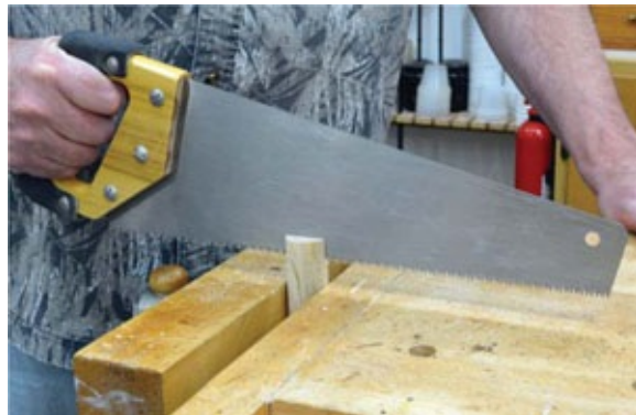
Photo 4 Cut a 1- \frac{1}{8} " dowel right down the middle to create the shooter "cylinder."
