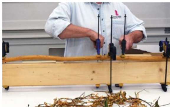
Photo 5 Clamped firmly to this length of 2x6, the sapling will straighten as it dries.
