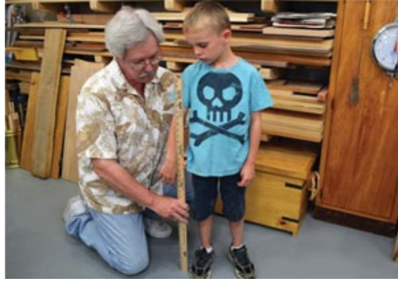
Photo 1 A good height for a workbench is the distance from floor to wrist.
