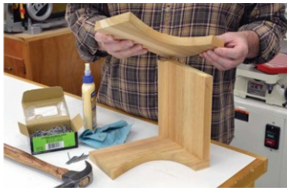
Photo 4 Attach the two sides to the completed shelf bottom with glue and nails.
