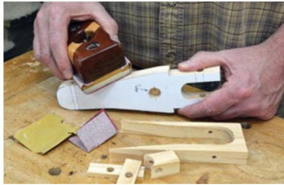
Photo 4 Sand all the freshly cut edges smooth with a sanding block.
