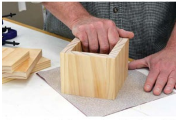
Photo 3 Sanding the box on a sheet of sandpaper held to a flat surface cleans up the bottom edge to prepare for gluing the bottom into place.
