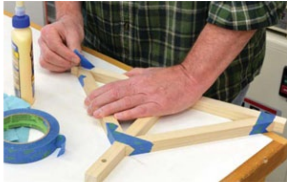
Photo 7 Apply glue to the ends of the frame diagonals, and tape them tightly in place until dry.
