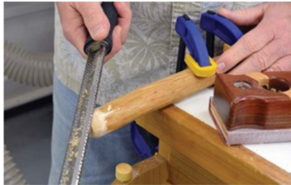
Photo 7 Use any combination of file, rasp or sanding block to round over the cut ends.
