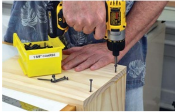
Photo 6 Drive the screws home, setting them \frac{1}{4} " below the wood surface.
