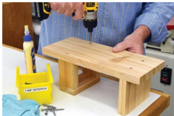
Photo 9 Assemble the feeder by driving exterior-grade screws through the back.
