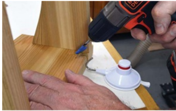
Photo 9 To prevent drilling all the way through the roof, mark your drilling depth with masking tape right on the drill bit.
