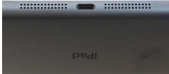
Photo 12 The iPad Mini has two speakers that fit over the sound channel openings inside the assembly.
