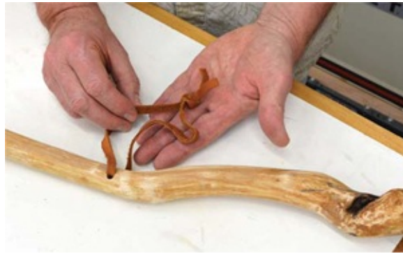
Photo 10 To create the wrist strap, pass the cord through the drilled hole, then knot it securely.
