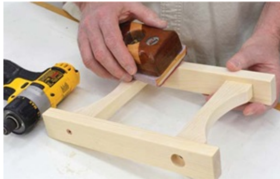
Photo 7 Give the winder a good sanding all around, making sure to round over the front edges of the string spindle.
