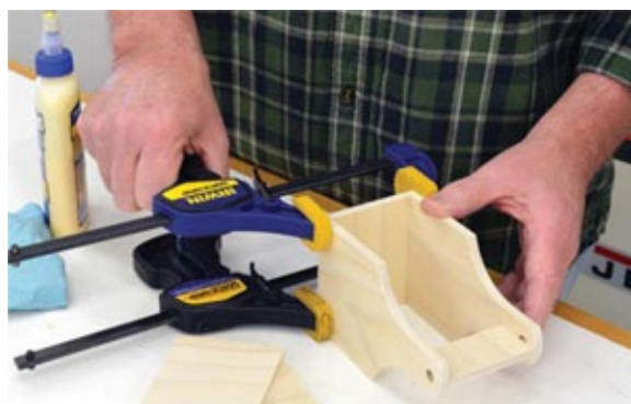
Photo 11 Glue and clamp the bottom of the counterweight box between the two sides. A piece of scrap acts as a spacer at the top.
