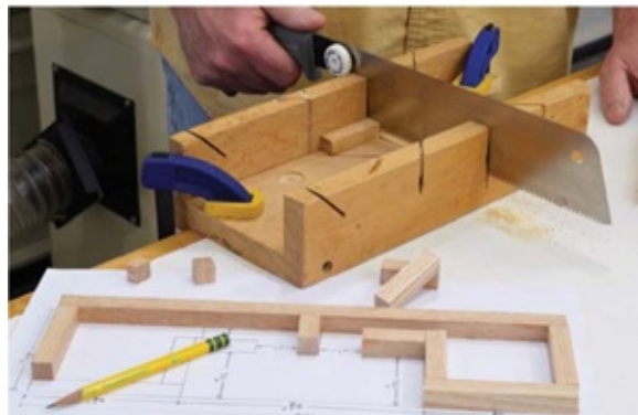
Photo 4 As you cut the spacers for the interior of the speaker, keep things in order by arranging them on the pattern.
