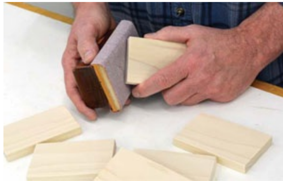
Photo 1 Sand each block smooth and use the sanding block to lightly round all edges.
