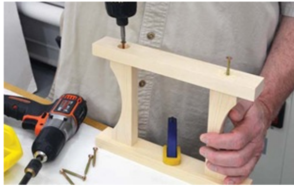
Photo 6 Drive screws in place to reinforce the assembly.
