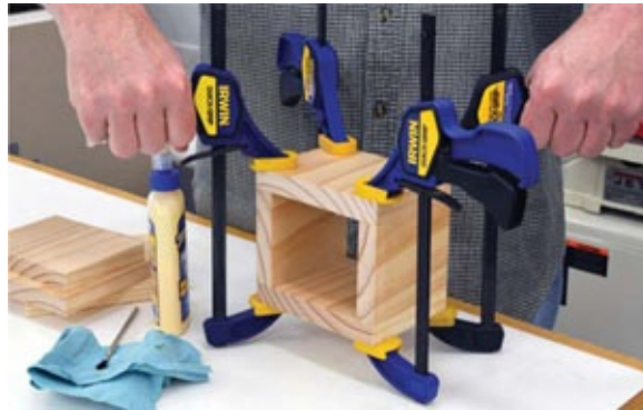
Photo 2 Clamp the box assembly until the glue dries.
