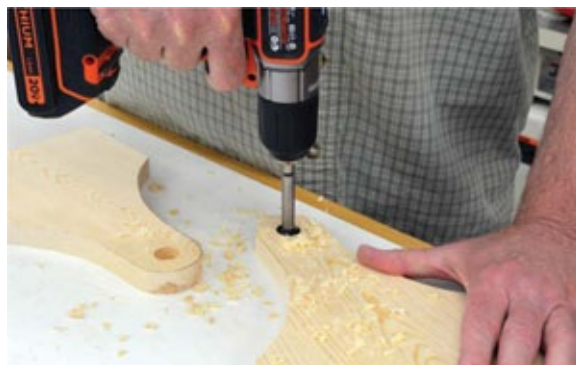
Photo 5 Forstner bits are perfect for drilling stopped holes in the toolbox ends.
