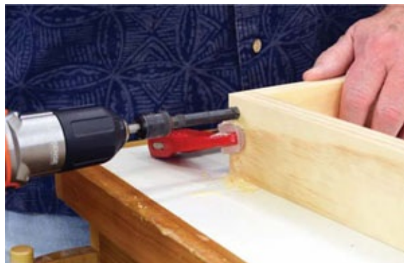
Photo 8 Countersunk pilot holes will allow screws to set flush against the wood.
