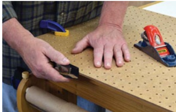
Photo 2 Cutting pegboard can leave a rough edge, but a small plane or a sanding block will smooth the soft material quickly.
