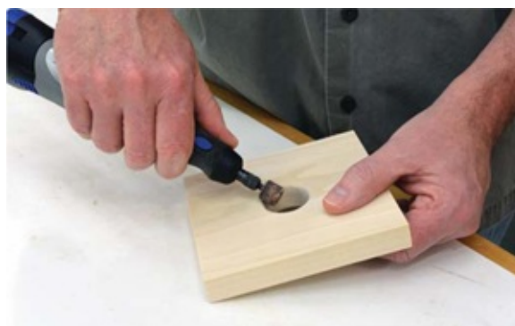
Photo 5 Round over the edges of the top hole with a rotary tool, or by hand with rolled up sandpaper.
