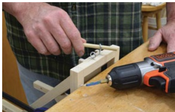
Photo 18 Twist the screw eyes into the frame so the holes are aligned.
