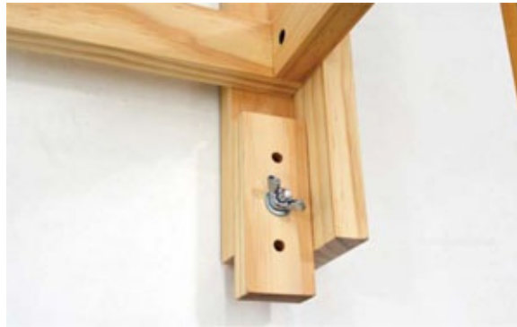
Photo 10 Plan for the future with leg extenders to raise the workbench height as your little woodworker grows.
