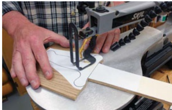
Photo 4 For the tightly curved sword hilt, a scroll saw will do a better job than the jigsaw.
