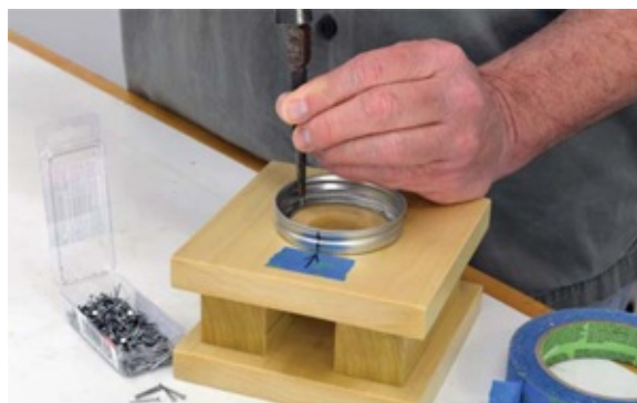
Photo 10 Use a nail set to drive \frac{5}{8} " nails to secure the inverted jar lid in the center of the dispenser top.
