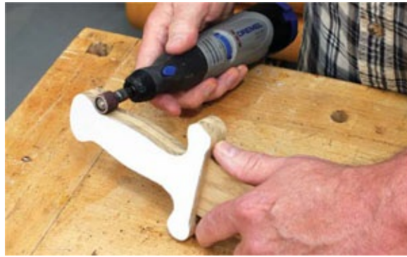
Photo 8 A rotary tool outfitted with a sanding drum quickly smooths the curved sections of the sword.
