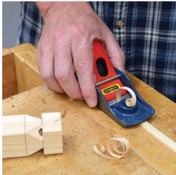
Photo 9 Remove ⅛" of material from a dowel to create the air diverters.
