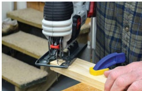
Photo 3 Cut the curve at the bottom of the frame sides with a jigsaw.
