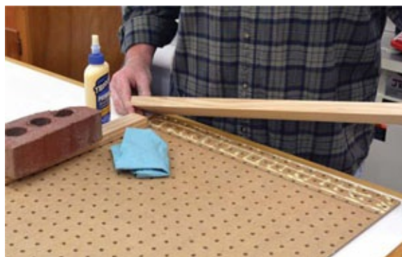
Photo 4 Pegboard glues very securely to bare wood, so no other fasteners are required. The brick is being used to clamp one of the frame pieces.
