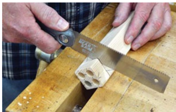
Photo 8 Cut the whistle opening notches carefully; a fine-cut saw is best.
