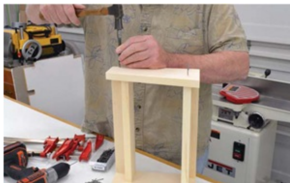
Photo 5 When the glue has dried, reinforce the display shelf with 4d finish nails and countersink them.
