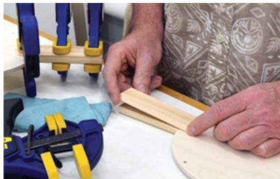
Photo 7 Glue the first half of the handle assembly to the paddle, then add the other handle side.
