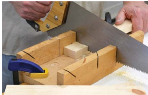
Photo 1 Cut all the parts except the handles from standard 1x2 pine.
