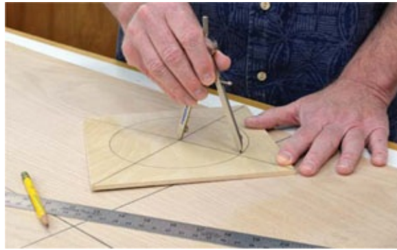
Photo 1 A compass and ruled guidelines help to accurately place the hole reinforcement.
