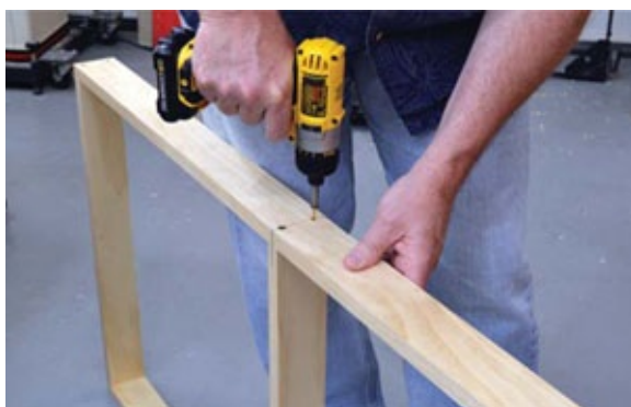
Photo 9 A pair of screws in the center of each side completes the frame.
