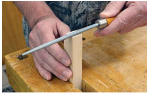
Photo 6 Use a round file to form a small notch for the rubber band to hook into.
