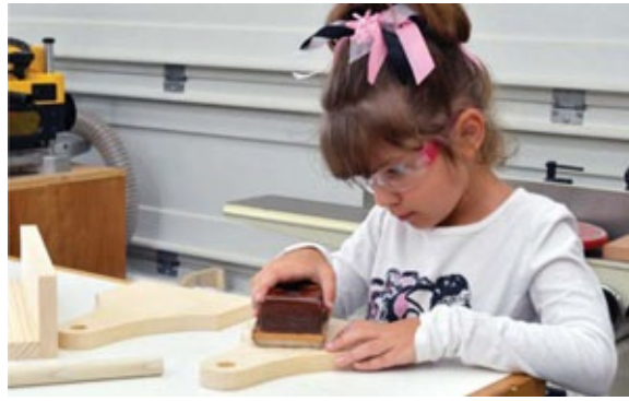
Photo 6 Sanding before assembly is always easier and more efficient.
