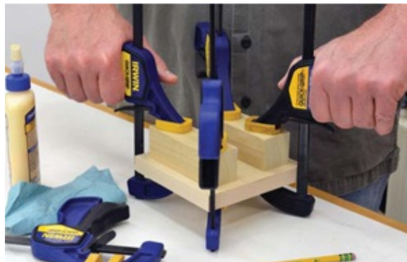
Photo 3 Glue and clamp the two sides into place on the bottom piece.
