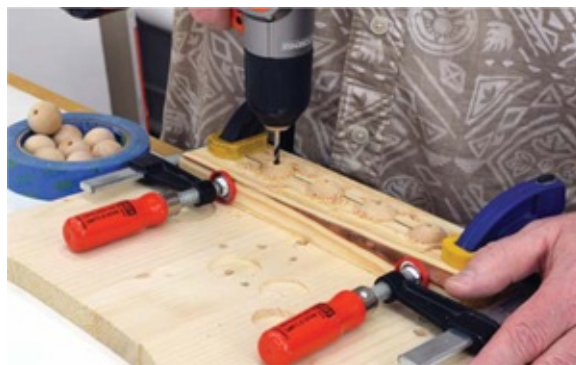
Photo 8 Secure the wooden balls in the drilling jig clamped to your worksurface, and drill holes all the way through.
