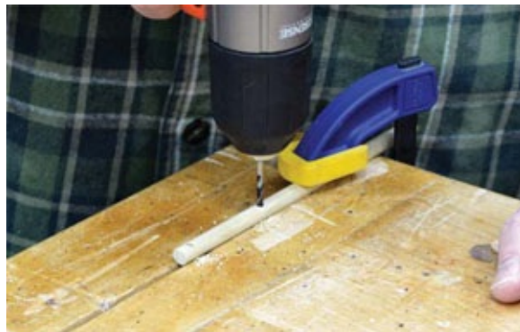
Photo 14 Drill \frac{1}{8}" holes through the beam axle dowel for the axle pins.
