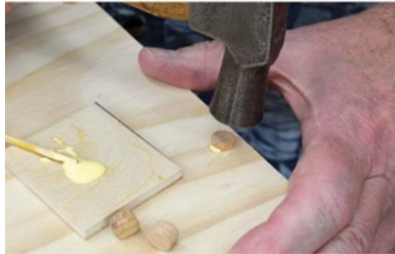
Photo 7 With a bit of glue in the countersink, tap in wooden plugs to hide the screw heads.
