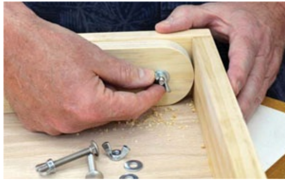
Photo 14 Wing nuts on each side can be tightened to hold the legs securely in either the open or closed position.
