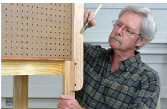
Photo 6 You can leave the rack's wood frame plain, or give it a few protective coats of polyurethane varnish.
