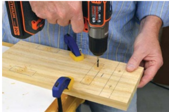
Photo 7 Drill pilot holes in the feeder back piece using your penciled guides on the front side.
