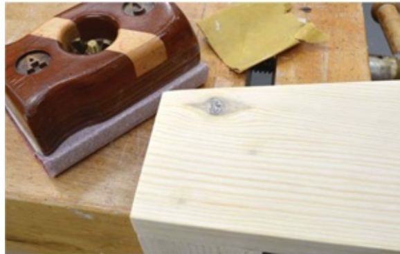
Photo 7 When the wood filler has dried, sand smooth. Those spots will disappear when you paint the shelf.
