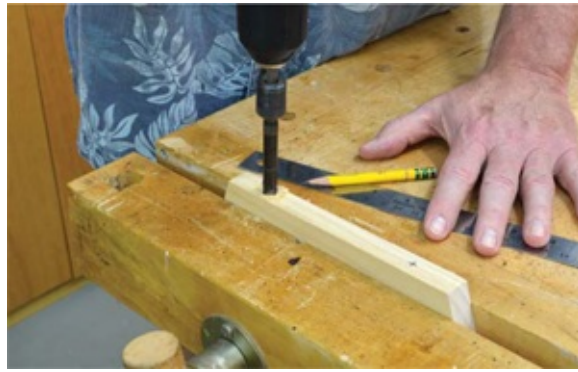
Photo 3 With the support foot upside down in a vise, drill countersunk pilot holes for the attachment screws.
