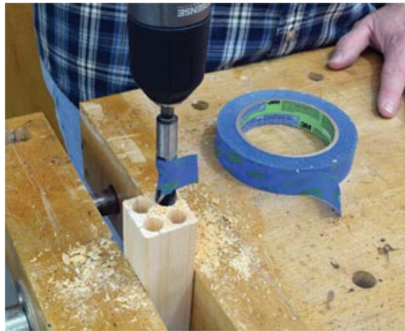
Photo 6 Drill the sound holes to finished depth, relocating the tape each time.
