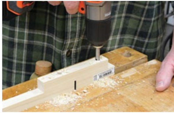
Photo 3 Drill the axle holes in the beam with a \frac{5}{16} " bit. A piece of scrap between the two sections helps prevent tear-out.
