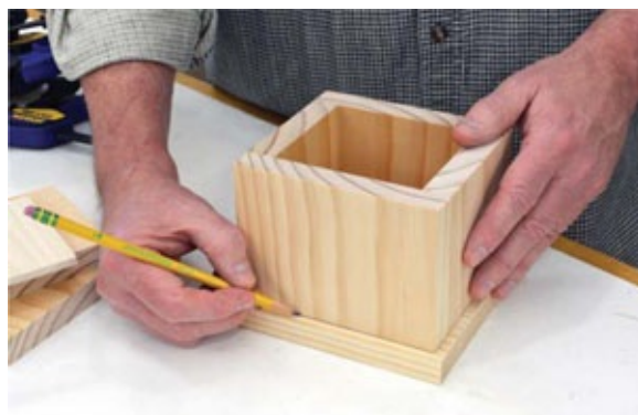
Photo 4 Lightly trace pencil lines onto the bottom piece around the inside and outside of the box.
