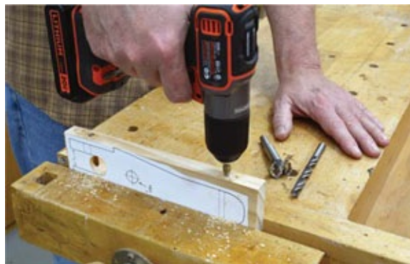
Photo 1 Drill a \frac{3}{8}" hole for the racer's rear axle, and a \frac{7}{32}" hole for the front axle.
