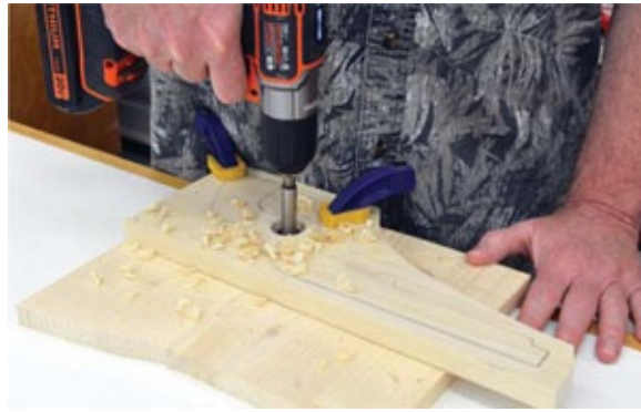
Photo 2 Drill a 1- \frac{1}{8} " hole for the trigger hole. The scrap beneath the workpiece prevents splintering on the back of the pattern.
