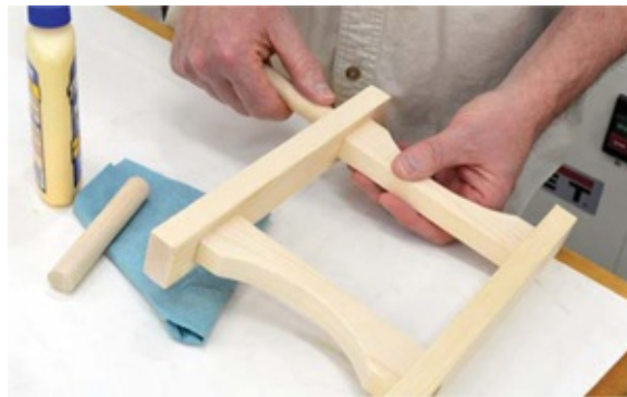
Photo 8 Glue the handles into place on each side of the winder.
