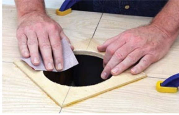
Photo 6 Sand away any splintering and roughness from the freshly cut edges of the target hole.
