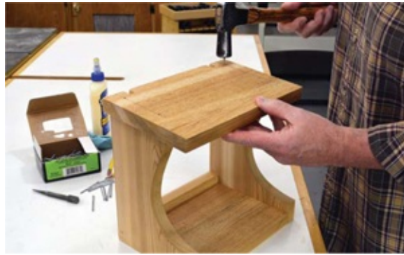
Photo 6 A penciled guideline helps place the nails accurately when attaching the roof.
