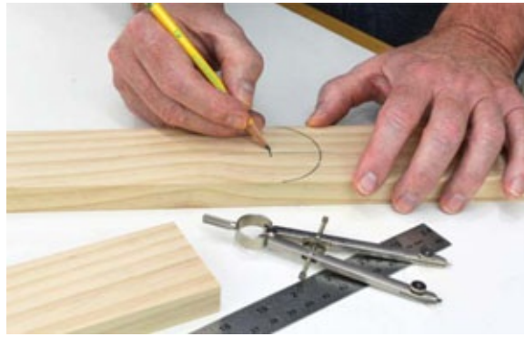
Photo 11 Use a compass to draw cut lines for the curved leg ends.
