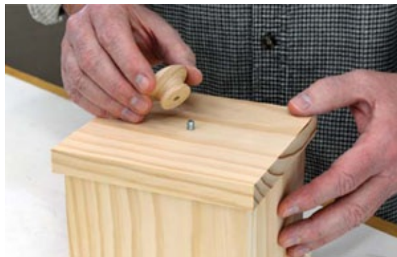
Photo 9 A simple cabinet knob adds a nice detail and makes it easy to remove the top.
