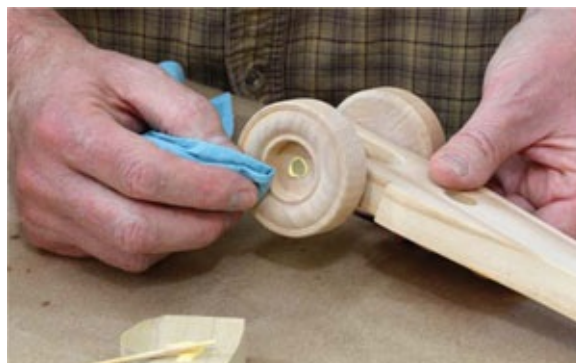
Photo 6 You're sure to get some glue squeeze-out when mounting the rear wheels – wipe it off right away.
