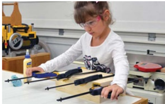
Photo 2 Edge-to-face glue joints are plenty strong in this application without additional fasteners. Be sure that the ends of all three pieces line up flush.
