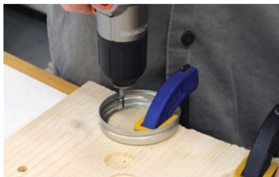
Photo 9 Clamp the jar lid down and carefully drill \frac{1}{16} " mounting holes through its rim.
