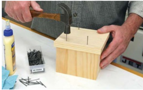
Photo 6 Glue the bottom in place, then strengthen the joint with 4d finish nails.
