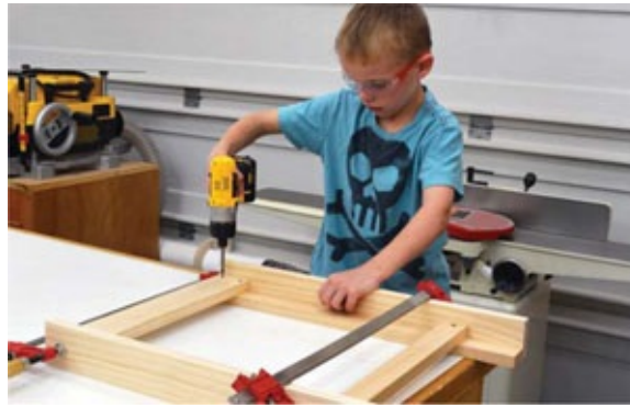
Photo 5 Starting with the workbench ends, attach the upper and lower stretchers with glue and countersunk screws.
