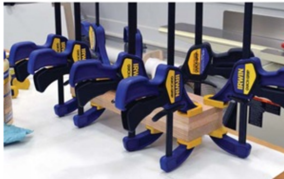
Photo 6 With the spacers in place, clamp the front to complete the assembly.
