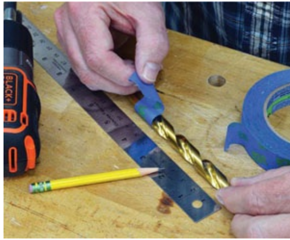
Photo 5 Mark the bit with masking tape to indicate drilling depth for the first hole at 4”.
