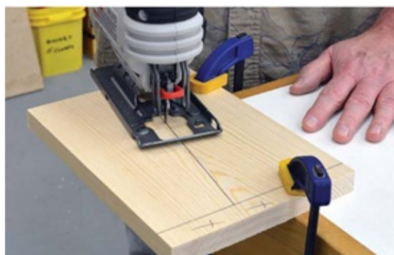
Photo 1 Both shelf sides can be cut from a single piece of 1x8 pine.
