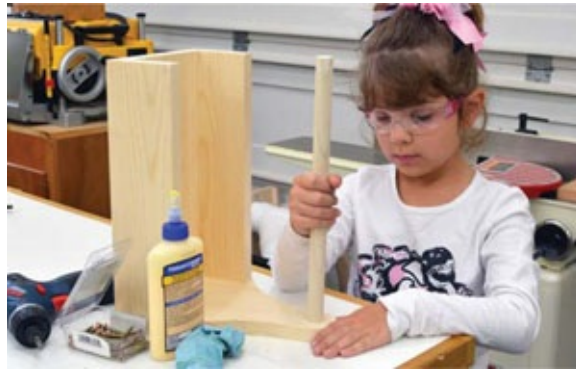
Photo 7 It's essential to have everything close at hand – glue, fasteners, drill/driver, clamps – during assembly.
