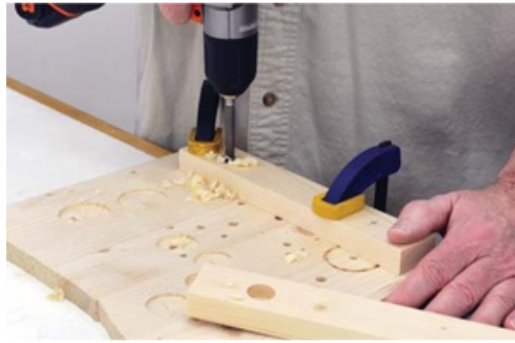
Photo 3 Drill \frac{3}{4} " holes for the handles in one end of the side pieces only.
