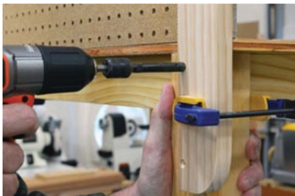
Photo 5 With the completed rack clamped to the workbench, drill countersunk pilot holes and screw it securely in place.
