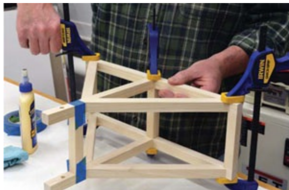
Photo 8 Glue and clamp the three crosspieces into place to assemble the frame. Note the fourth crosspiece taped in at the top as a temporary spacer.
