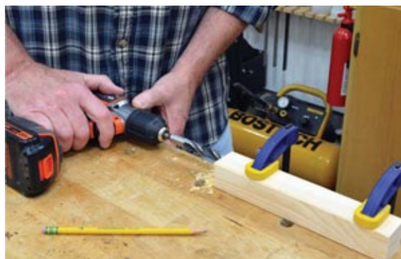
Photo 4 With the workpiece securely clamped and holding the drill squarely on the worksurface, drill four \frac{1}{2} "-diameter starter holes.
