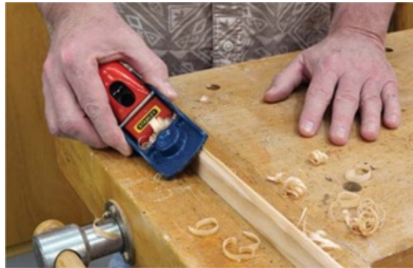
Photo 4 Use a small block plane to shave a bevel on the handle workpiece before cutting it to length.
