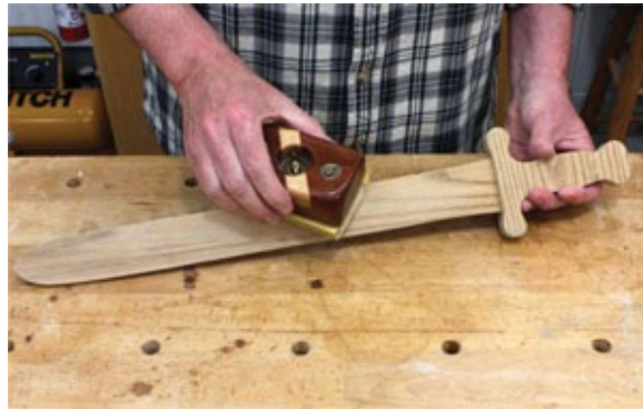
Photo 9 Use a sanding block for the faces and straight edges of the sword, rounding over all sharp edges.
