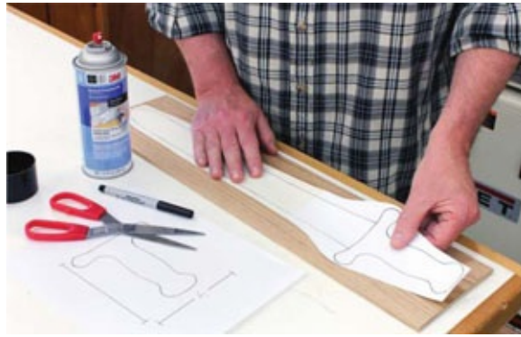
Photo 2 Press the pattern onto the workpiece, smoothing it out to remove wrinkles.
