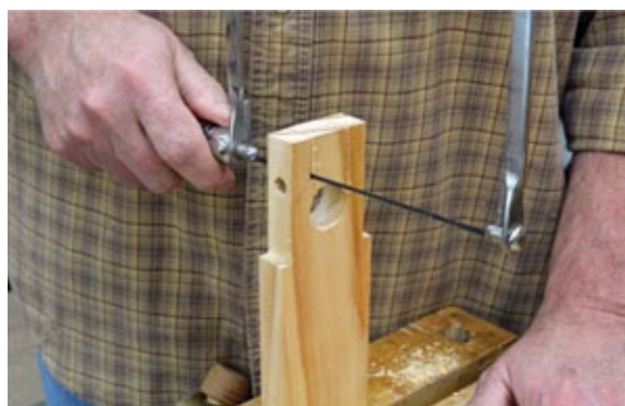
Photo 3 Cut out the racer body with a coping saw or, if you prefer, a scroll saw.
