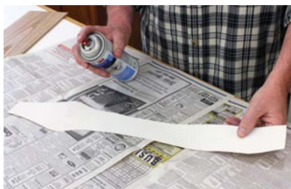
Photo 1 Apply spray adhesive to the back of the sword pattern.
