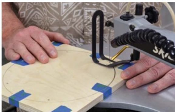
Photo 2 Cut out the stacked paddle shapes on the scroll saw, or with a coping saw.
