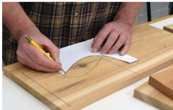
Photo 1 Trace the side patterns onto the workpiece, avoiding knots and other flaws in the wood if possible.
