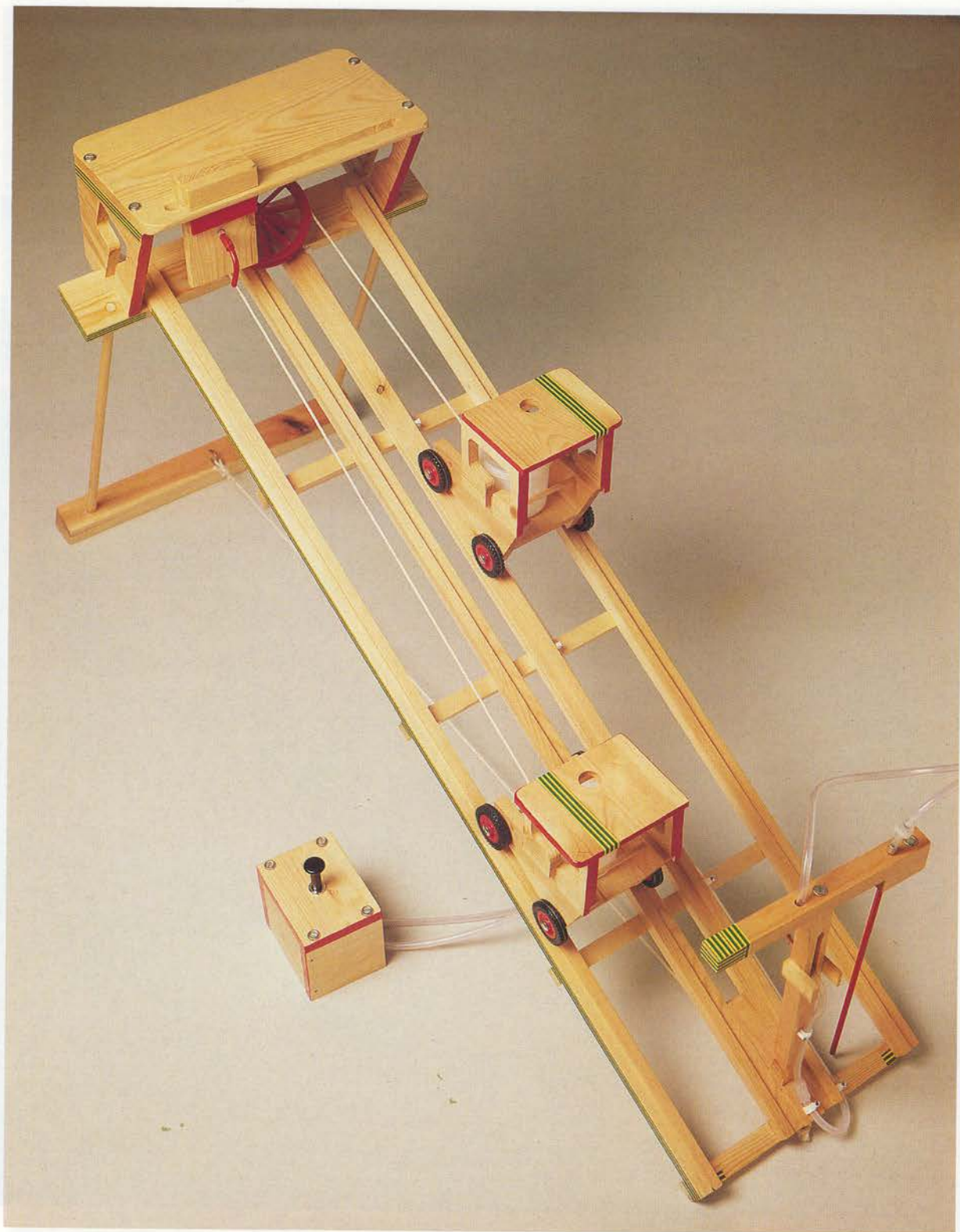
14. WATER-POWERED MOUNTAIN HOIST – this ingenious form of passenger transport is inspired by the Linton and Lynmouth Cliff Railway.
