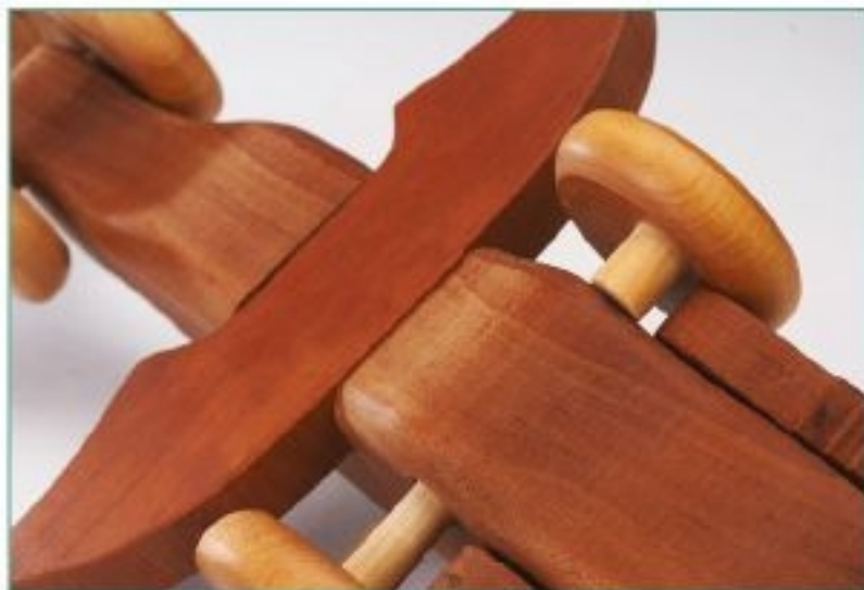
The pectoral fin is glued into a slot in the bottom of the body.
