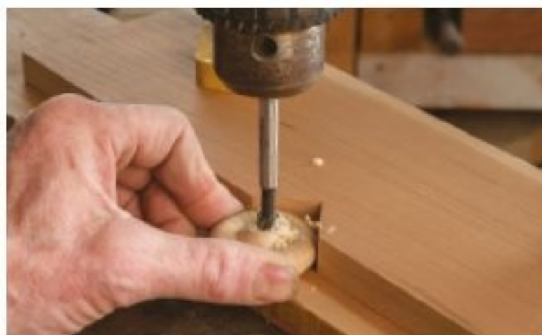
Figure 3.10. This simple jig is essential for accurately drilling offset axle holes in wheels.
