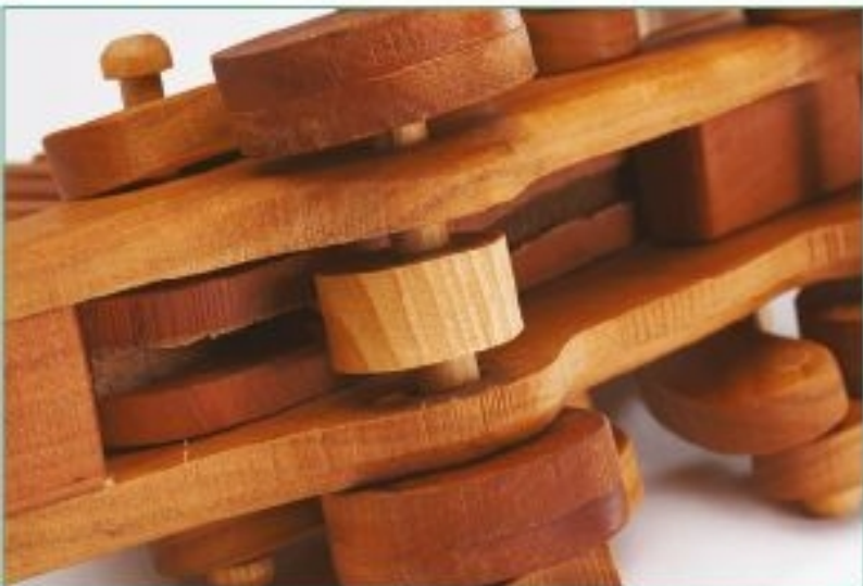
The cam wheel, mounted on the rear axle, causes the sail to bob up and down and the mouth to open and close.
