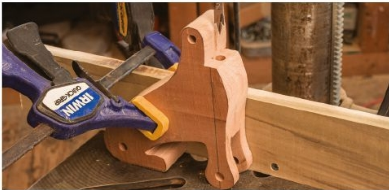
Figure 16.2. Use a simple jig made of two boards glued together at a right angle to hold the body firmly in a vertical position as you drill the hole for the drive dowel.
