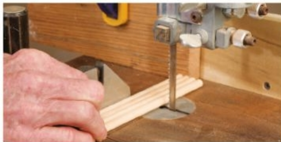
Figure 3.1. The scrap clamped to the fence will help you cut several dowels to the same length. The scrap is clamped in front of the blade so the pieces don't bind as they pass the blade.
