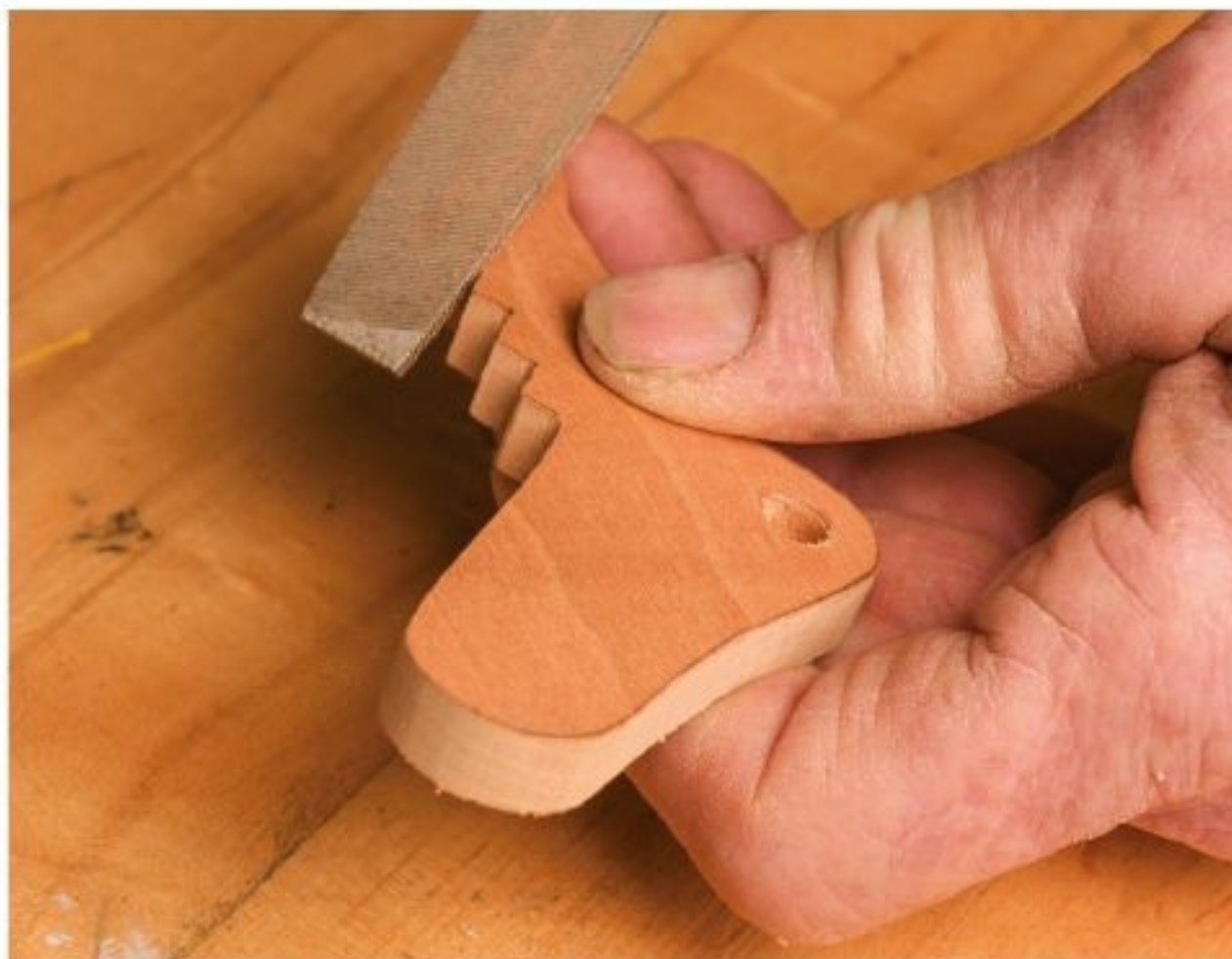
Figure 12.1. Use a flat file to put a nice, clean bevel on each of the teeth.
