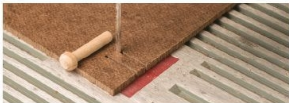
Figure 3.5. To cut a peg to length, butt the head against the edge of a scrap of hardboard. Hold it firmly as you pass it by the blade.
