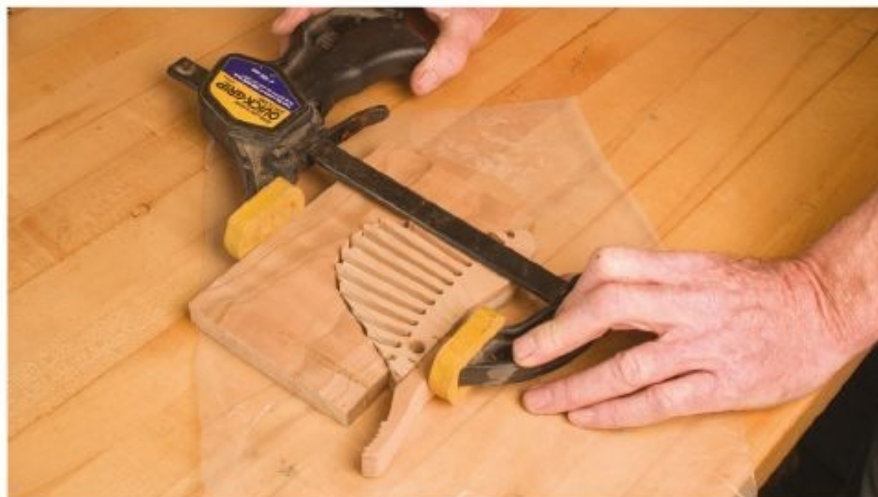
Figure 22.2. I used a piece cut out like the silhouette of the top of the sail to clamp the pieces against when attaching the lower jaw.
