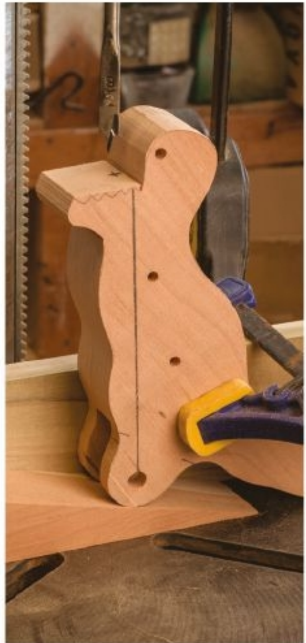
Figure 21.2. Clamping the body to a simple jig with a block under the axle hole will ensure accurate drilling of the long \frac{3}{8} " (1cm) hole for the drive dowel.
