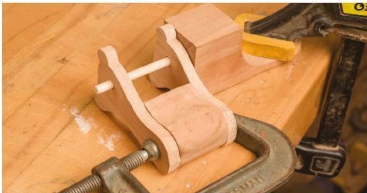
Figure 4.1. Using the jig to line up the two sides of the assembly, press the three pieces firmly together. Make sure the side next to the jig is flat against it and that the whole assembly can slide freely along the \frac{1}{4} " (6mm) dowel.
