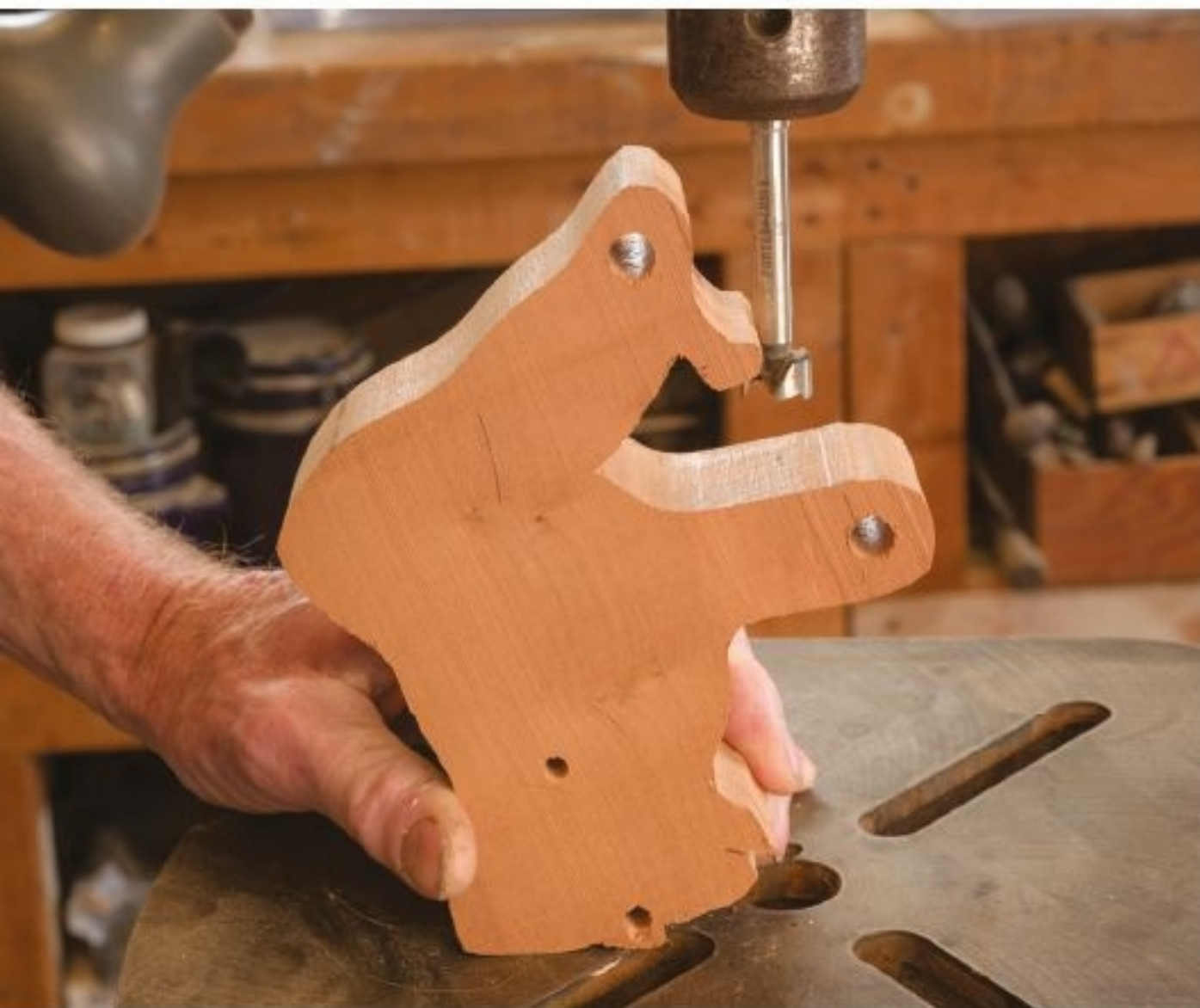
Figure 10.1. Rest the Gorilla on its forehead to drill the \frac{1}{2} " (1.3cm) hole for the knot of the pull cord.
