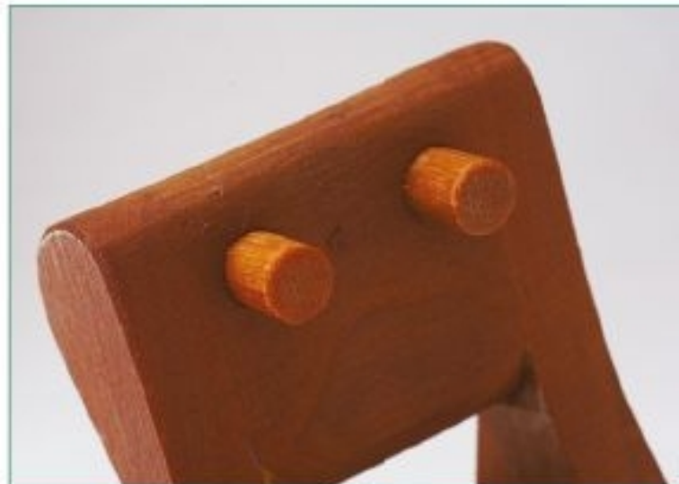
The teeth are glued into holes drilled in the bottom of the head spacer.
