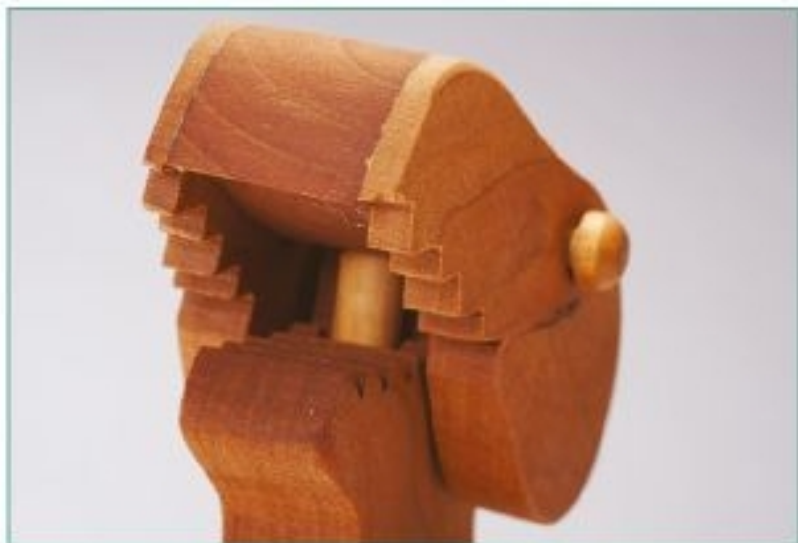
The drive dowel, inserted through a hole in the Tyrannosaurus's body, opens and closes the mouth in a roar.
