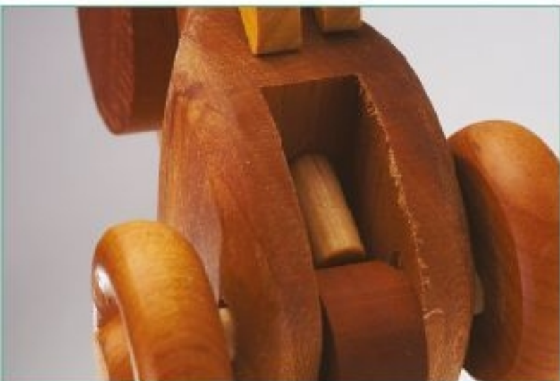
The cam wheel, hidden inside the dado slot, lifts and lowers the drive dowel, which move the Walrus's head up and down.
