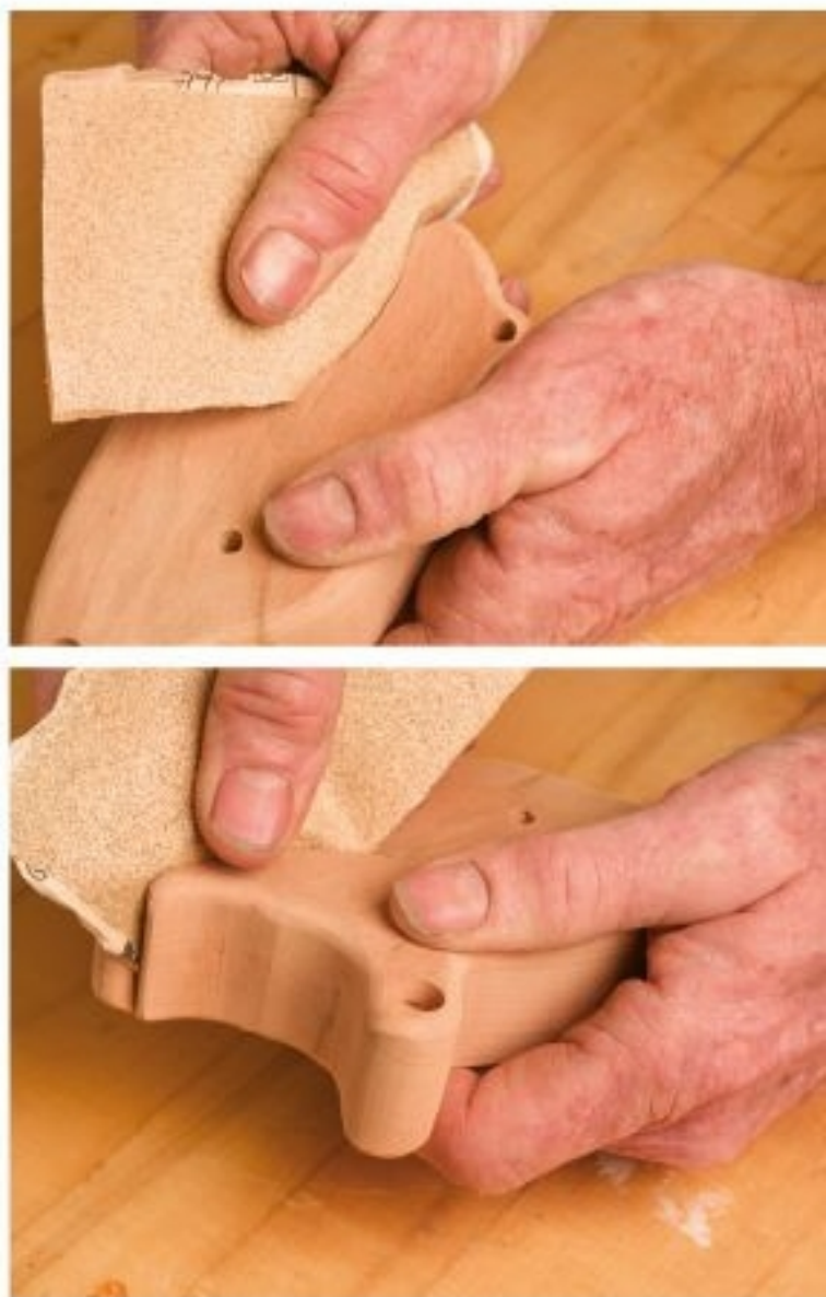
Figure 5.2. Break the edges of the mouth line by pulling the sandpaper through the mouth upward and then downward.
