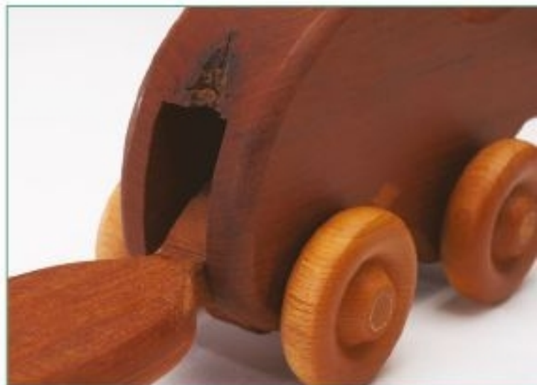
The dado slot cut in the body allows the space for the tail to move up and down.
