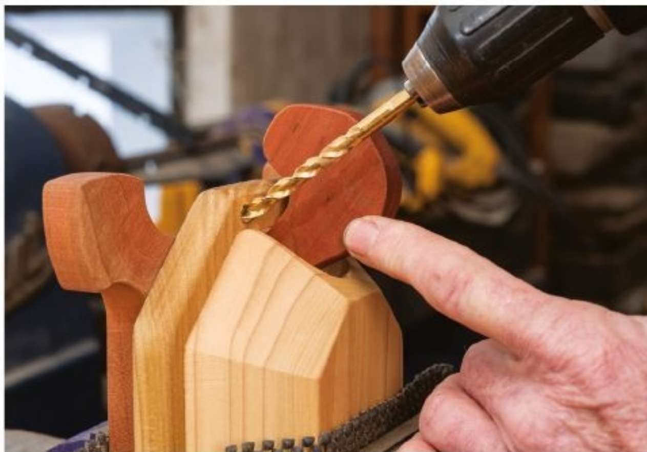
Figure 17.8. Drill these holes at a compound angle toward the side and back.
