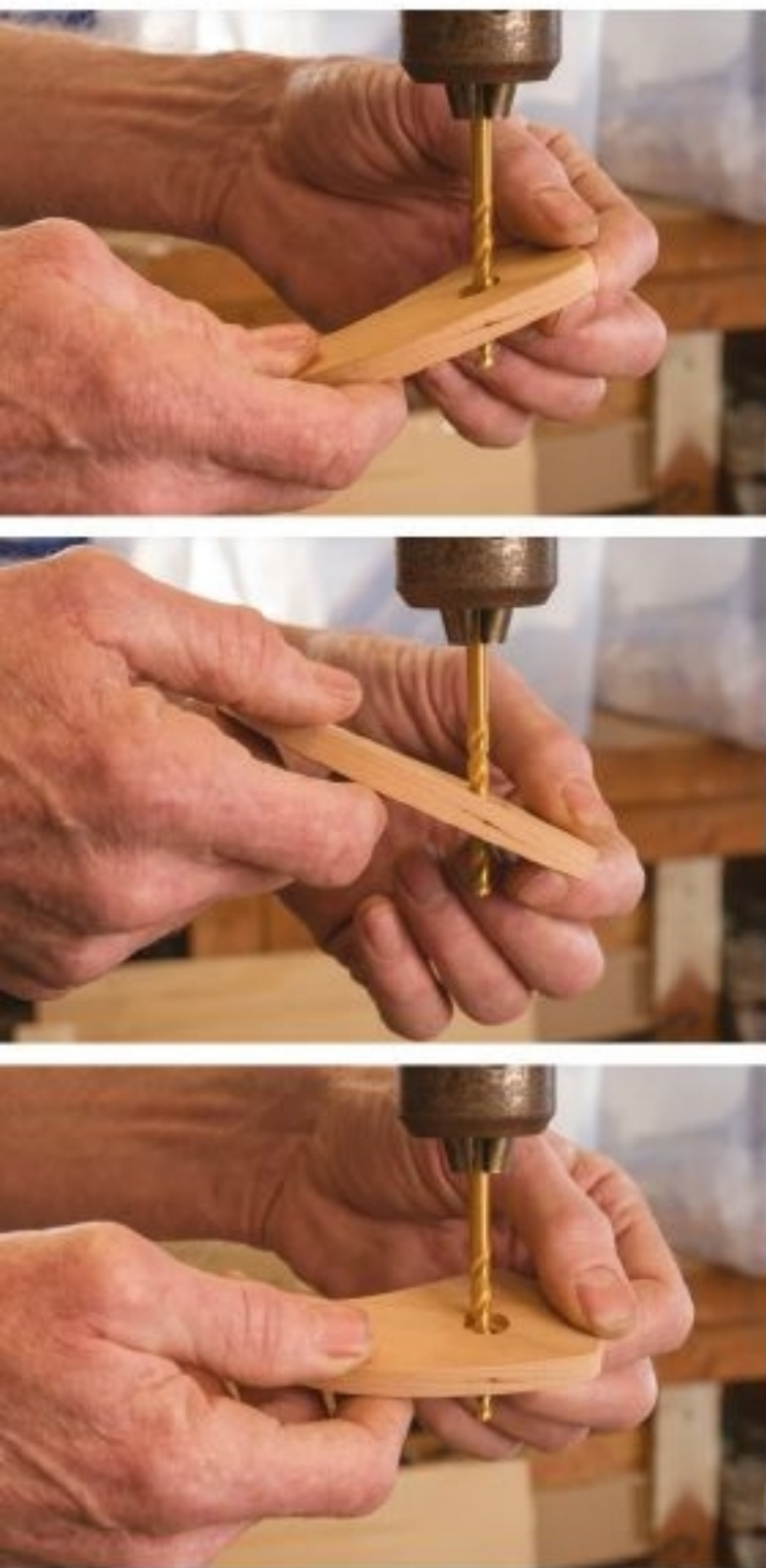
Figure 23.5. Flair the hole in the flipper outward (top and bottom) by tilting it around in a circle while it is on the drill bit.
