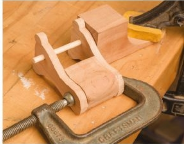
Figure 3.15. Using the jig to line up the two sides of the assembly, press the three pieces firmly together. Make sure the side next to the jig is flat against it and that the whole assembly can slide freely along the 1/4" (6mm) dowel.
