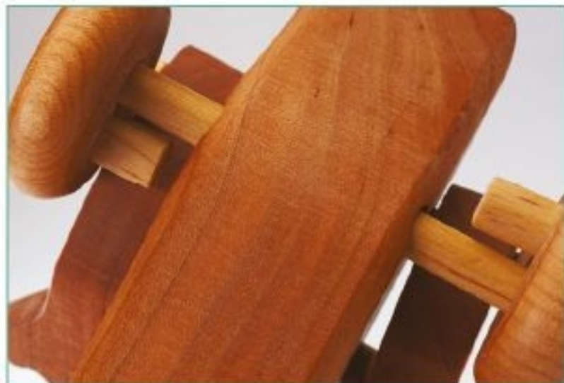
The wheel plugs are positioned so one is up while the other is down. This moves the legs one at a time so the Duck appears to be walking.
