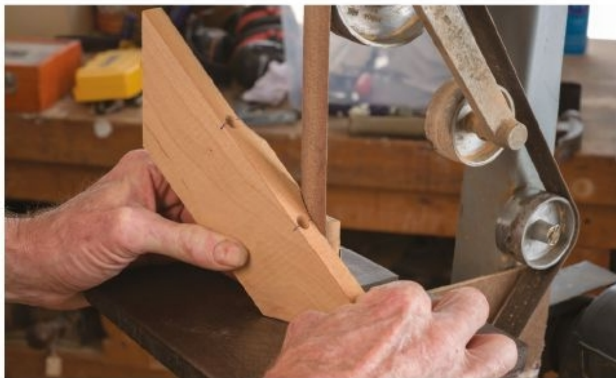
Figure 17.5. Sand the curved cut the same way you cut it out.
