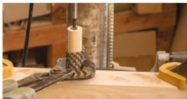
Figure 15.2. Drill a \frac{1}{8} " (2.1 cm) hole, about 2\frac{1}{2} " (6.4 cm) deep, in a middle of a 2x4. Clamp it to the drill press table with the hole centered under the bit. Grip the \frac{3}{4} " (1.9 cm) dowel with a piece of inner tube and pliers as you drill the axle hole through the center.
