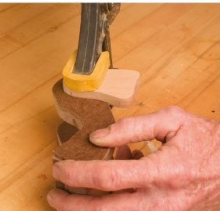
Figure 18.2. Use this template to position the ears as you glue them one at a time.
