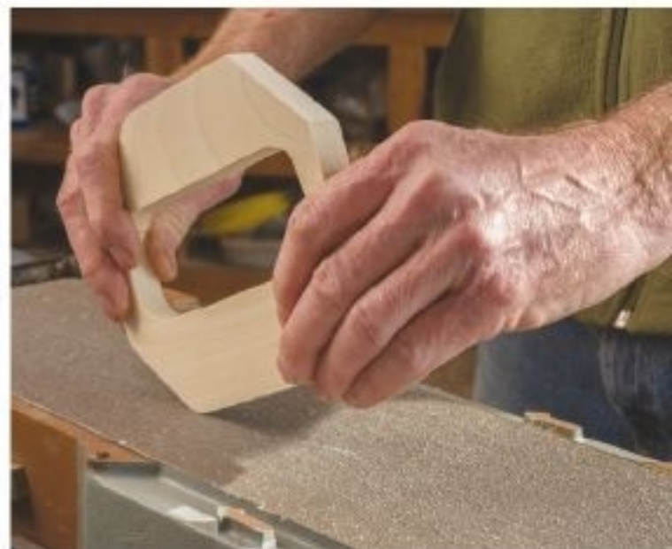
Figure 17.3. Holding the shell base vertically on the belt sander, sweep around each corner to gently round them.
