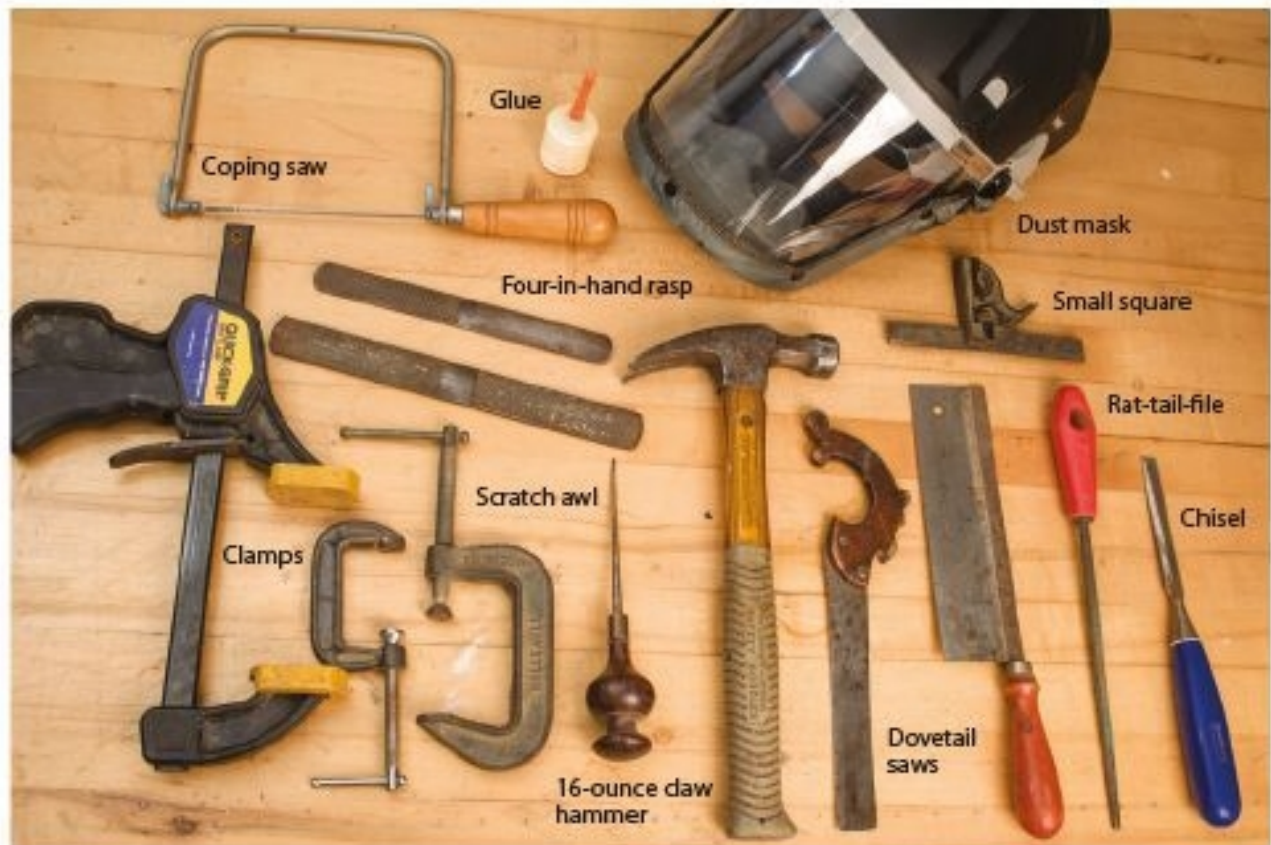
Figure 2.2. You don't need a lot of hand tools to make toys, just the few basic cutting, pounding, gluing, clamping, and measuring tools shown here.
