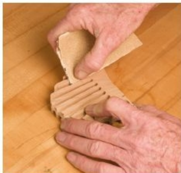
Figure 22.1. Hold each rib firmly as you lightly sand the edges.
