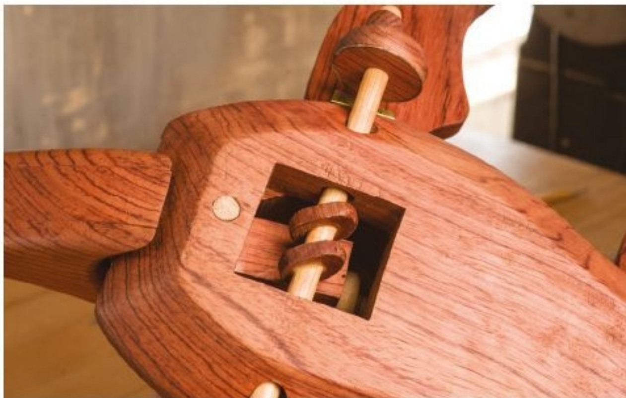
Figure 23.1. As the axle turns, the ovals tip one way and then the other, moving the head and neck back and forth by means of the peg that rides between the ovals. (Note the 1" [2.5cm] wheel reduces the friction and helps the head move more easily.)
