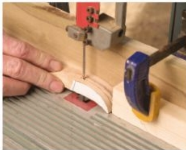
Figure 3.2. Make accurate dead-end lengthwise cuts (like the Walrus's tusks) by clamping a scrap to the fence beyond the blade.
