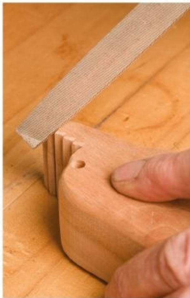
Figure 14.2. Use a small flat file to put a nice, clean bevel on the edges of each tooth.
