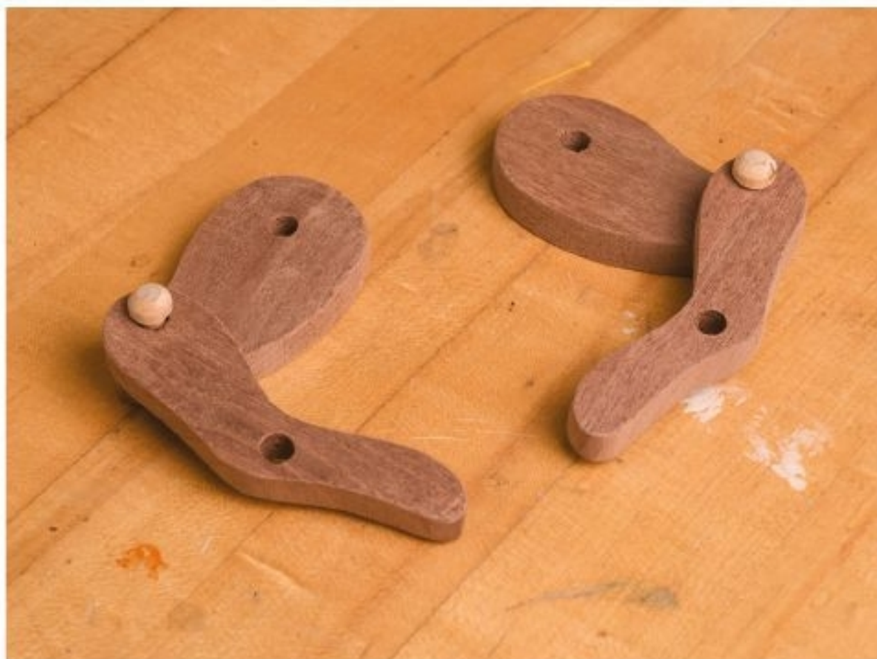
Figure 11.1. Be sure to assemble the legs in two opposing sets. This may seem obvious, but it's an easy mistake to make, and it's infuriating to have to cut the legs apart and redrill them.
