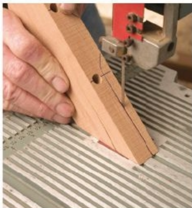
Figure 17.4. Hold the foot piece firmly, resting the cut-off corner on the band saw table as you cut the curve on the top of each foot.
