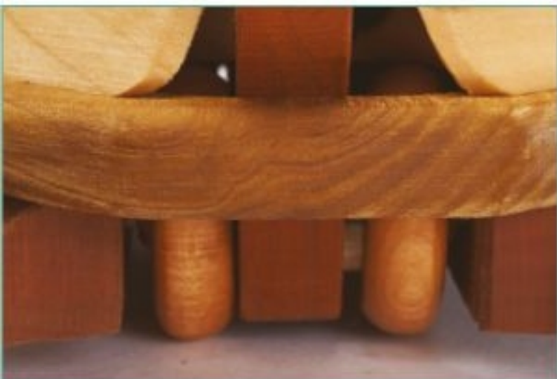
The inner drive axles, mounted in off-center holes in the wheels, cause the Turtle's head and tail to move in and out of the shell.
