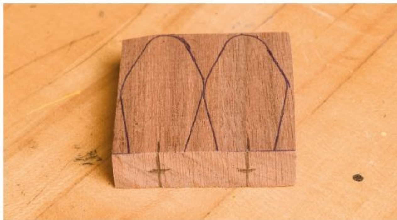
Figure 7.1. Lay out the flippers perpendicular to the end grain. The edge that is to be drilled should be flush against the end grain edge.
