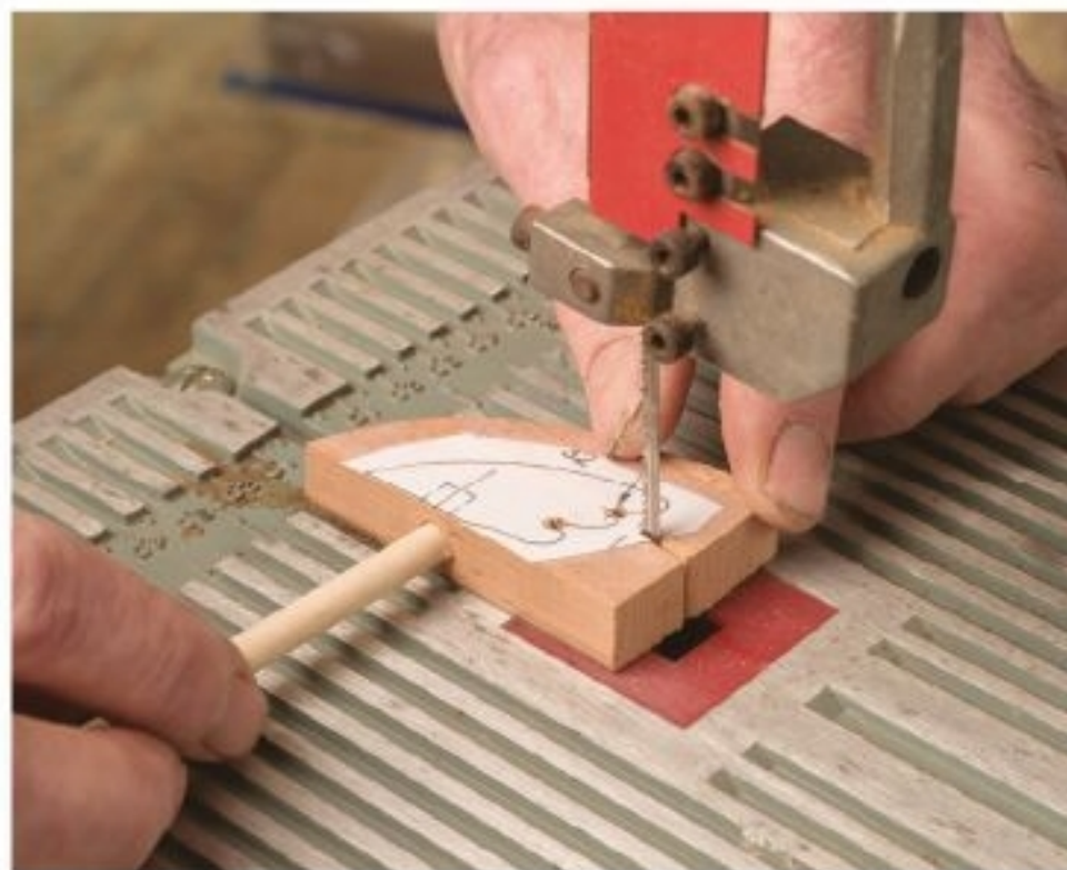
Figure 13.2. I stick a temporary dowel in the holes in the flippers to make it safer and easier to cut them out and sand them.
