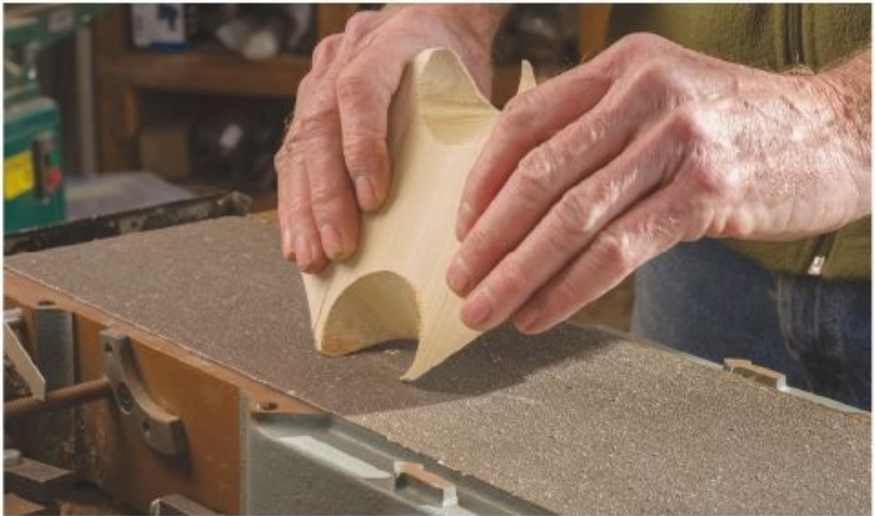
Figure 17.2. To round over the bottom of the head hole and tail hole sections of the shell, hold these surfaces lightly on the belt sander, one at a time, and rock them smoothly toward you and away from you.
