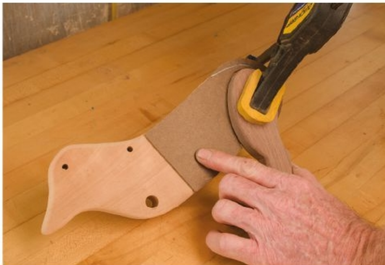
Figure 18.3. Leave extra material around the back of the template so it won't break. Use the template to line up the first hind leg, and then line up the second leg perfectly with the first. Make sure the axle is square and spins freely, and then clamp the legs, using pads or scraps to protect the surface of the legs.
