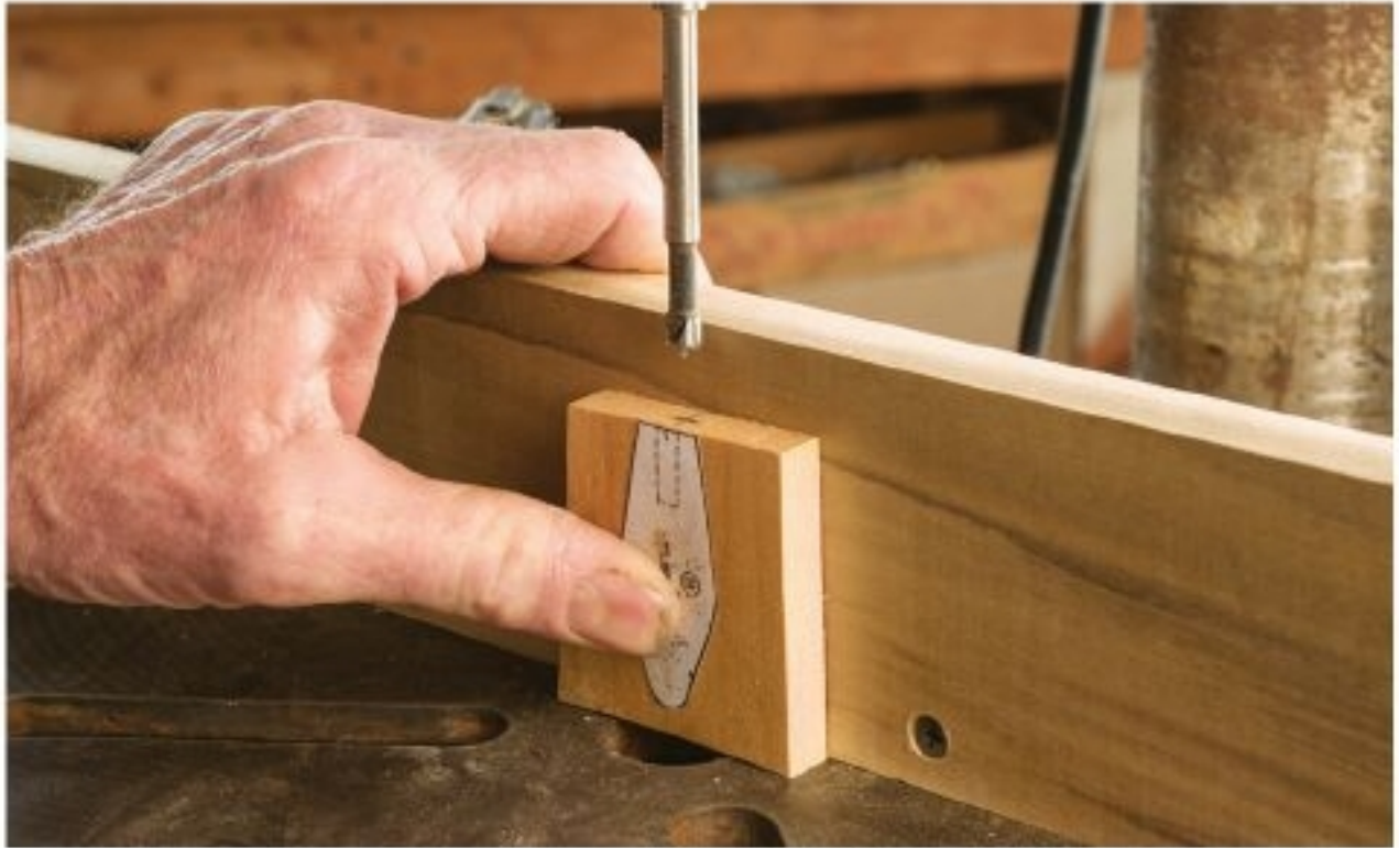
Figure 7.2. Use a square block to hold the flippers perpendicular to the drill press table as you drill the \frac{7}{16} " (6.5mm) holes.
