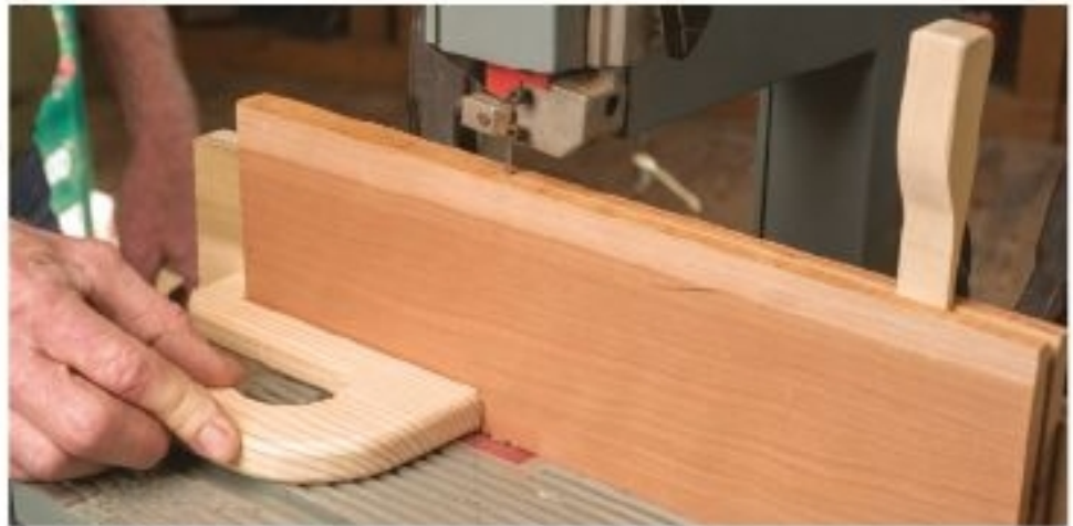
Figure 3.3. Clamp the makeshift rip fence to the band saw table, making sure it is parallel to the blade. Sometimes internal stresses in a board are released as it is resawn. This can cause the resawn pieces to press together, binding the blade. A small wedge (kerf keeper) pressed into the kerf, beyond the blade, will counteract this tendency.
