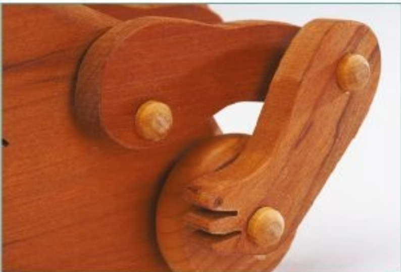
Attaching the leg to an off-center hole in the wheel causes the leg to move up and down as the wheel turns.
