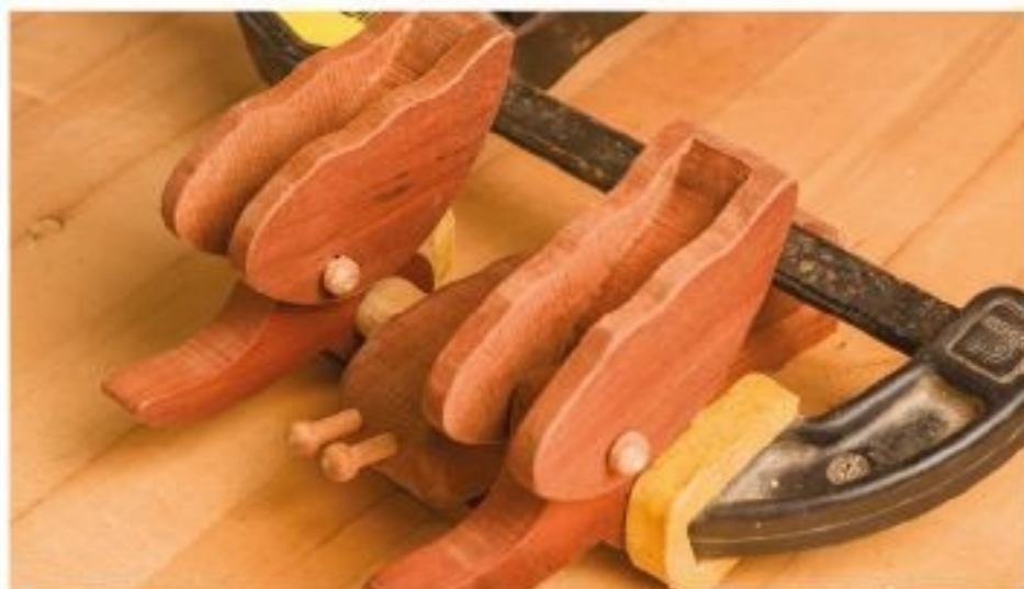
Figure 15.3. Make sure you clamp both claws at the same angle. If they are too high, they'll flop back and won't close again. If they're too low, the dowel pegs won't be able to open them.
