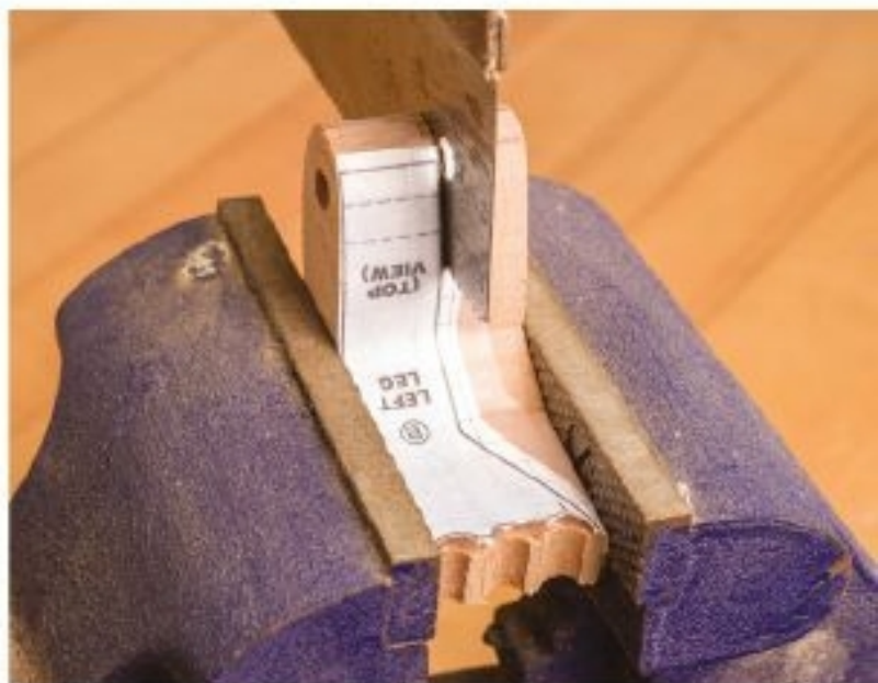
Figure 8.1. Cut out the legs with a back saw or a dovetail saw.
