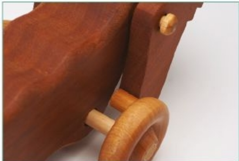
The front wheel plugs push on the back of the Crocodile's jaw, lifting the head.
