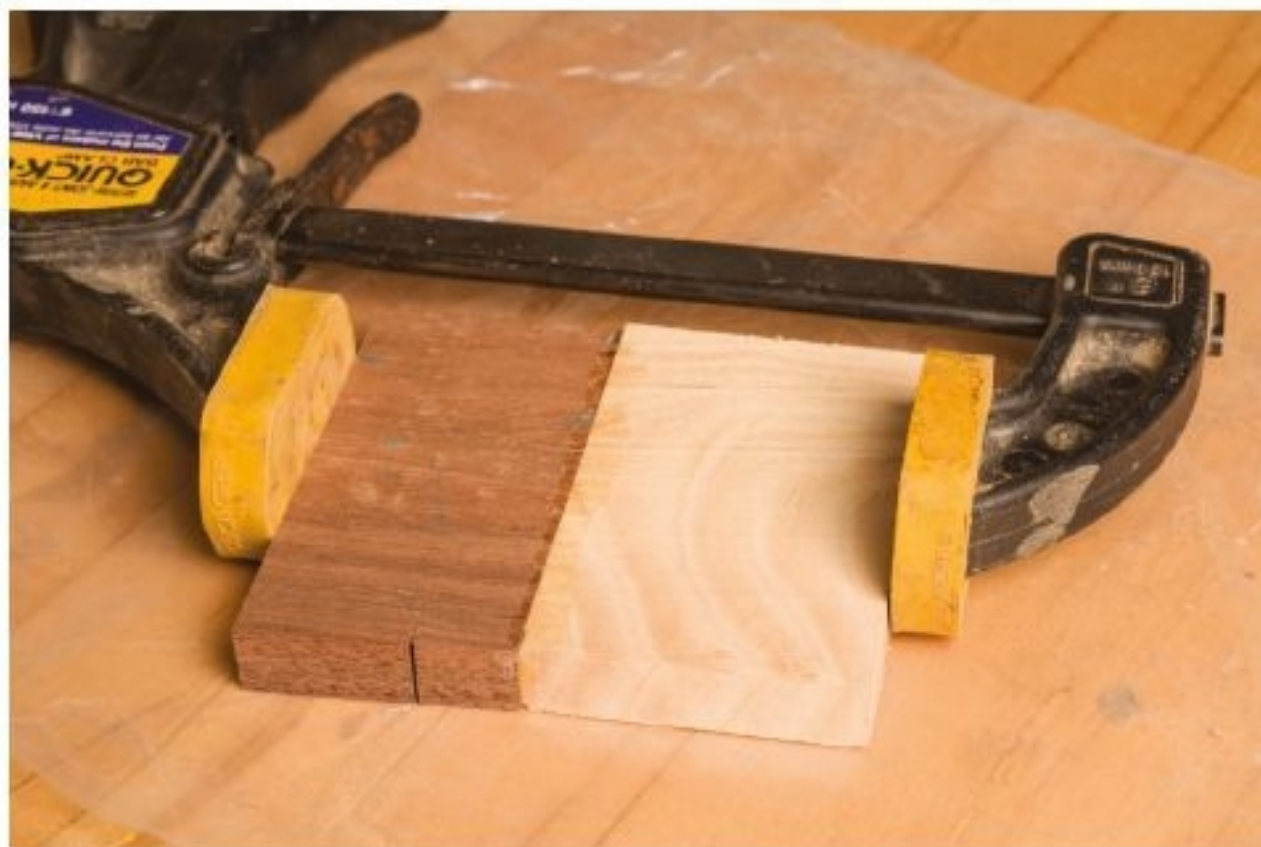
Figure 9.1. Glue the two spacers together, end grain to end grain, before they are put between the sides. Use plenty of glue, as the end grain tends to absorb more.
