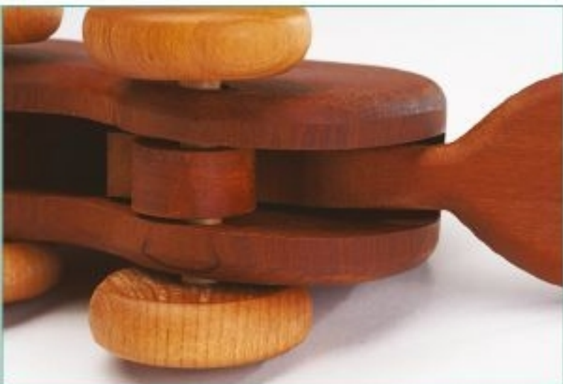
The cam wheel lifts and lowers the tail as the tail axle turns.
