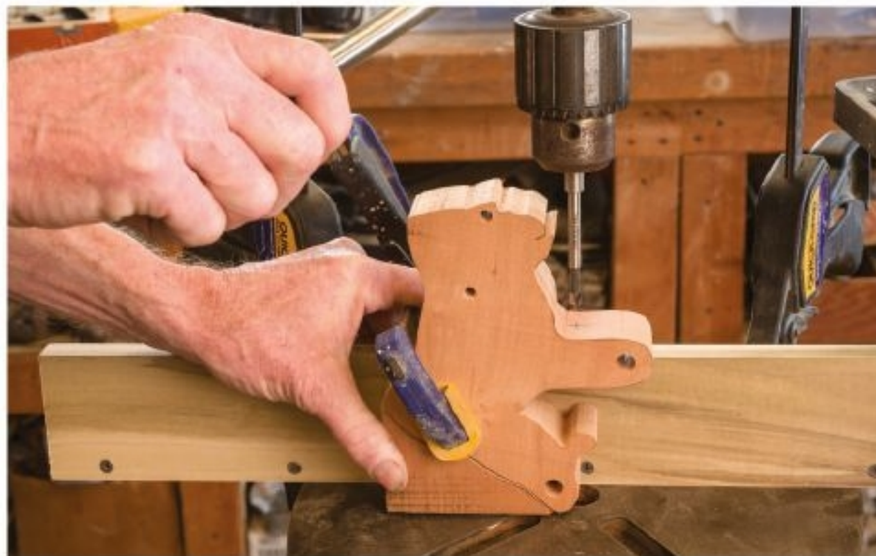
Figure 10.2. Clamp the Gorilla to a simple jig to drill the \frac{1}{4} " (6mm) hole.
