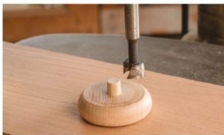
Figure 3.9. A dowel in a board will locate wheels accurately for drilling peg holes. If you use raised hub wheels, make a depression for the hubs to sit in as you drill.
