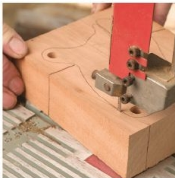
Figure 3.8. Relief cuts will also help you make tight inside or outside curves. Be sure to turn the saw off and wait for the blade to stop moving before you back out of a cut, or you risk pulling the blade off the wheels.
