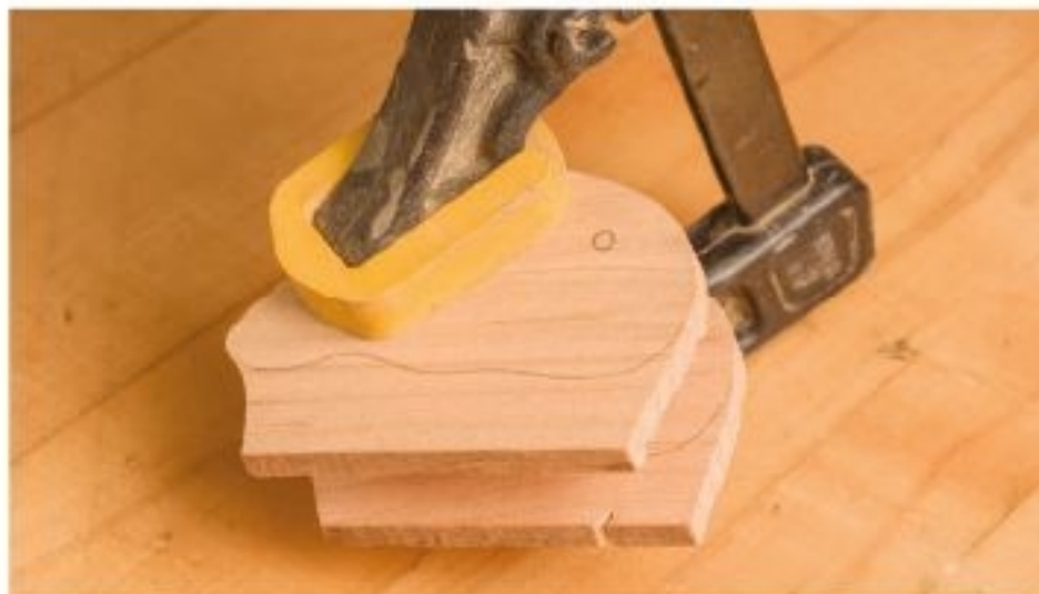
Figure 15.1. Cut out enough of the claw sides to position the spacer, and glue both claw assemblies. This will enable you to position the peg holes perfectly, after the glue is dry.
