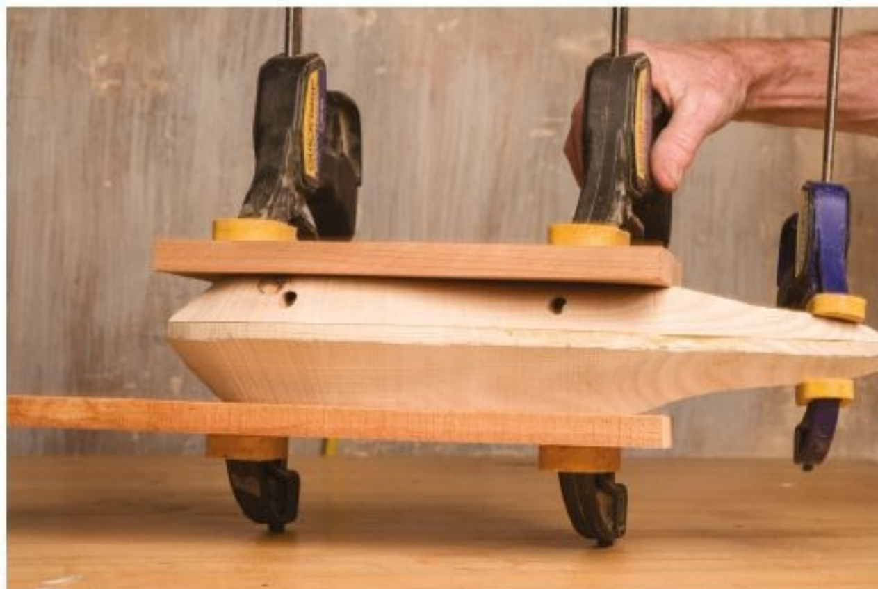
Figure 23.3. You can use two boards to spread the pressure out and provide clamping surfaces as you glue the two main body pieces together.
