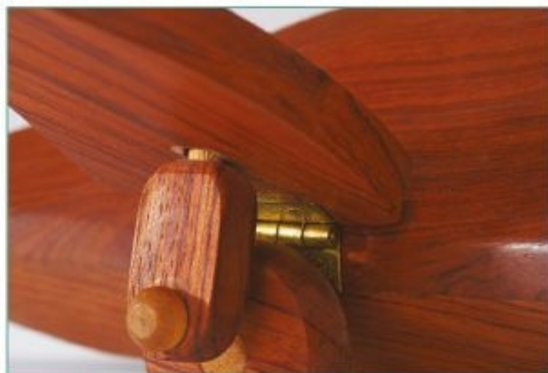
The pitman arms, mounted on the wheels, push the flippers up and down to make Nessie swim.
