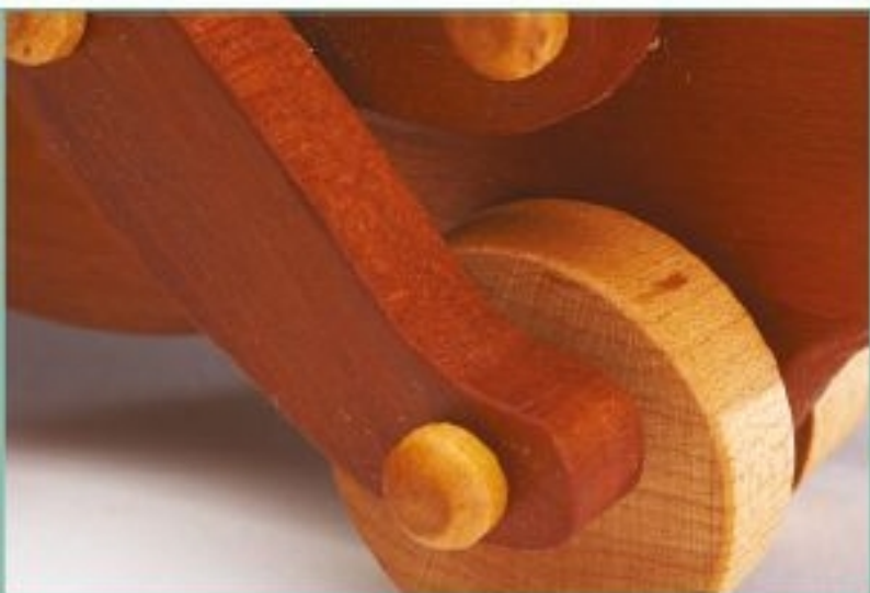
The front legs are pegged to opposing holes in the front wheels so the Brontosaurus appears to be lumbering forward.
