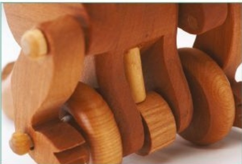
The cam wheel, mounted on the front axle, lifts and lowers the drive dowel.
