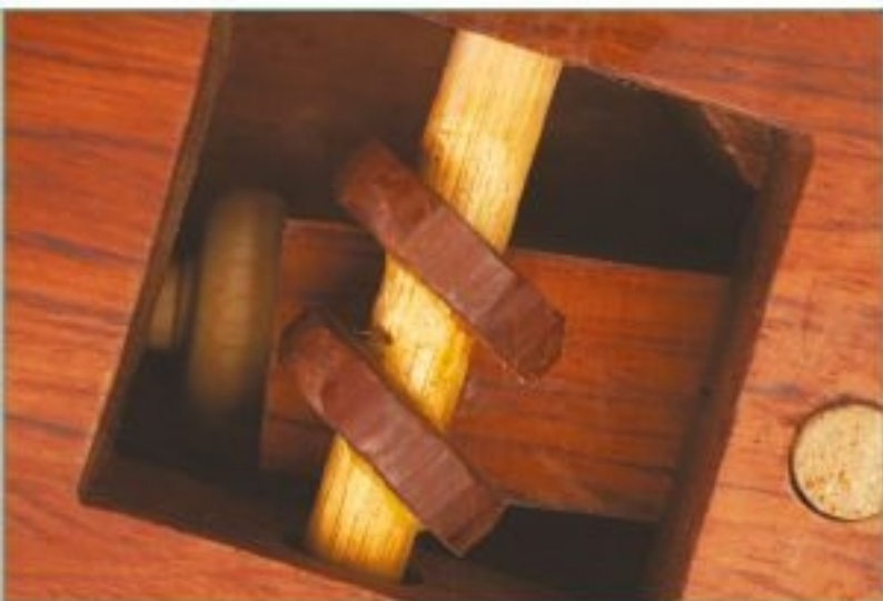
The two oval wheels mounted on the front axle are used to sway the head from side to side.
