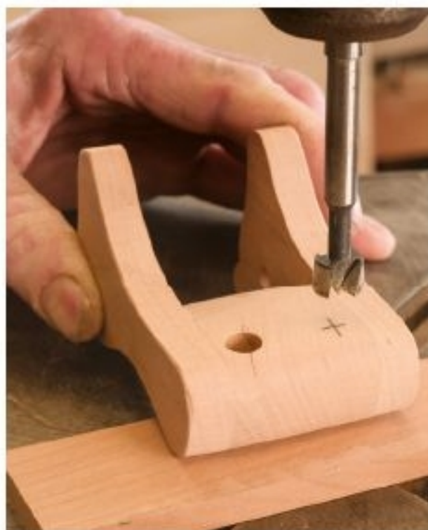
Figure 4.2. Use a scrap under the Hippo's nose to support it at the proper angle to drill the holes for the teeth.
