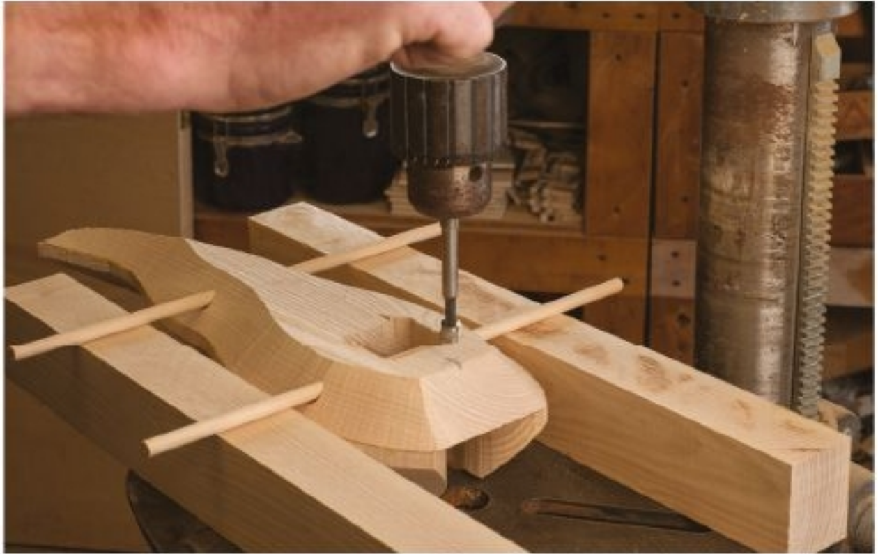
Figure 23.4. If you put dowels through the axle holes and rest them on thick scraps of equal thickness, you can drill the pivot hole accurately on the drill press, in spite of the awkward shape of the piece.
