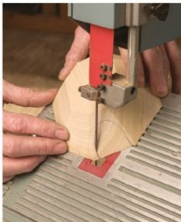
Figure 17.1. This is a difficult cut, so use a sharp \frac{1}{8} " (3mm) blade and take your time. Once you pass the top of the arc, anticipate the curve and try to keep ahead of it as you saw or you'll be forced off the line.
