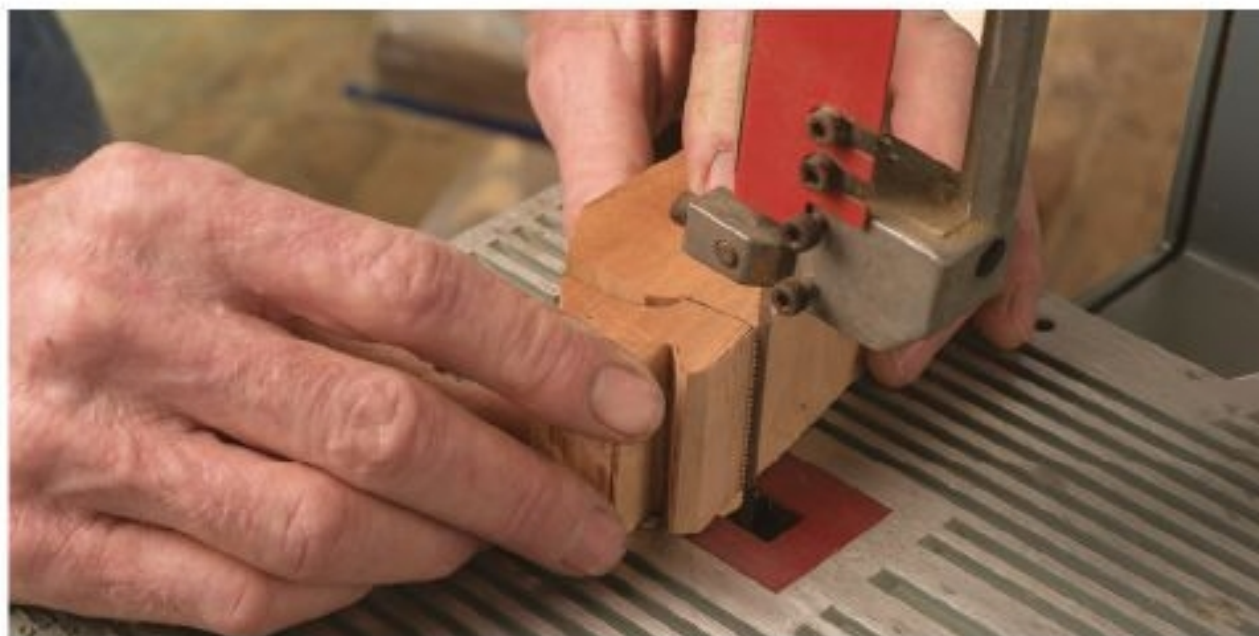
Figure 16.3. Lay out the spacer with a big piece to hold on to so you can keep your fingers away from the blade on the band saw or scroll saw.
