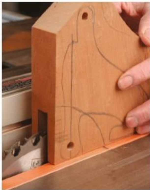
Figure 16.1. Make a pencil mark on the table of the table saw showing where the blade meets the table. That's where you will end the cut.
