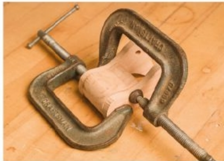
Figure 3.16. Be careful not to let the parts shift as you apply pressure to the clamps. Take the assembly off the jig to apply the second and possibly the third clamp.
