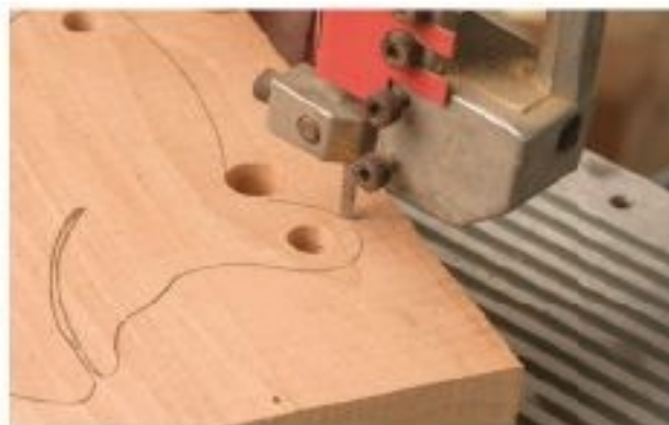
Figure 3.7. Tight inside curves can be cut very accurately by drilling the appropriate diameter hole first.
