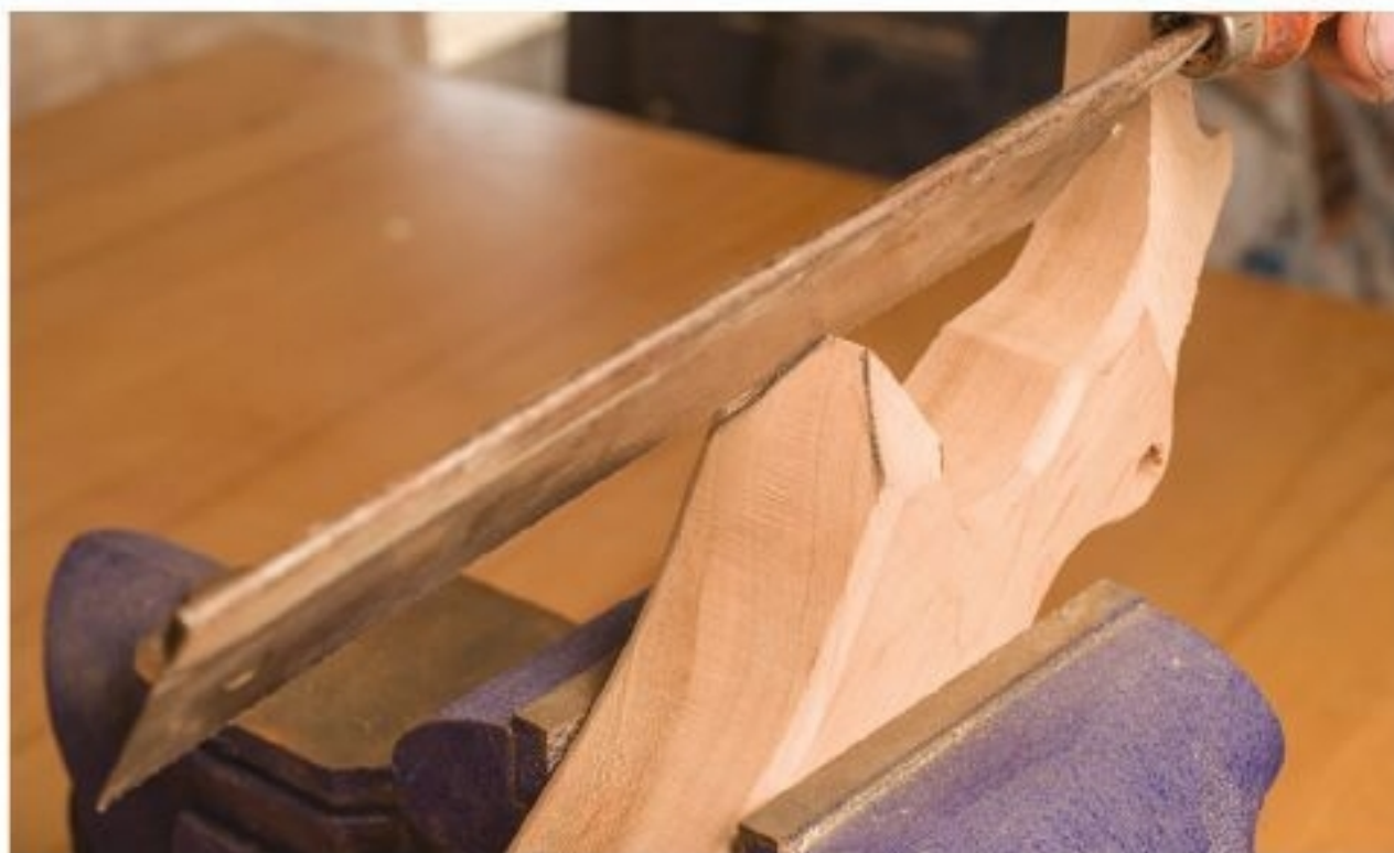
Figure 14.1. A pencil line will help you cut away the sides of the dorsal fins.
