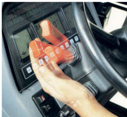
The power shuttle control lever, mounted beneath the steering wheel, allowed for forward, neutral and reverse changes.
