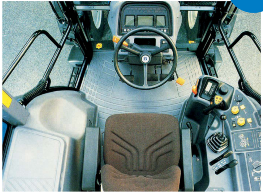
A publicity photograph showing the layout inside the 60/M Series cab. Note the controls for the top spec Range Command transmission to the right of the seat.
