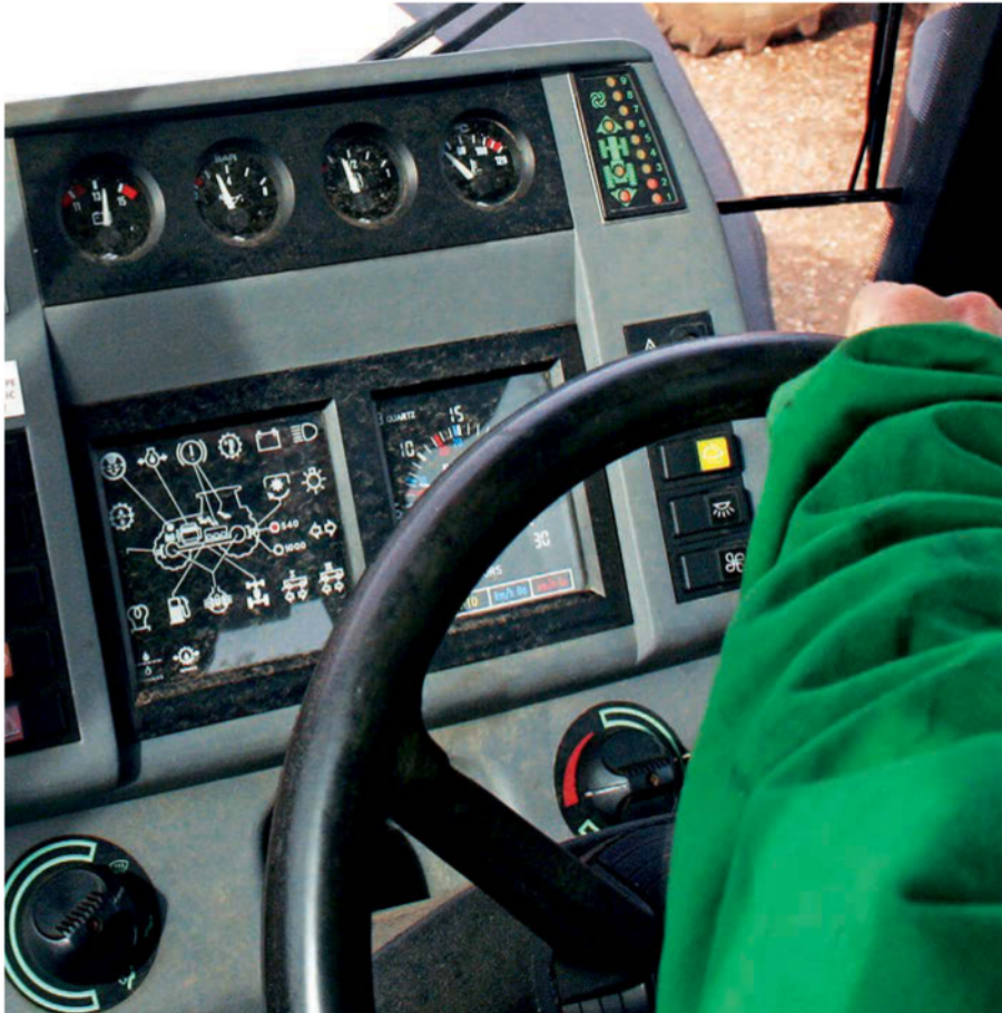
● Left: A mixture of dials, switches and lights characterised the Racing 165's comprehensive dashboard which, despite not having the touch screens of today's machines, was very advanced back in the early 1990s. Right: An advanced, joystick-type lever controlled the 165's transmission, with a button to select the nine powershift speeds and others to operate the rear linkage settings.
