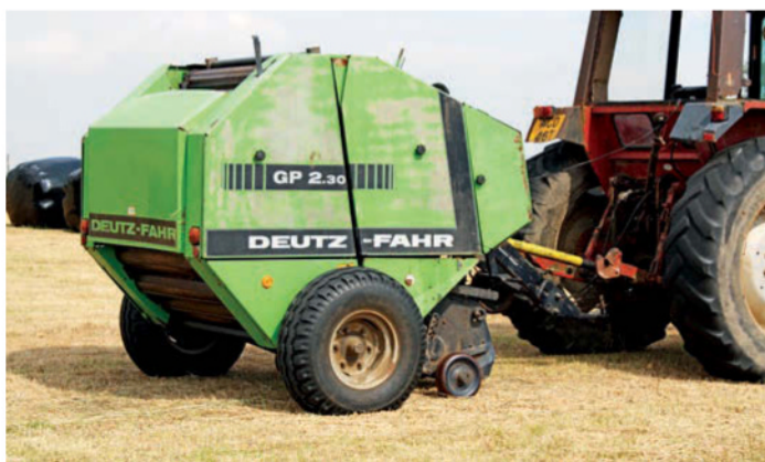
Left: Deutz-Fahr also built a range of fixed-chamber balers, including the GP 2.30 model that produced quite small-sized bales. Right: Rubber belts also formed the basis of the Vermeer round balers that were rebadged as part of the Massey Ferguson range. Here the belts on a 1450 model can clearly be seen as it ejects a finished bale. Photo: Kim Parks
