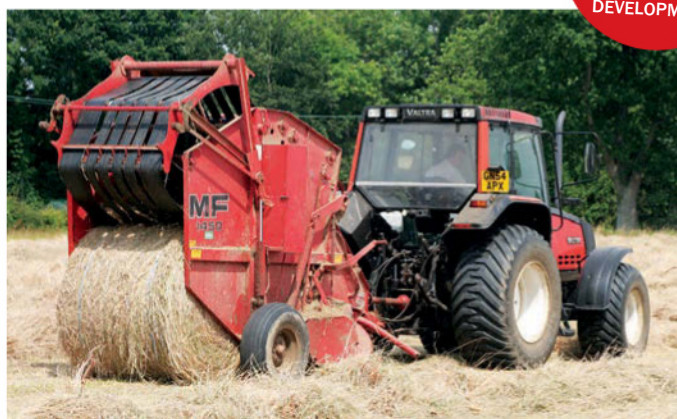
Left: Deutz-Fahr also built a range of fixed-chamber balers, including the GP 2.30 model that produced quite small-sized bales. Right: Rubber belts also formed the basis of the Vermeer round balers that were rebadged as part of the Massey Ferguson range. Here the belts on a 1450 model can clearly be seen as it ejects a finished bale. Photo: Kim Parks
