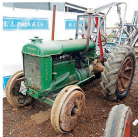
● A Henderson trencher is fitted to this very original Fordson Standard N.
