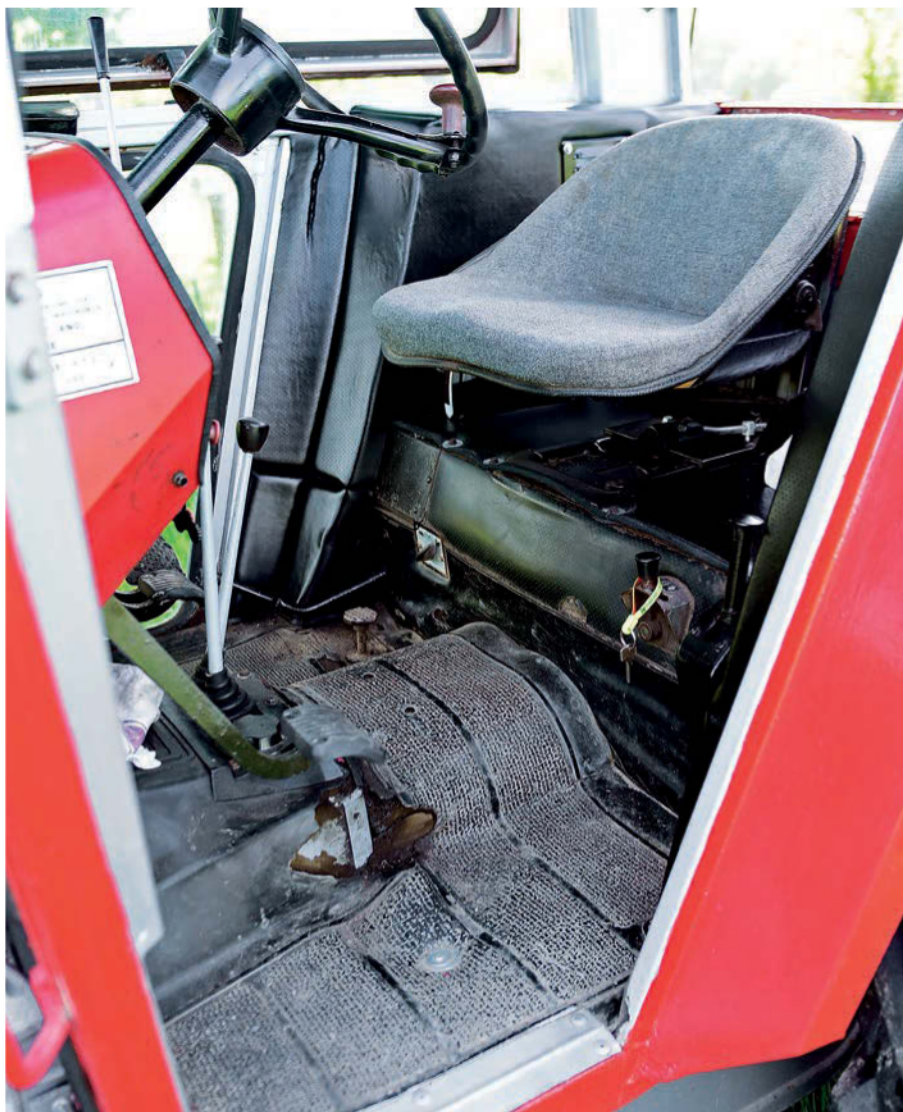
It was the tractor's cab that demanded the most attention during the restoration. The interior was re-clad, and the original, broken seat was replaced with a 'new' secondhand one.
