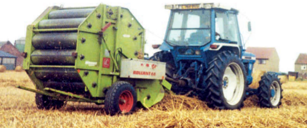
Claas adopted a different approach with its fixed-chamber balers, the first of which were the Rollant machines from 1977. This Rollant 44 was a very popular model during the late 1970s and early '80s in the UK. Note the two metal ramps at the rear that helped to roll the bale further away from the rear door when it opened.
