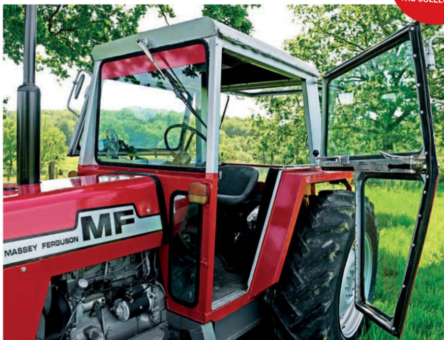
The cab door was badly distorted when the tractor arrived but now sits square and operates perfectly. More improvisation sees lengths of bicycle inner tube used as a door seal.
