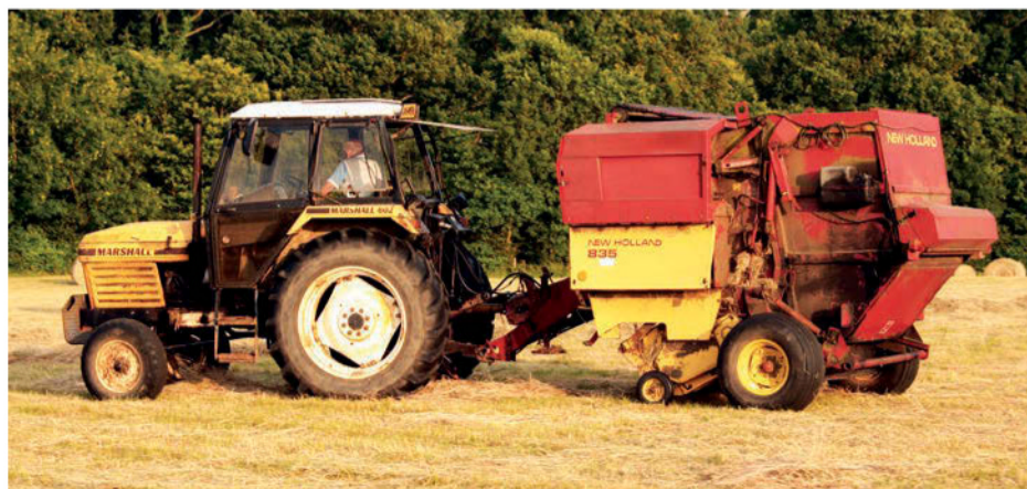
Left: A New Holland 835 baler at work behind a Marshall 802. Its chain and slot bale chamber meant that only one size of bale could be produced. Right: New Holland was a round baler pioneer and this early example is seen in the 1970s, at a farm show in the south of England where it no doubt attracted plenty of interest from farmers. Photo: Kim Parks
