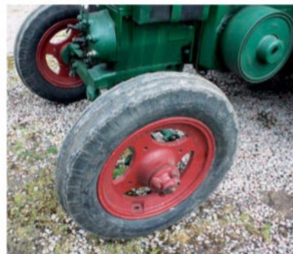
The 12/20's front 19in Dunlop centres should be silver and, although serviceable, the tyres will be changed for a more knobbly-style period tread pattern.
