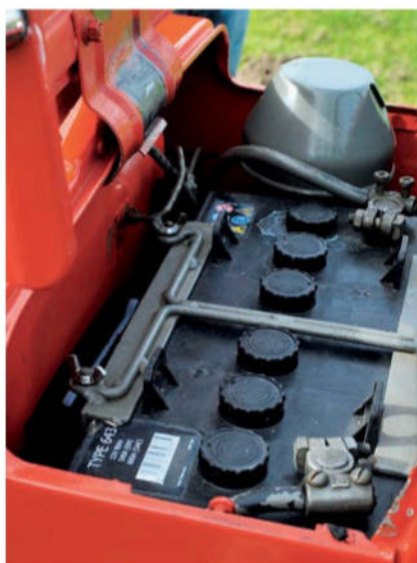
The battery is found beneath a hinged panel towards the rear of the bonnet. The hinges often got broken, and it's quite common for the compartment cover to be missing altogether.
