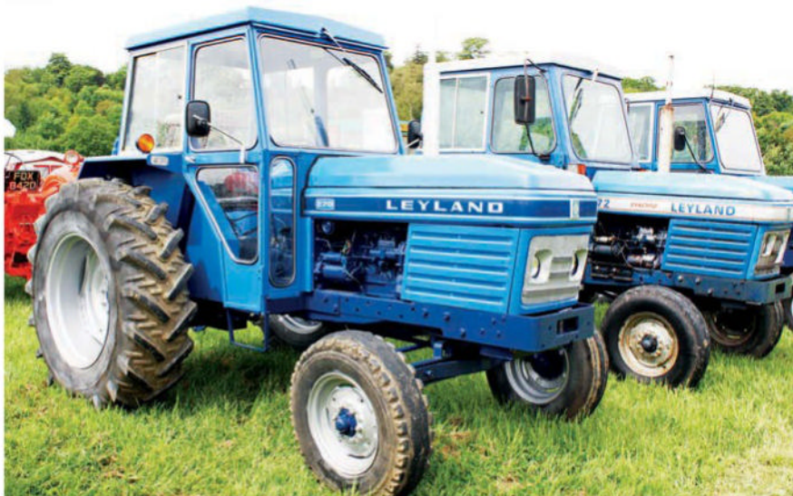
● Powered by the 4/98 engine and with 70hp on tap, the Leyland 270 was the replacement for the 384, but was no longer the flagship of the range.
