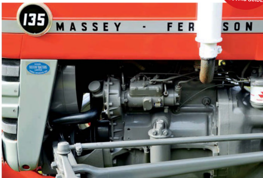
The extremely reliable, 45.5hp, Perkins AD3-152, 2.5-litre, three-cylinder, diesel engine powered most 135s. A petrol model was available with an engine from the Standard Motor Company, but most of those went for export.
