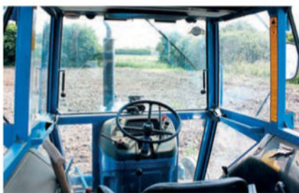
This hard-worked, 85hp, 6610 II is still showing the original, striped upholstery on the seat. The Super-Q cab's flat floor is clear to see. All the main controls are clustered on the right-hand side of the driver's seat.
