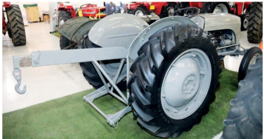
● Ant Bradford's Ferguson TE-20 features an original crane on the back.
