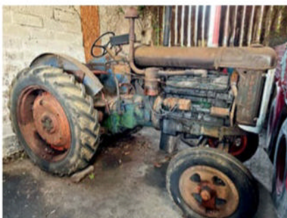
There are a number of Fordson E27Ns being sold, including this very early, green example that was converted during its working life to Perkins P6 power.
