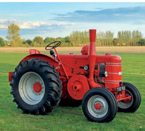
The 3A on light duties to fully bed-in the new big end fitted during its engine rebuild.
