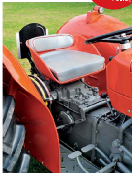
Left: The 135's hydraulics are both reliable and functional. The tractor will happily pull a two-furrow plough. Right: The seat was un-sprung on early 135s, but featured comfortable cushions. The design was updated later in the production run.
