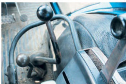
A view from inside a 4610's AP (All Purpose) cab, illustrating the excellent all-round visibility thanks to the slim pillars. The gearbox is operated using floor-mounted levers and an uncluttered dashboard provides tractor information in analogue form. A constant-mesh Dual Power gearbox delivered 16 speeds on the TW range, and was controlled by these two long levers positioned to the right of the driving seat.
