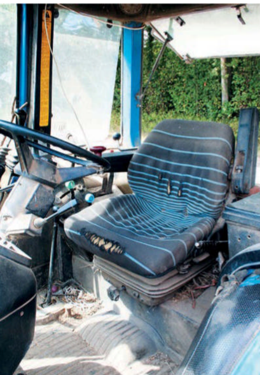
This hard-worked, 85hp, 6610 II is still showing the original, striped upholstery on the seat. The Super-Q cab's flat floor is clear to see. All the main controls are clustered on the right-hand side of the driver's seat.
