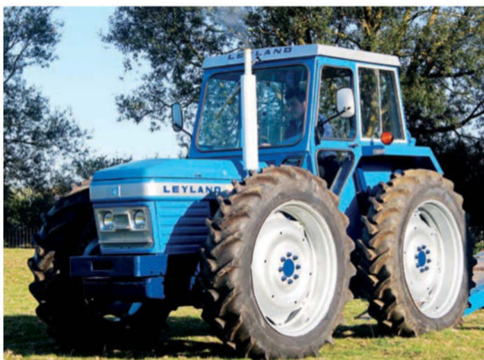
● Left: The four-wheel drive version of the 2100 was the 4100. Leyland gave County Commercial Cars the task of adapting its twin-propshaft design with heavy cast front axle, producing a very purposeful machine. The County parts were assembled on the production line at Bathgate. Right: The new Leyland Golden Harvest range was introduced late in 1980, based heavily on the older models but with improvements such as new brakes. The 262 became the 602 and, as can be seen, it was still available with the old Victor quiet cab (by then called the QM cab).
