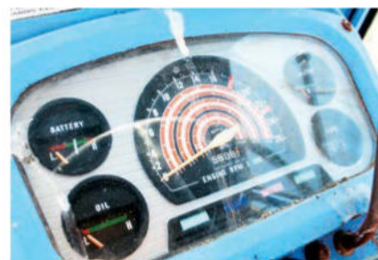
● Since 1967, the same Smiths Instruments dashboard was fitted on the last Nuffield and then all the later Leyland tractors, as shown on this 472. Details about the various engine functions were clearly presented on gauges either side of the main display.
