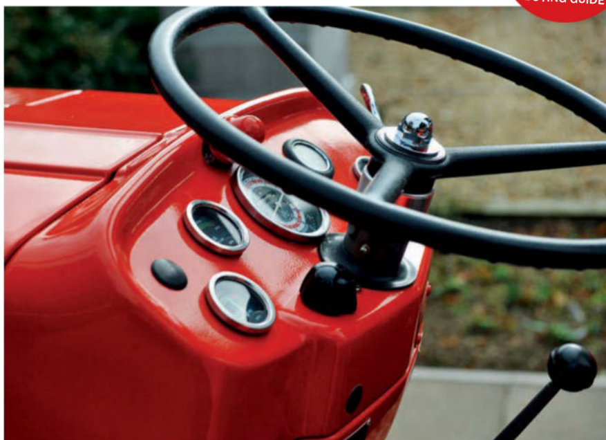
The MF 135 benefitted from a comprehensive instrument array. Note the centrally-placed tractorometer; this was offset to the right on later models. Also, the tractor's all-important serial number is displayed on the riveted-on plate below the instrument cluster, the top of which can just be seen here.
