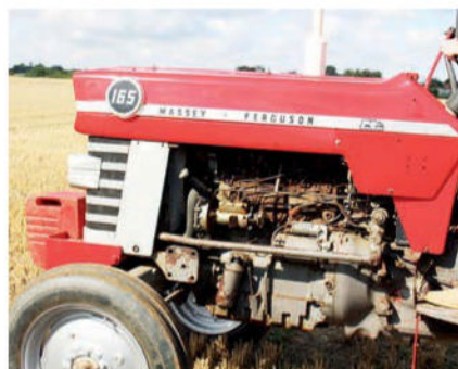
A four-cylinder, 58.3hp Perkins AD4.203 engine lay at the heart of the MF 165. It was the same unit as that used in the earlier MF 65 Mark II.
