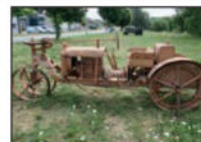
Avery 5-10 Friction Drive - 1920 - older restoration
