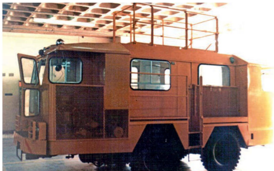
The original photograph of the 'tunnel buggy', taken by its creator, Peter Batistich. Note the platform on the top, allowing engineers to work on the tunnel roof if needed.
