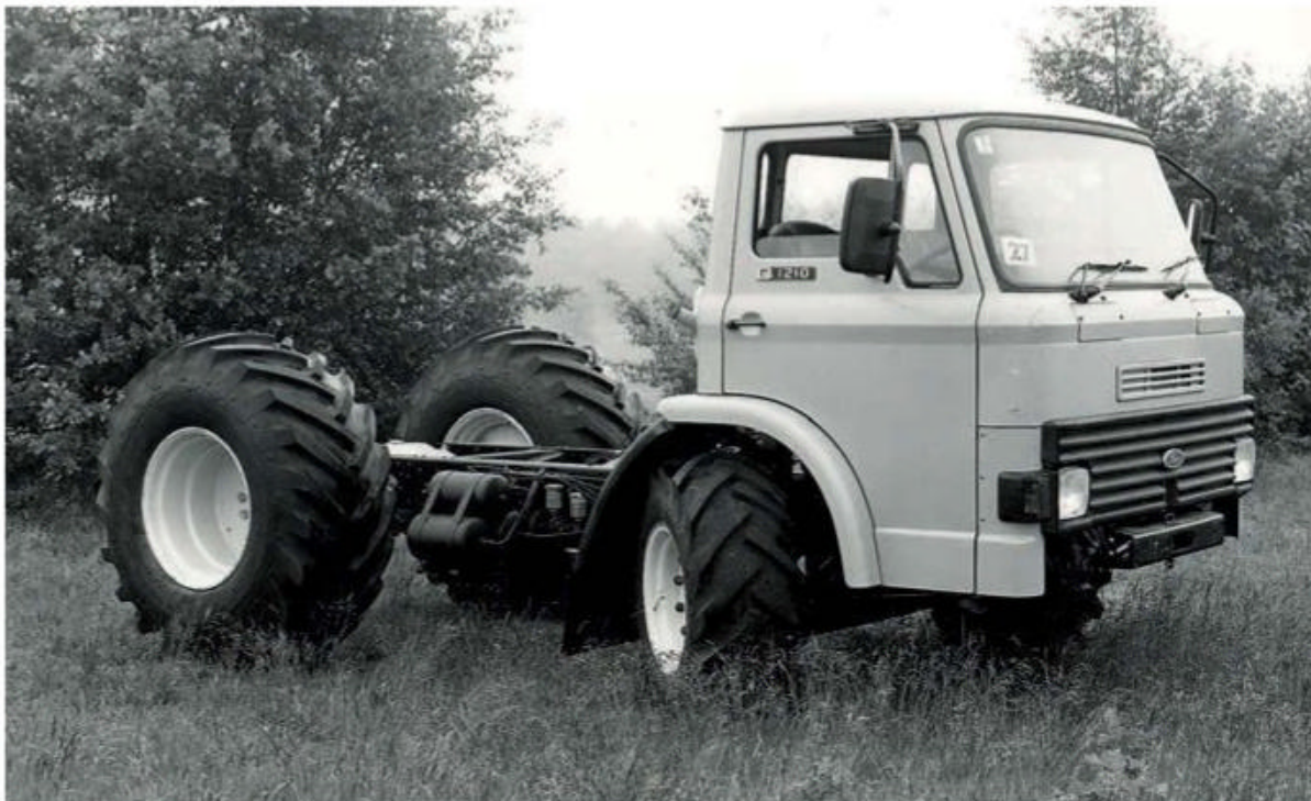
The Tractruck was based heavily on a Ford D Series truck and had a very purposeful stance.
