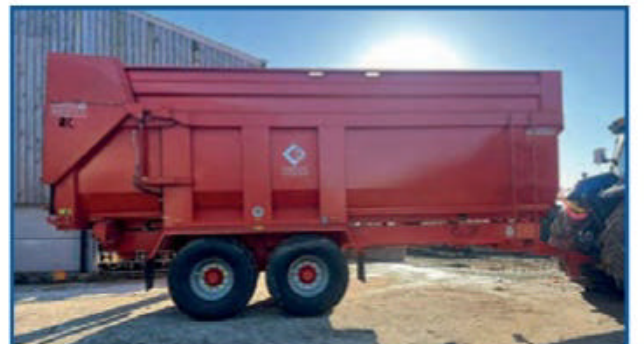
2023 18 Ton Larrington trailer, Harvester model, half pipe internal body, single tipping ram, 560 michelin trailxib tyres, silage sides, 10 stud axles, 406 x 120 brakes, twin line air brakes, single line hydraulic load sensing line, side ladder, hard wood body support blocks Ex Hire unit done very little work £30,000 + VAT
