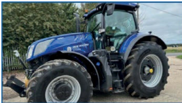
2022 New Holland T7.315 HD, Auto command, 1174hrs, 5 spools + midmounts, front linkage with couplers, front PTO, PLMi cab, full GPS, full spec. 710/70/42's & 600/70/30. £157,000 + vat
