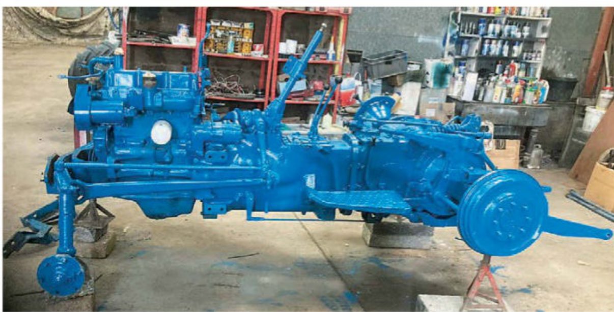
Left: The strip down of the tractor is well underway. Right: Ford Blue two-pack paint starts to go on.
