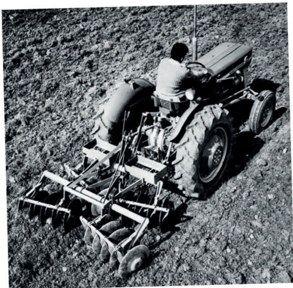
The Massey Ferguson 722 is one of the most recognisable mounted disc harrows produced. Easily adjustable from the driver's seat, gang angles could be changed in four-degree increments from 0-20 degrees, and working widths were 6ft, 7ft, or 8ft. 18in-diameter discs, at 6½in spacing, were standard across the board, with plain and scalloped available. The two largest models were category I and II.
