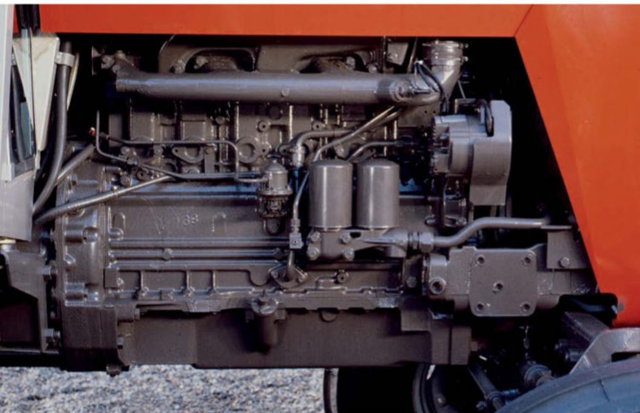
At the heart of the 2000 Series was Perkins' proven six-cylinder unit – the 6.3544. The two smallest models were naturally aspirated, while the 2680 (seen here) and 2720 used a turbocharged version. The largest model also featured a charge cooler. Photo: AGCO.
