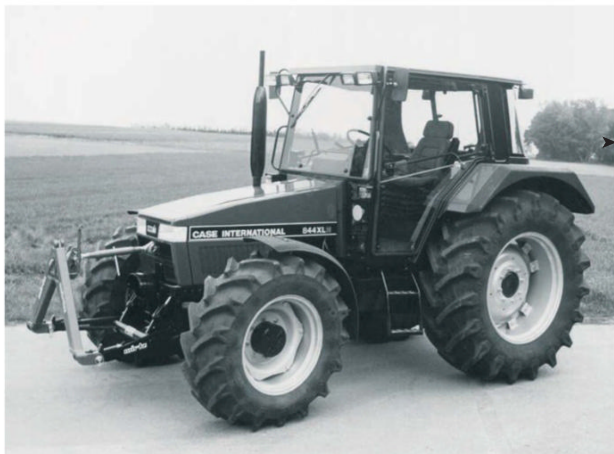
Featuring a front linkage capable of lifting two tonnes, a front PTO, and the famous ‘drop nose’ that became available on ‘Plus’ models, this ‘ultimate’ version of the Case IH 844XLN had a list price of £36,995 in 1993.
