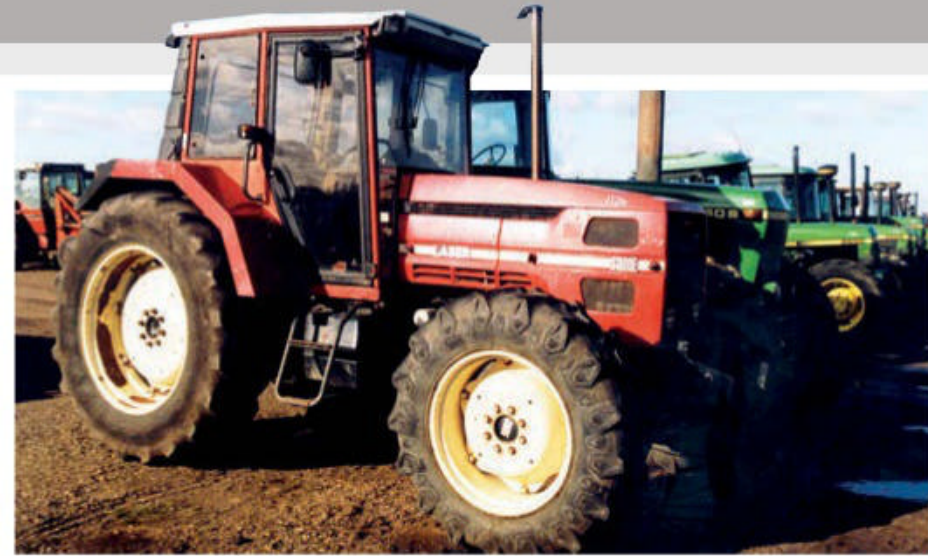
The SAME Laser was the red equivalent to the Lamborghini '6 Line' and shared many components, such as the cab. The engines, however, were very different, as the range used SAME air-cooled diesel engines and the smallest, the 100, was a five-cylinder tractor.
