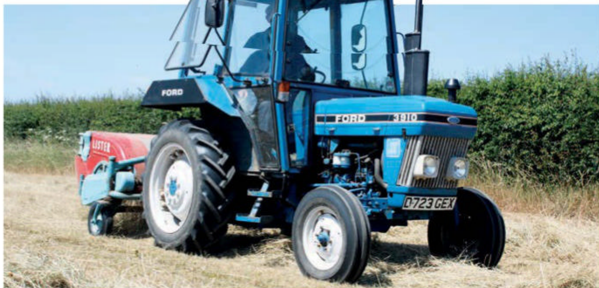
Rated at 47hp (DIN), the 3910 is well suited to tasks such as this. Photo: Jonathan Whitlam.
