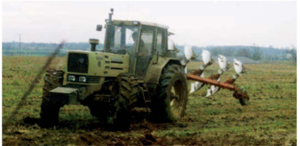
The SAME Laser was the red equivalent to the Lamborghini '6 Line' and shared many components, such as the cab. The engines, however, were very different, as the range used SAME air-cooled diesel engines and the smallest, the 100, was a five-cylinder tractor.
