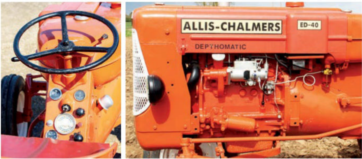
Left: The dashboard of the ED-40 was neatly positioned on the raked section under the steering wheel, with all the necessary instruments included. Note how narrow the tractor is here, just in front of the driving seat. Right: The engine chosen was a Standard Motor Company 23C, four-cylinder diesel engine of 2.3-litre capacity. It produced 37hp before being tweaked to give 41hp during the ED-40's third year of production. This engine was tried and tested, as it was used in Ferguson and MF tractors, but it had a reputation of being difficult to start from cold.
