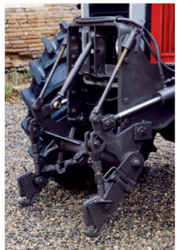
The 2000 Series was Massey Ferguson's first range to be offered with the option of a front linkage and PTO. Photo: AGCO.
